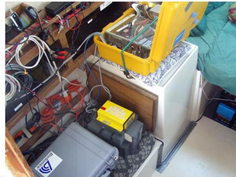
Figure 1. The critical settings used for the BioSonics DT-X echosounder (Table). Swing-arm in traveling position with 420 kHz (top) and 38 kHz (bottom) transducers and Trimble antenna (Upper Image). Inside V-Berth of survey vessel with (left-to-right) BioSonics DT-X echosounder, Trimble receiver, and acquisition PC (Lower Image).
