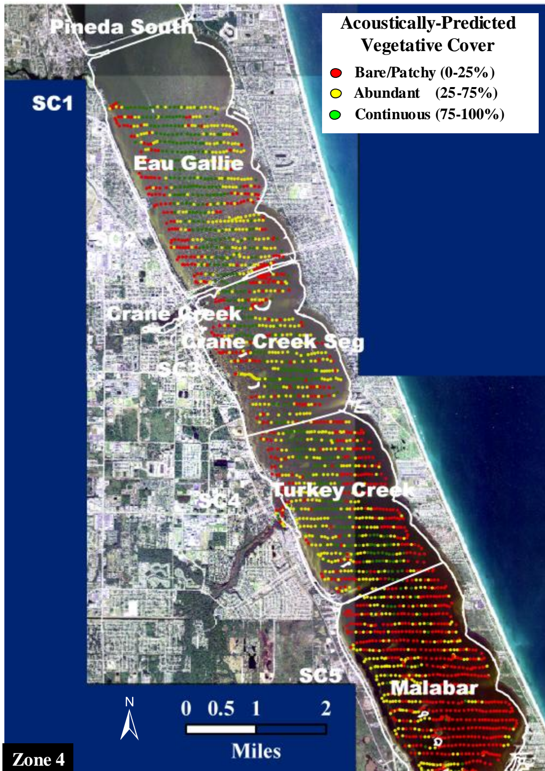
Appendix B 5. 2005 QTC View 200 kHz survey. Actual trackplot of acoustic classifications, based on blocks of twenty records. Red is bare/patchy cover, yellow is abundant cover, and green is continuous cover. Vegetative cover includes both branched and bladed morphologies.
