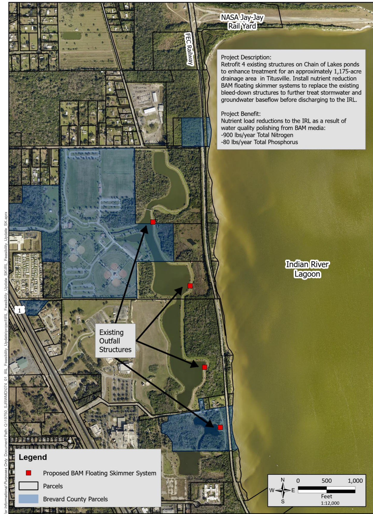
Figure 4-3 Chain of Lakes Enhanced Nutrient Reduction – Alternative 1
