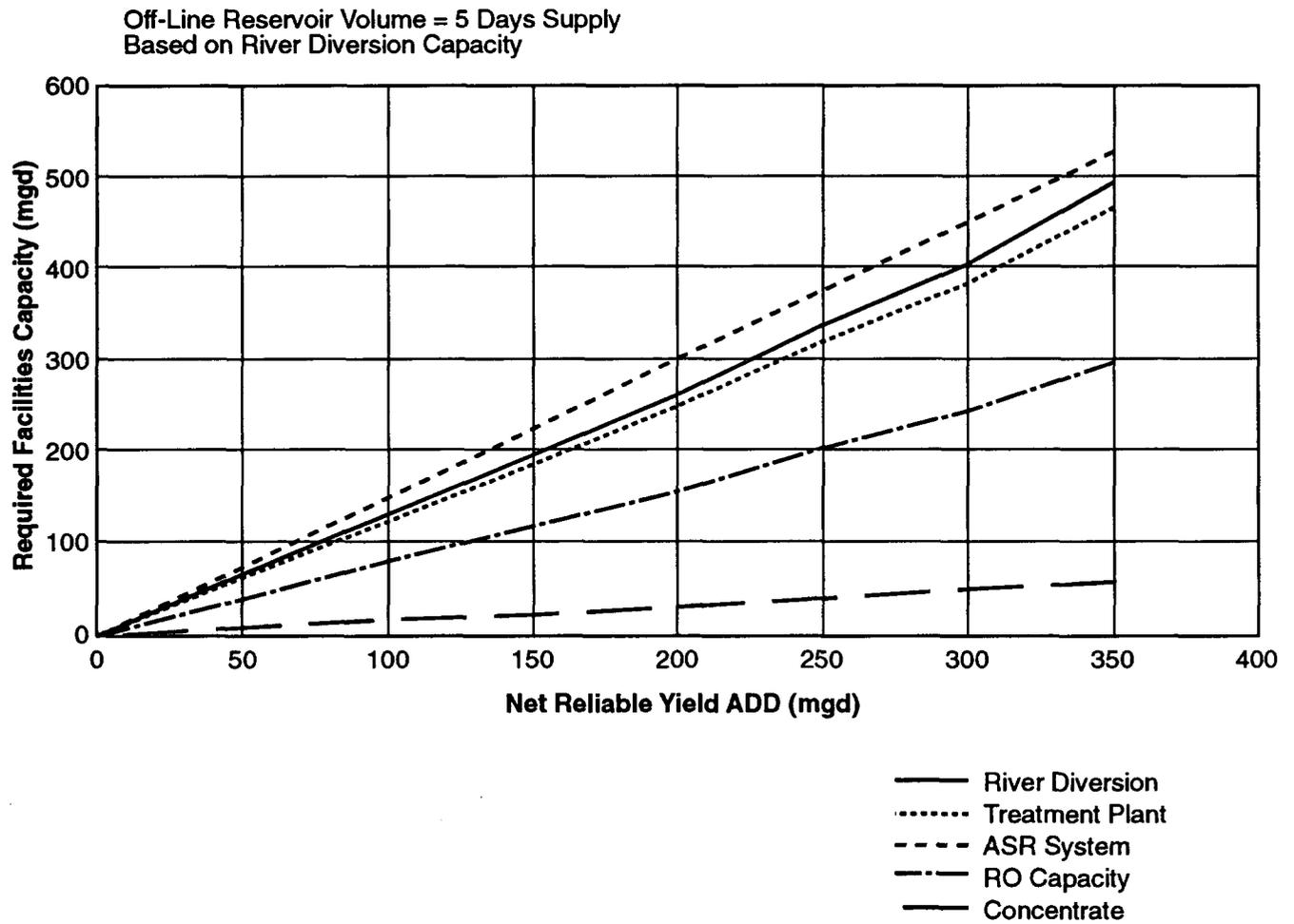
Figure 26. Surface Water Facility Requirements for St. Johns River near De Land.
