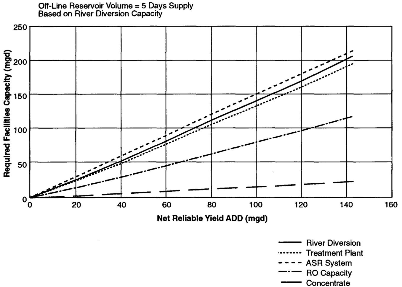
Figure 24. Surface Water Facility Requirements for St. Johns River near Titusville.
