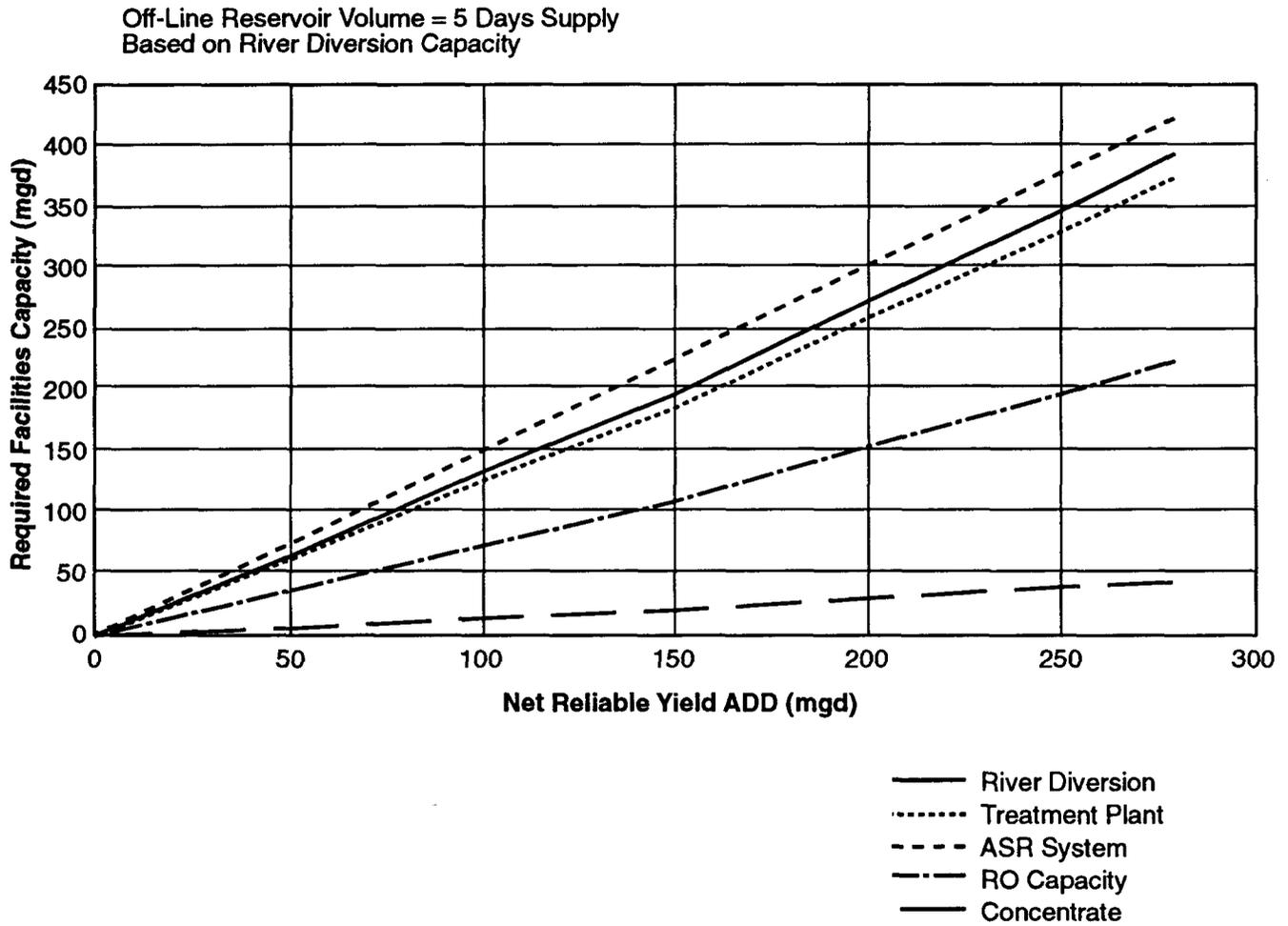
Figure 25. Surface Water Facility Requirements for St. Johns River at Sanford.
