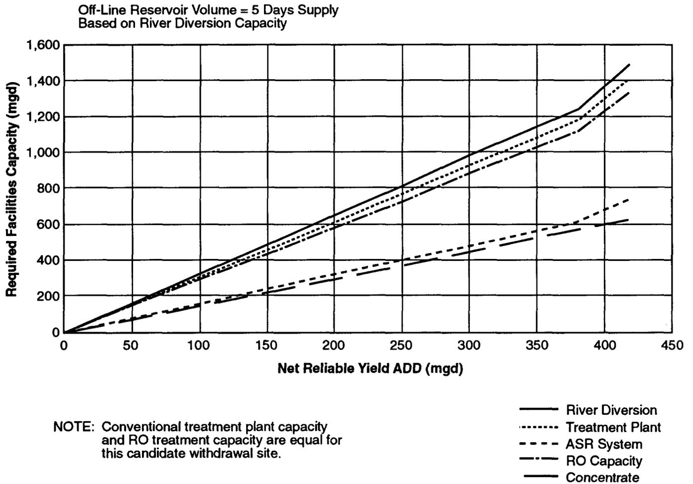
Figure 27. Surface Water Facility Requirements for St. Johns River above Jacksonville.
