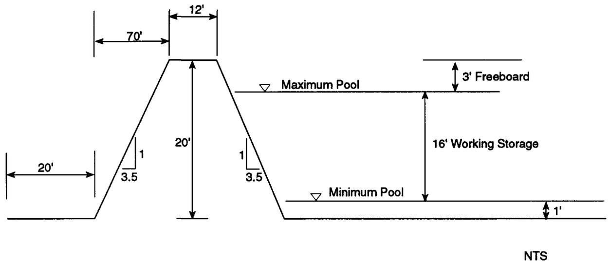
**Figure 4. Typical Section of Off-Line Storage Perimeter Levee.**
