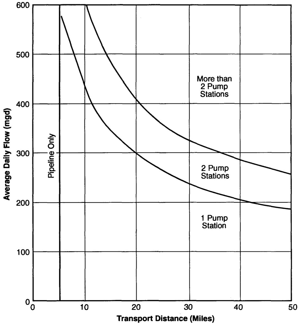
**Figure 7. Criteria for Selection of Appropriate Number of Pumping Stations**
