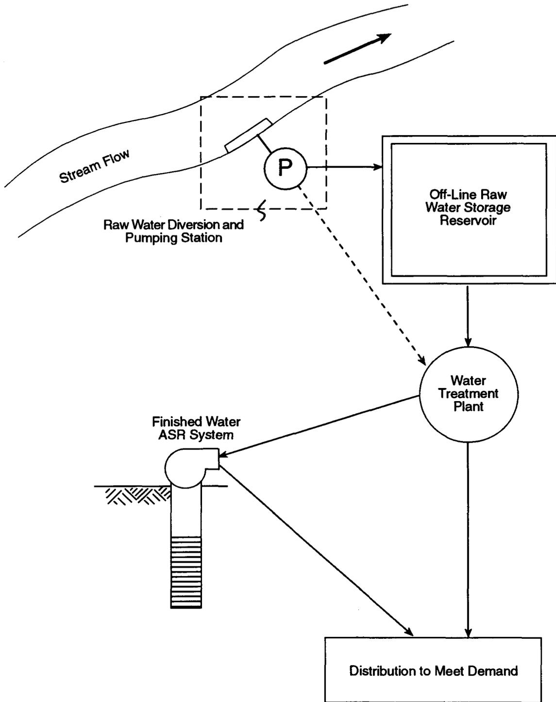
**Figure 1. Facilities Required to Develop Reliable Surface Water Supply to Meet Urban Demands.**
