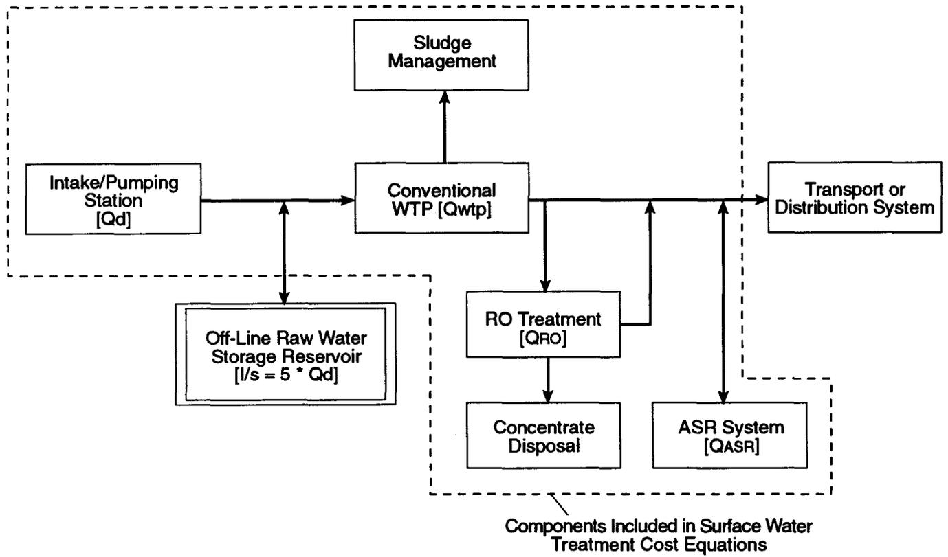
**Figure 5. Major Components of Complete Surface Water Supply Storage and Treatment System.**
