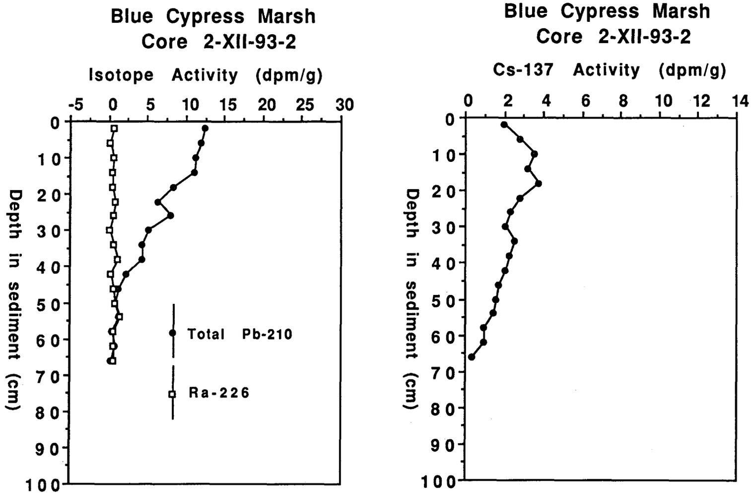
Figure 56. Blue Cypress Marsh Core 2-XII-93-2 total  $^{210}\text{Pb}$  &  $^{226}\text{Ra}$  activity ( $\text{dpm g}^{-1}$  dry) and  $^{137}\text{Cs}$  activity ( $\text{dpm g}^{-1}$  dry).
