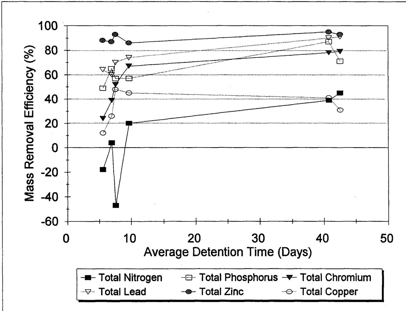
Figure 5-1. Effects of Detention Time on Overall Mass Removal of Selected Parameters in the DeBary Detention with Filtration Pond.
