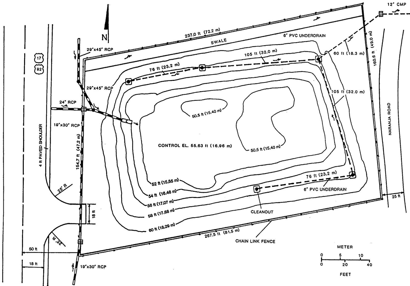
Figure 3-3. Drainage and Pond Details for the DeBary Detention with Filtration Site.
