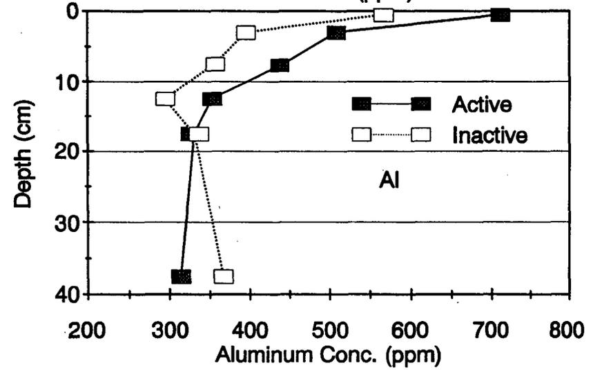
Figure 4-17. Comparison of Sediment Concentrations of Chromium, Iron, Manganese and Aluminum in the Top 50 cm of Active and Inactive Filter Areas at the DeBary Detention with Filtration Site.
