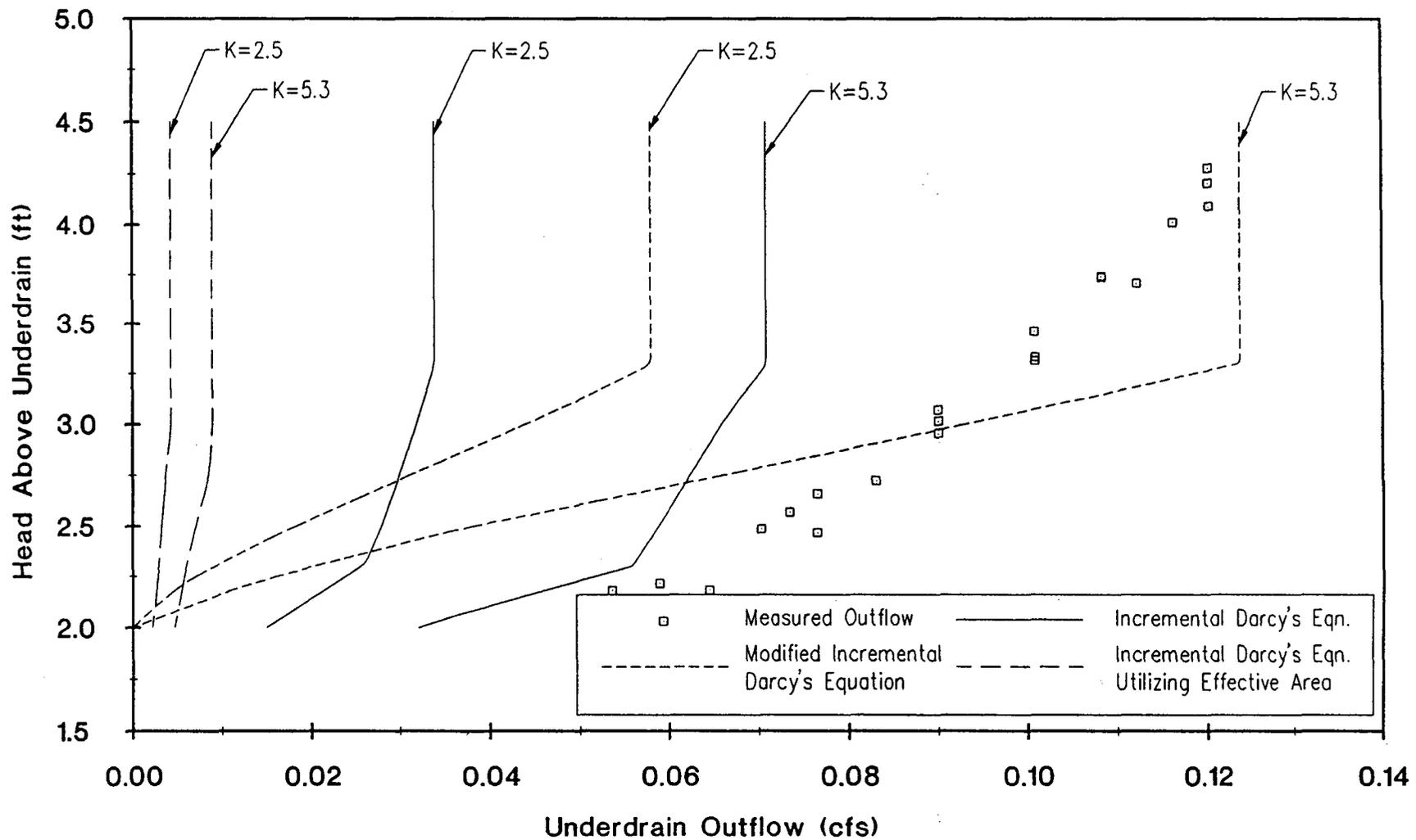
Figure 4-30. Comparison of Measured and Calculated Drawdown Curves for a Side Bank Filter with 20-30 Silica Sand Media.
