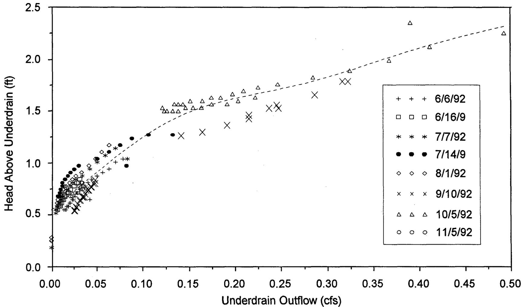
Figure 4-23. Filter Drawdown Characteristics of Selected Storm Events in June-November at the DeBary Research Site.
