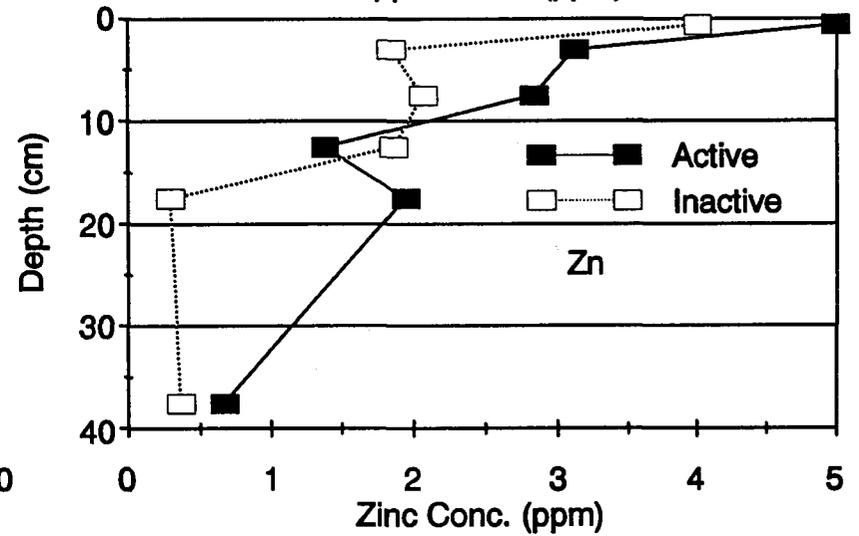
Figure 4-16. Comparison of Sediment Concentrations of Cadmium, Copper, Lead and Zinc in the Top 50 cm of Active and Inactive Filter Areas at the DeBary Detention with Filtration Site.
