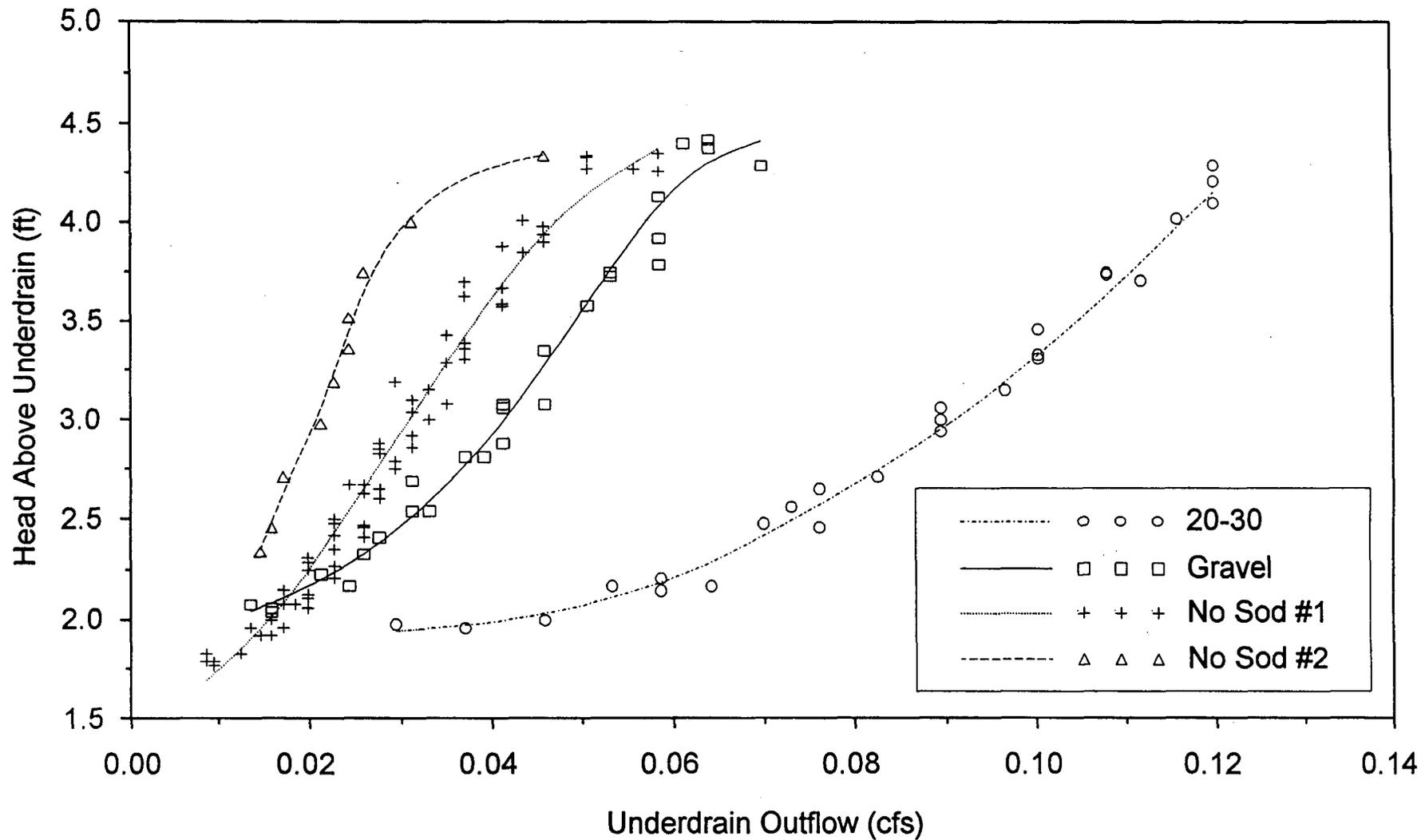
Figure 4-25. Measured Drawdown Characteristics of Various Side Bank Filter Configurations with No Sod Cover.
