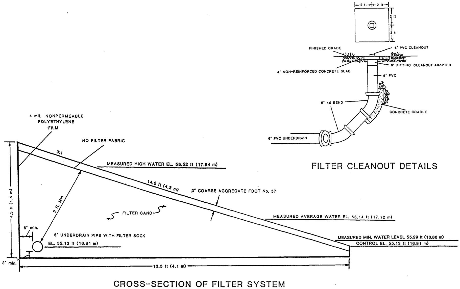
Figure 3-4. Filter Details for the Side Bank Filter System at the DeBary Detention with Filtration Pond Site.
