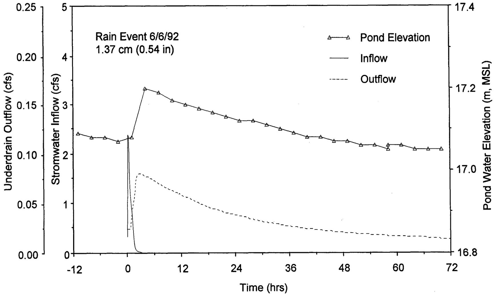
Figure 4-19. Relationships Between Inflow, Outflow and Pond Stage for a 1.37 cm (0.54 in) Rain Event on June 6, 1992.
