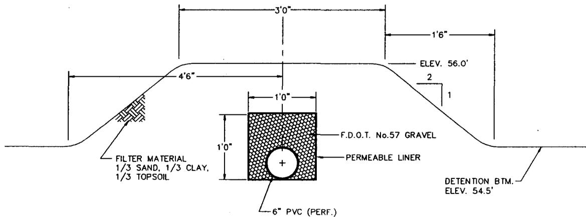
**CROSS-SECTION OF FILTER BERM**
