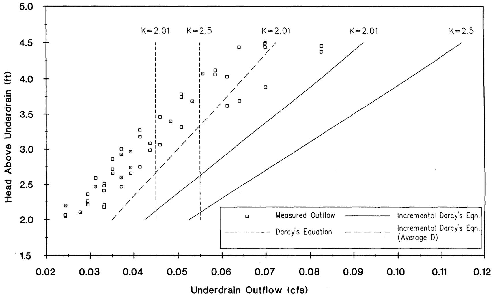
Figure 4-27. Comparison of Measured and Calculated Drawdown Curves for the Vertical Bottom Filter with No Sod Cover.
