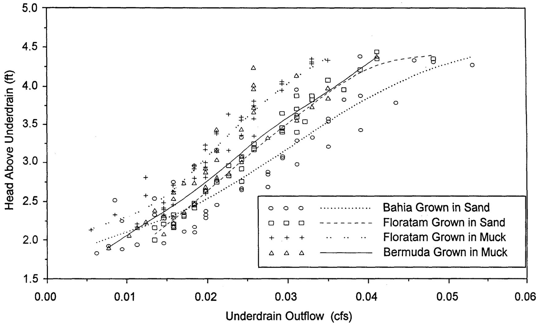
Figure 4-26. Measured Drawdown Characteristics of a Side Bank Filter Covered with Various Sod Types.
