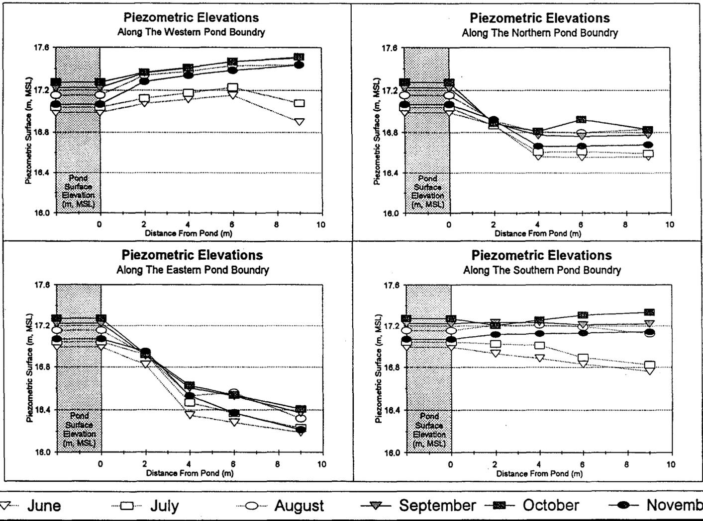
Figure 4-2. Horizontal Piezometric Gradients Along the West, East, North and South Sides of the DeBary Detention Pond.
