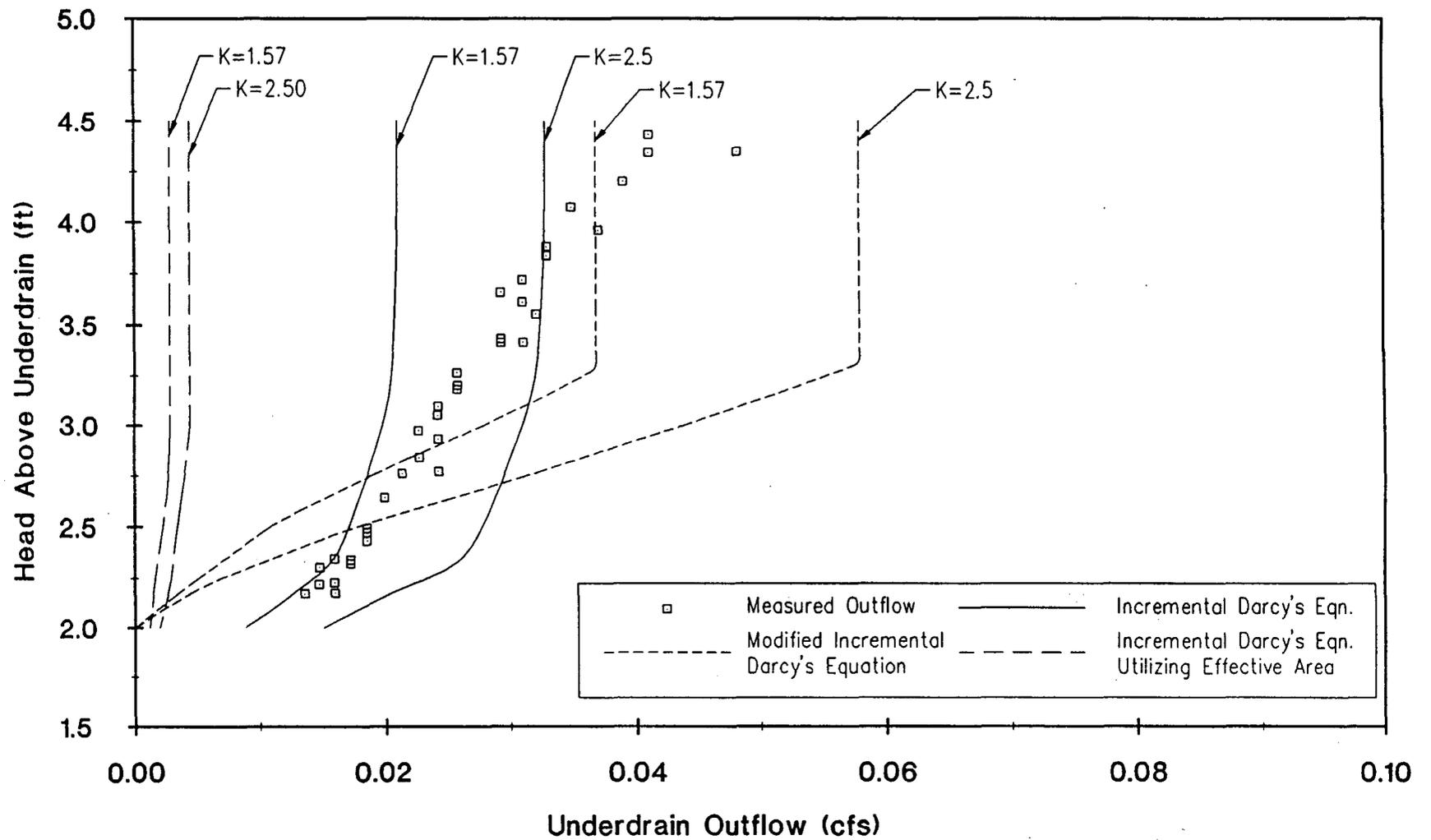
Figure 4-32. Comparison of Measured and Calculated Drawdown Curves for a Side Bank Filter Covered with St. Augustine Sod Grown in Sand.
