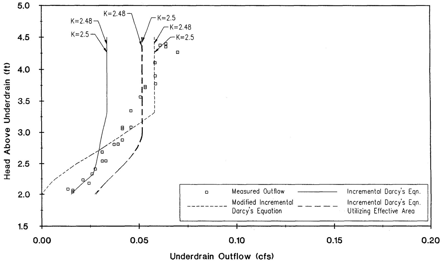
Figure 4-29. Comparison of Measured and Calculated Drawdown Curves for a Side Bank Filter with a Gravel Envelope Around the Underdrain Pipe.
