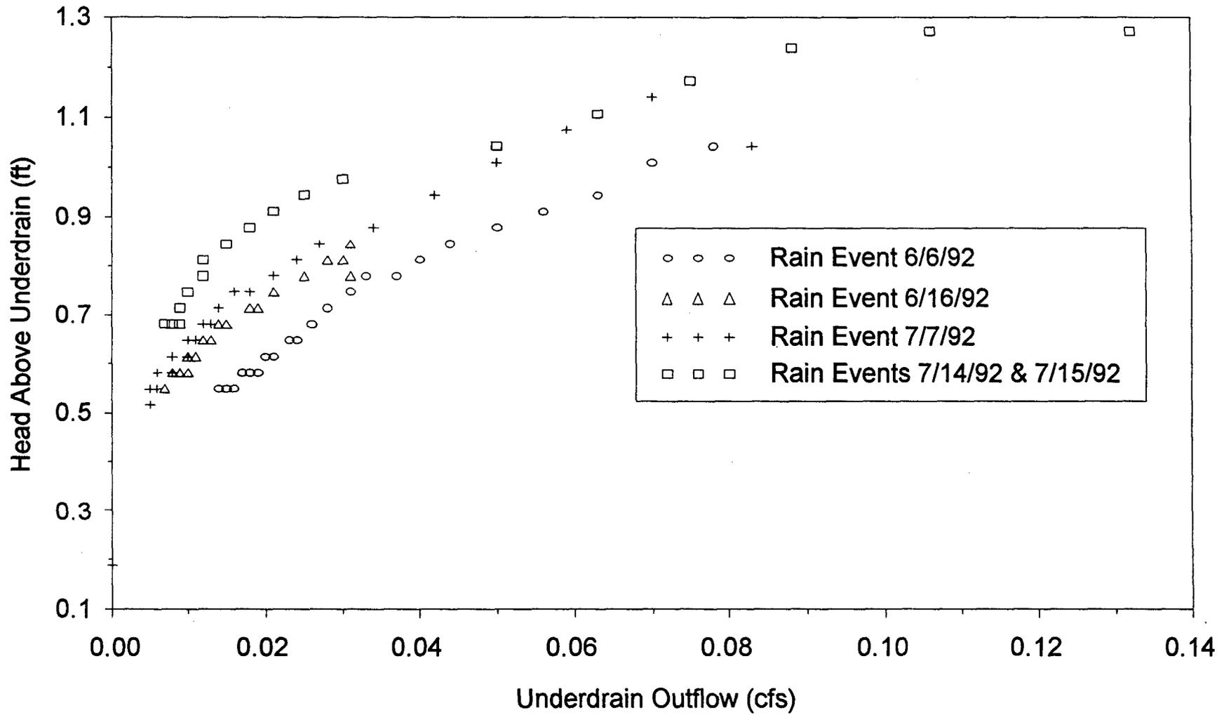
Figure 4-22. Filter Drawdown Characteristics of Selected Storm Events in June-July at the DeBary Research Site.
