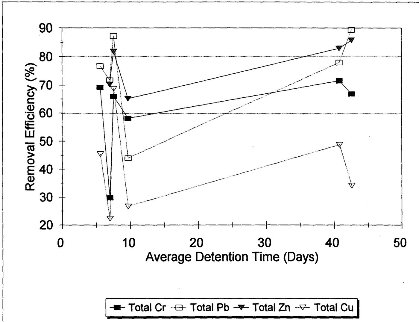
Figure 5-3. Effects of Pond Detention Time on Removal of Total Chromium, Lead, Zinc and Copper within the Pond.
