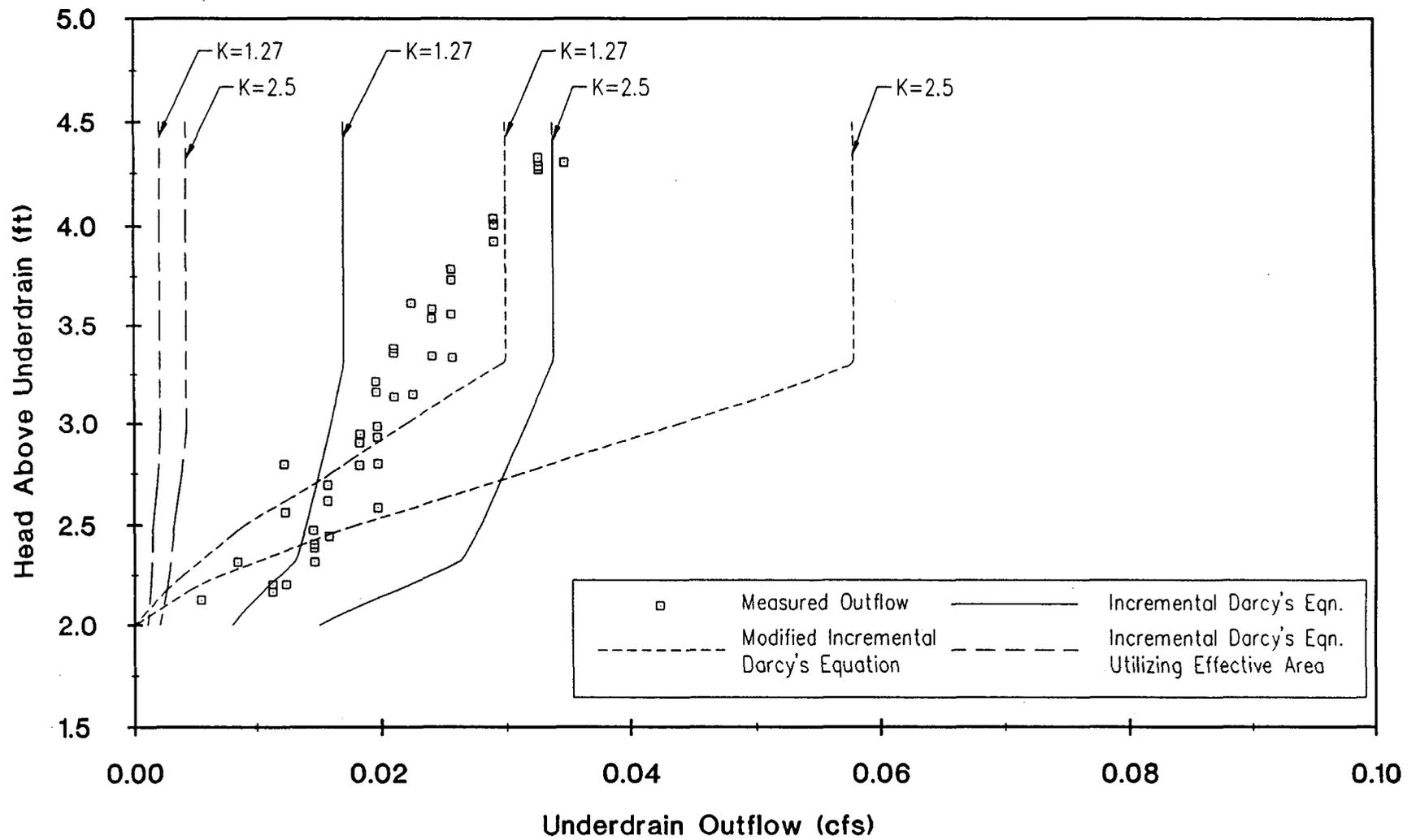
Figure 4-33. Comparison of Measured and Calculated Drawdown Curves for a Side Bank Filter Covered with St. Augustine Sod Grown in Muck.
