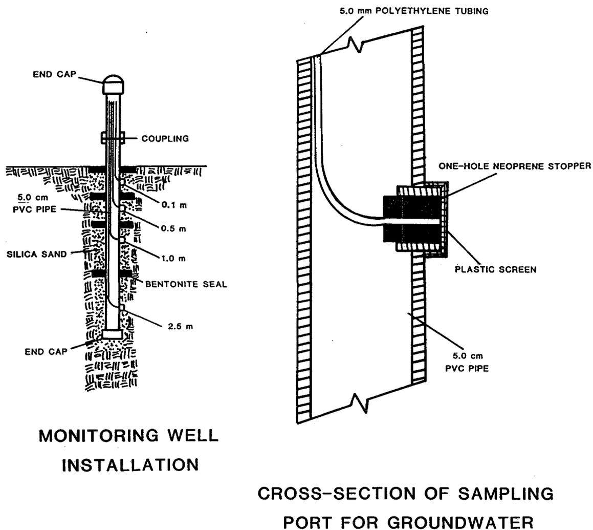
Figure 3-6. Schematic of a Typical Multiport Monitoring Well.
