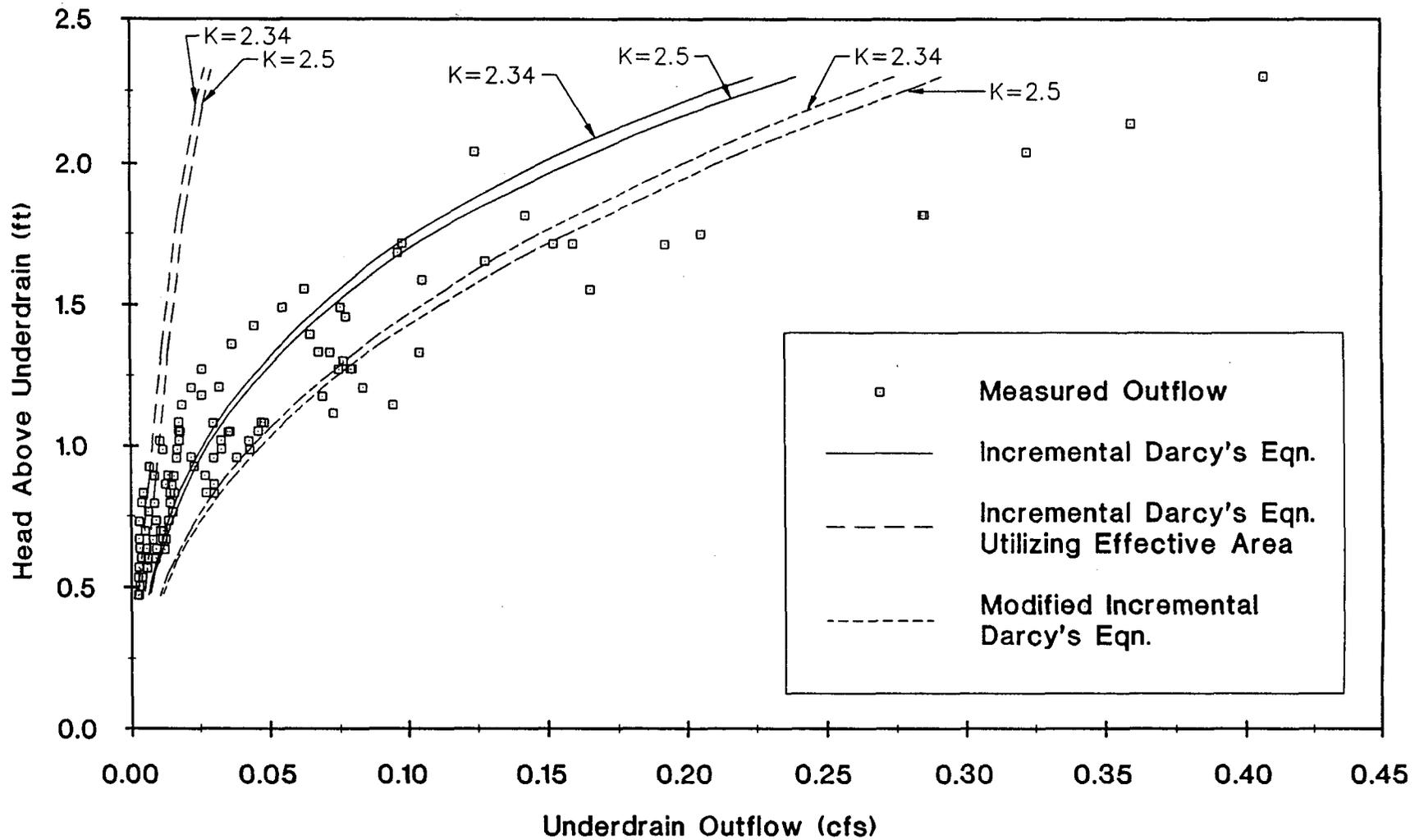
Figure 4-24. Comparison of Measured Drawdown at the DeBary Detention with Filtration Site and Calculated Drawdown Using Common Design Equations.
