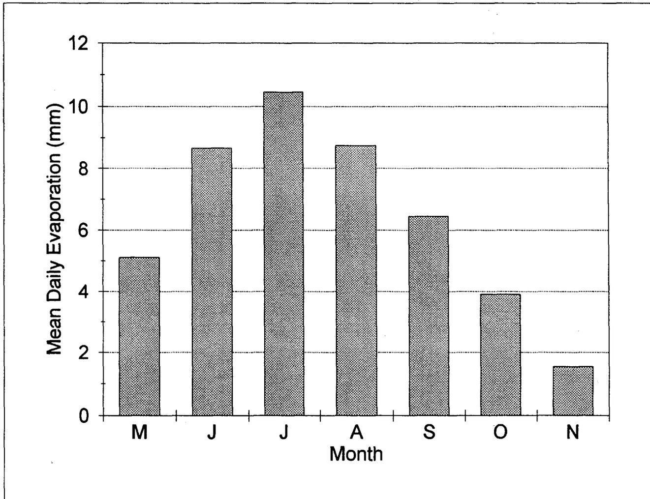
Figure 4-5. Mean Daily Evaporative Losses Measured at the DeBary Research Site from May to November 1992.
