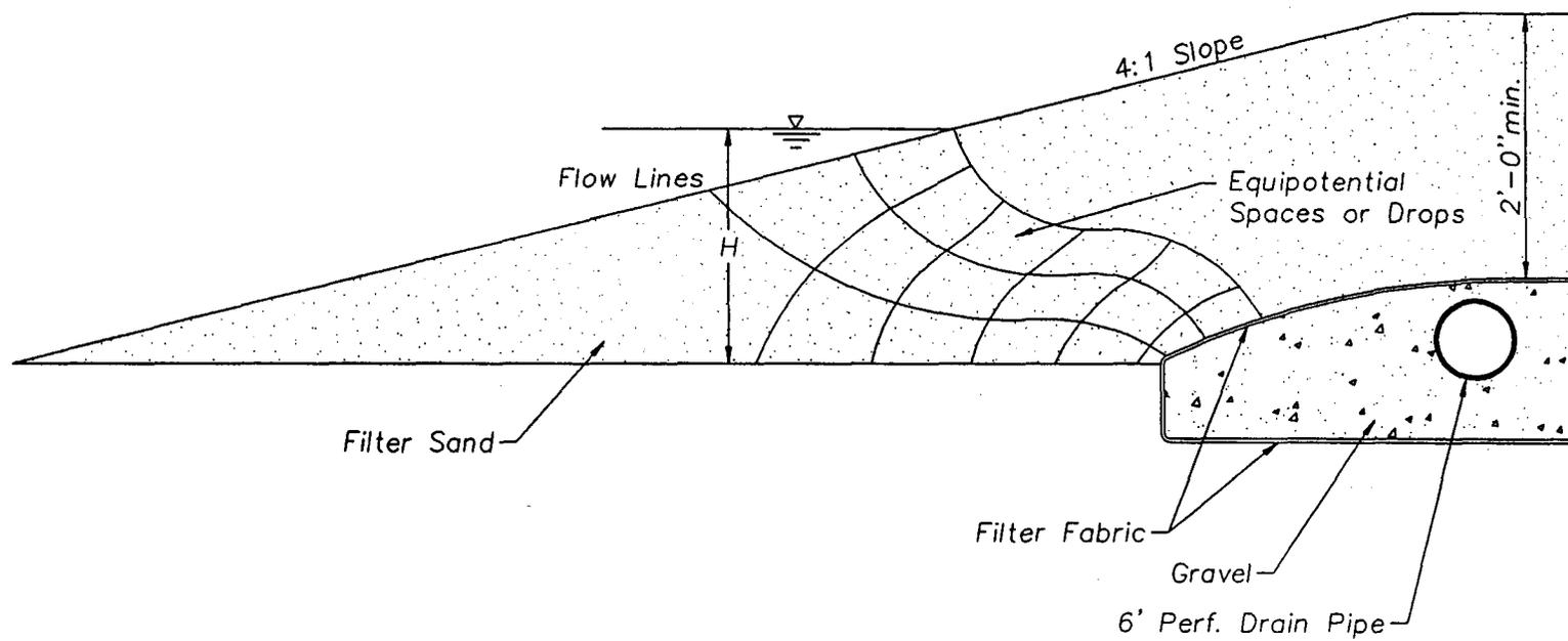
Figure 2-6. Flow Net Diagram Illustrating Lines of Seepage Through a Typical Side Bank Filtration System.
