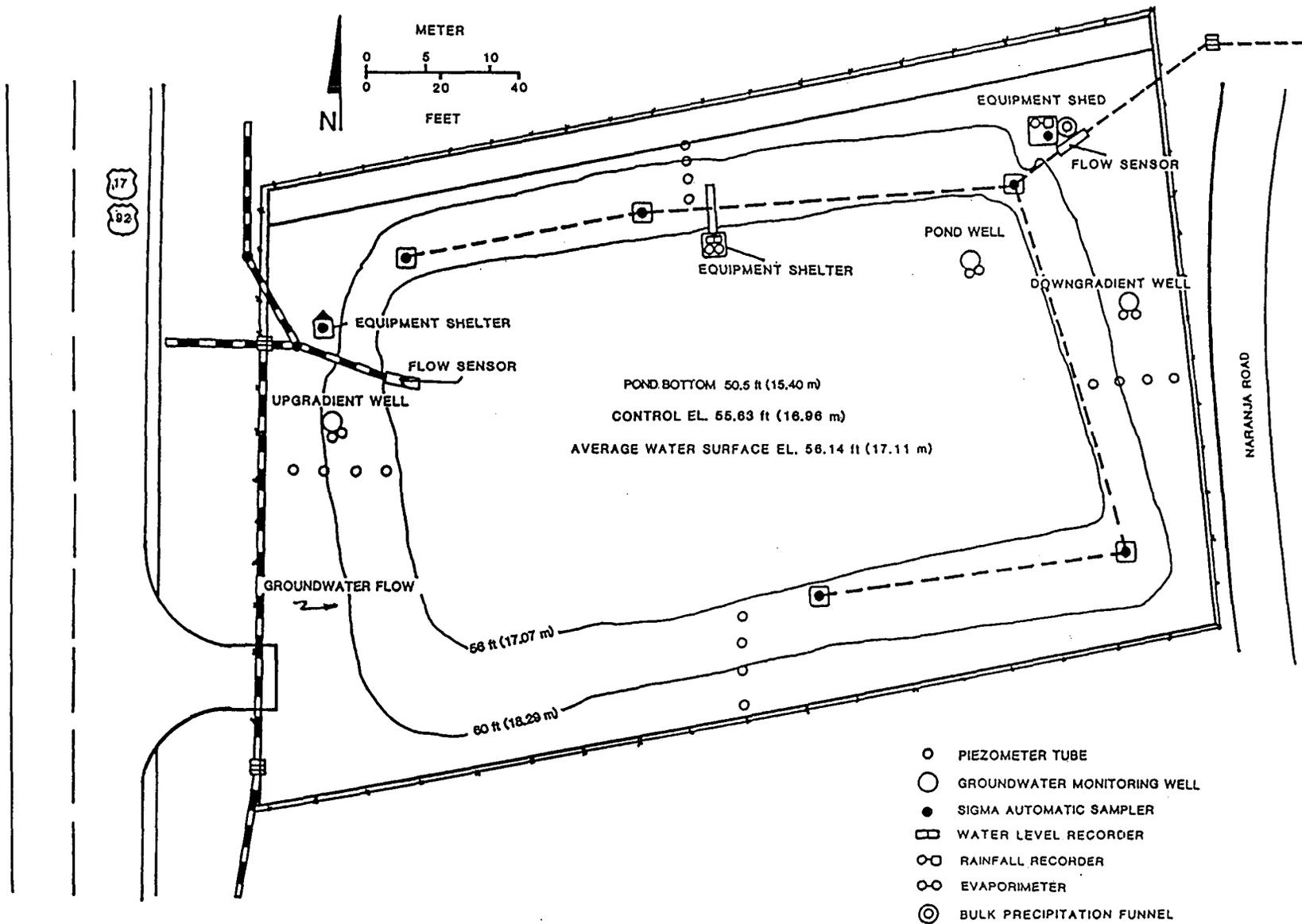
Figure 3-5. Field Instrumentation Used at the DeBary Detention with Filtration Pond Site.
