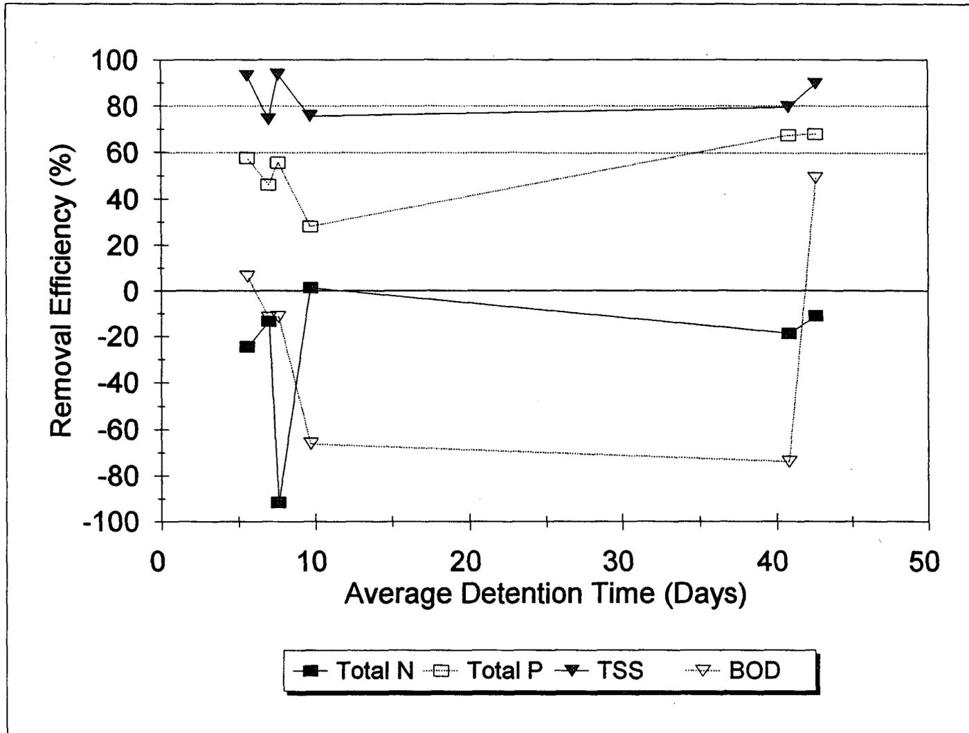
Figure 5-2. Effects of Pond Detention Time on Removal of Total Nitrogen, Total Phosphorus, TSS and BOD within the Pond.
