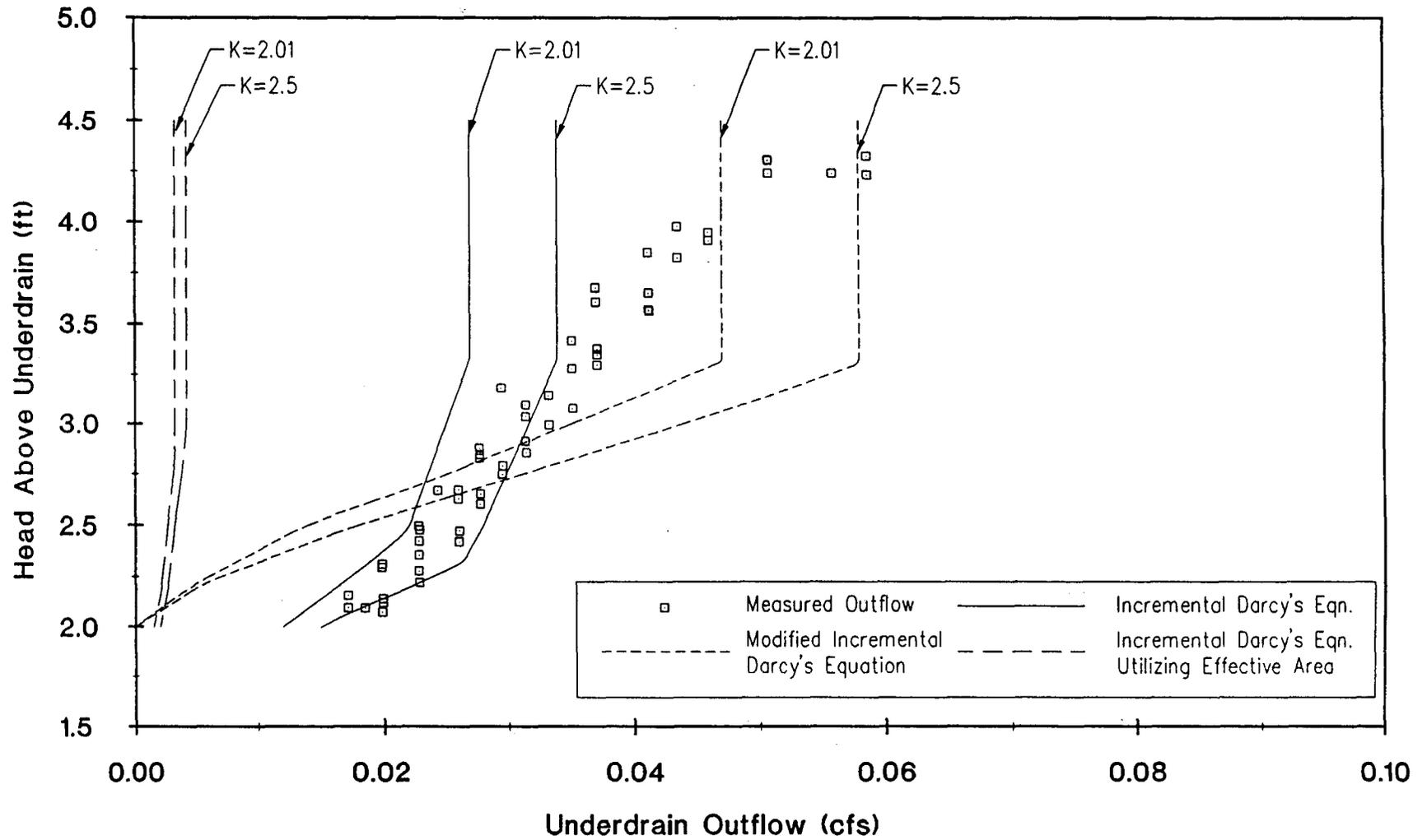
Figure 4-28. Comparison of Measured and Calculated Drawdown Curves for a Side Bank Filter with No Sod Cover.
