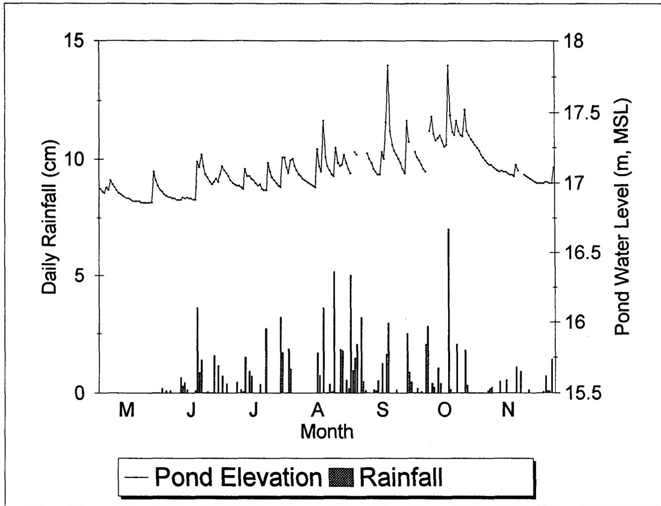
Figure 4-1. Relationships Between Rainfall and Pond Surface Elevation at the DeBary Research Site.
