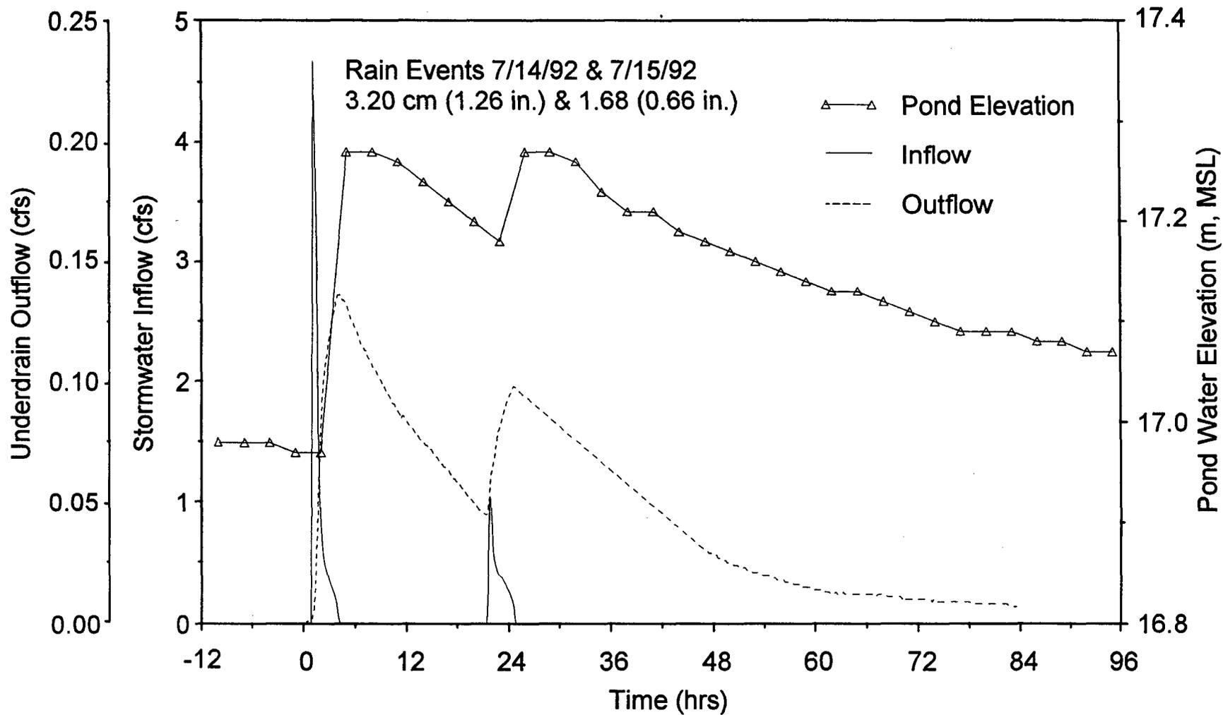
Figure 4-21. Relationships Between Inflow, Outflow and Pond Stage for Sequential Rain Events of 3.20 cm (1.26 in) and 1.68 cm (0.66 in) on July 14-15, 1992.
