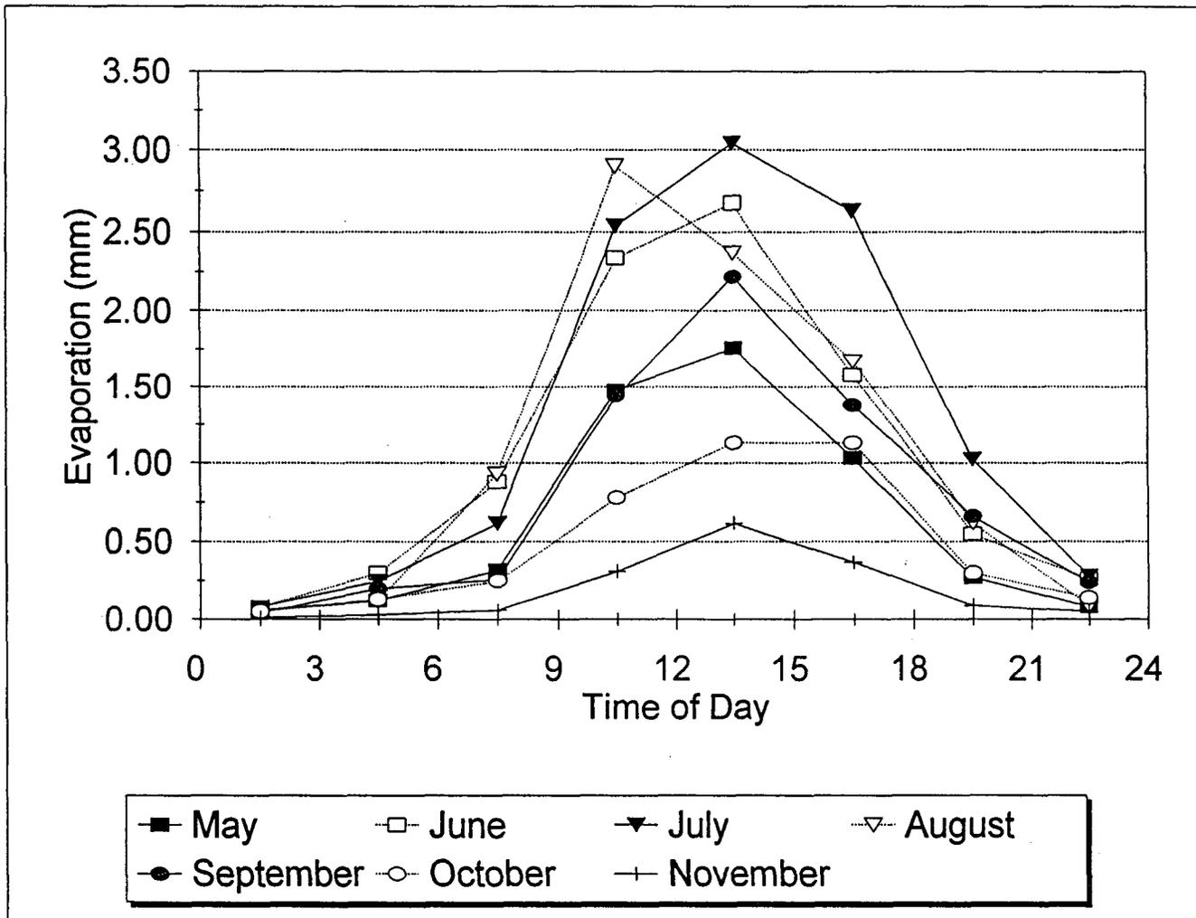
Figure 4-4. Hourly Evaporative Losses Measured at the DeBary Research Site.
