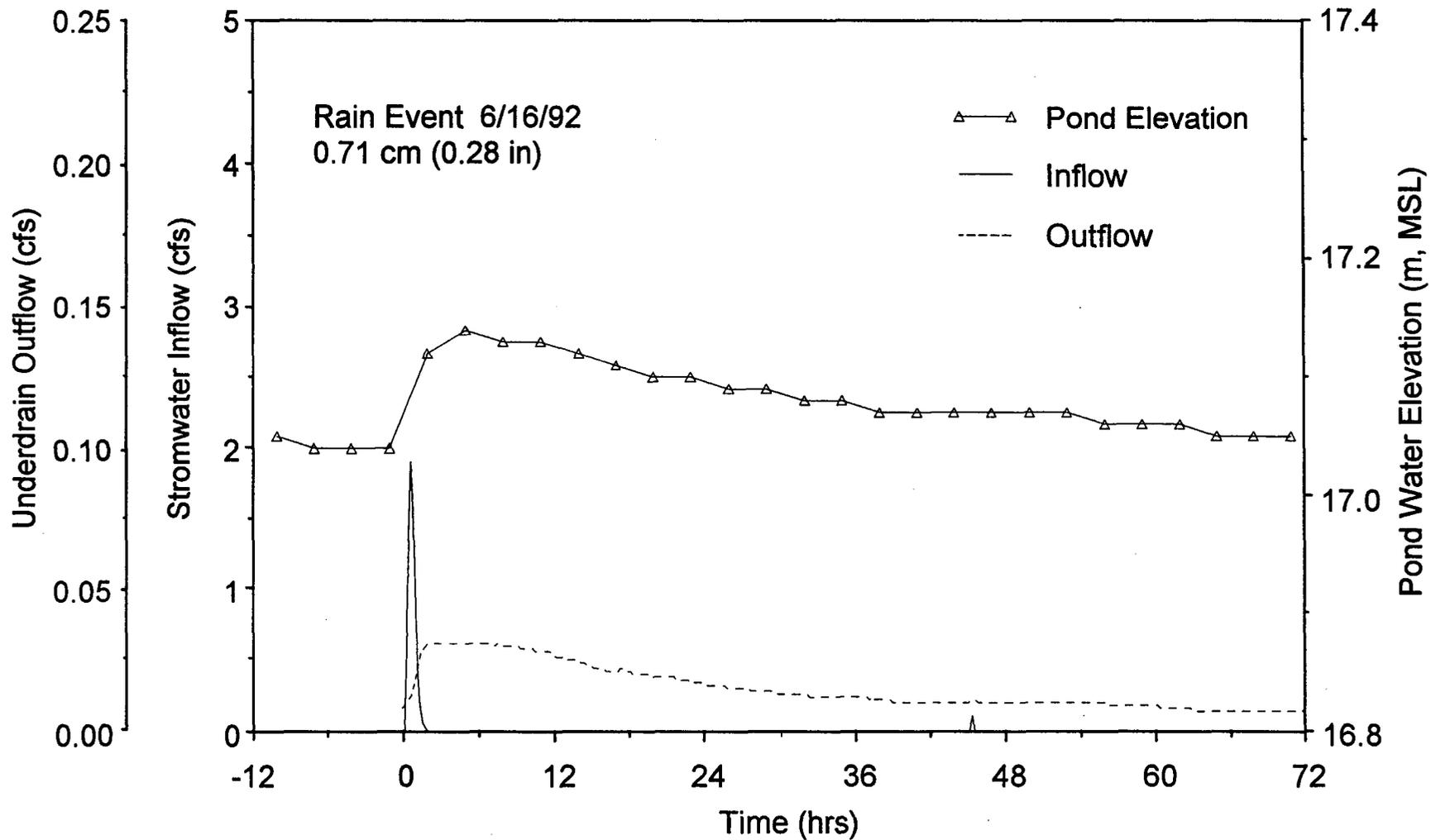
Figure 4-18. Relationships Between Inflow, Outflow and Pond Stage for a 0.71 cm (0.28 in) Rain Event on June 16, 1992.
