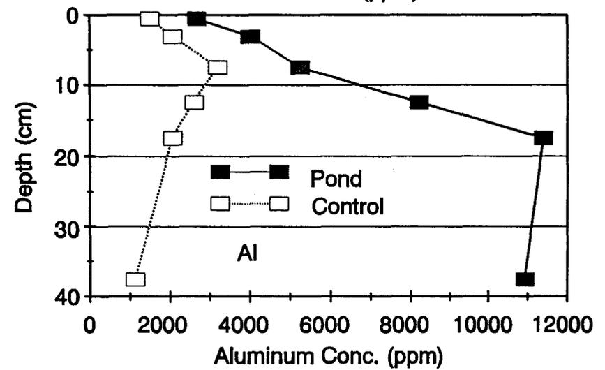
Figure 4-14. Comparison of Sediment Concentrations of Chromium, Iron, Manganese and Aluminum in the Top 50 cm of Pond and Control Areas at the DeBary Detention with Filtration Site.
