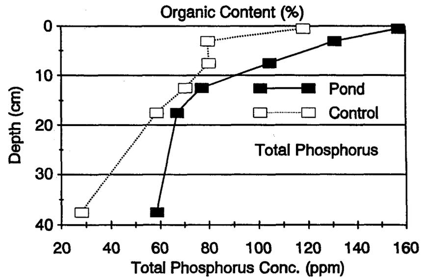
Figure 4-12. Comparison of Sediment Concentrations of Moisture Content, Organic Content, Total Nitrogen, and Total Phosphorus in the Top 50 cm of Pond and Control Areas at the DeBary Detention with Filtration Site.
