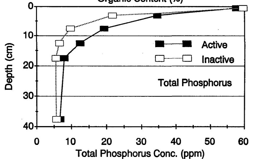
Figure 4-15. Comparison of Sediment Concentrations of Moisture Content, Organic Content, Total Nitrogen and Total Phosphorus in the Top 50 cm of Active and Inactive Filter Areas at the DeBary Detention with Filtration Site.
