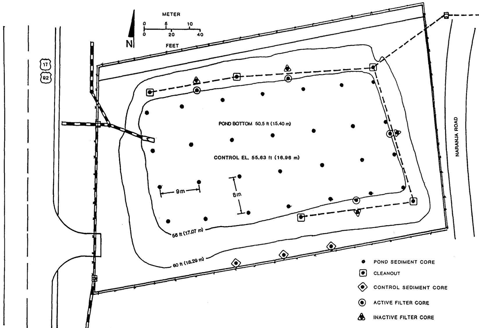
Figure 3-7. Sample Locations for Collection of Soils and Sediments at the DeBary Detention with Filtration Pond Site.
