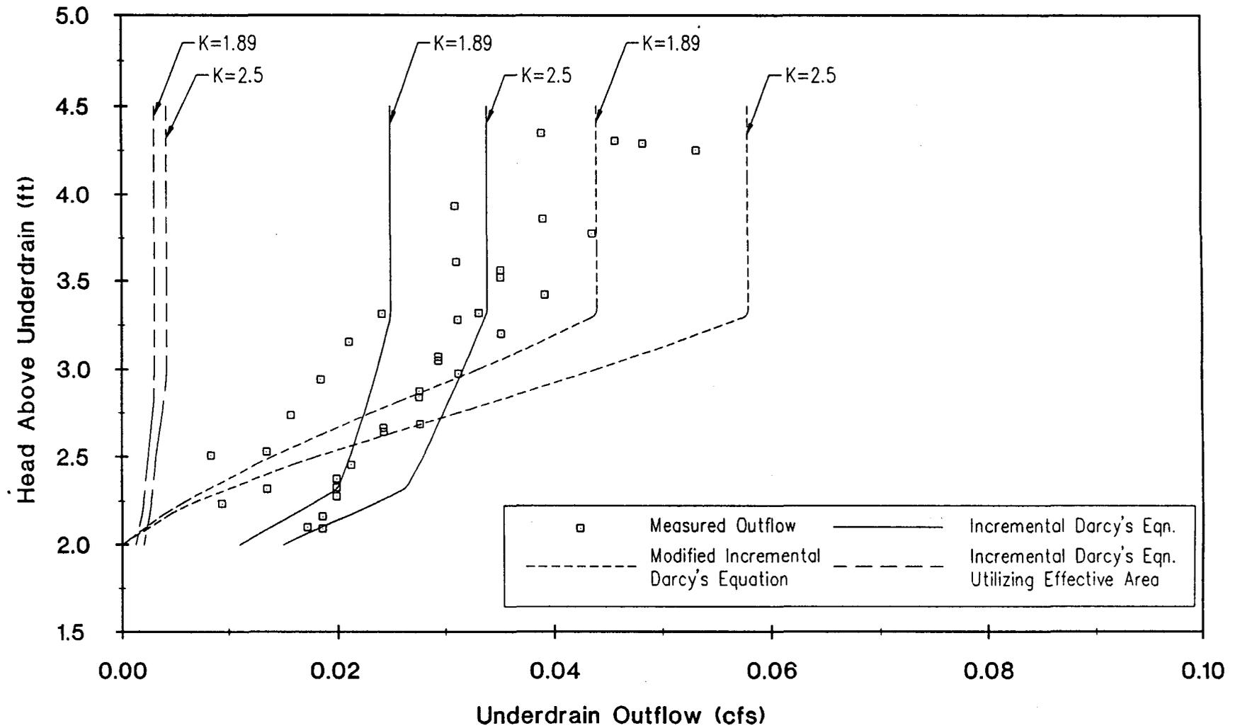
Figure 4-31. Comparison of Measured and Calculated Drawdown Curves for a Side Bank Filter Covered with Bahia Sod Grown in Sand.
