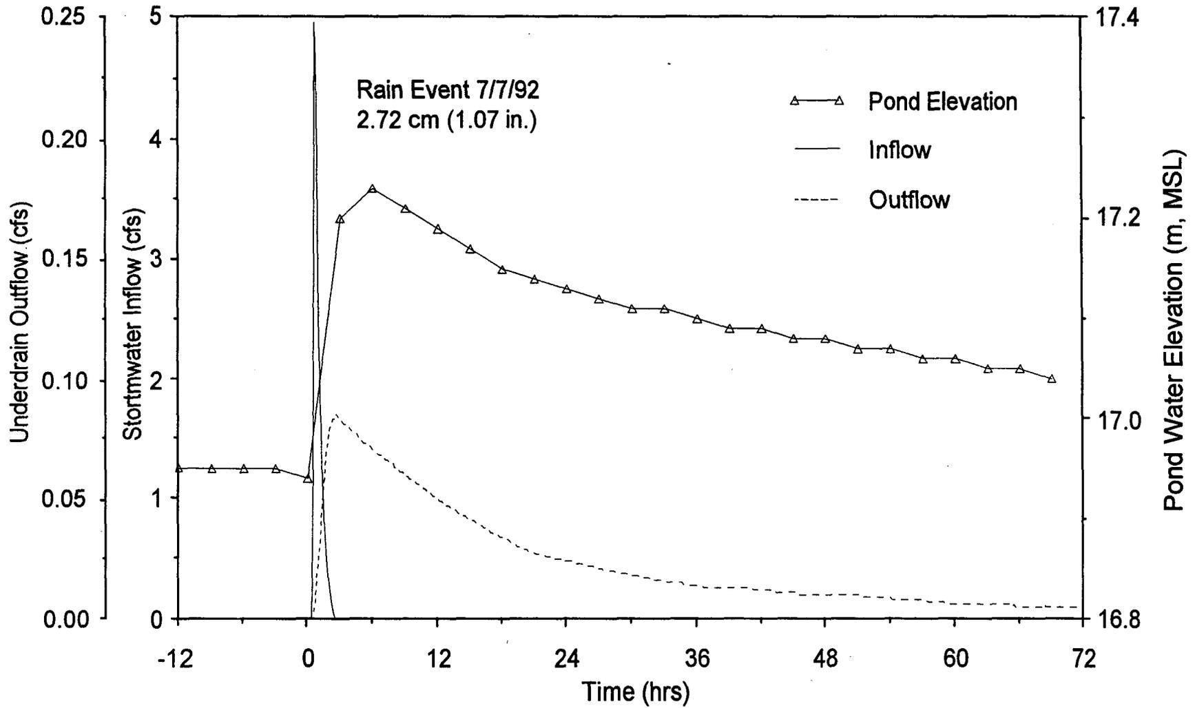
Figure 4-20. Relationships Between Inflow, Outflow and Pond Stage for a 2.72 cm (1.07 in) Rain Event on July 7, 1992.
