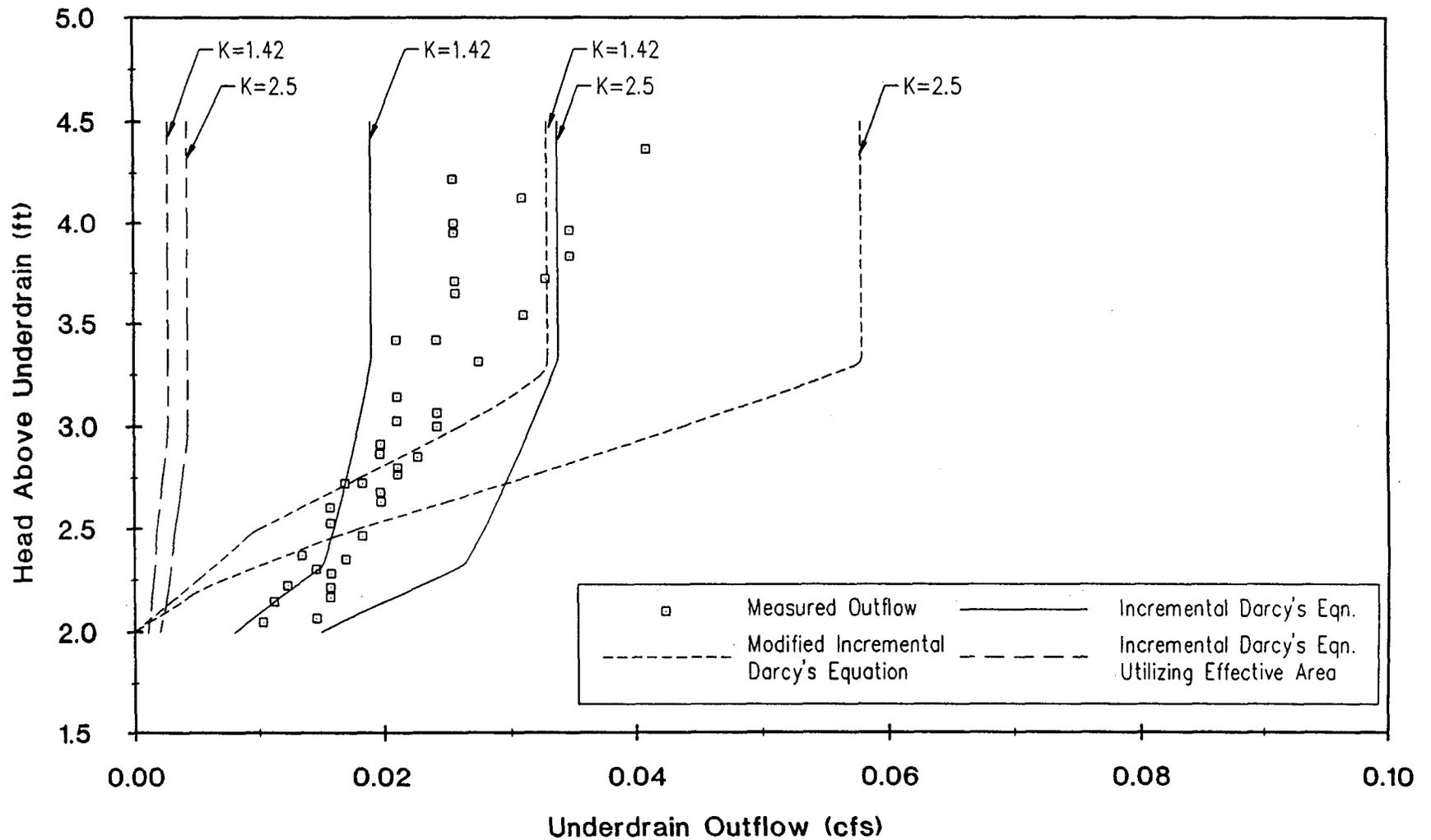
Figure 4-34. Comparison of Measured and Calculated Drawdown Curves for a Side Bank Filter Covered with Bermuda Sod Grown in Muck.
