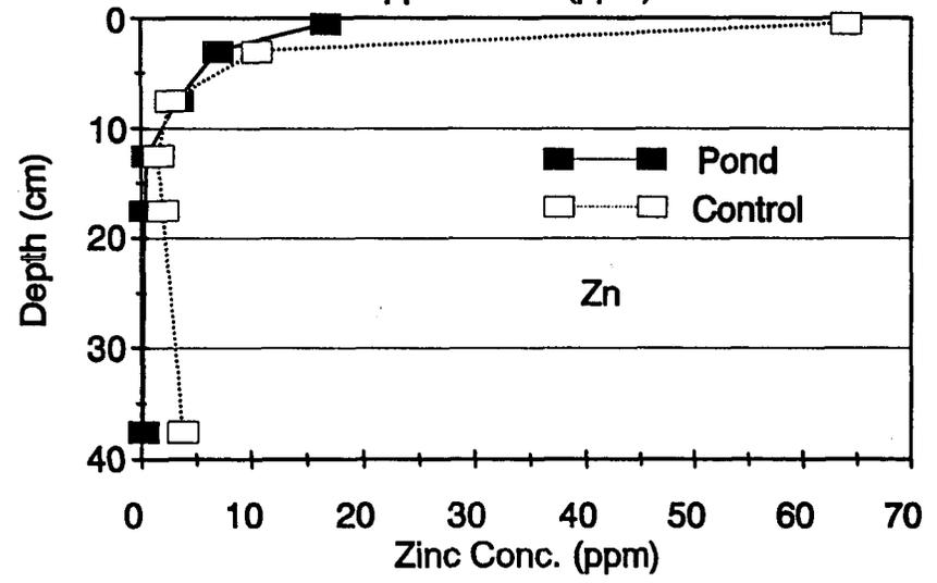
Figure 4-13. Comparison of Sediment Concentrations of Cadmium, Copper, Lead and Zinc in the Top 50 cm of Pond and Control Areas at the DeBary Detention with Filtration Site.
