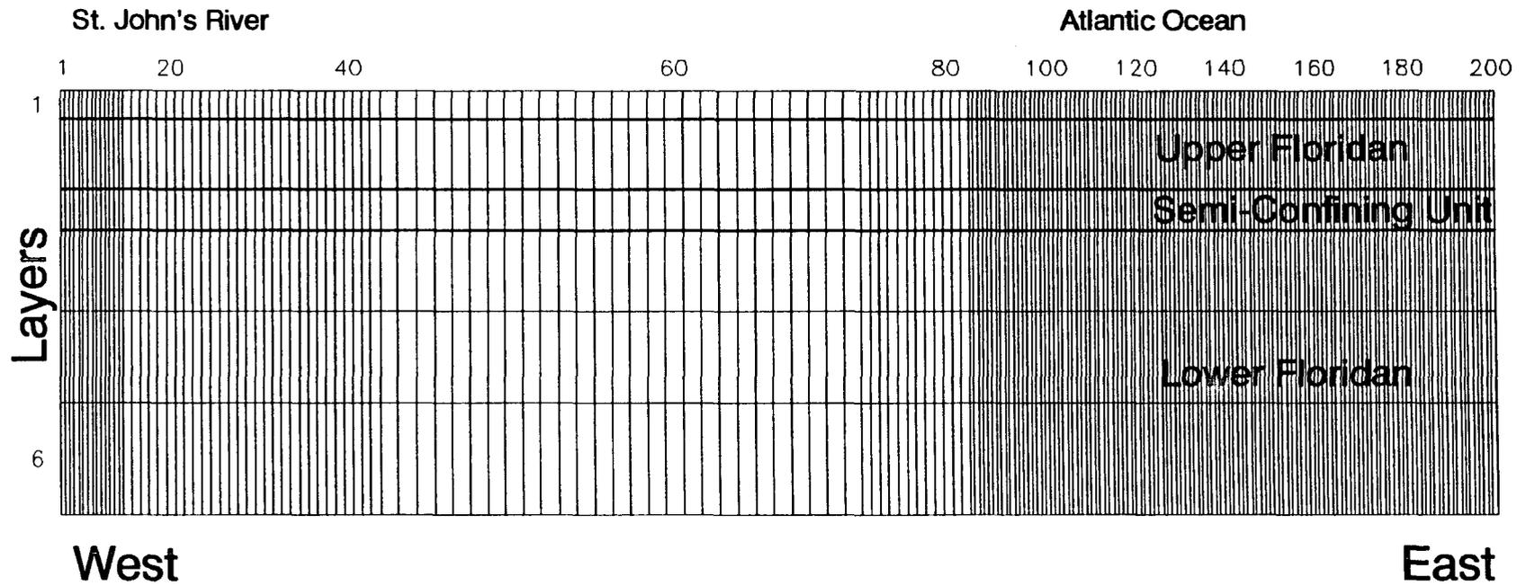
Figure 17. Cross-sectional model finite-difference grid (six layer model).
