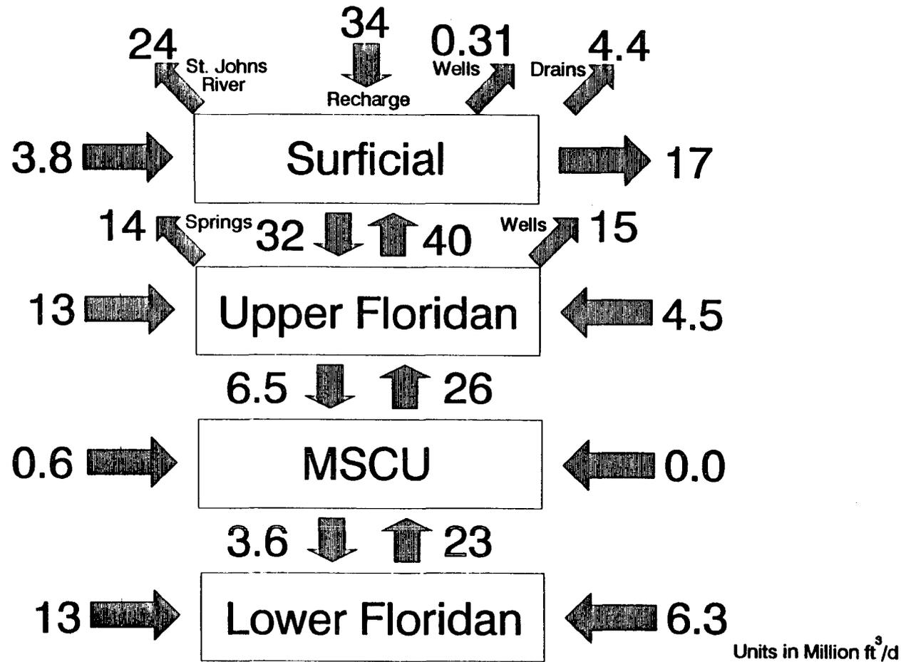
Figure 82. Ground-water flow mass balance analysis for the 2010 three-dimensional model (pumping from existing and proposed wellfields).
