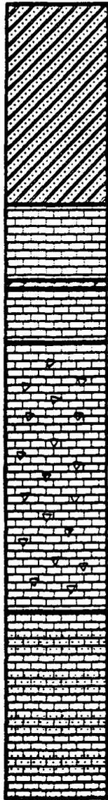
SAND, CLAY AND SHELL, CLAY IS GRAY TO GREEN, CLAY IS PLASTIC, SAND IS GENERALLY FINE GRAINED, PHOSPHATIC
