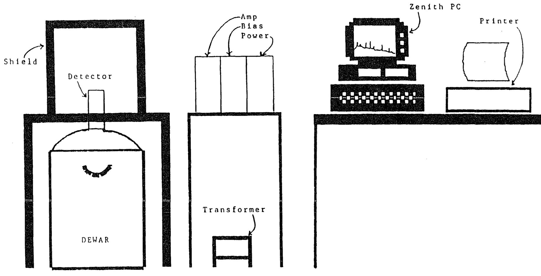
Figure 2: Diagram of the counting system at the Department of Environmental Engineering Sciences, University of Florida. (See text for specifics.) (after Nagy, 1988)
