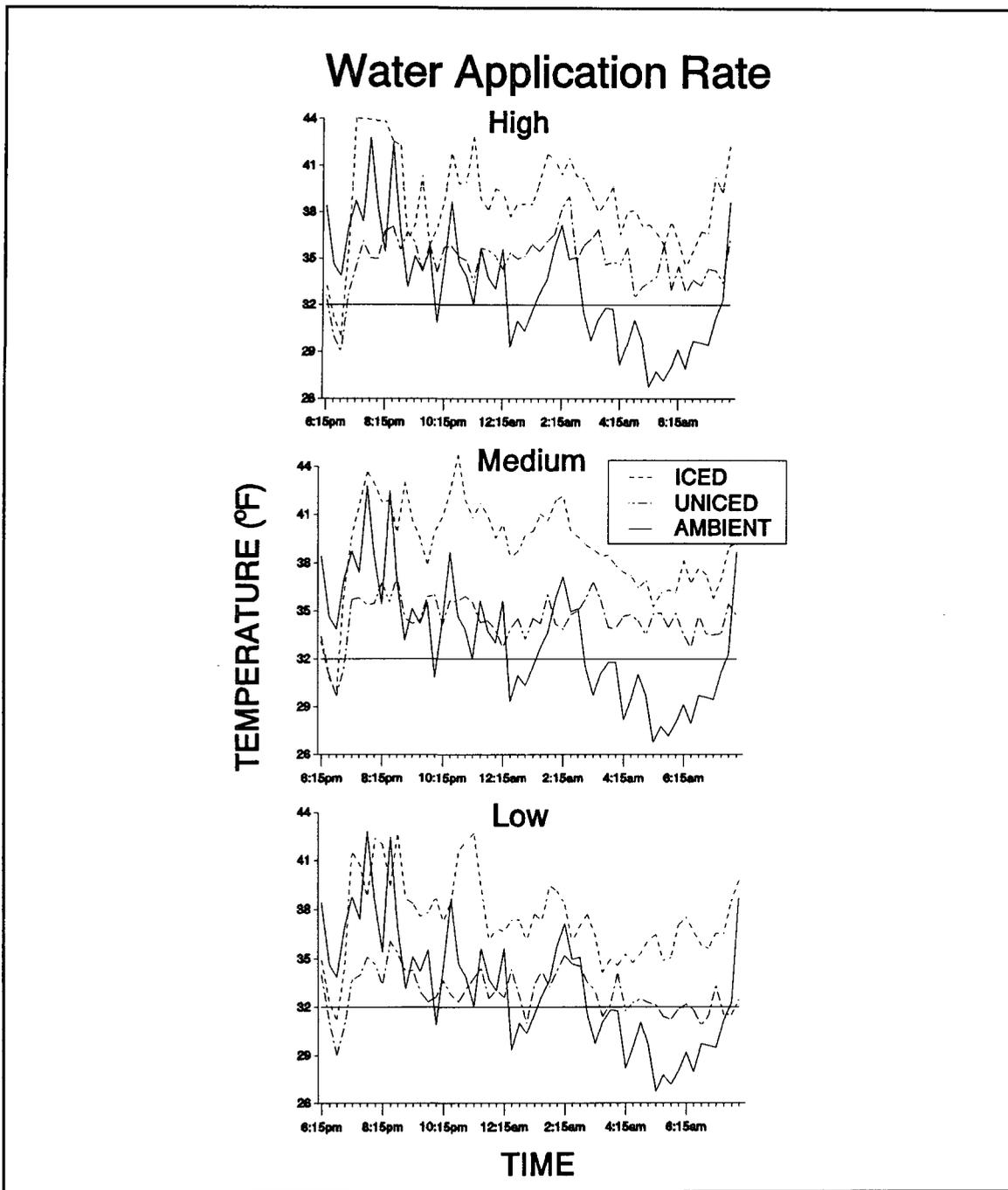
Figure 14. Comparison of leaf temperatures in iced and uniced shadehouses receiving 0.12 inch/hr [0.30 cm·hr<sup>-1</sup>] (low), 0.22 inch/hr [0.56 cm·hr<sup>-1</sup>] (medium), or 0.30 inch/hr [0.76 cm·hr<sup>-1</sup>] (high) water application rates on February 16-17, 1991.
