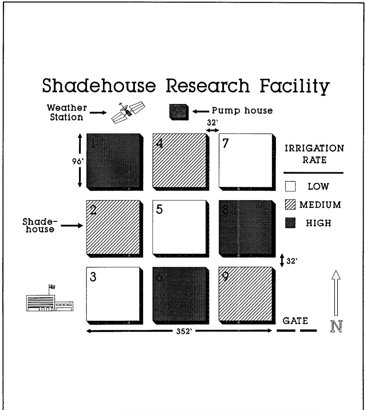
**Figure 8.** Latin-square design of irrigation water application rate treatments at shadehouse research facility in Pierson, Florida.
