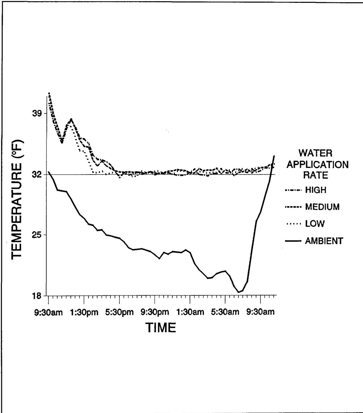
Figure 17. Outside ambient air temperatures (solid line) and leaf temperatures inside iced shadehouses equipped with side curtains and cold protected using low, medium and high water application rates (Table 5) on December 23-24, 1989.
