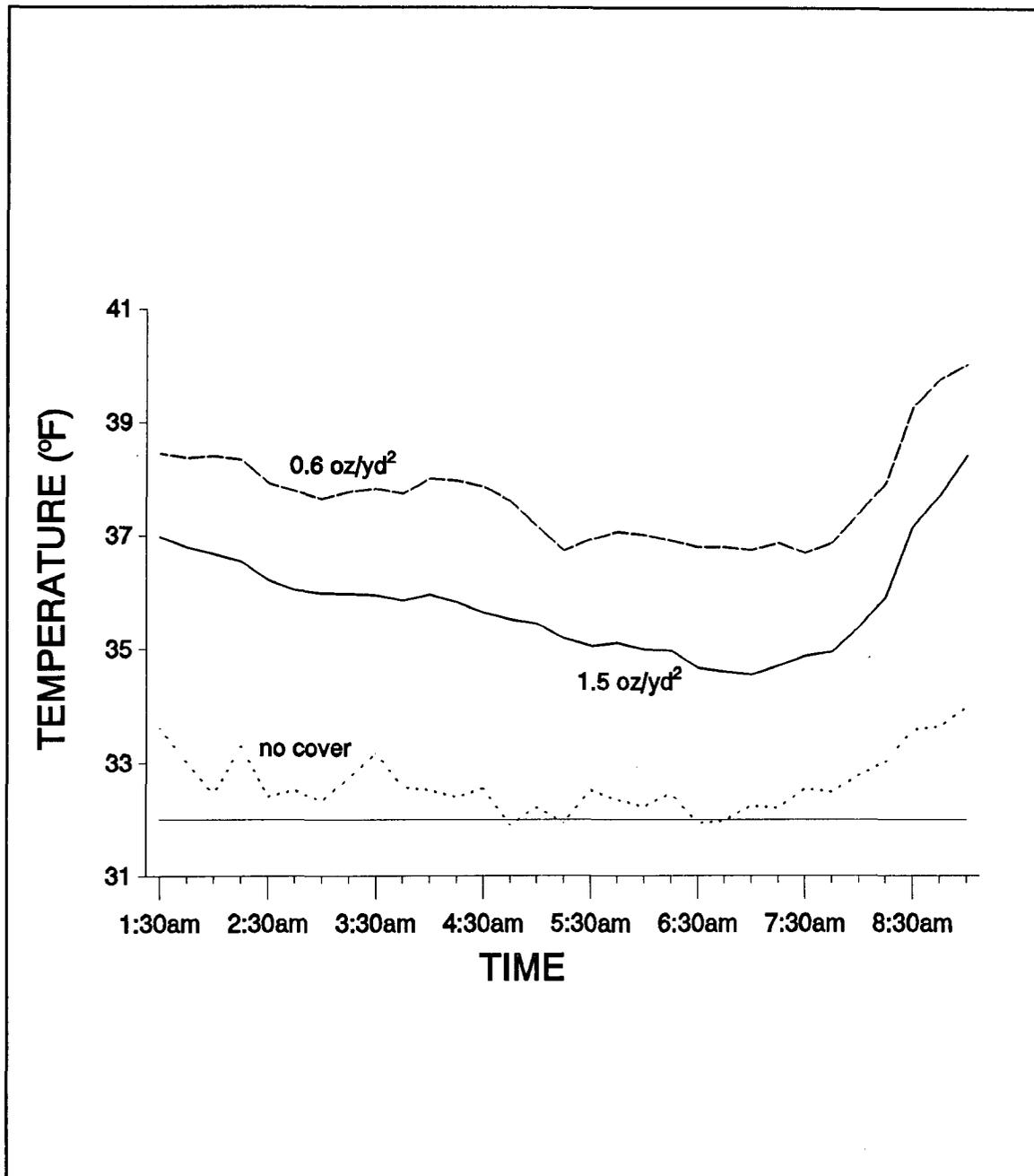
Figure 20. Temperatures measured approximately 18 inches [46 cm] above the soil surface outside crop covers and at the underside of the crop covers in iced shadehouses receiving overhead irrigation on February 15-16, 1991.
