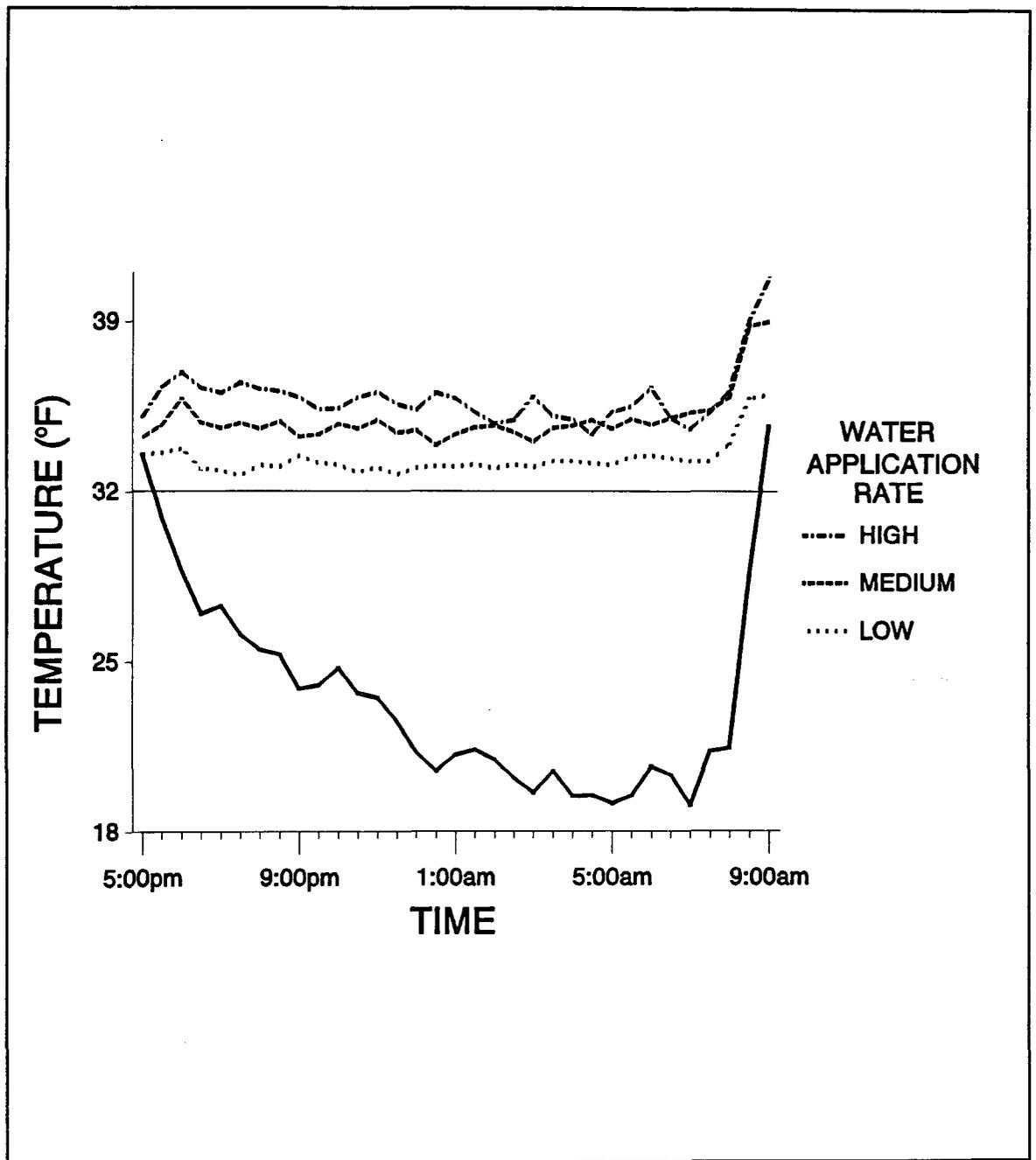
Figure 12. Outside ambient air temperatures (solid line) and leaf temperatures inside iced shadehouses equipped with side curtains and cold protected using three different irrigation water application rates (Table 4) on December 24-25, 1989.
