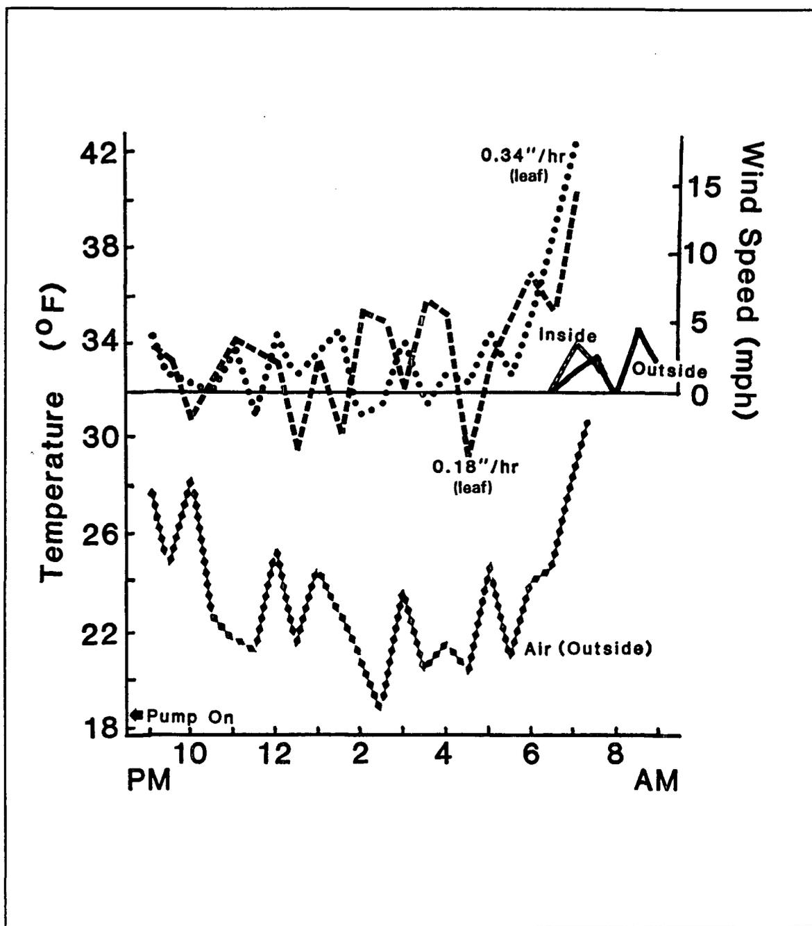
Figure 1. Comparison of leaf (---, ....) and air (-----) temperatures when using conventional irrigation sprinklers (1.1 rpm, 0.34 inch/hr [8.6 mm·hr<sup>-1</sup>]) and frost protection sprinklers (2.9 rpm, 0.18 inch/hr [4.6 mm·hr<sup>-1</sup>]) during a radiation freeze (Stamps and Mathur, 1982). The wind was calm until sunrise both inside and outside the shadehouse.
