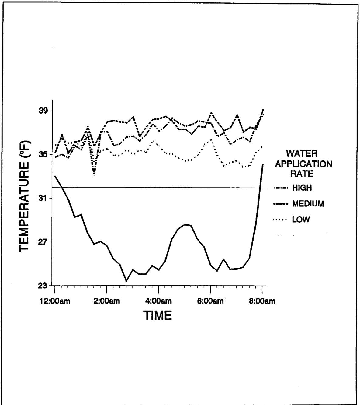
Figure 11. Outside ambient air temperatures (solid line) and leaf temperatures inside iced shadehouses equipped with side curtains and cold protected using three different irrigation water application rates (Table 3) on December 3-4, 1989.
