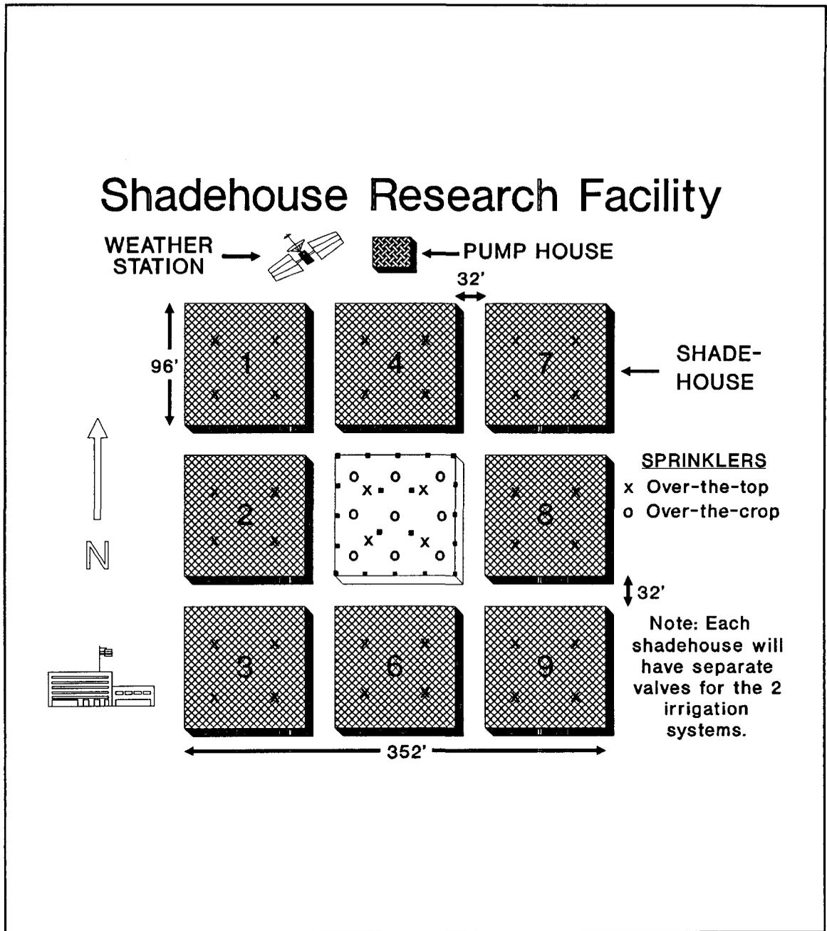
**Figure 9.** Schematic of shadehouse research facility in Pierson, Florida. Note that the shade fabric has been removed from the center shadehouse to reveal the layout of the over-the-crop irrigation systems. Each shadehouse was equipped with both over-the-shadehouse (over-the-top) and over-the-crop irrigation systems.
