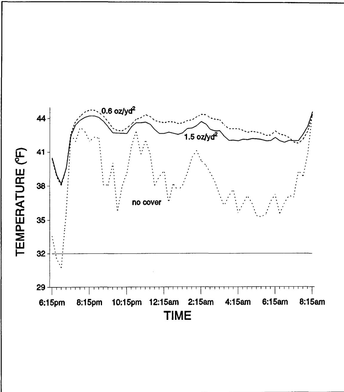
Figure 16. Temperatures measured 9 inches [24 cm] above the soil surface outside and under crop covers in iced shadehouses receiving overhead irrigation on February 16-17, 1991.
