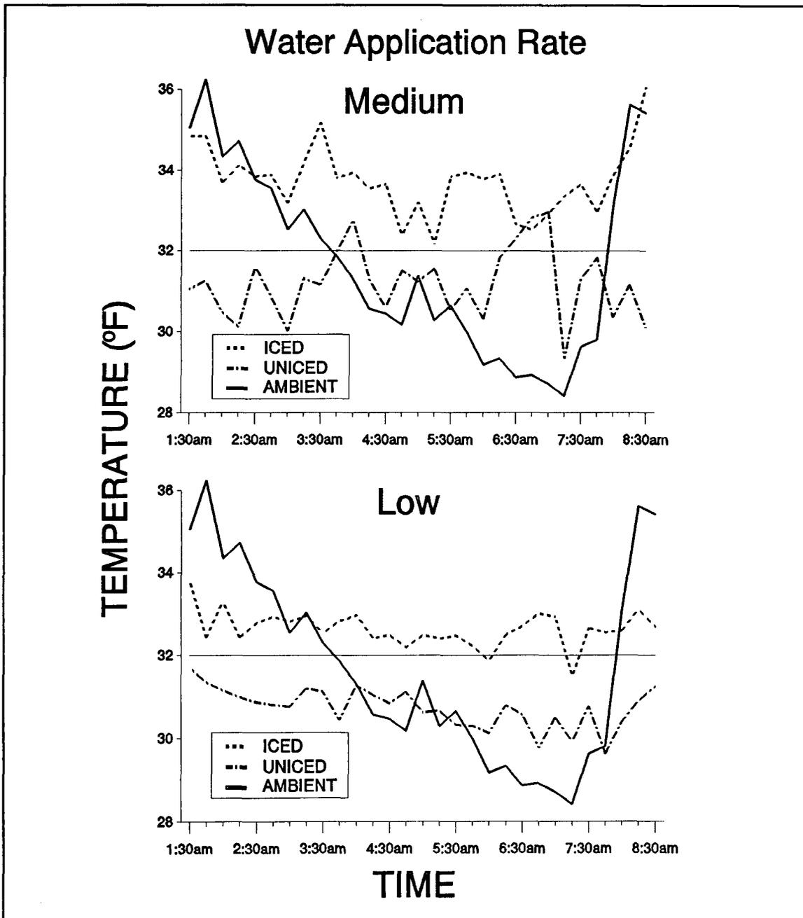
**Figure 19.** Comparison of temperatures in iced versus uniced shadehouses irrigated at low and medium application rates (Table 6) during an advective freeze on February 15-16, 1991. Data from the high irrigation application rate houses was not considered reliable and, therefore, is not reported.
