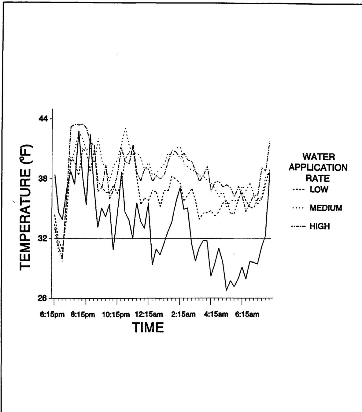
Figure 13. Outside ambient air temperatures (solid line) and leaf temperatures inside iced shadehouses equipped with side curtains and cold protected using three different irrigation rates (Table 5) on February 16-17, 1991.
