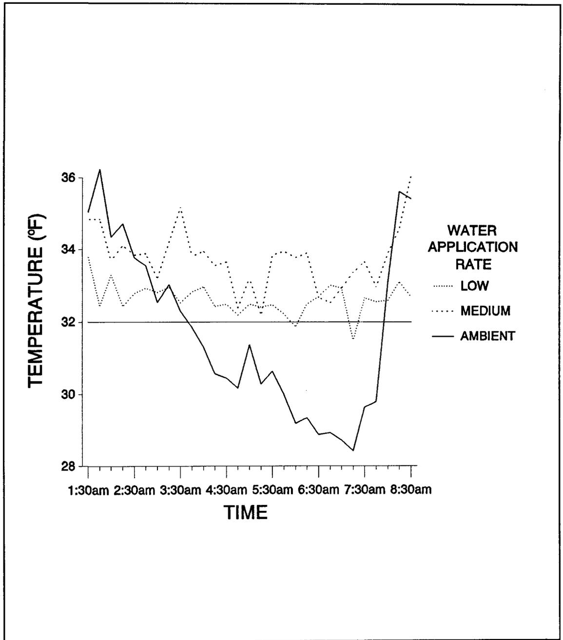
**Figure 18.** Outside ambient air temperatures and leaf temperatures inside iced shadehouses equipped with side curtains and cold protected using low and medium water application rates (Table 6) on February 15-16, 1991. Data from the high irrigation application rate houses was not considered reliable and, therefore, is not reported.
