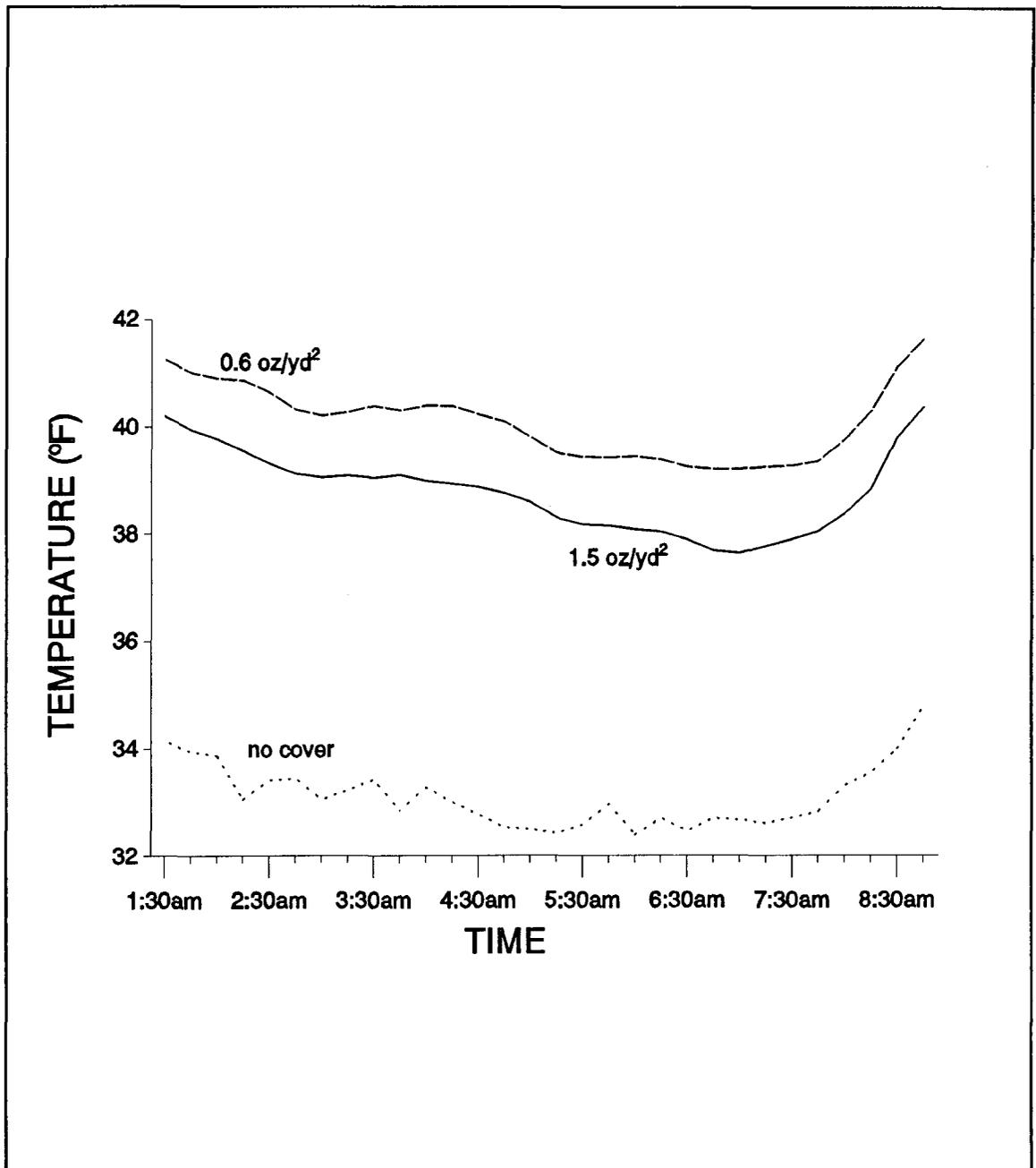
Figure 21. Temperatures measured 9 inches [23 cm] above the soil surface outside crop covers and under crop covers in iced shadehouses receiving overhead irrigation on February 15-16, 1991.
