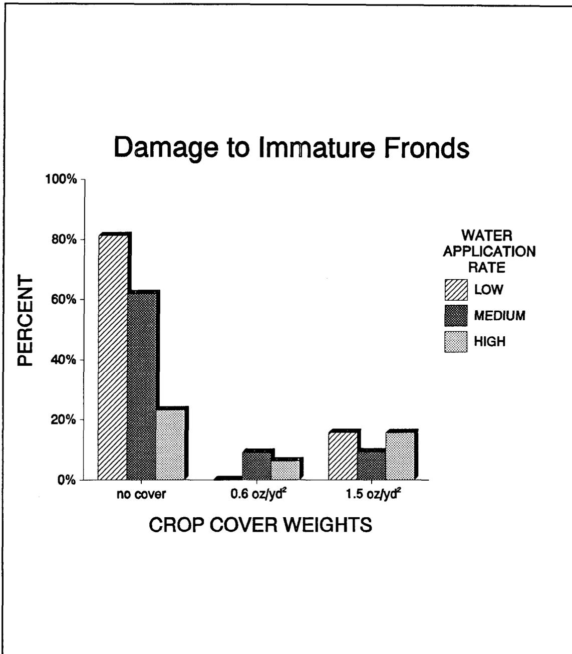
**Figure 22.** Percentage of immature fronds with cold damage following the February 1991 freeze. Treatments included three water application rates (0.12, 0.22 or 0.30 inch/hr [0.3 cm, 0.56 or 0.76 cm·hr<sup>-1</sup>]), two spunbonded polypropylene crop cover weights (0.6 or 1.5 oz/yd<sup>2</sup> [20 or 51 g·m<sup>-2</sup>]), and a control with no crop cover.
