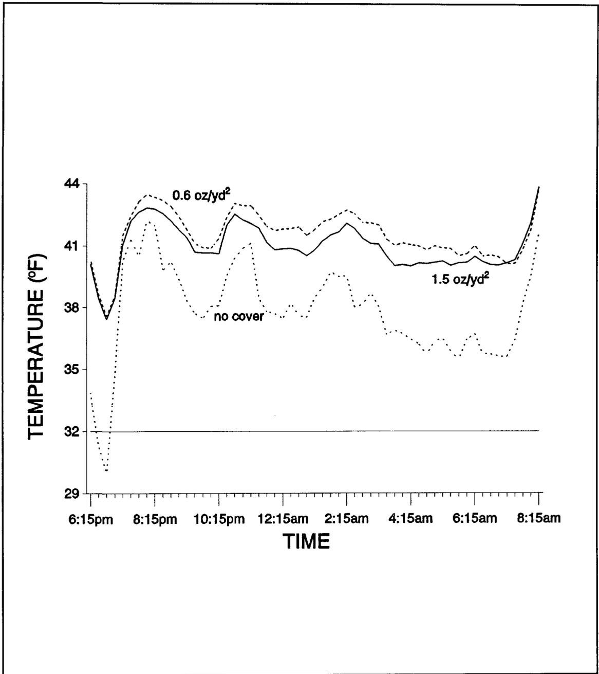
Figure 15. Temperatures measured approximately 18 inches [46 cm] above the soil surface outside crop covers and at the underside of the crop covers in iced shadehouses receiving overhead irrigation on February 16-17, 1991.
