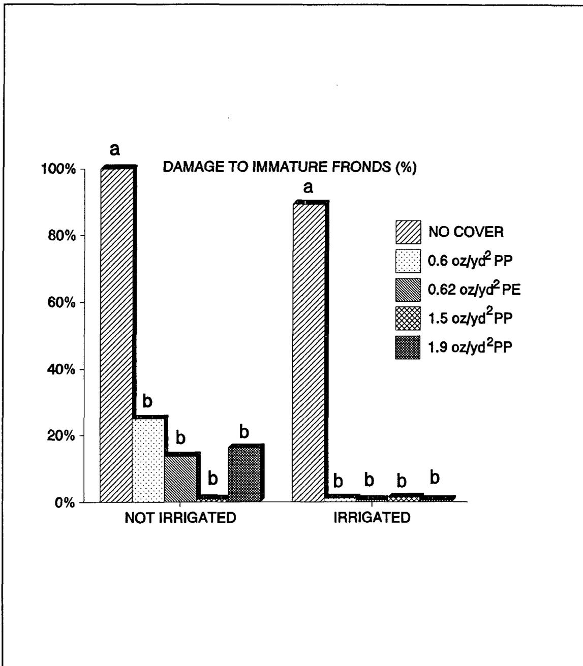
Figure 7. Frond damage under 0.6, 0.62, 1.5, or 1.9 oz/yd<sup>2</sup> [20, 21, 51, or 64 g · m<sup>-2</sup>] spunbonded polyester (PE) or polypropylene (PP) crop covers compared with no crop cover, with and without over-the-crop irrigation (Stamps, 1991).
