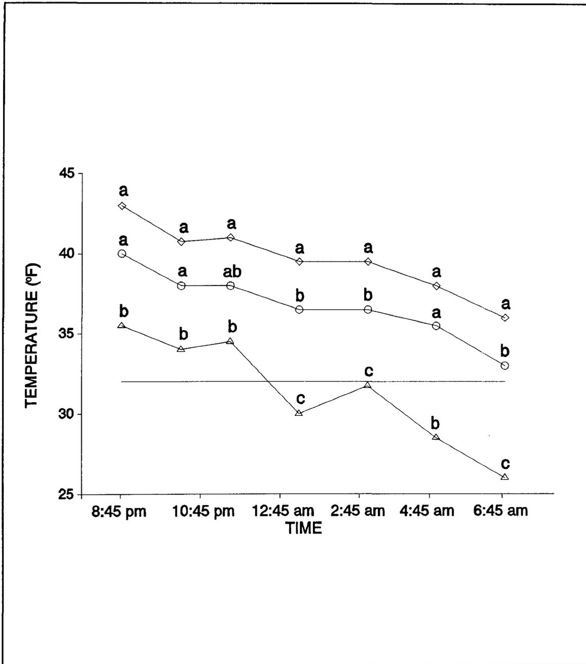
Figure 4. Temperatures 9 inches [23 cm] above the soil surface under 0.6 oz/yd<sup>2</sup> [20 g·m<sup>-2</sup>] (---○---) or 1.5 oz/yd<sup>2</sup> [51 g·m<sup>-2</sup>] (---◇---) spunbonded polypropylene crop covers or no cover (—△—) (Stamps, 1990b). For a given time, temperatures marked with the same letter are not statistically different (Duncan's new multiple range test, *P*=0.05).
