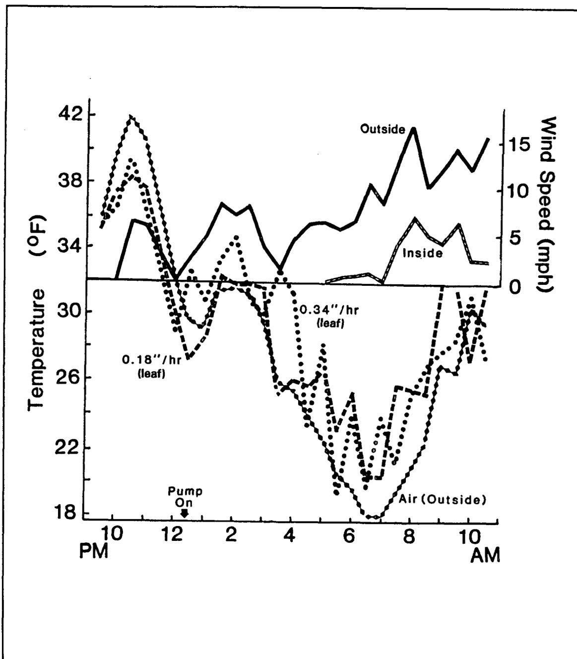
**Figure 2.** Comparison of leaf (---, ....) and air (----) temperatures when using conventional irrigation sprinklers (1.1 rpm, 0.34 inch/hr [8.6 mm·hr<sup>-1</sup>]) and frost protection sprinklers (2.9 rpm, 0.18 inch/hr [4.6 mm·hr<sup>-1</sup>]) for cold protection during an advective freeze (Stamps and Mathur, 1982). The highest wind speed recorded inside the fernery was 6.8 mph [10.9 km·hr<sup>-1</sup>].
