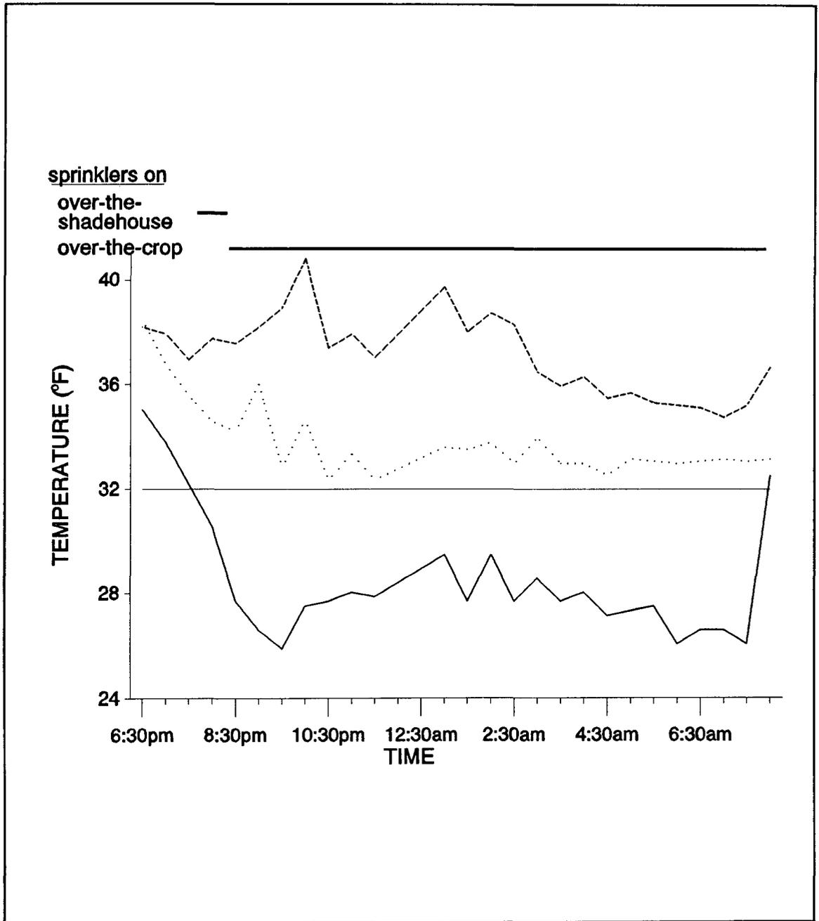
**Figure 3.** Ambient air temperatures outside shadehouses (—) and inside uniced (.....) and iced (- - -) shadehouses. The irrigation rate inside both shadehouses was 0.25 inch/hr [6.4 mm·hr<sup>-1</sup>] (Stamps, 1989).
