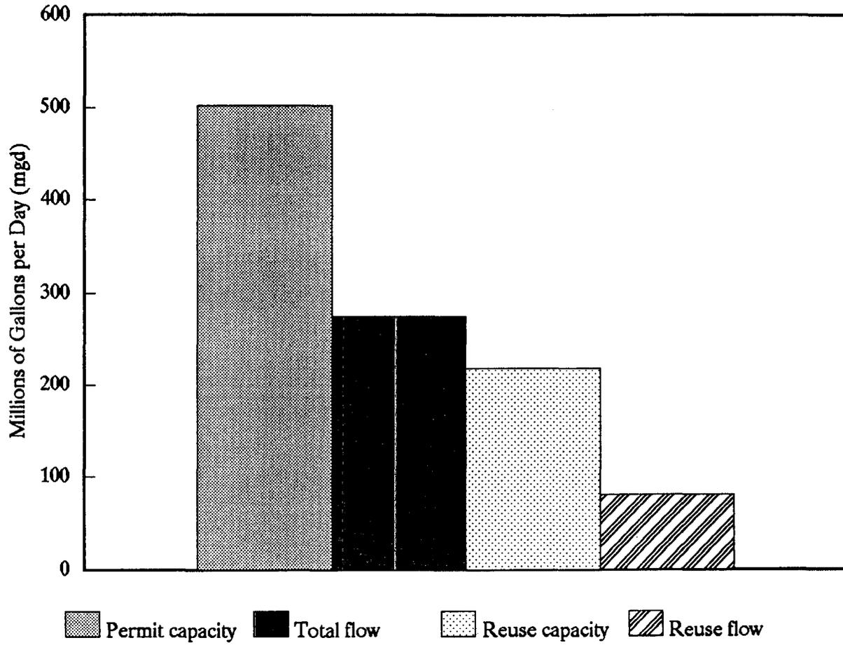
Figure 4. Wastewater treatment plant capacity and flow, St. Johns River Water Management District, 1989
