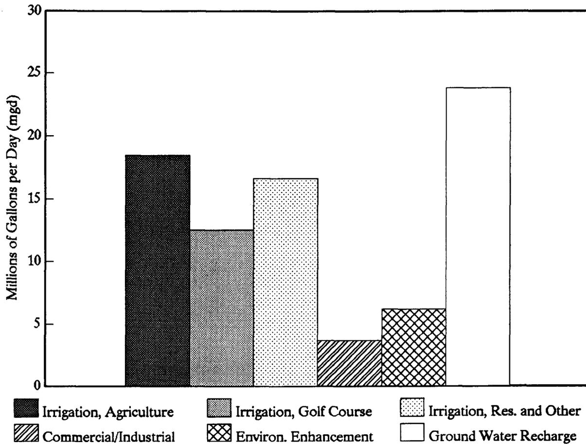
Figure 7. Wastewater reuse in the St. Johns River Water Management District, 1989. *The most common form of wastewater reuse was irrigation.*
