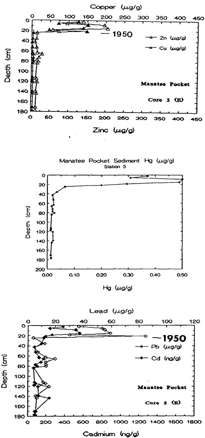
Figure 24. Vertical profiles for concentrations of copper, zinc, mercury, lead and cadmium in sediments from Manatee Pocket.
