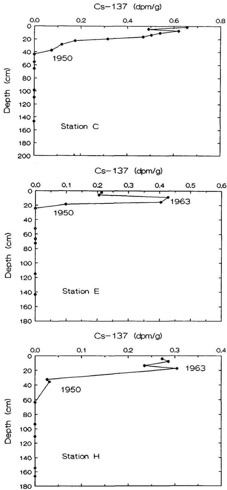
Figure 21. Vertical profiles of Cs-137 in sediments from stations C, E and H (Figure 12) in Manatee Pocket with age estimates as described in text.
