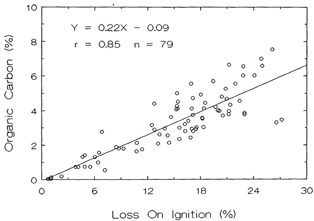
Figure 2. Scatter plot showing concentrations of organic carbon versus Loss On Ignition for sediments from the Indian River Lagoon.
