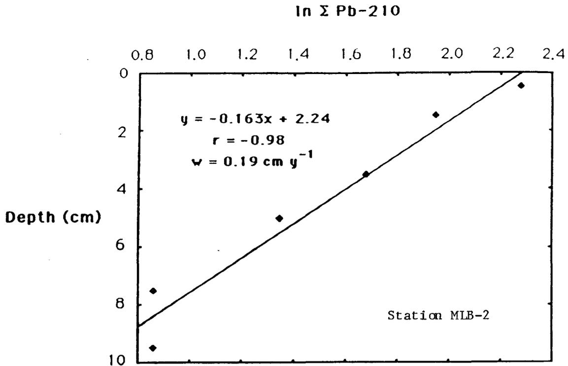
Figure 23. Vertical profiles of total Pb-210 in sediments from the Melbourne area of the Indian River Lagoon
