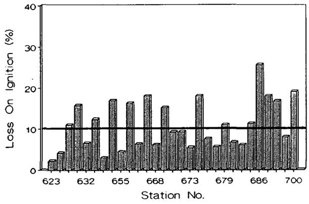
Figure 13. Histograms showing percent Loss on Ignition (LOI) in Indian River Lagoon sediments from stations 1-700. Solid line identifies 10% LOI. Sediments with greater than 10% LOI are characterized as muck.
