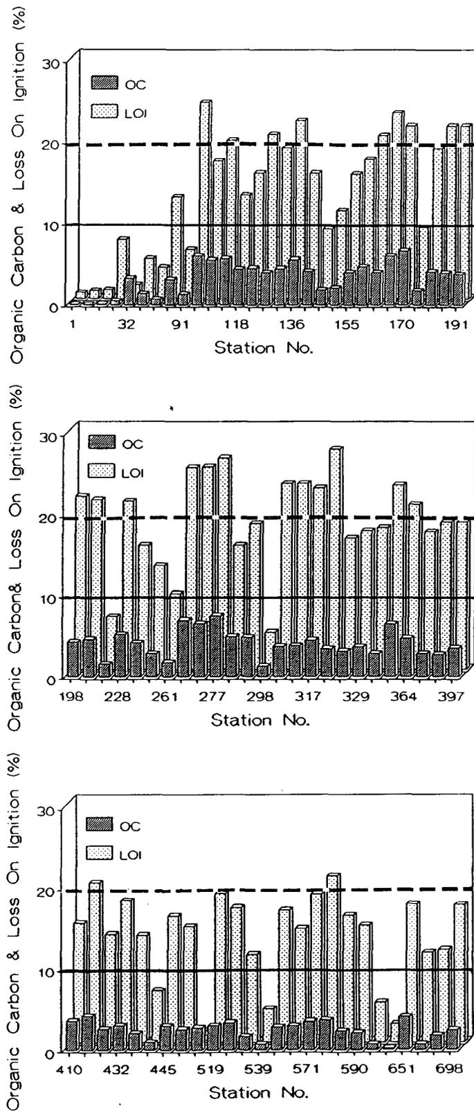
Figure 14. Histograms showing percent organic carbon and Loss On Ignition (LOI) in sediments from selected stations in the Indian River Lagoon. Solid line identifies 10% LOI, the minimum level for muck sediments. The dashed line identifies 20% LOI for very organic-rich sediments.
