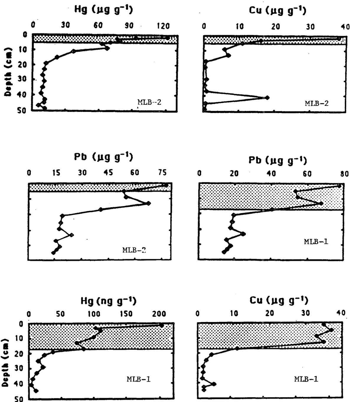
Figure 25. Vertical profiles for concentrations of mercury, copper and lead in sediments from the Melbourne area of the Indian River Lagoon. Shaded surface layer identifies muck sediment.
