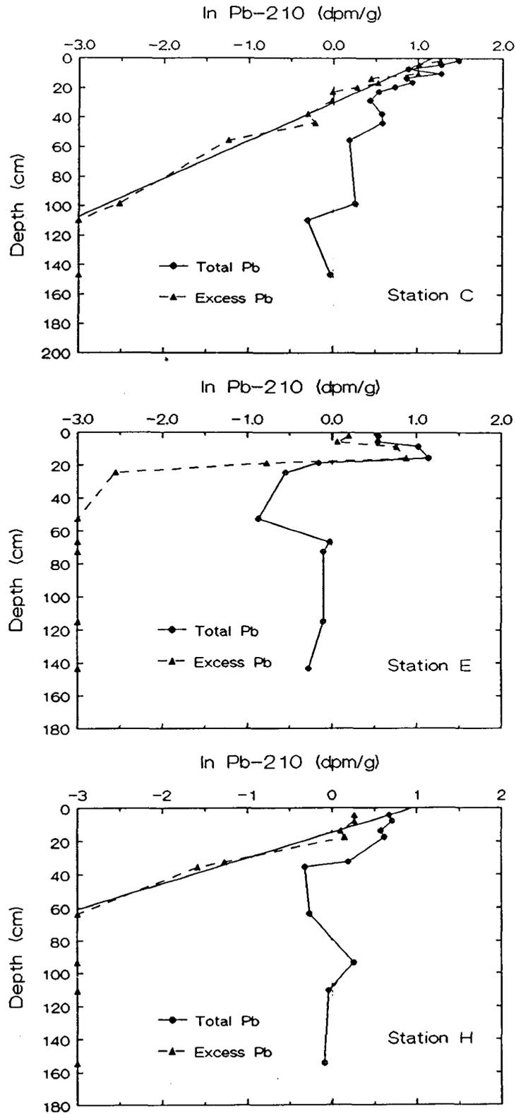
Figure 22. Vertical profiles of total and excess Pb-210 in sediments from stations C, E and H (Figure 12) in Manatee Pocket. Straight line for stations C and H gives best fit for excess Pb-210 versus depth in the sediment.
