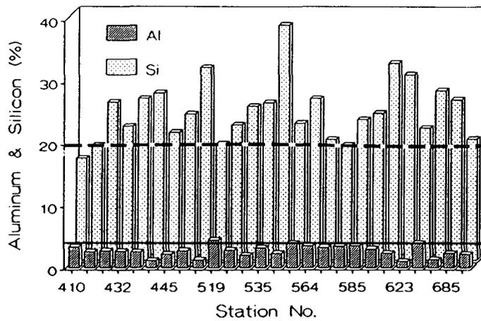
Figure 17. Histograms showing percent aluminum and silicon in sediments from selected sites in the Indian River Lagoon. Solid line at 4% identifies typical aluminum concentrations for muck sediments. Dashed line at 20% identifies average silicon values for lagoon sediments.
