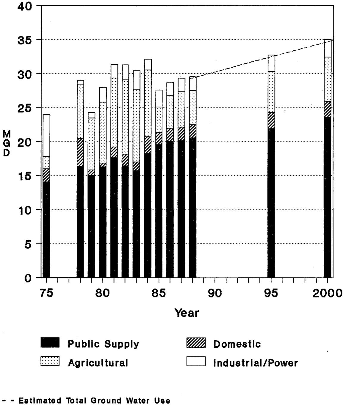
Figure 13a. Actual and projected ground water use for Alachua County
