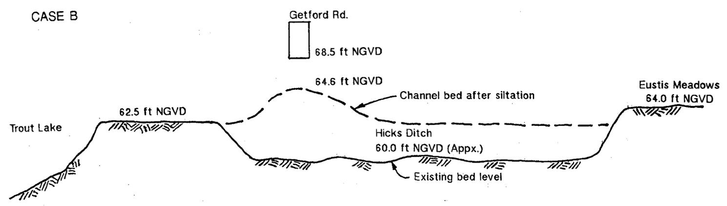
Figure 12. Assumed Hicks Ditch siltation for modeling
