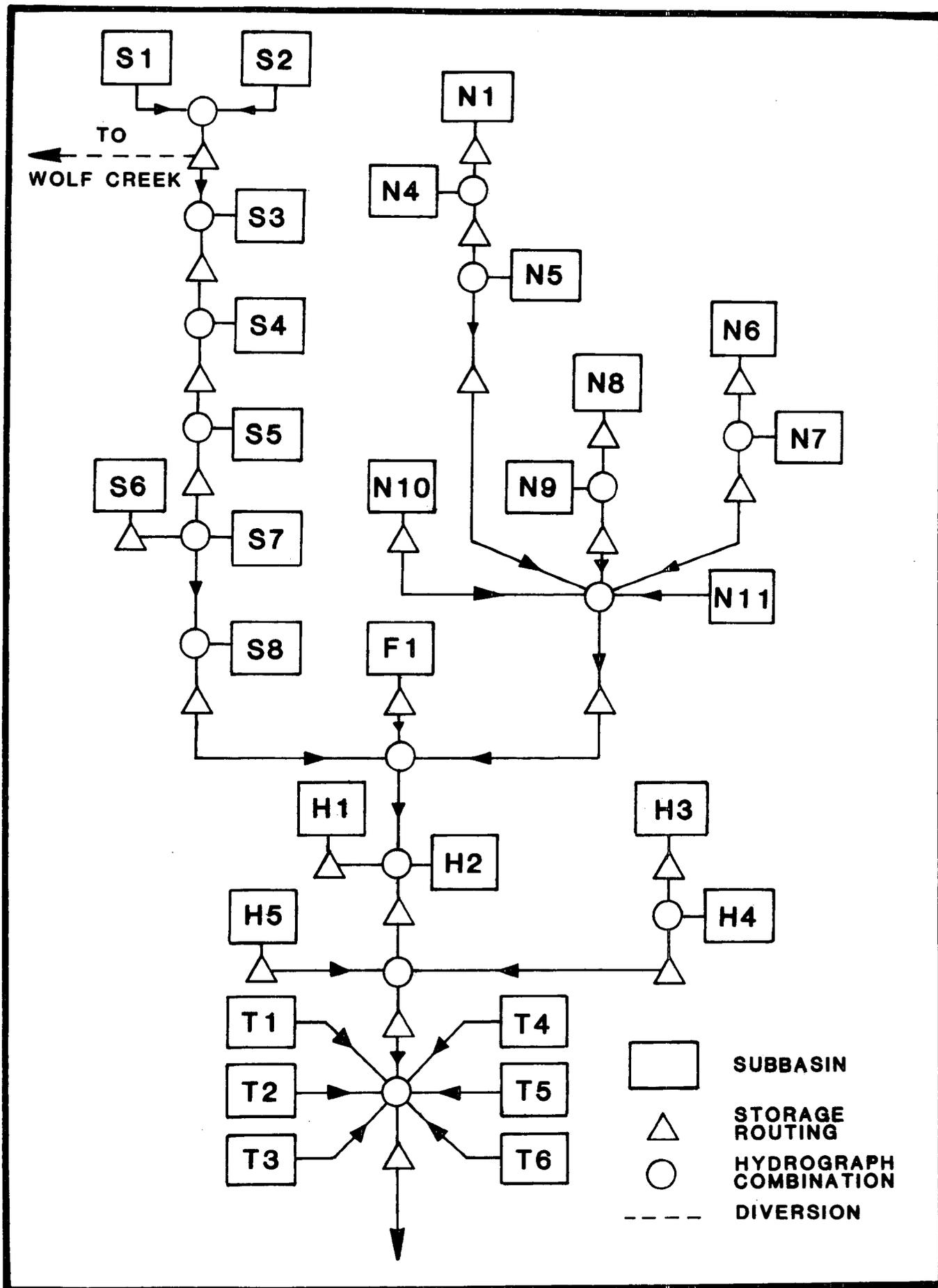
Figure 10. Schematic of the drainage in the Hicks Ditch basin
