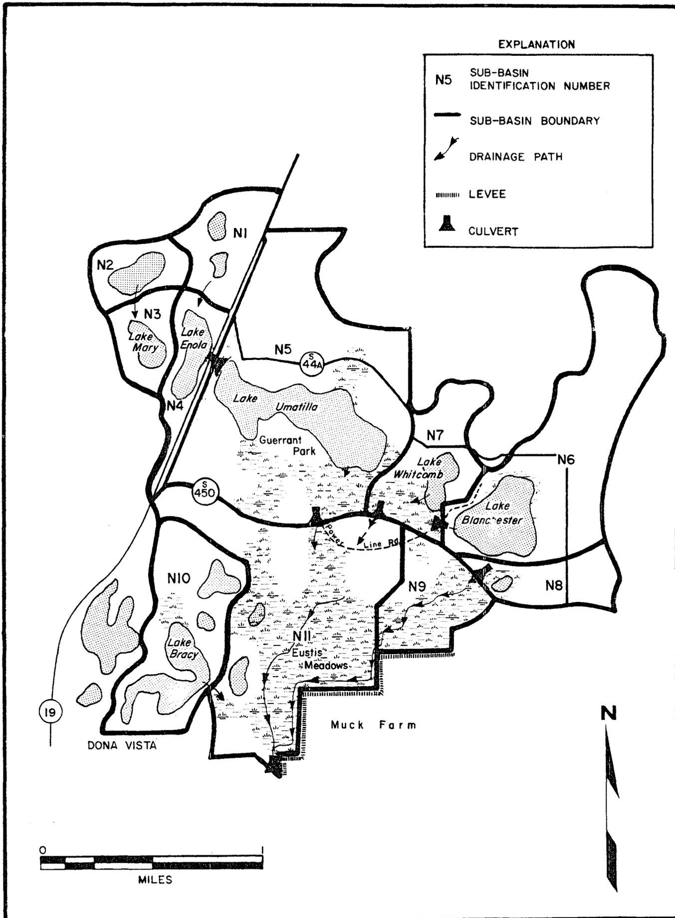
Figure 6. Drainage patterns in the northern region of the Hicks Ditch basin
