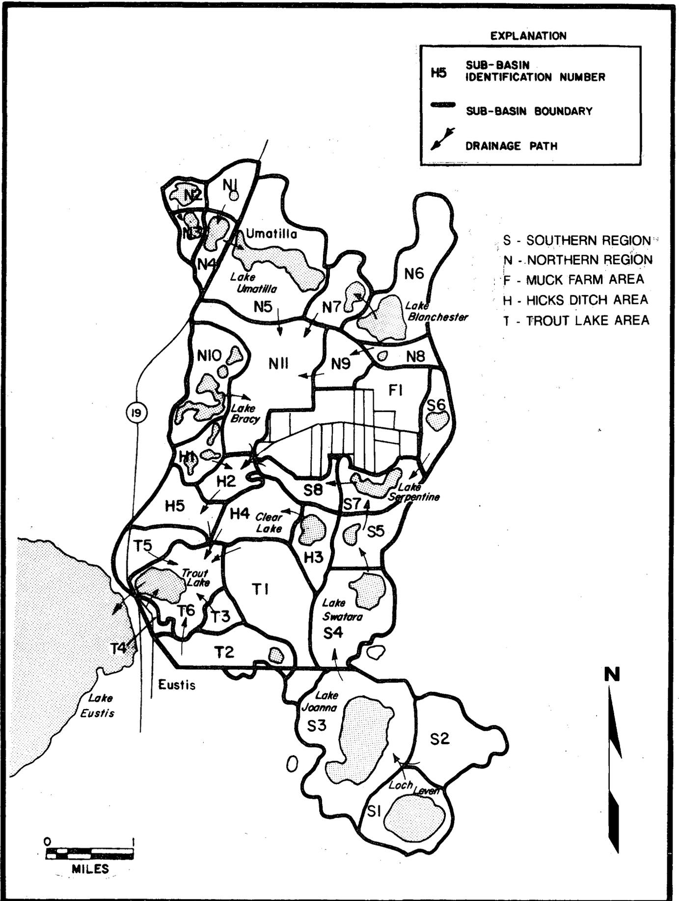
Figure 4. Subbasin delineation in the Hicks Ditch drainage basin
