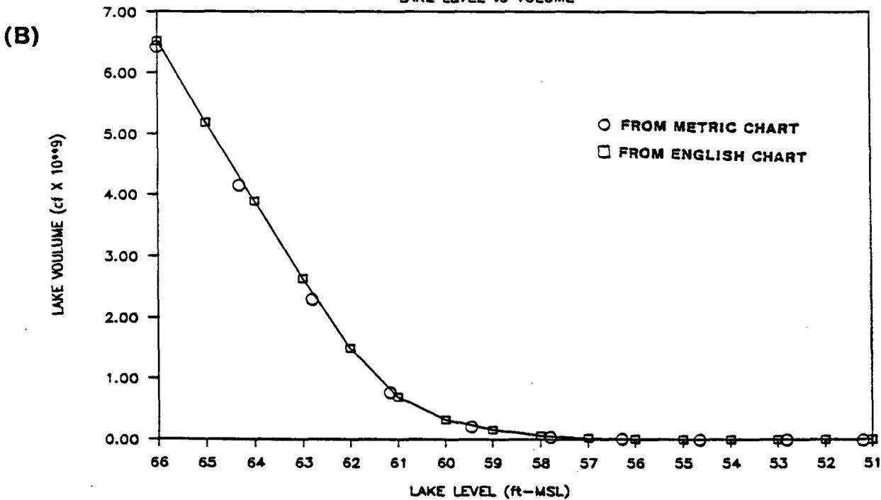
Figure 7. Hypsographic Curves for Lake Apopka Providing (A) Surface Area vs Lake Level, and (B) Lake Volume vs Lake Level
