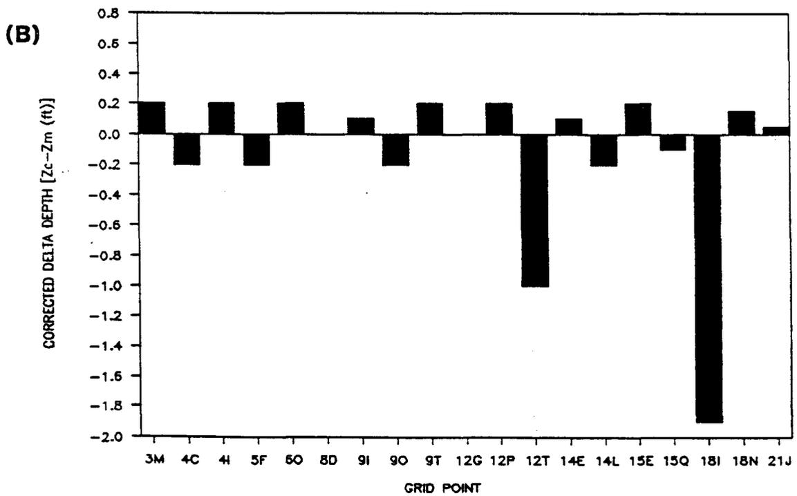
Figure 3. Difference between Survey Data ( $Z_m$ ) and Calibration Point Data ( $Z_c$ ): (A) Prior to Final Calibration and (B) After Final Calibration
