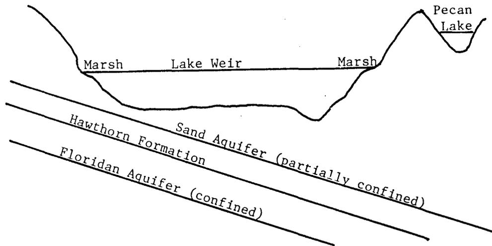
Figure 1-2. Geologic map of Lake Weir watershed showing the Floridan aquifer and an unconfined sand aquifer (adapted from Messer, 1975).
