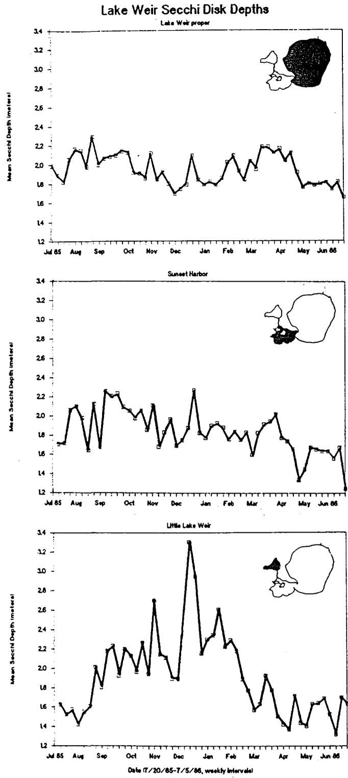
Figure 3-7. Mean Secchi disk depths for each of Lake Weir's three basins at weekly intervals throughout the year.
