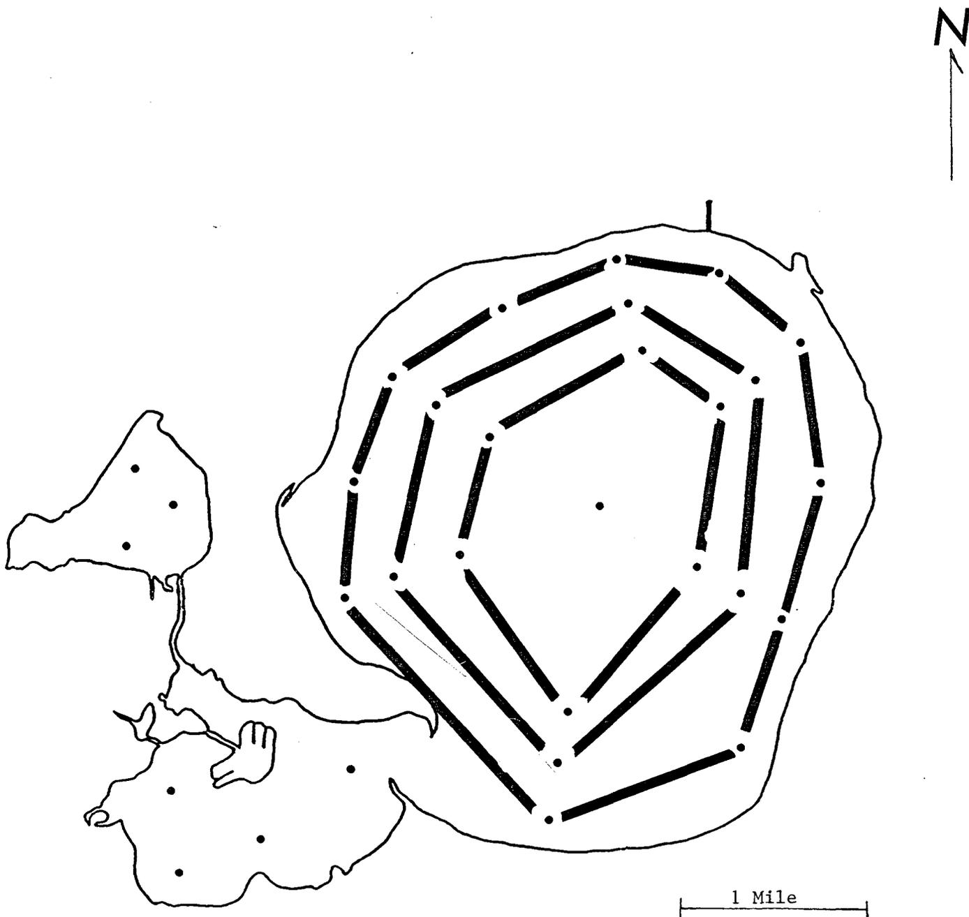
Figure 3-8. Map of Lake Weir Secchi disk stations grouped in three concentric rings to test the effect of proximity to shoreline.
