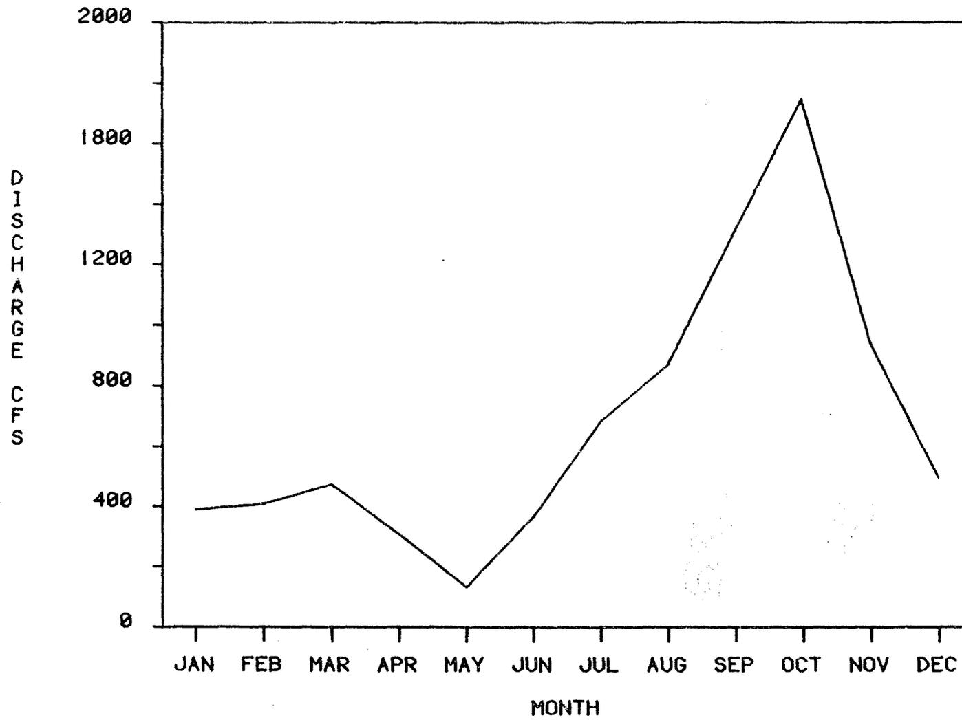
Figure 4. Mean monthly discharge (cfs) of the St. Johns River at US 192 (SR500), two miles south of Lake Washington, 1940 - 1984.
