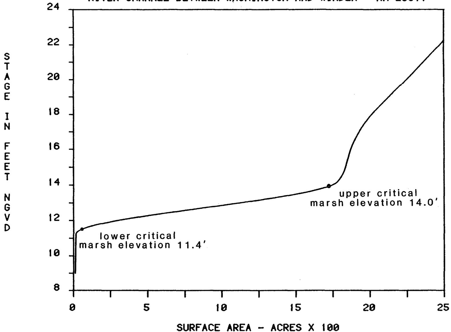
Figure 20. Stage area curve for RM 253.1, 1.3 miles downstream of the Lake Washington weir.
