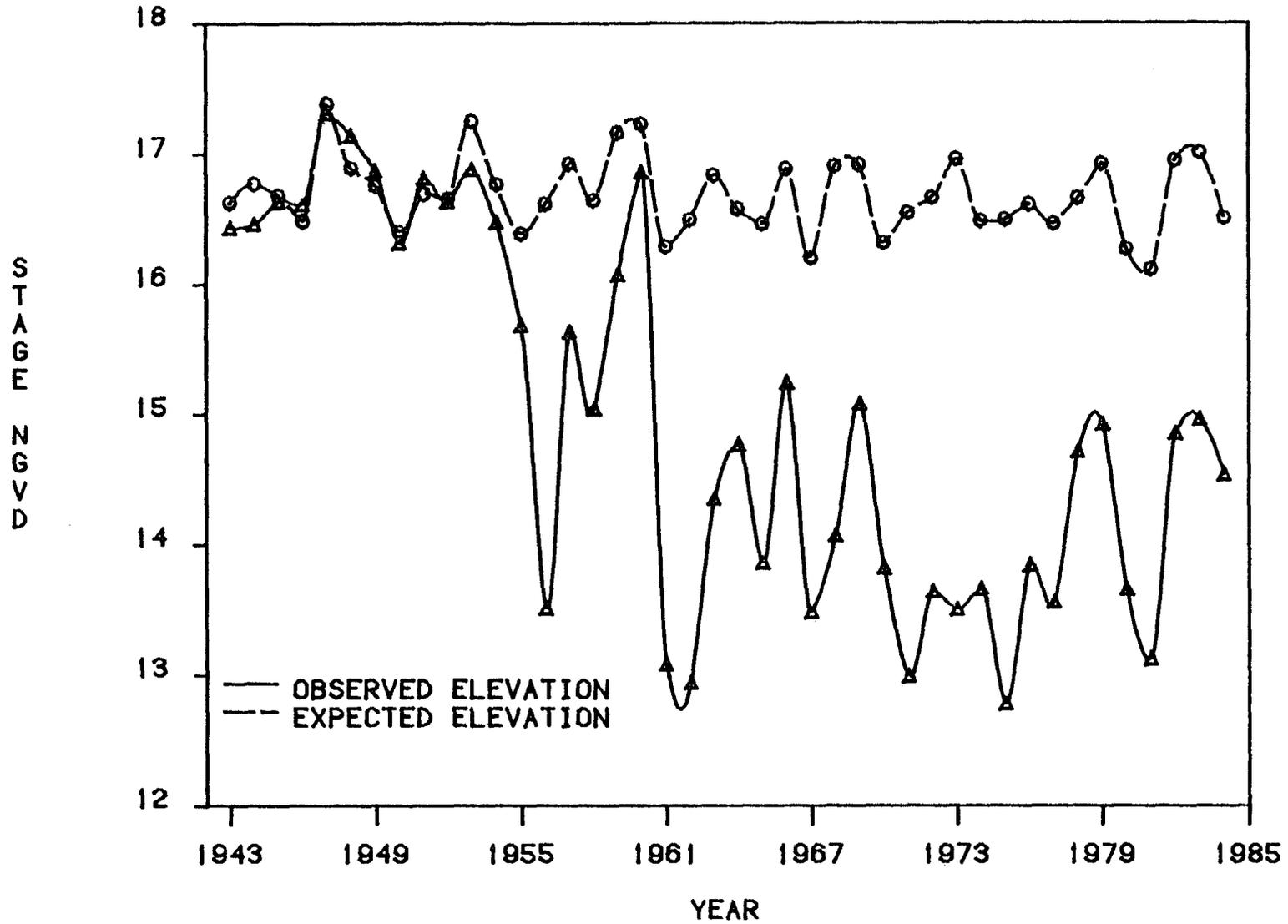
Figure 10. Observed and expected relationship between rainfall and surface water elevation at Lake Washington from 1943-1984. Expected stages were calculated using the formula,  $\text{Stage} = 14.9 + 0.0356 \cdot \text{Rainfall}$ , determined using the regression of average stage vs. rainfall for the period 1943-1952 ( $R^2 = 0.72$ ).
