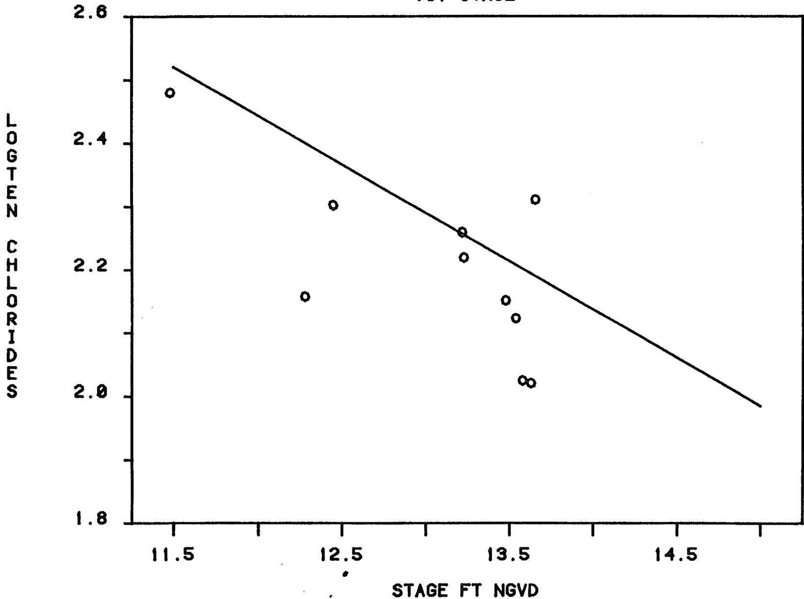
Figure 24. Relationship between annual maximum chloride concentrations and surface water stages in Lake Washington, 1977-1986. Regression equation:  $\log \text{ chlorides (MG/l)} = 4.28 - 0.153 (\text{stage in ft. NGVD})$ ,  $F_{1,8} = 15.93$ ,  $p < 0.005$ ,  $R^2 = 66.6$ .
