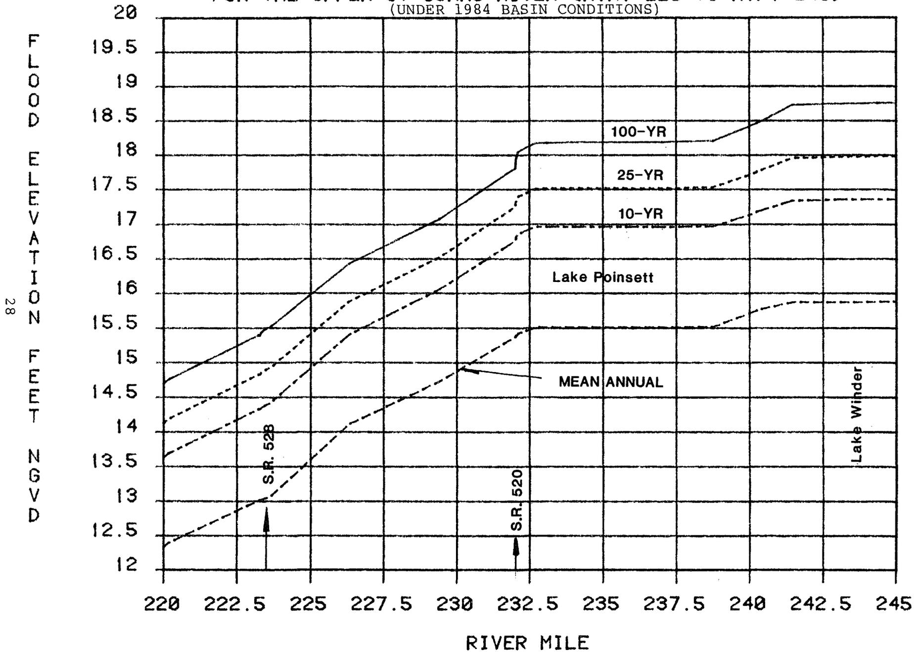
Figure 16. MEAN ANNUAL, 10 YR, 25 YR, AND 100 YR FLOOD PROFILES FOR THE UPPER ST JOHNS RIVER (R.M. 240 TO R.M. 265) (UNDER 1984 BASIN CONDITIONS)
