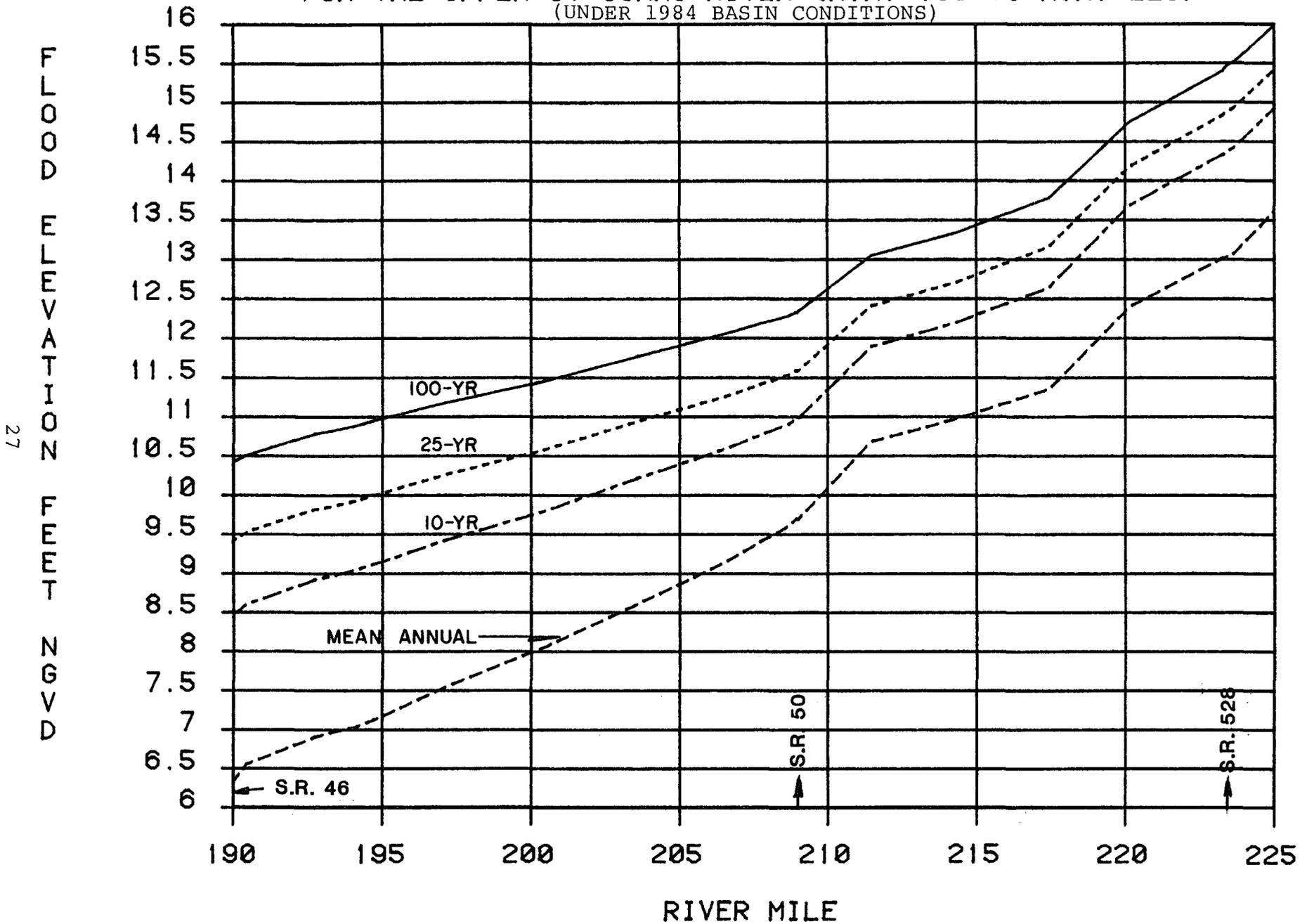
Figure 15. MEAN ANNUAL, 10 YR, 25 YR, AND 100 YR FLOOD PROFILES FOR THE UPPER ST JOHNS RIVER (R.M. 220 TO R.M. 245)
