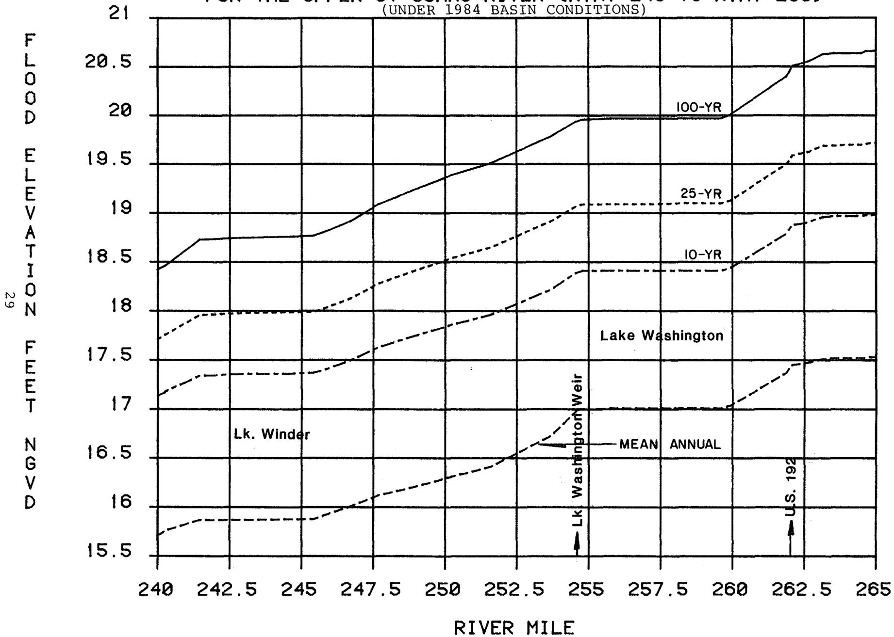
Figure 17. MEAN ANNUAL, 10 YR, 25 YR, AND 100 YR FLOOD PROFILES FOR THE UPPER ST JOHNS RIVER (R.M. 260 TO R.M. 280) (UNDER 1984 BASIN CONDITIONS)
