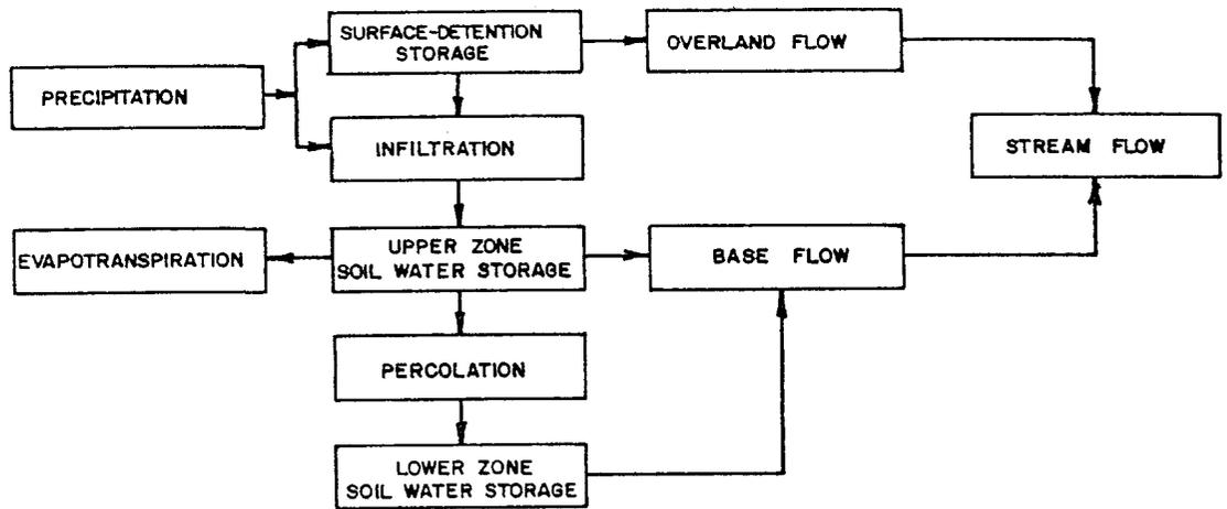
Figure 10. Flow Chart for USJHM Runoff Routine
