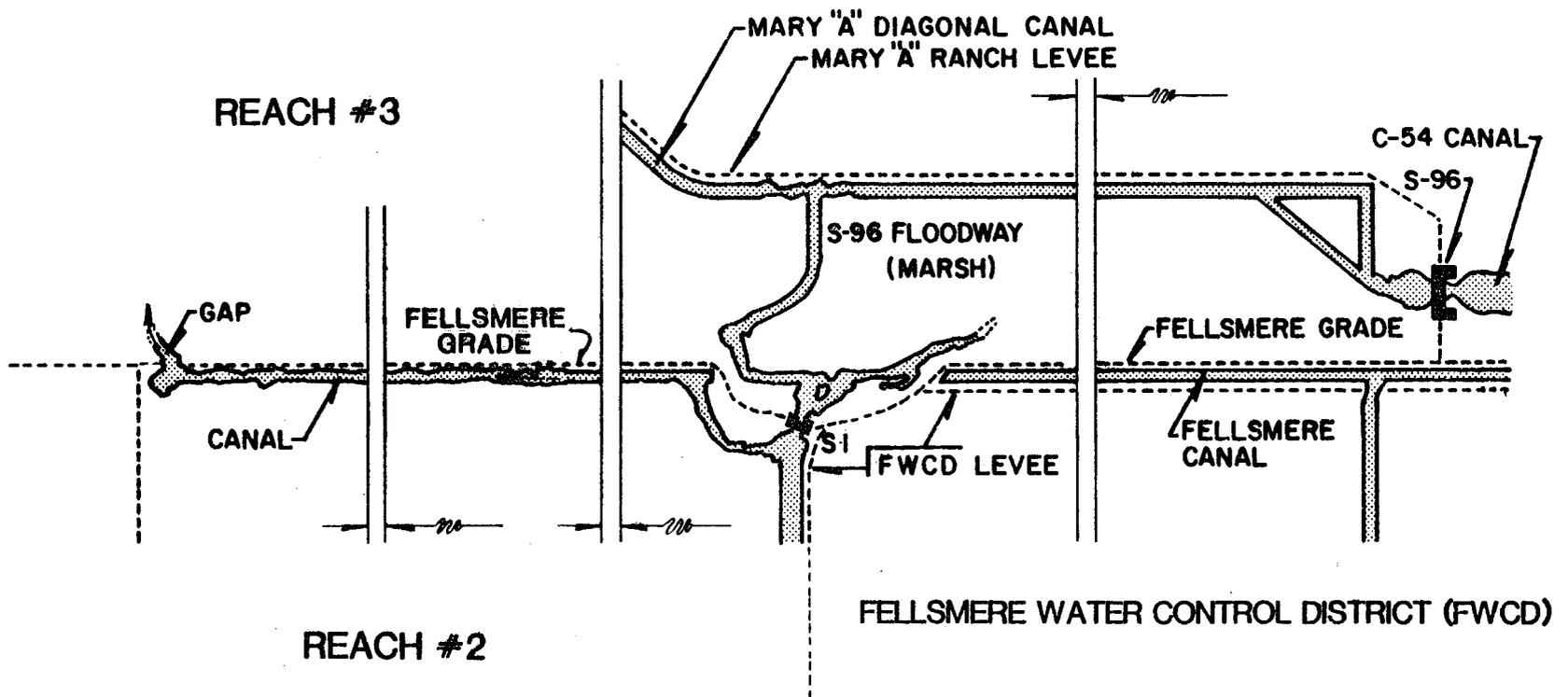
Figure 13. The Canal and Structure Configuration near Fellsmere Grade.
