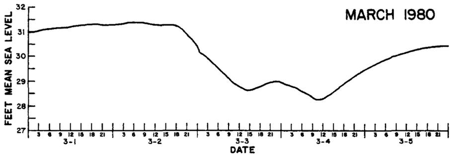
FIGURE 7. -- Hydrographs Showing Fluctuations in the Potentiometric Surface of the Floridan Aquifer at Observation Well 238 Concurrent with the Most Severe Freezes of Winters 1977-80
