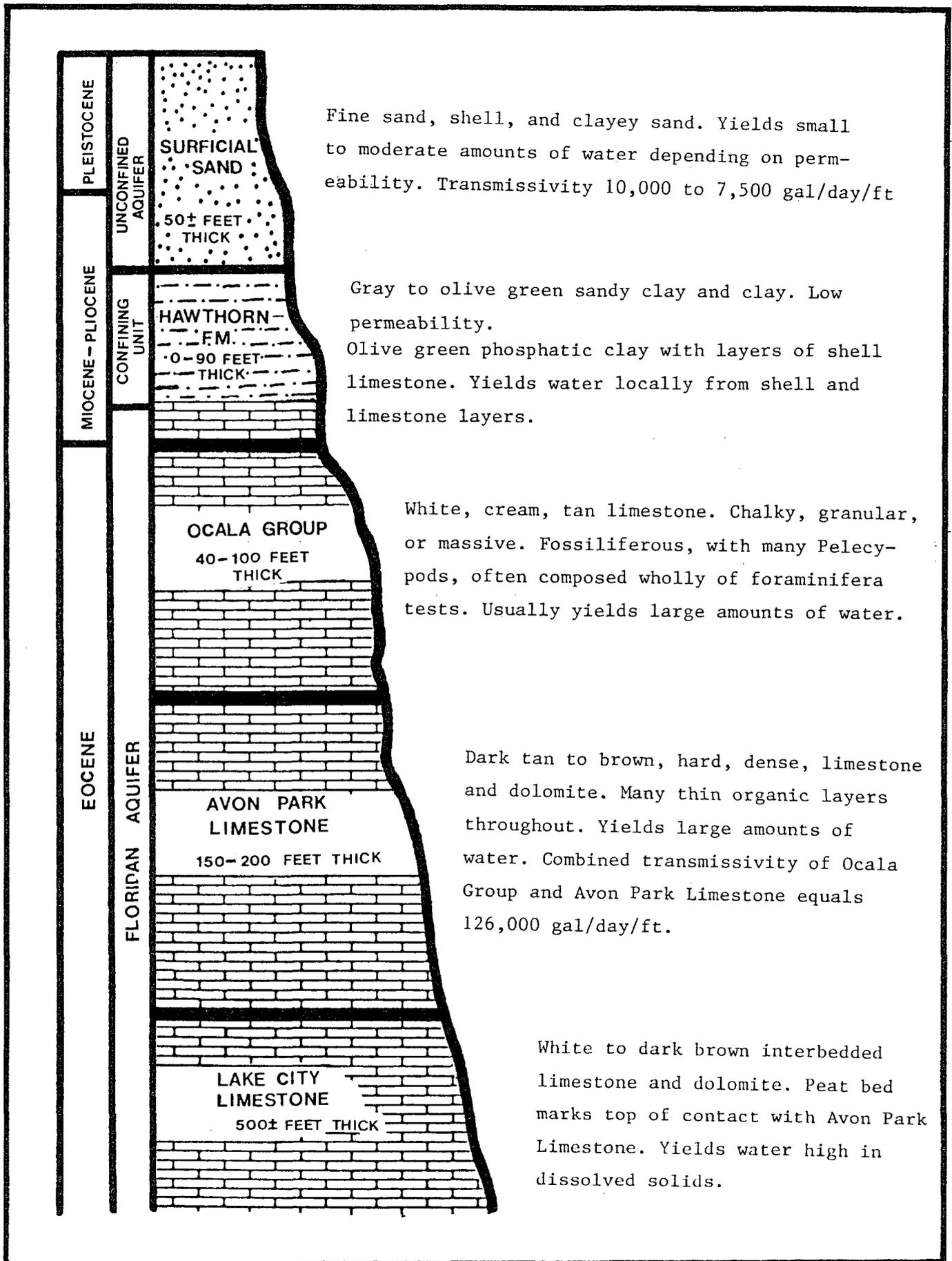
FIGURE 4. -- Idealized Geologic Section of Hydrologically Significant Rock Units Under the Crescent City Ridge
