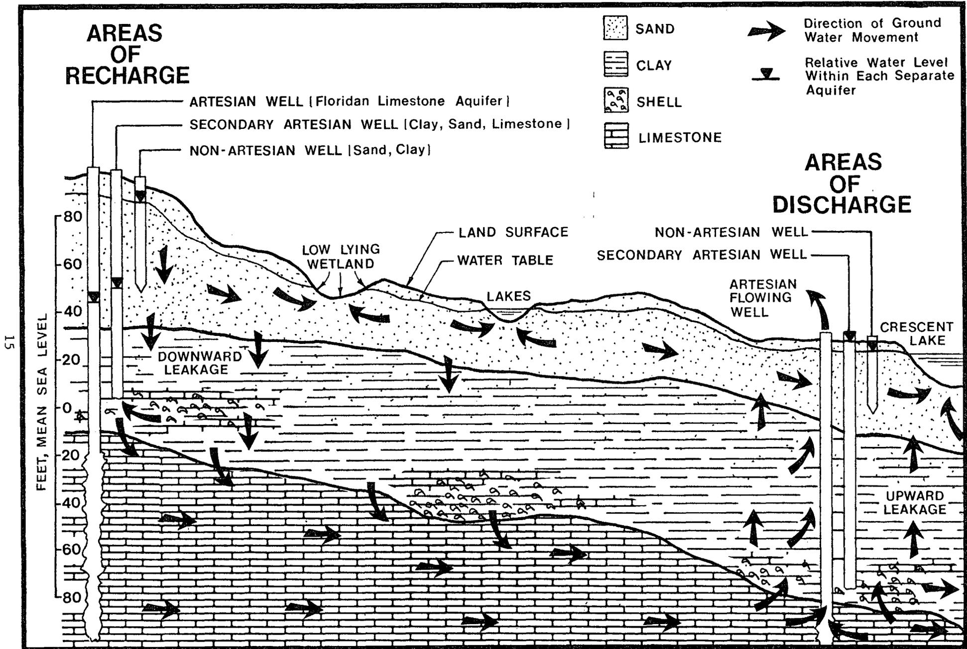
FIGURE 5. -- Diagram Showing Relationship Between Non-Artesian, Secondary Artesian, and Artesian Aquifers on the Crescent City Ridge
