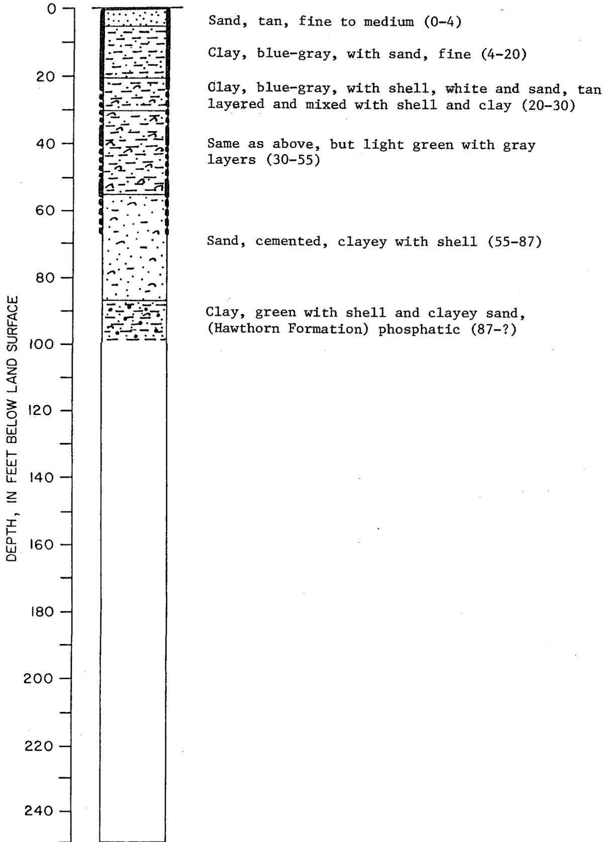
FIGURE C1-15. -- Generalized Picture of Five Test Holes at Mayport Naval Base
