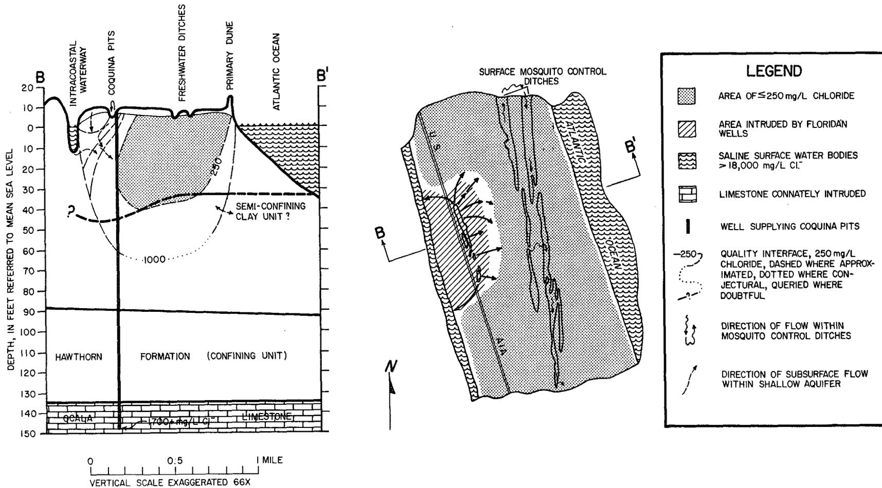
FIGURE 19. -- Cross Section B-B' Showing Shallow Aquifer Pollution by Discharge from Connately Intruded Floridan Wells
