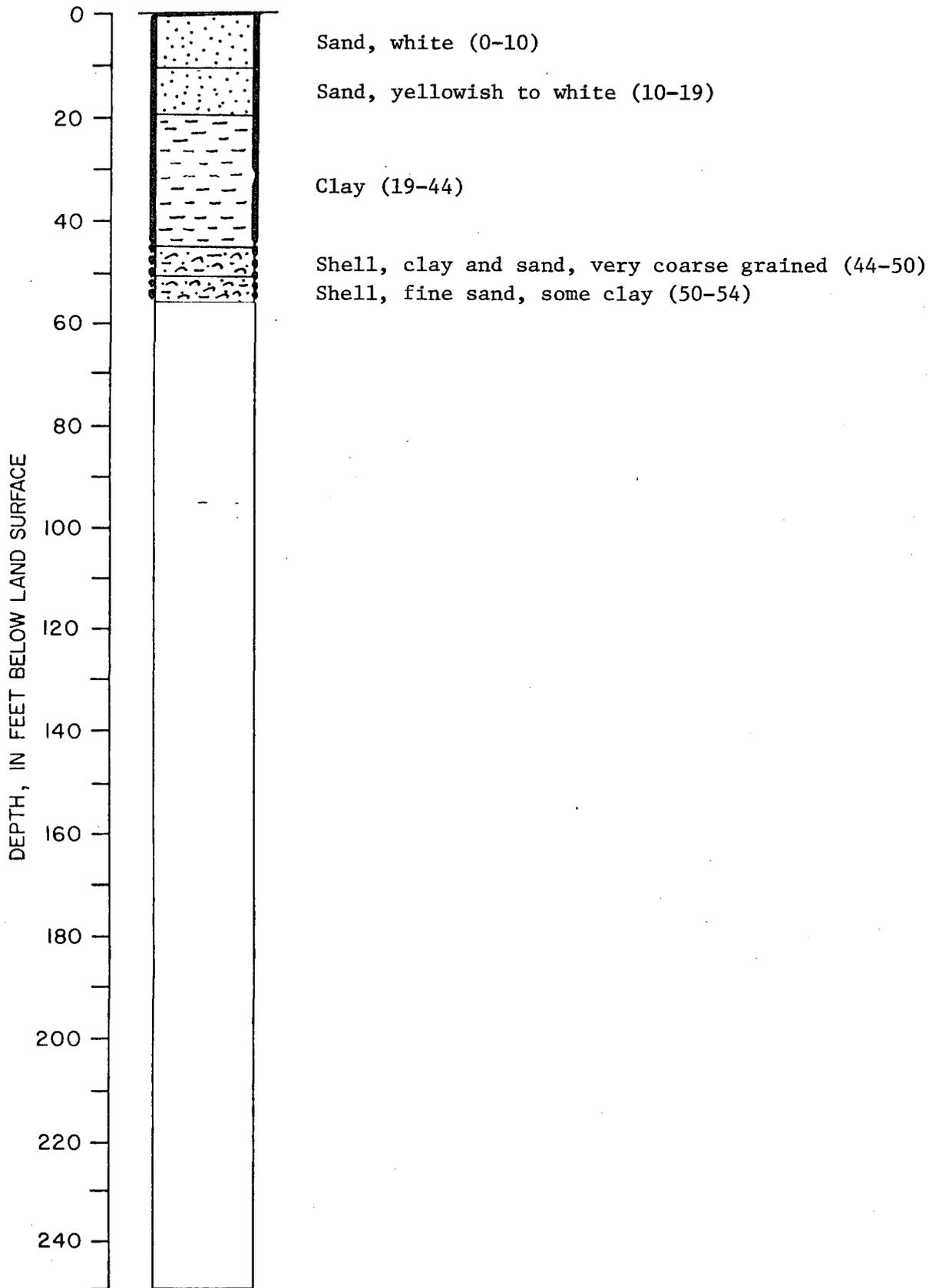
FIGURE C1-13. -- Test Well N-20 at Yulee Forestry Tower
