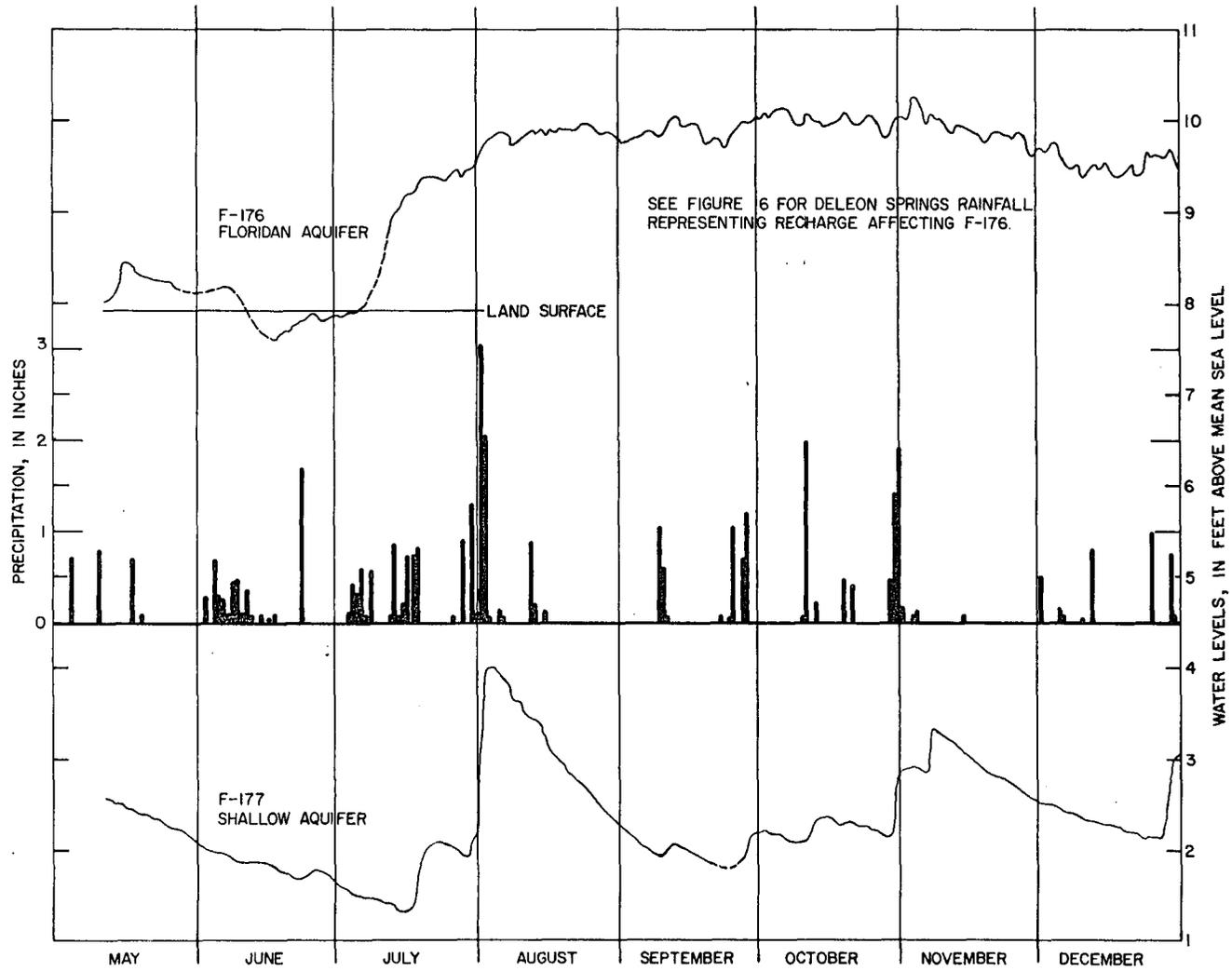
FIGURE 5. -- Hydrographs of a Shallow (F-177) and Floridan (F-176) Aquifer Well Compared With Local Rainfall at Bulow Ruins
