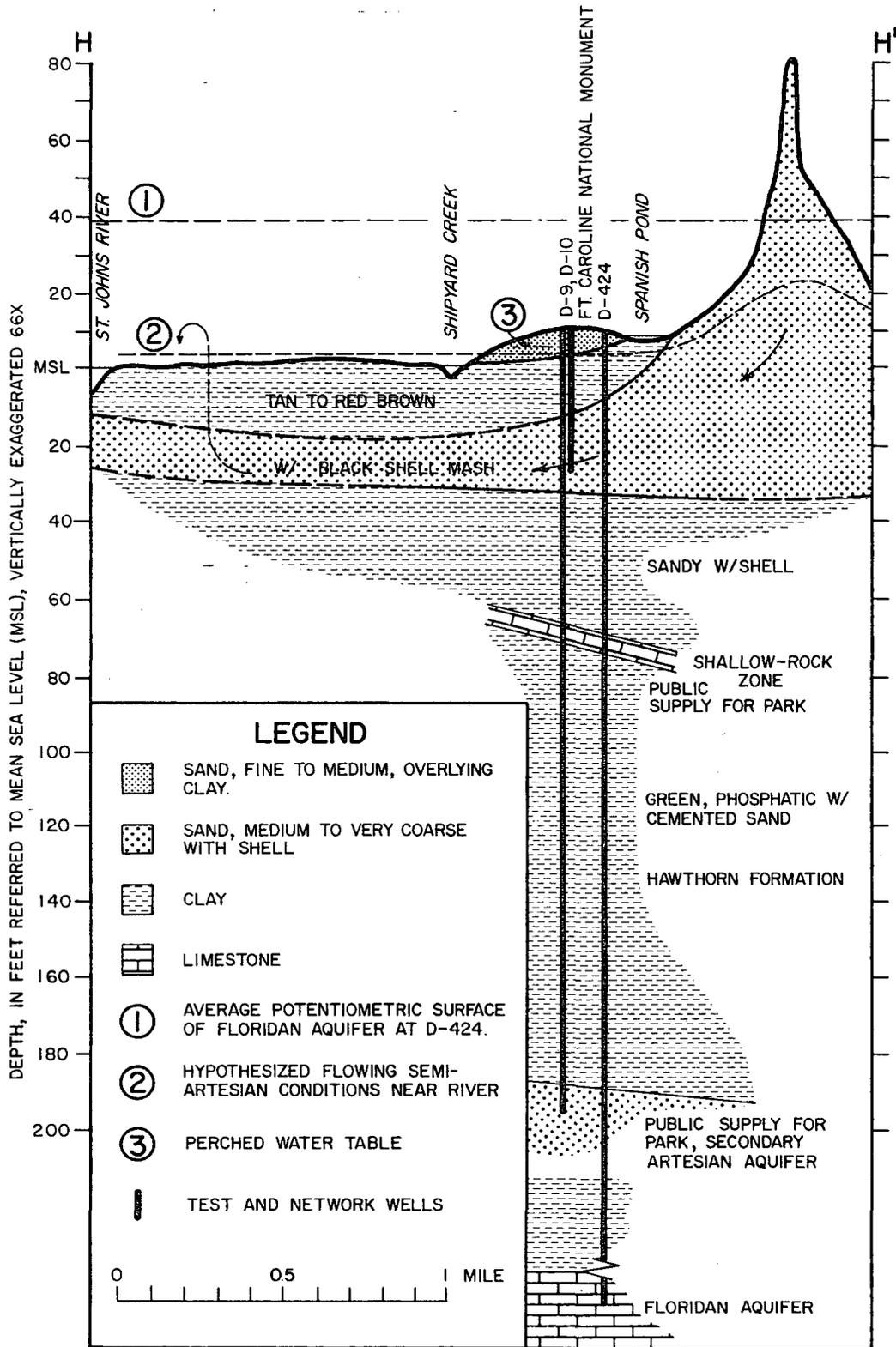
FIGURE 25. -- Generalized Cross Section H-H' at Ft. Caroline National Monument Showing Geology and Aquifers Known to be Present in Local Area
