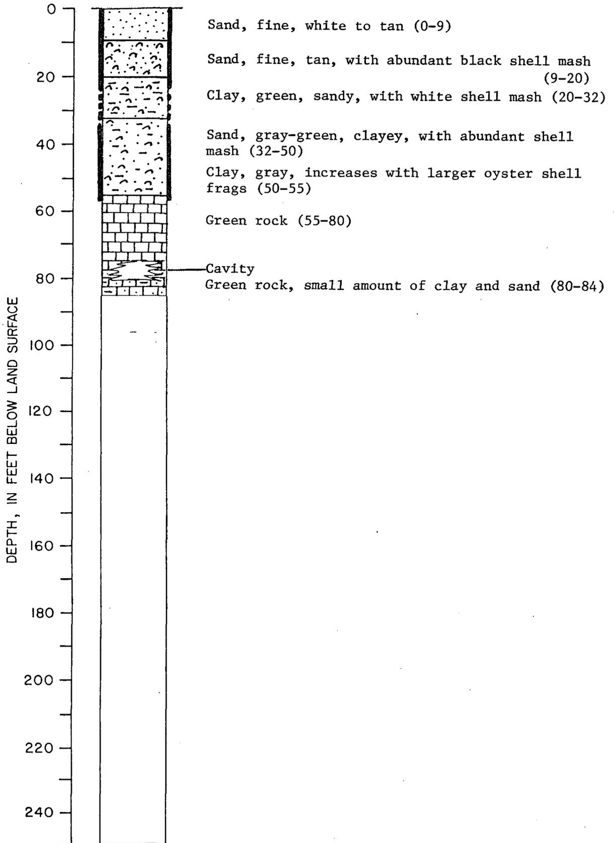
FIGURE C1-11. -- Test Wells N-18 and N-19 at Ft. Clinch State Park
