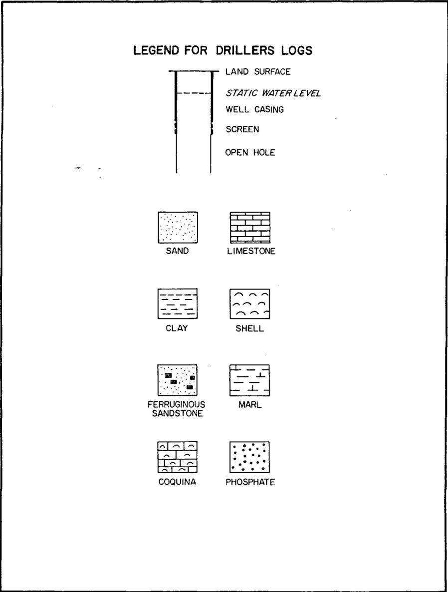
FIGURE C1-1. -- Legend for Drillers' Logs
