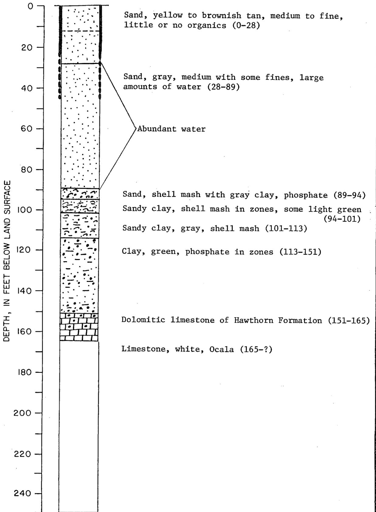
FIGURE C1-6. -- Test Well SJ-499 and DNR Core Hole at Faver Dykes State Park
