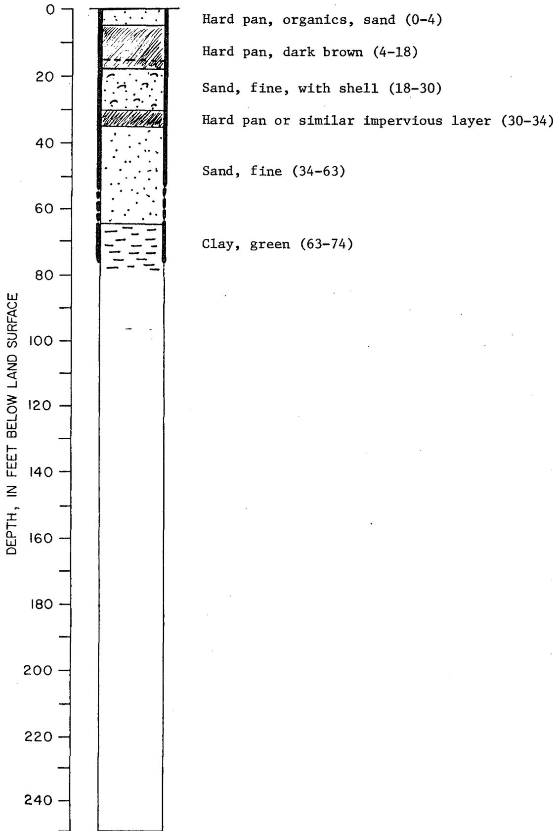
FIGURE C1-7. -- Test Well SJ-500 at Durbin Tower
