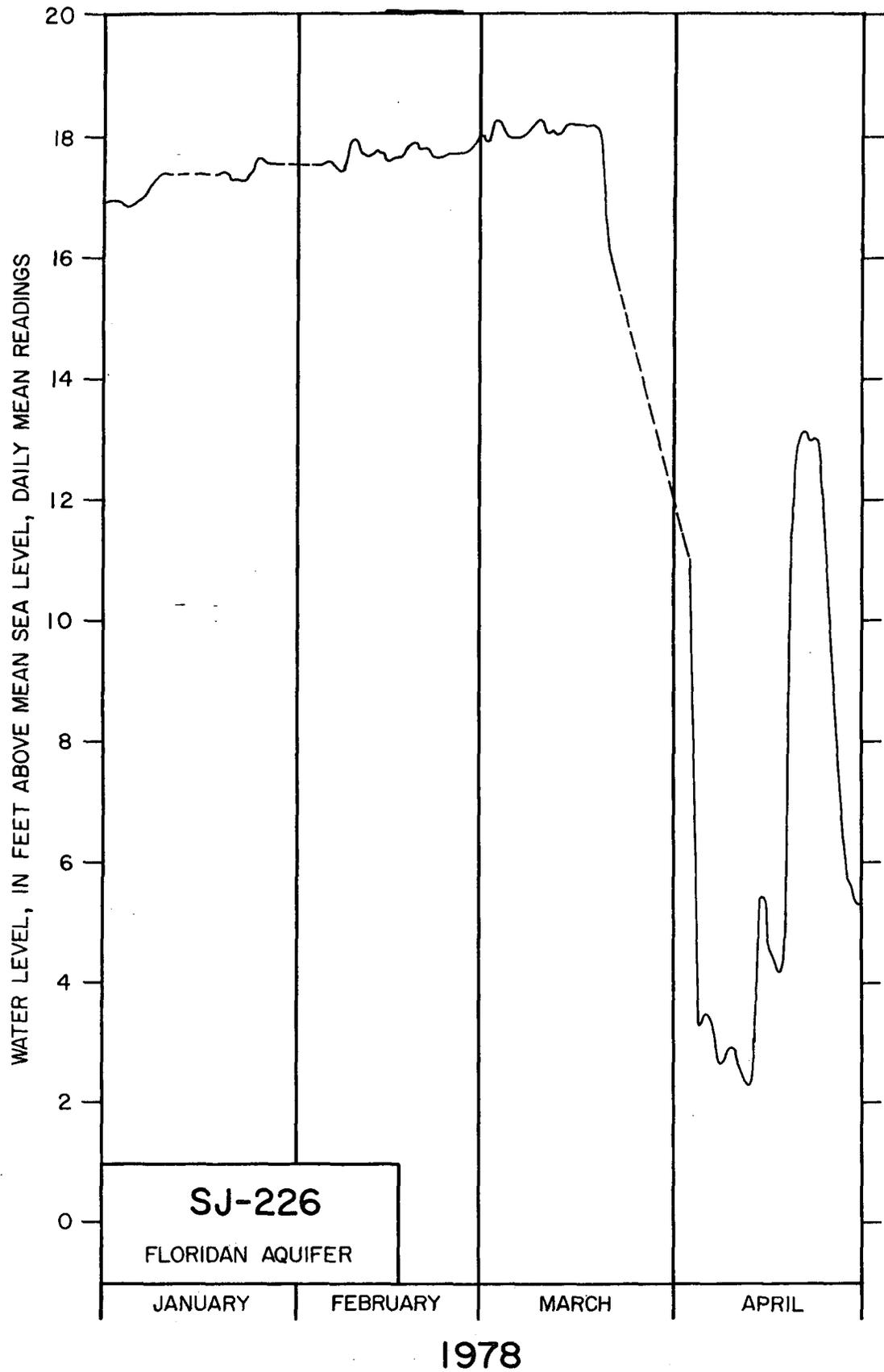
FIGURE 9. -- Typical Water Level Fluctuations Due to Agricultural Pumpage in a Connate Floridan Aquifer Well Near Hastings, Florida
