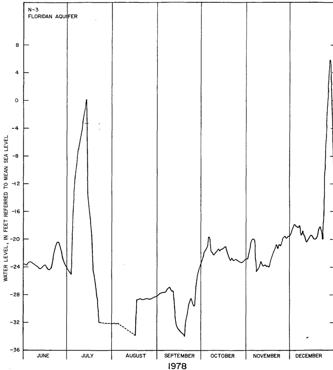
FIGURE 8. -- Typical Water Level Fluctuations Due to Industrial Pumpage of the Floridan Aquifer in the Fernandina Beach Area, Nassau County, Florida
