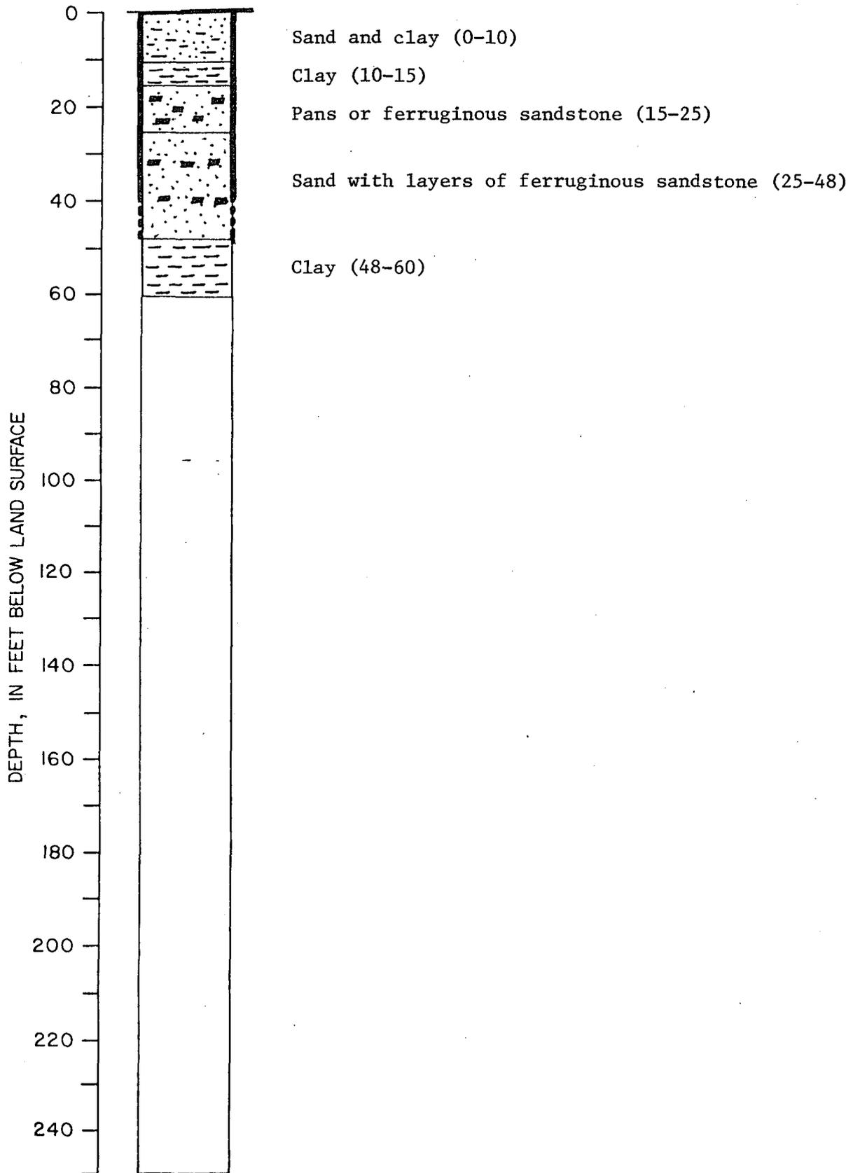
FIGURE C1-14. -- Test Well D-14 at Tisonia Forestry Tower
