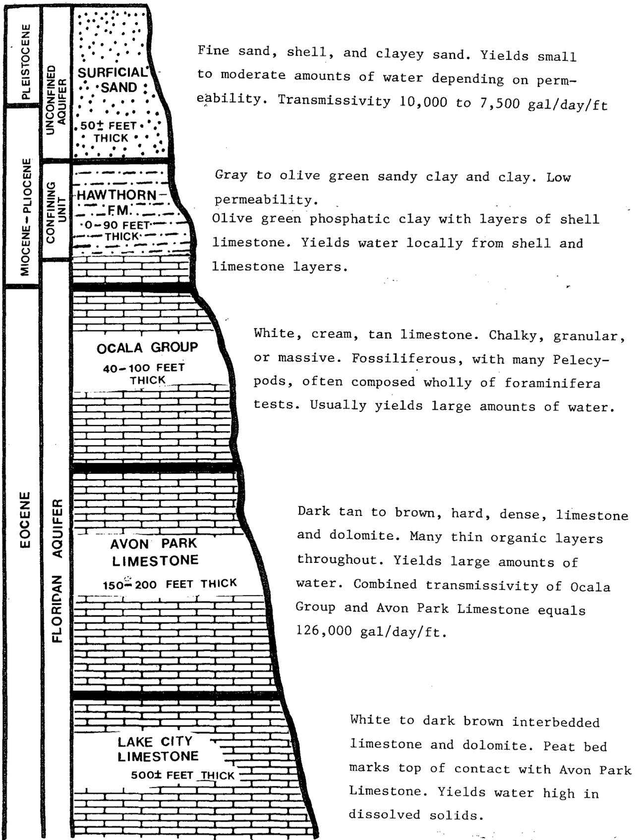
FIGURE 5. -- Idealized Geologic Section of Hydrologically Significant Rock Units Under the Crescent City Ridge
