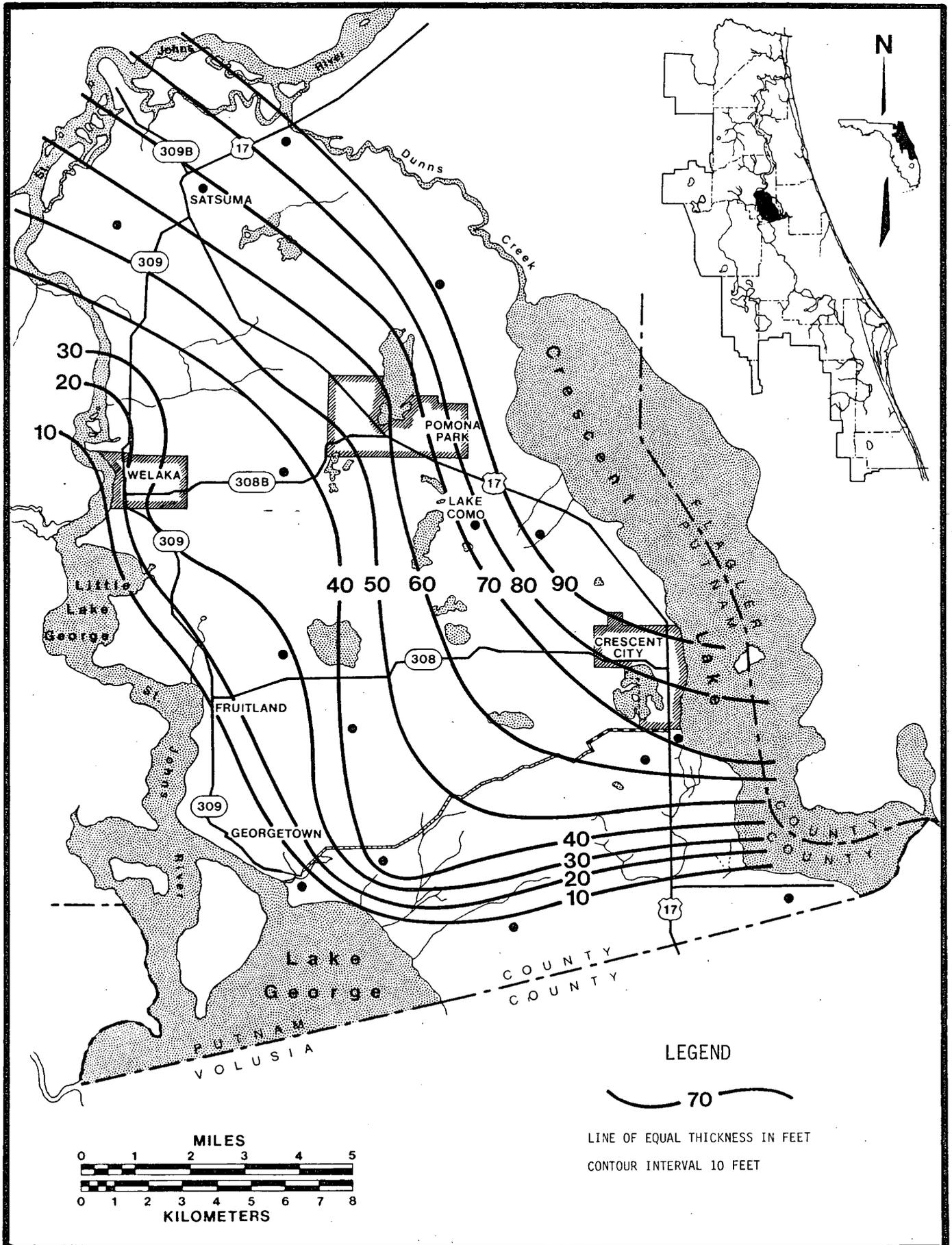
FIGURE 7. -- Map of Crescent City Ridge Showing Thickness of Confining Unit for the Floridan Aquifer
