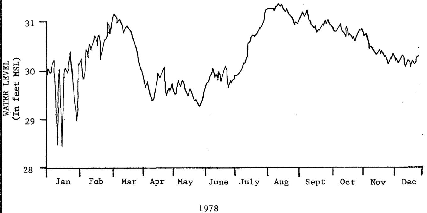
FIGURE 14. -- Hydrograph of Daily Mean Water Levels at Floridan Aquifer Well No. 238 for Years 1977-78
