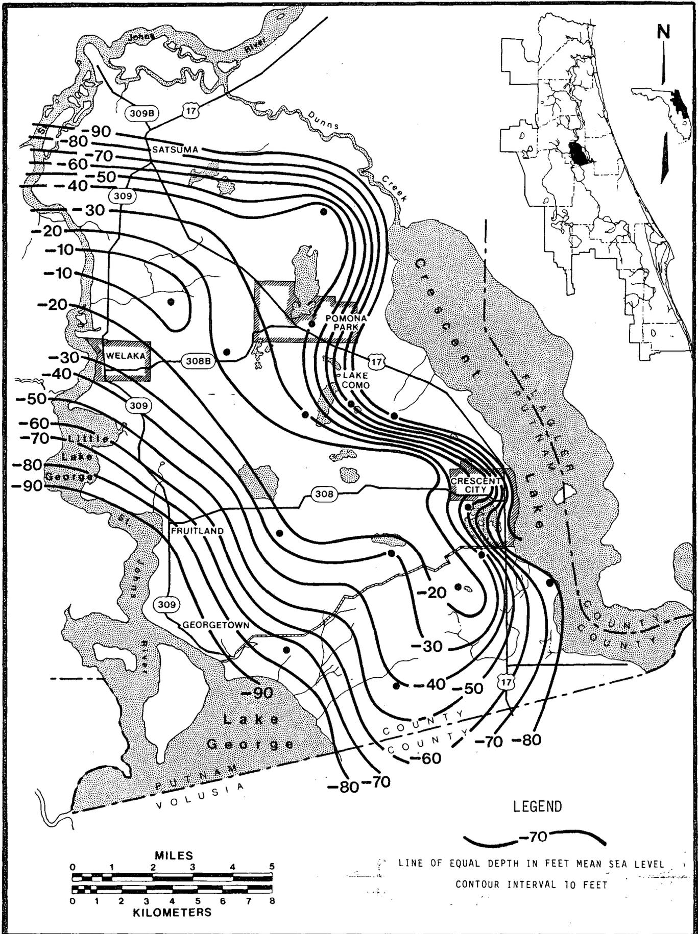
FIGURE 6. -- Map of Crescent City Ridge Showing Elevation of Top of Rock Forming the Floridan Aquifer
