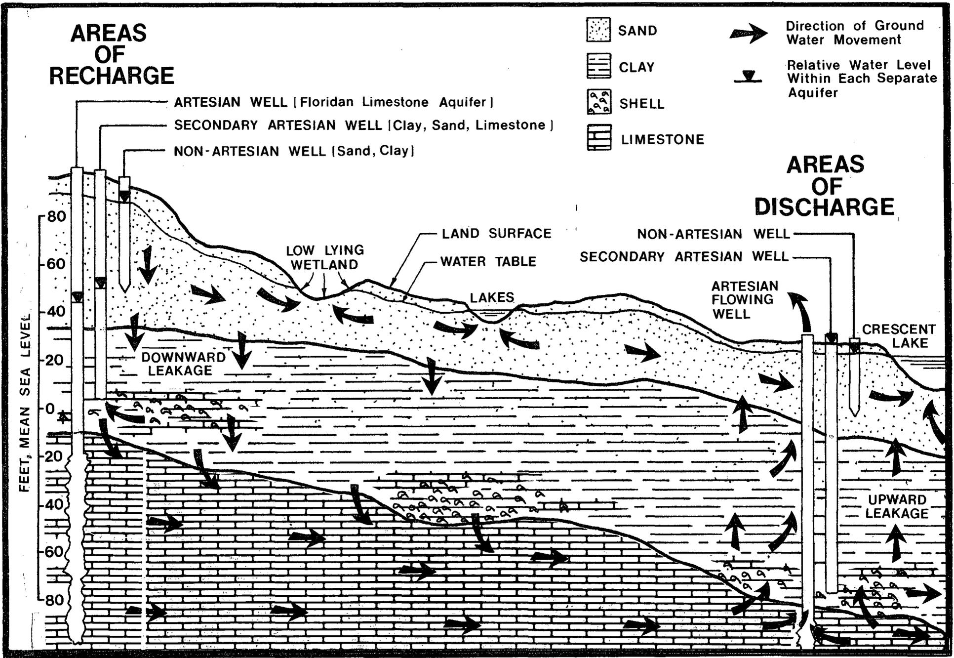
FIGURE 10. -- Diagram Showing Relationships Between Non-Artesian, Secondary Artesian, and Artesian Aquifers on the Crescent City Ridge
