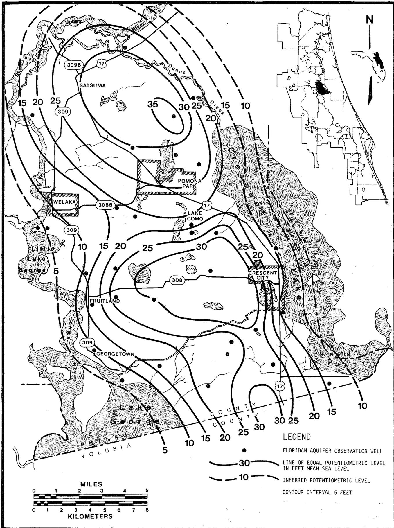
FIGURE 3. -- Map of Crescent City Ridge Showing Potentiometric Surface of Artesian Aquifer for May 1978
