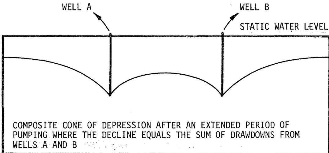
FIGURE 34. -- Development of Composite Cones of Depression by Simultaneous Pumping Wells
