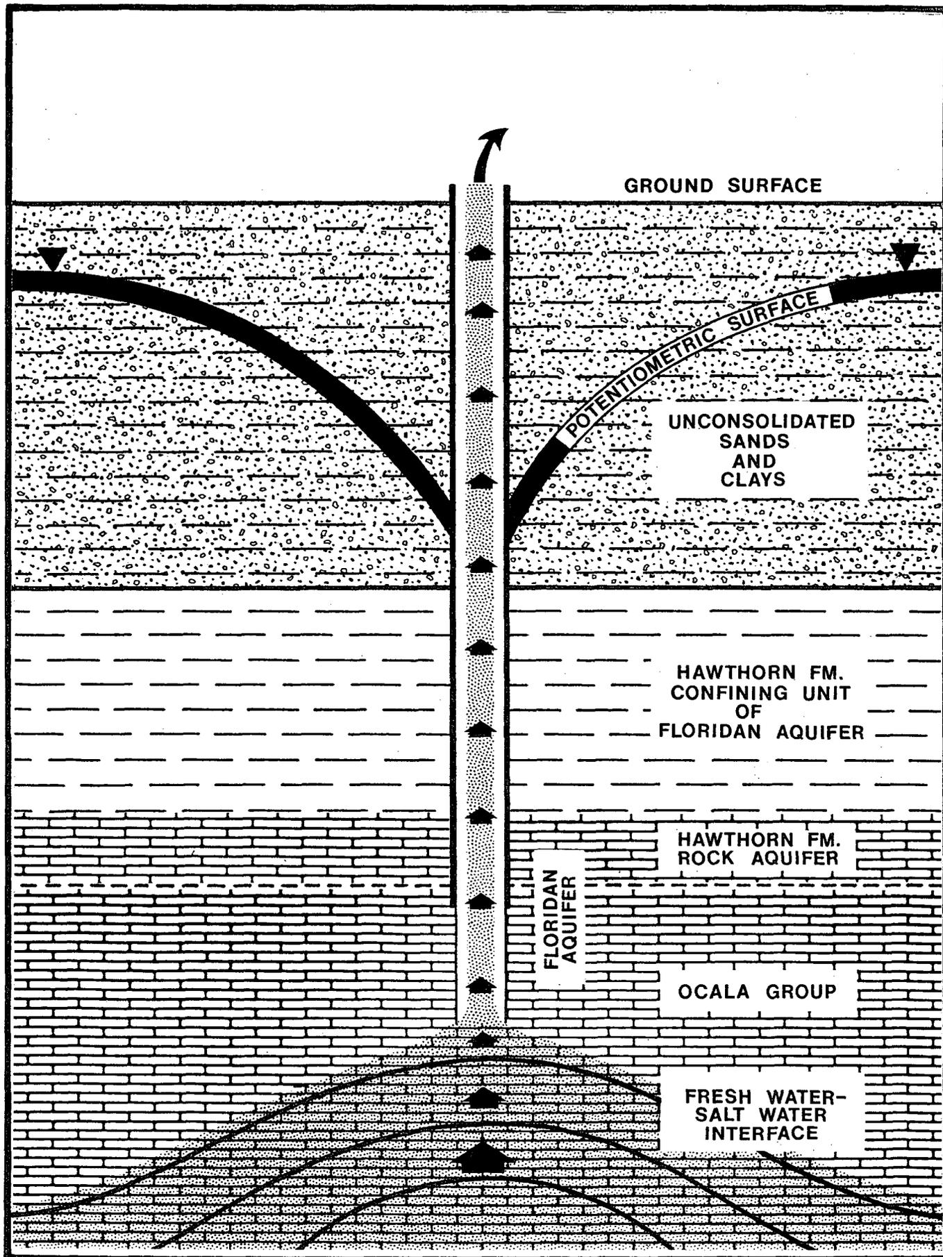
FIGURE 35. -- Schematic Diagram of Salt Water Coning as Related to the Tri-County Area
