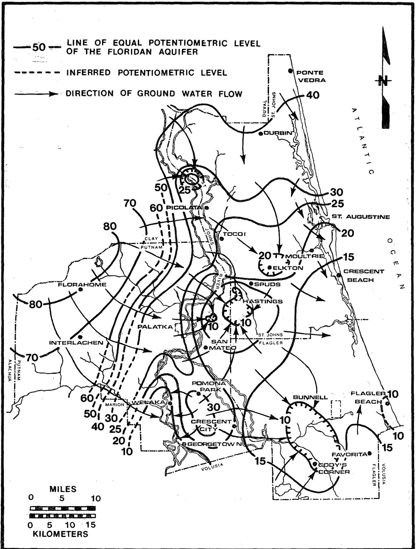
FIGURE 29. -- Potentiometric Level and Generalized Direction of Ground Water Movement Within the Tri-County Area, March 1975
