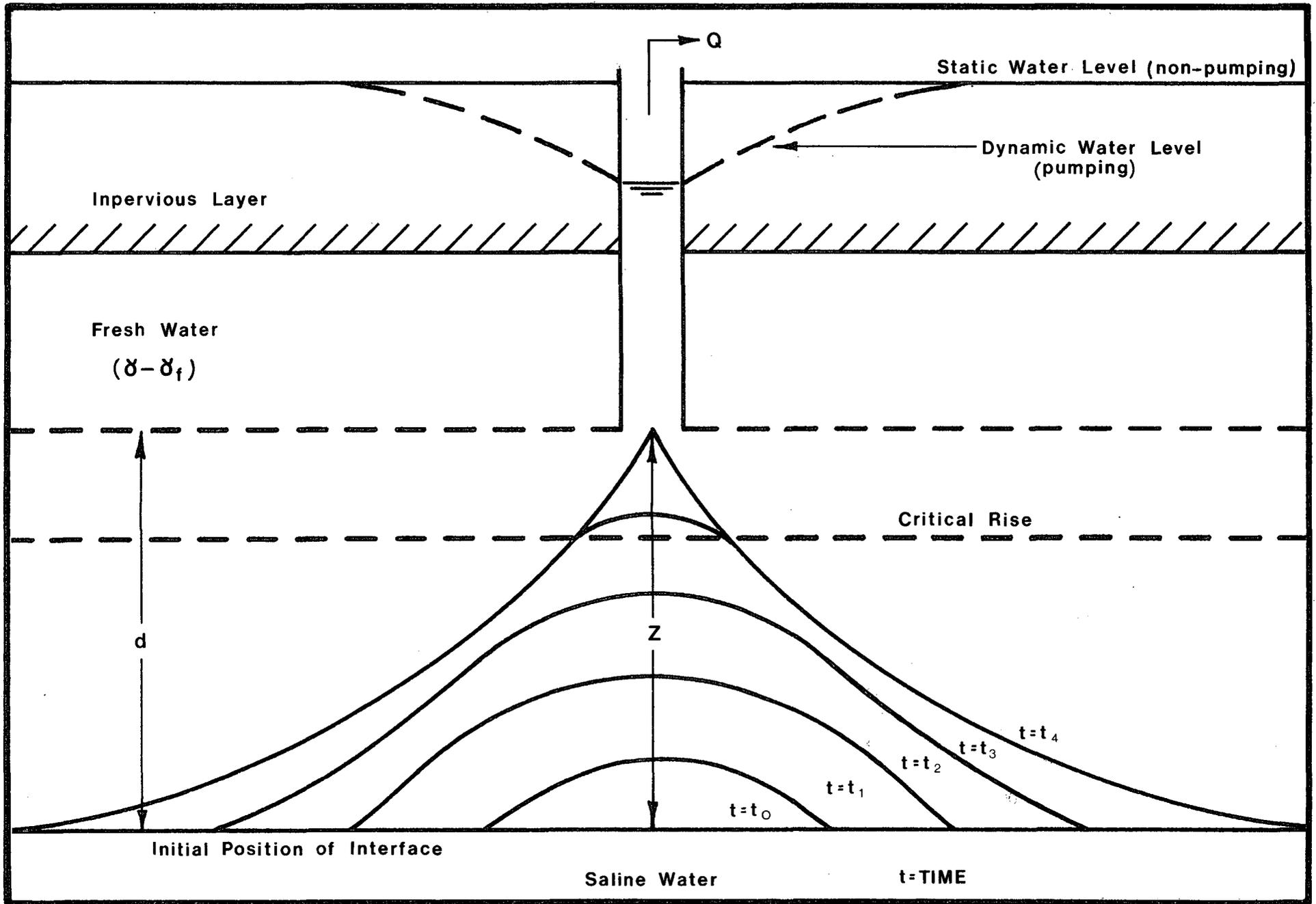
FIGURE 36. -- Upconing of an Abrupt Interface Below a Pumping Well (After Muskat, 1946 and Bear and Dagan, 1964 and 1968)
