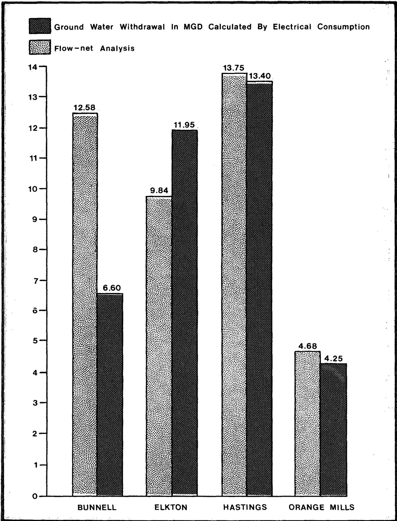
FIGURE 31. -- A Comparison of the Ground Water Withdrawals as Calculated by the Electrical Consumption Method and by Flow-Net Analysis
