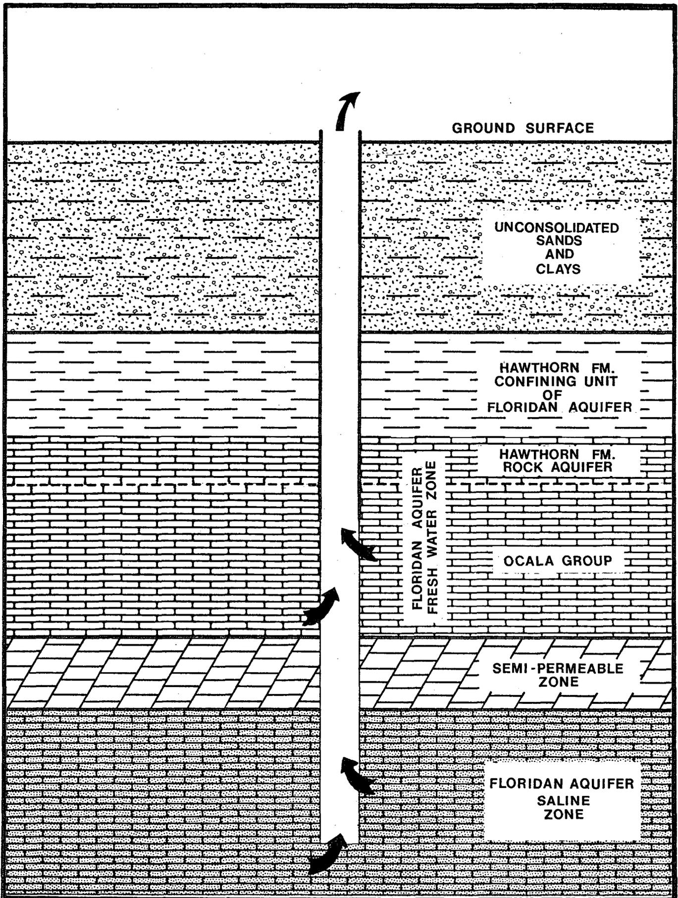
FIGURE 32. -- Diagram Showing the Contamination of the Fresh Zone Within the Floridan Aquifer from the Deeper Saline Zone
