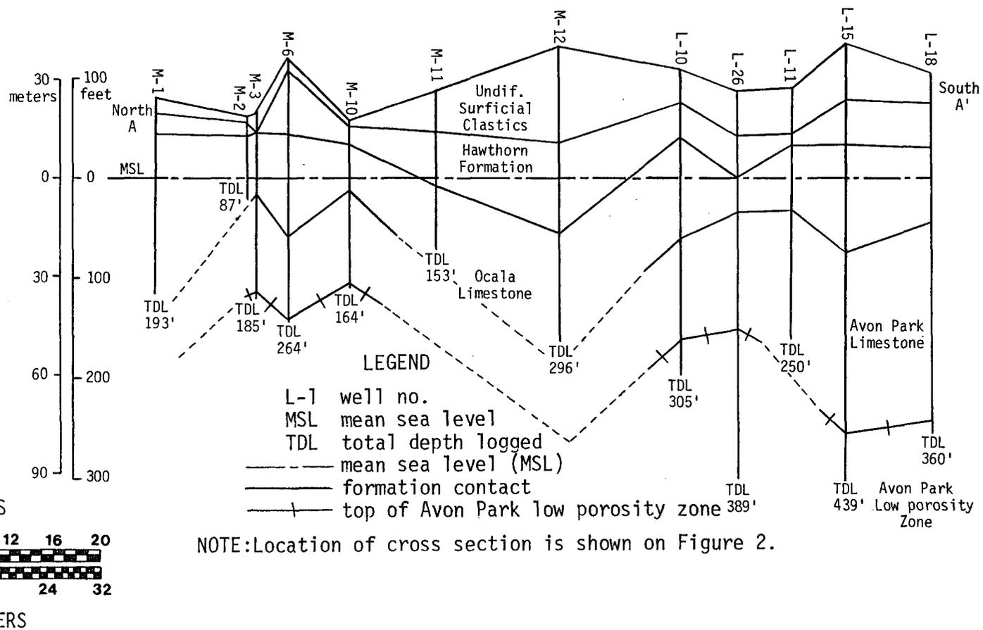
Figure 5. North South Cross Section A-A'
