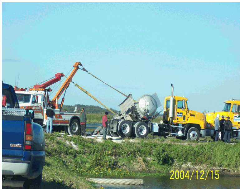
Figure 25. Getting tow truck assistance after tanker slides off levee.
