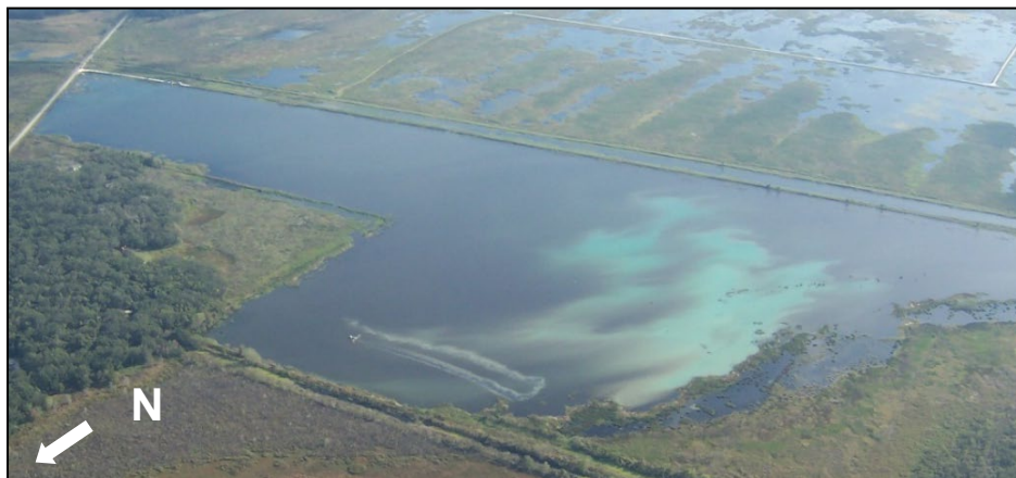
Figure 24. Trail of liquid alum floc in S.N. Knight North.
