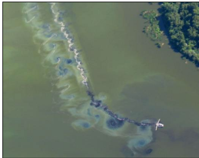
Figure 33. A plume of sediment (dark color) being suspended behind the barge during an application at Lake Harris Conservation Area.
