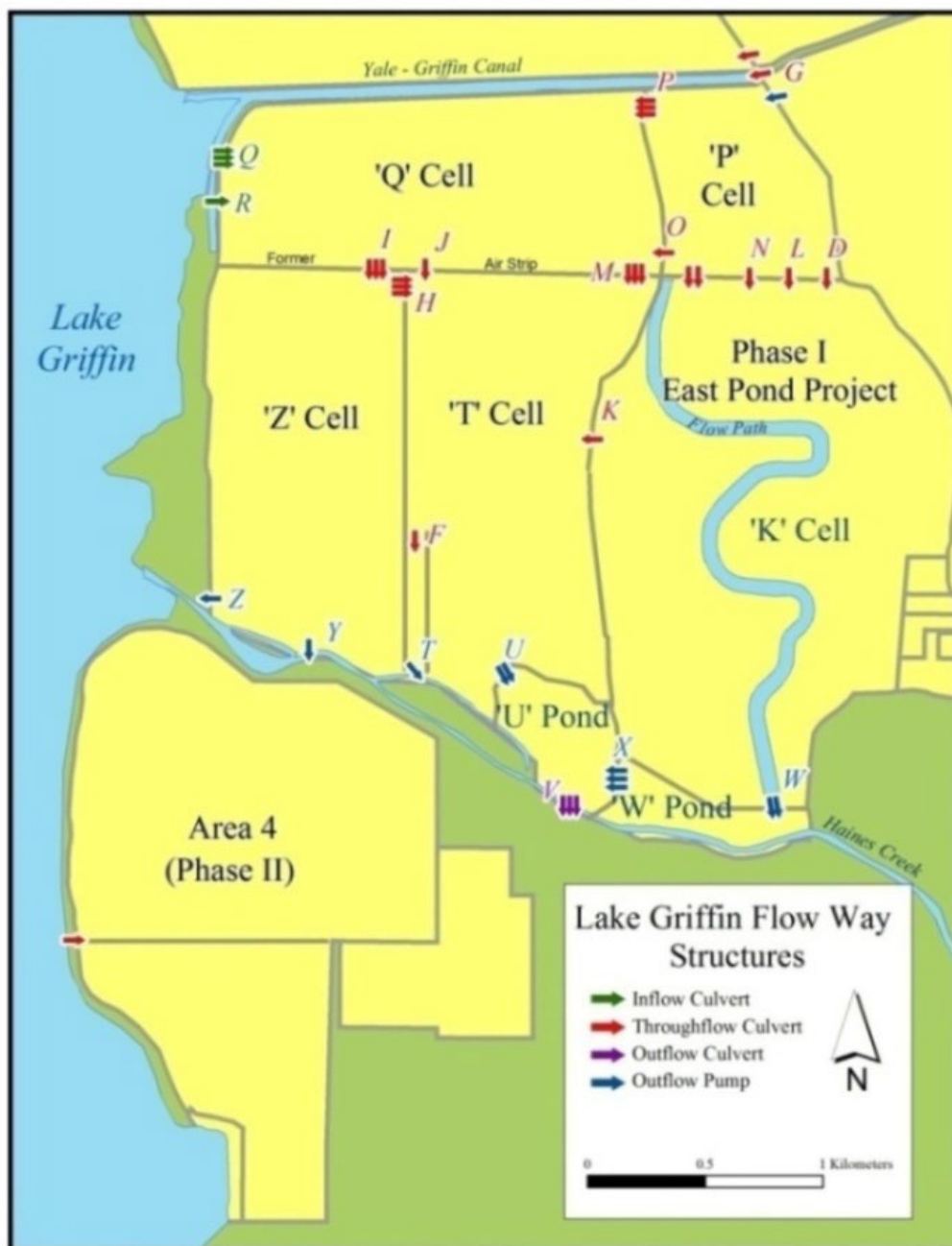
Figure 2. Lake Griffin Flow-Way and connection structures.
