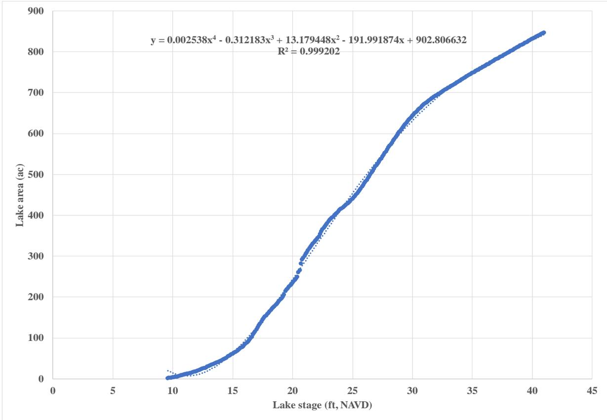
Figure D-2. Relationship between lake level and surface area at Lake Butler west
