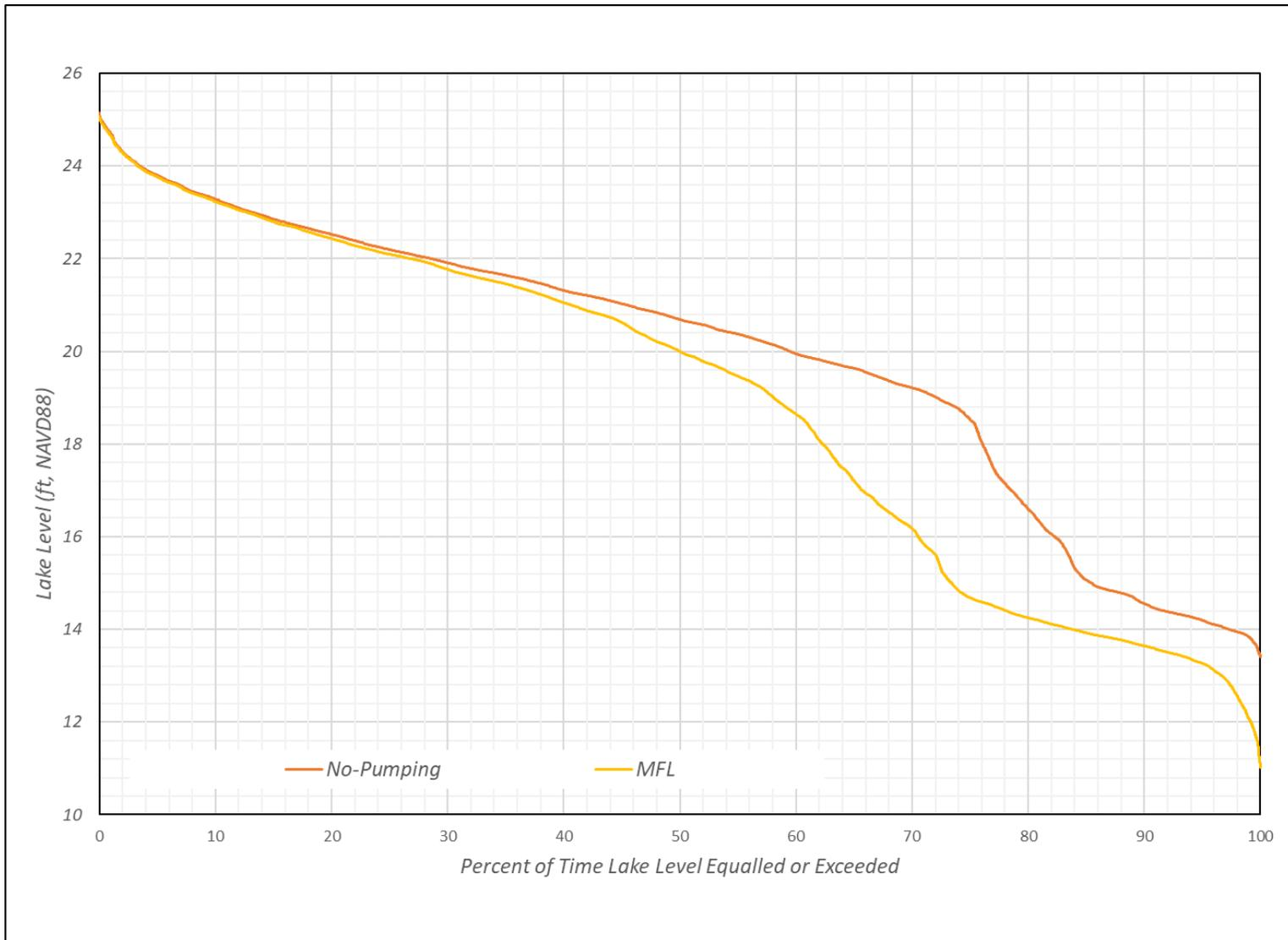
Figure D-1. No-pumping condition and MFLs condition exceedance curves for Lake Butler
