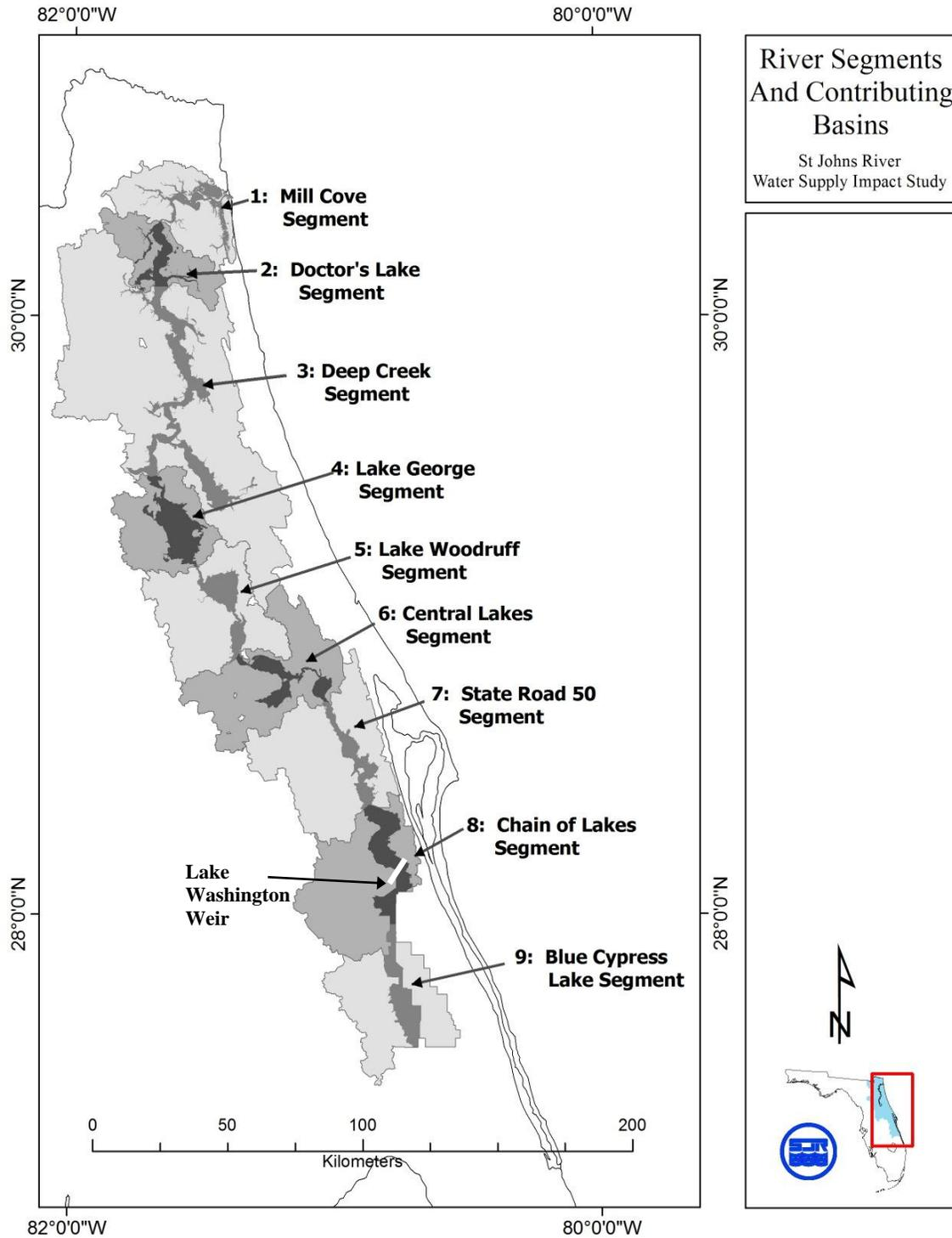
Figure 3-1. River segments in the St. Johns River with their associated wetland areas (shaded in dark grays) and drainage basins (shaded in light grays). The white line in segment 8 shows the approximate location of the Lake Washington weir, which is the southern terminus of the analyses of possible effects from water withdrawals.
