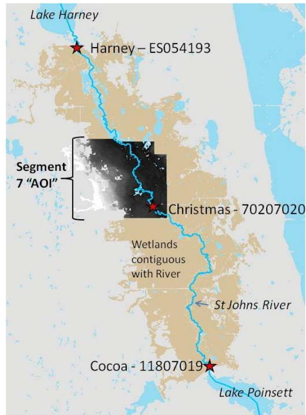
Figure 15. Location of stage gages in the St. Johns River for Segment 7 Hydroperiod Tool analysis. Note that the Cocoa station was used for the Segment 8 HT work.
