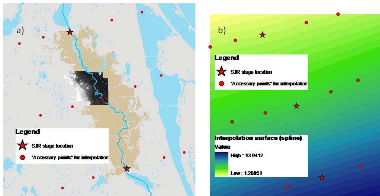
Figure 16. Interpolation of water surface for segment 7 study area. a) Distribution of “accessory” points across the floodplain necessary to generate surface in GIS; b) an interpolated surface. Note the diagonal distribution of elevations in figure b, extending River stage values perpendicular to the general direction of the River.
