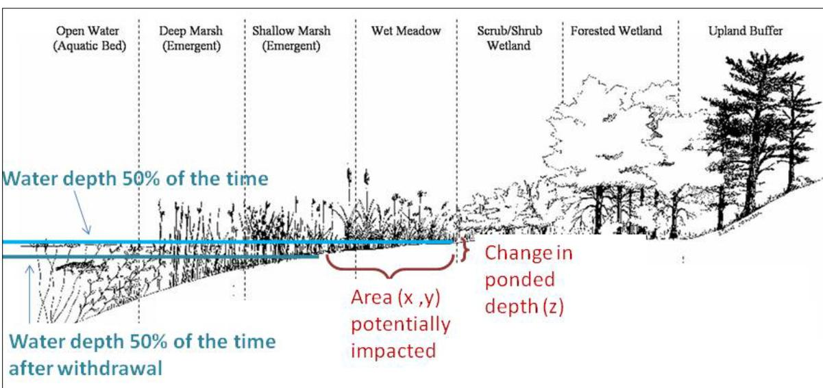
Figure 7. Areal effect of change in River stage ( $z$ ) as seen in cross sectional representation of the 50% exceedence water level and the resulting area of inundation for both the historical (natural) condition and a proposed withdrawal scenario. (Wetland cross section Figure from [http://www.newp.com/pdf/NEWP\\_WetlandCrossSection.pdf](http://www.newp.com/pdf/NEWP_WetlandCrossSection.pdf))
