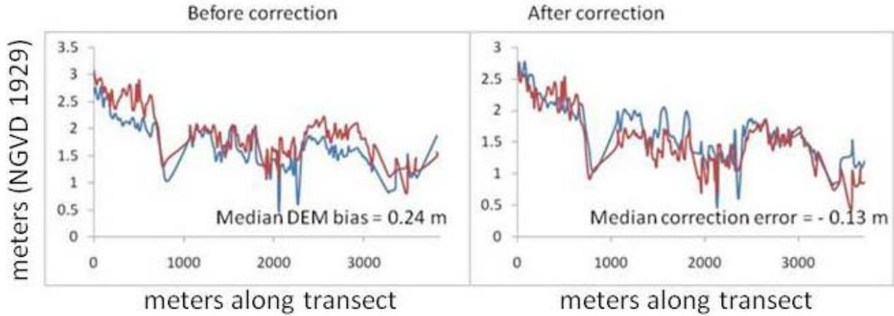
Figure 20. H-1 transect comparison of DEM elevation to MFL elevation before and after DEM correction. N = 203, emergent aquatic vegetation removed. Blue lines in both Figures represent the MFL surveyed elevation and the red lines are the LiDAR-derived DEM elevations.
