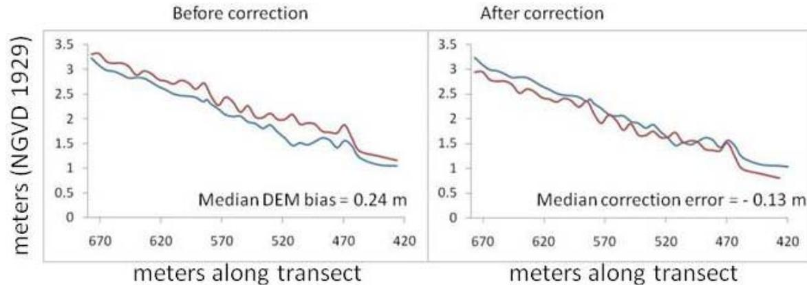
Figure 21. Ruth transect comparison of DEM elevation to MFL elevation before and after DEM correction. N = 40, emergent aquatic vegetation removed. Blue lines in both Figures represent the MFL surveyed elevation and the red lines are the LiDAR-derived DEM elevations.
