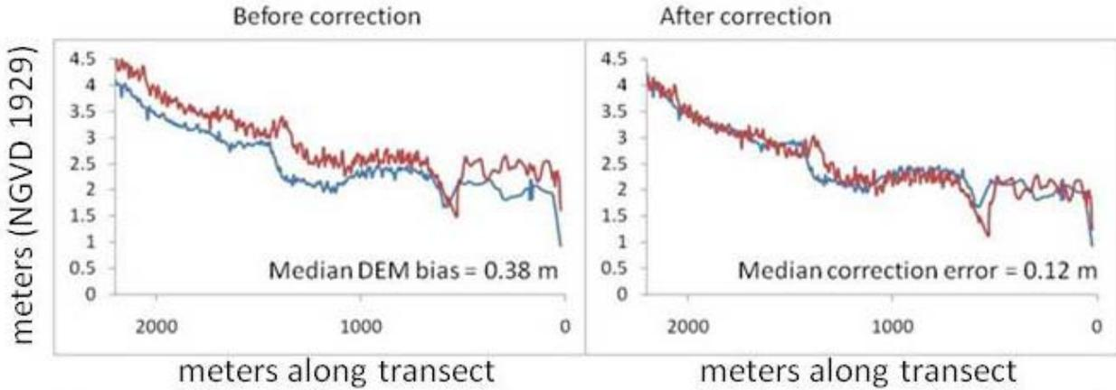
Figure 18. Cone transect comparison of DEM elevation to MFL elevation before and after DEM correction. N = 321, emergent aquatic vegetation removed. Blue lines in both Figures represent the MFL surveyed elevation and the red lines are the LiDAR-derived DEM elevations.
