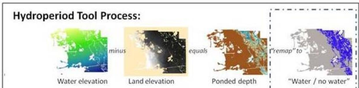
Figure 3. Basic Hydroperiod Tool function. Within the GIS a process commonly referred to as “Raster Math” executes a simple subtraction for each grid cell, subtracting the land elevation from the water elevation, to produce a new raster containing the water depth (ponded depth) for each grid cell.
