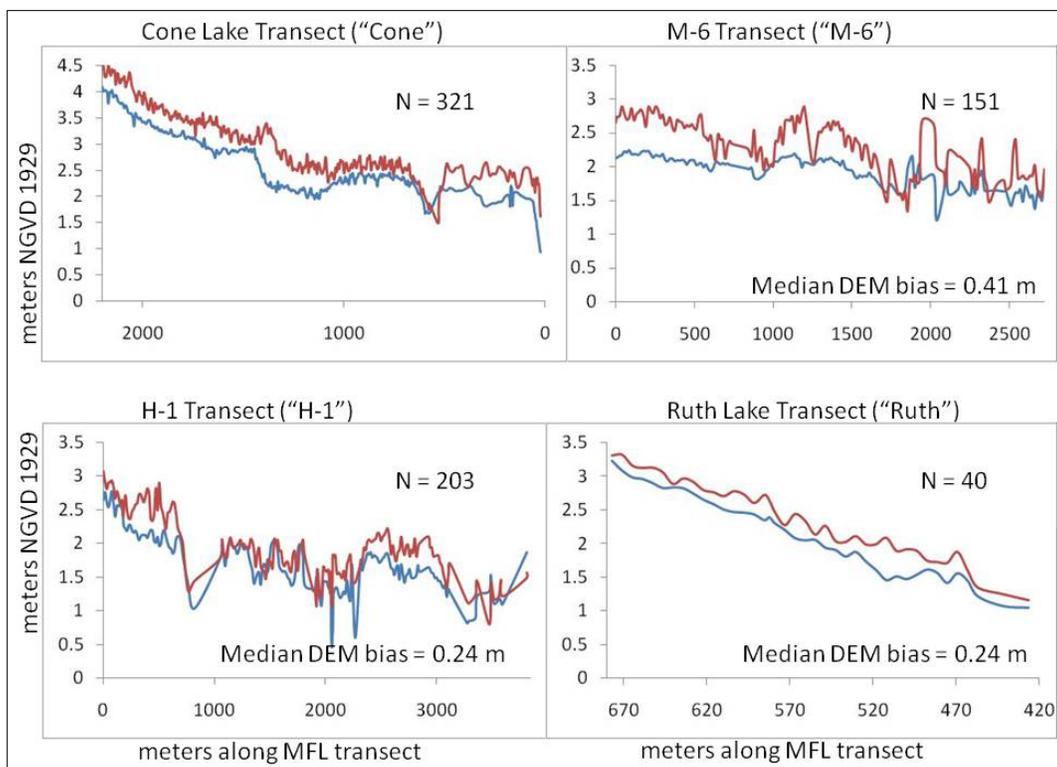
Figure 12. Comparison of LiDAR-derived DEM elevation to MFL survey elevation. Blue lines in all Figures represent the MFL surveyed elevation and the red lines are the LiDAR-derived DEM elevations.
