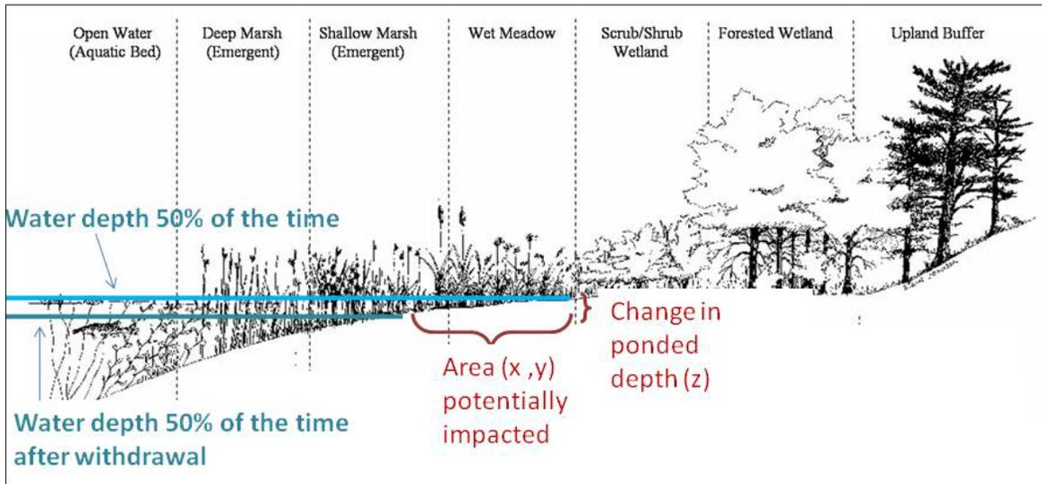
Figure 5. Cross sectional representation of the 50% exceedence water level and the resulting area of inundation for both the historical (natural) condition and a proposed withdrawal scenario. (Wetland cross section Figure from [http://www.newp.com/pdf/NEWP\\_WetlandCrossSection.pdf](http://www.newp.com/pdf/NEWP_WetlandCrossSection.pdf))
