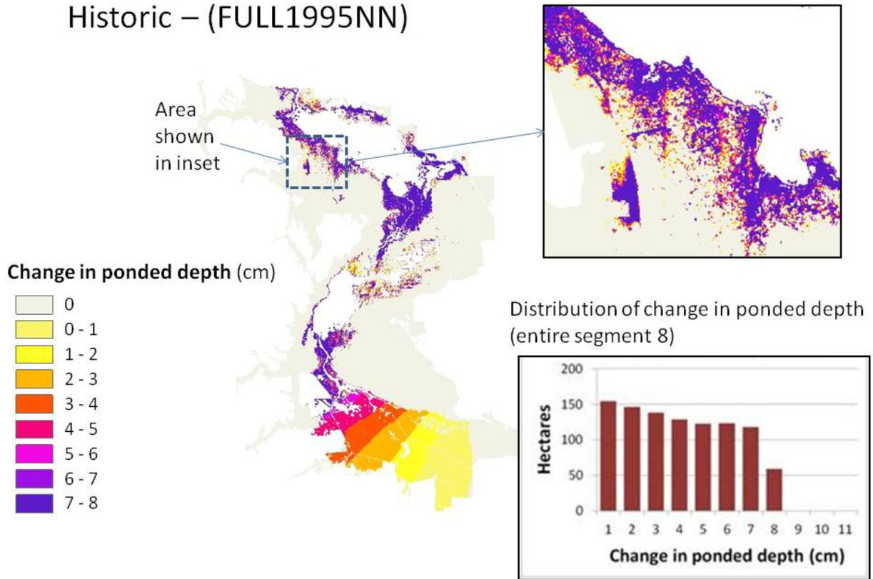
Figure 38. Change in ponded depth in areas remaining inundated at the 50% exceedence level for segment 8. Prepared for Floodplain Wildlife chapter, by subtracting results shown in Figure 37 from Figure 36. Note that most of the change is the result of areas that were historically being inundated no longer being inundated at this exceedence.
