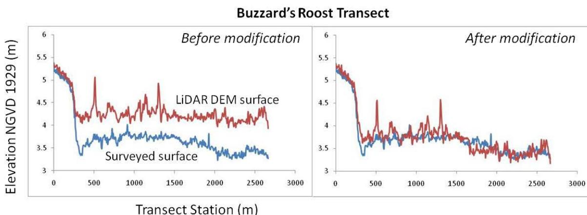
Figure 13. LiDAR surface before and after adjustment to fit surveyed transect, sample transect from Segment 8 (from Wetlands chapter).
