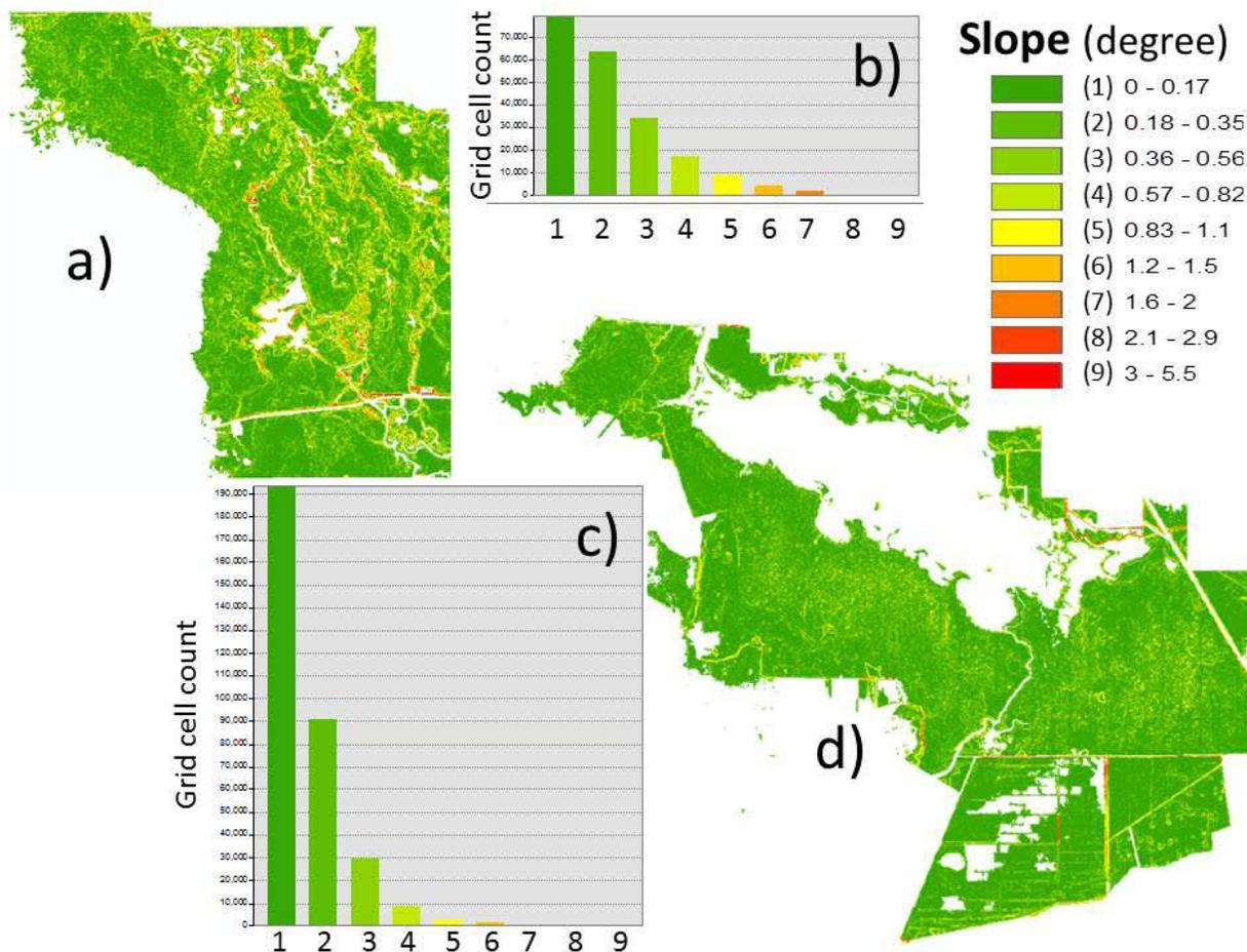
Figure 25. Distribution of DEM slope within St. Johns River floodplain. a) Segment 7 slope raster. b) Histogram demonstrating the distribution of slope in Segment 7 DEM, c), Histogram demonstrating the distribution of slope in Segment 8 DEM, d) Segment 8 slope raster. Legend is for both Figures and histograms. Segment 7 grid cell size = 15. 24 meters. Segment 8 grid cell size = 15 meters.
