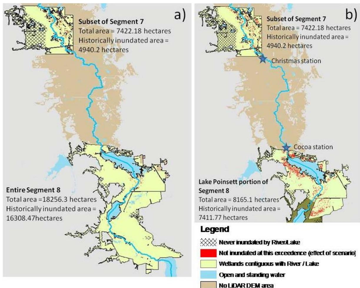
Figure 23. River floodplain. The area of contiguous wetlands historically inundated by the River, segments 7 and 8 are displayed in pale green. Panel a has the original Segment 8 area as reported in Chapters 10 and 13. Panel b displays a subset of Segment 8 which was created to facilitate comparison of results between the two Segments. The Segment 7 study area is 63% of the area of the Segment 8 study area shown in panel b.
