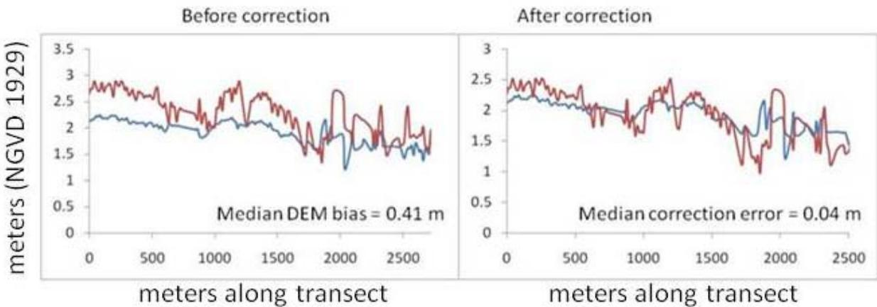
Figure 19. M-6 transect comparison of DEM elevation to MFL elevation before and after DEM correction. N = 151, emergent aquatic vegetation removed. Blue lines in both Figures represent the MFL surveyed elevation and the red lines are the LiDAR-derived DEM elevations.
