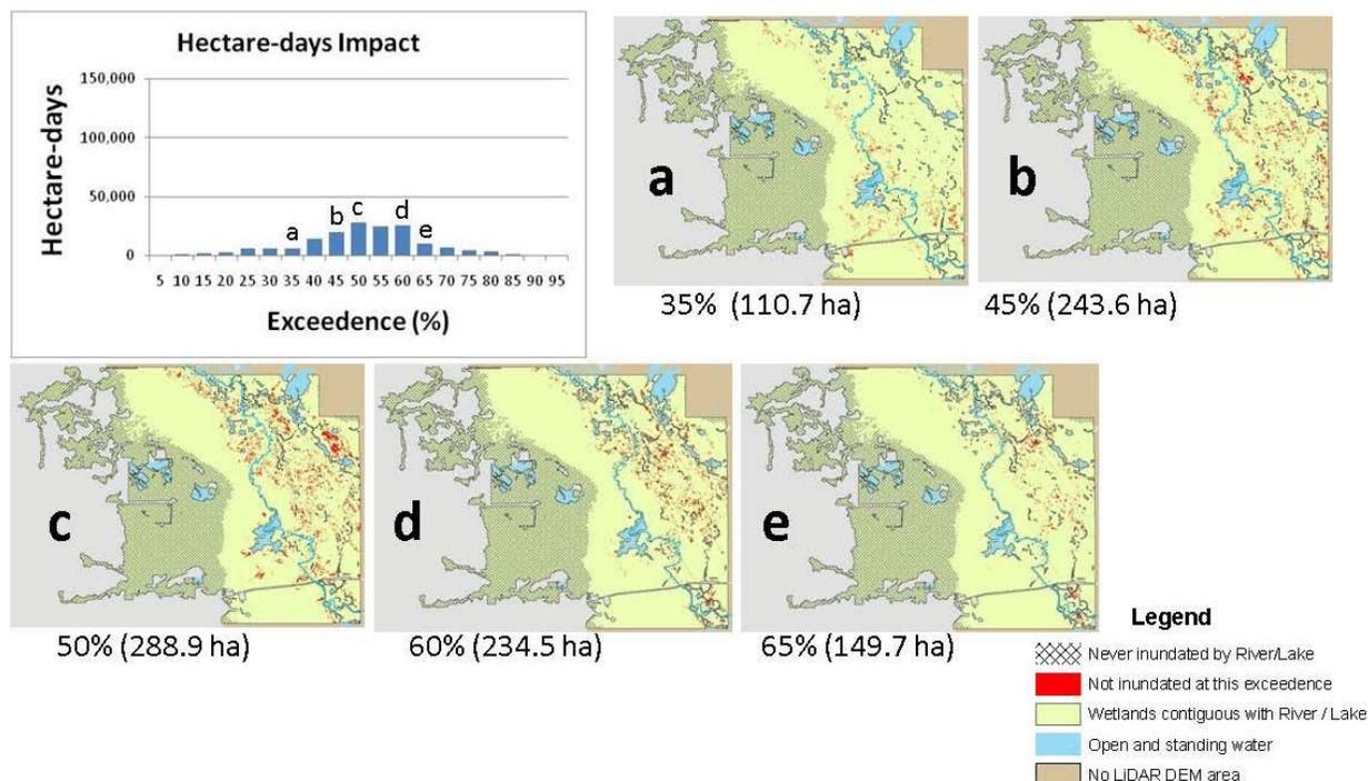
Figure 27. Areal extent and hectare-days effect of FULL1995NN scenario on Segment 7. Panels a through e are examples of dewatered areas experiencing fewer days of inundation at selected exceedences. Hectare-days effect at all exceedences shown in Figure in upper left corner.
