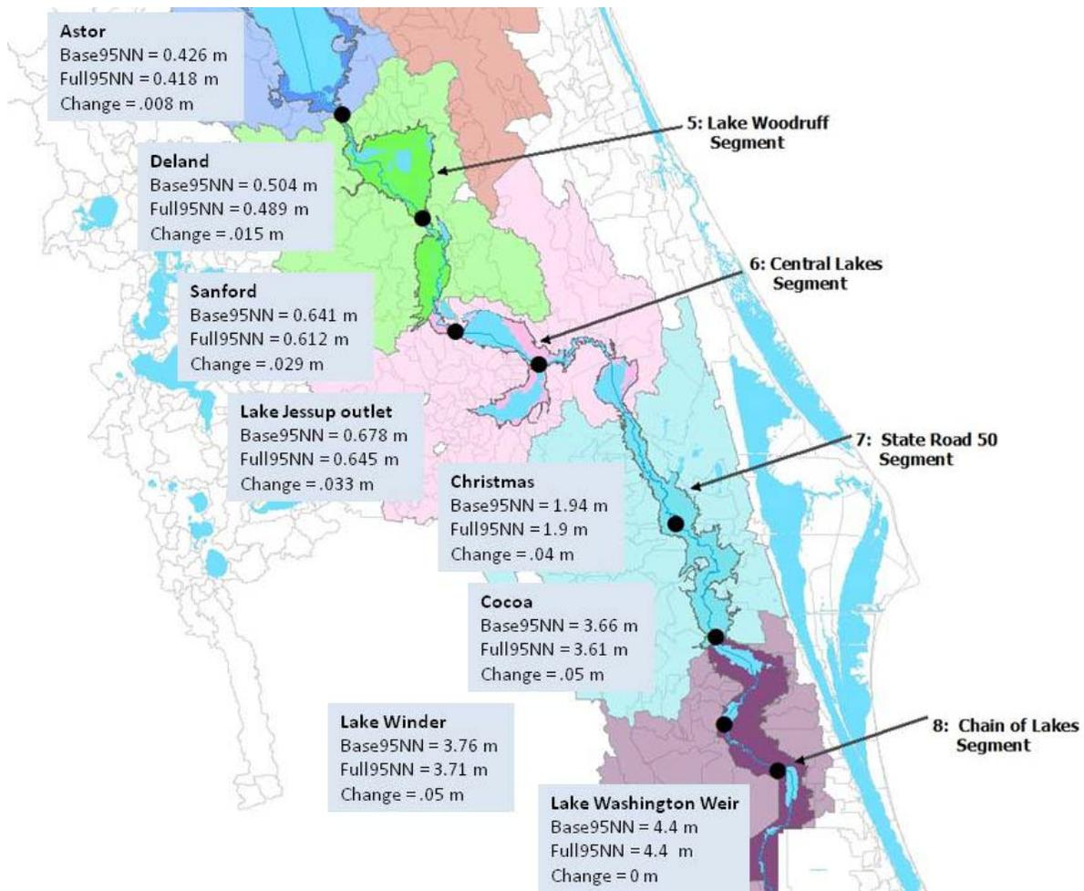
Figure 2. Modeled annual average water levels and change in water levels (m) at gauging stations under Base1995NN (historic conditions) and Full1995NN (withdrawal) scenarios. Scenarios described in Table 1. Note that the two stations in segment 8 (Cocoa and Lake Winder) have the greatest change in stage due to the proposed withdrawal scenario, both 0.05 m.
