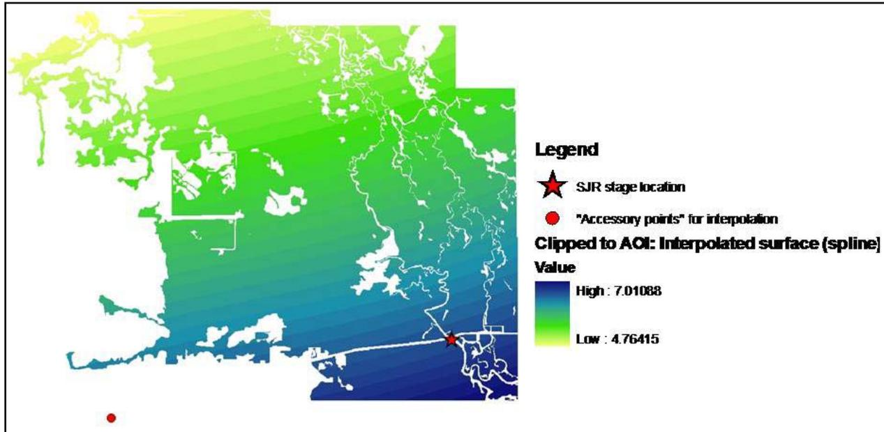
Figure 26. Interpolated surface for Segment 7 study area using the spline method. The banding pattern is an artifact of the classified symbolization (rather than stretched) in the GIS but more clearly shows that a surface described by a sloping flat pool was approximately achieved.
