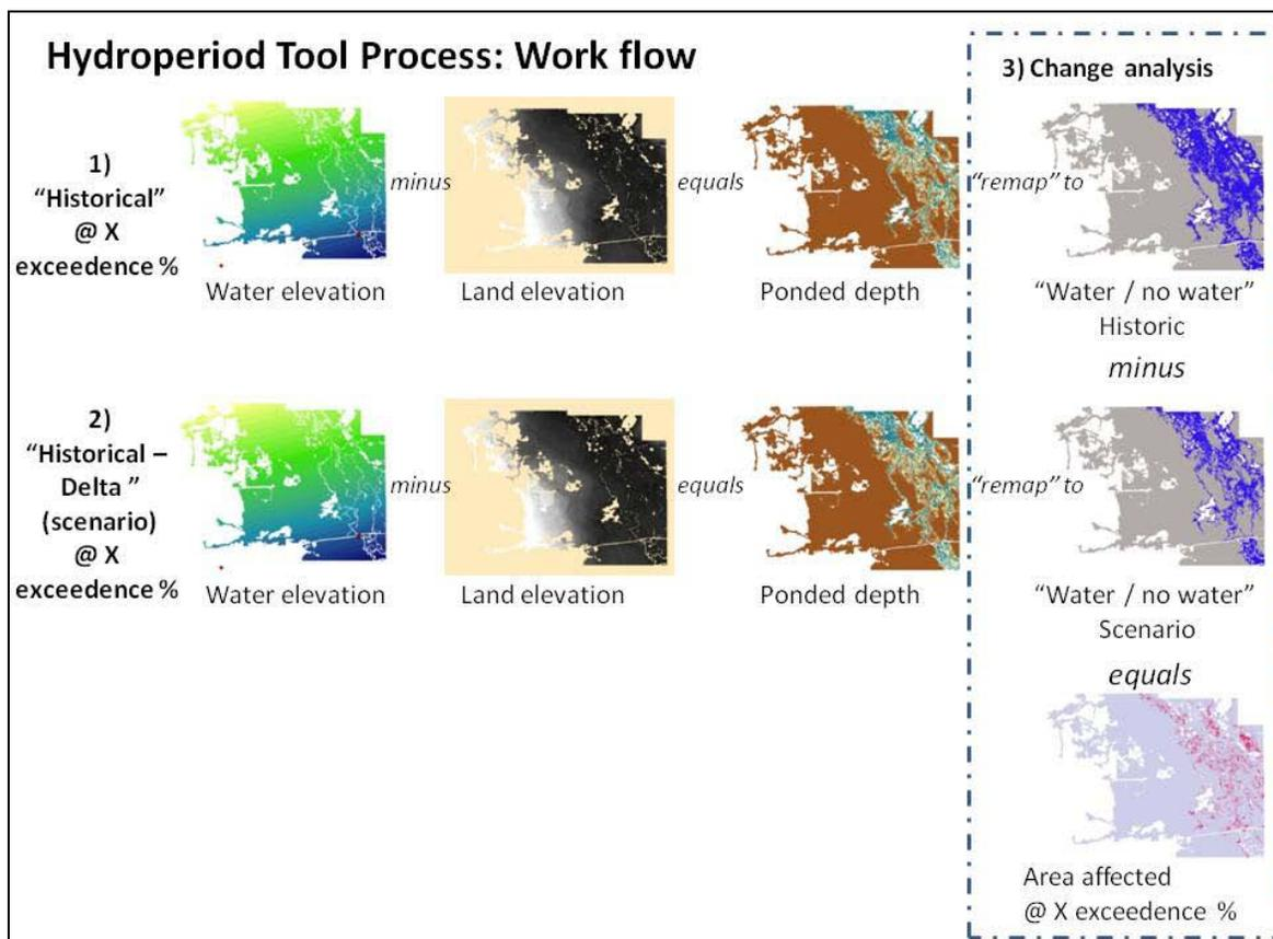
Figure 8. Summary of Hydroperiod Tool process. "Water elevation" in line 1 corresponds to the "water depth 50% of the time" in Figure 3. "Water elevation" in line 2 corresponds to the "water depth 50% of the time after withdrawal" in Figure 3. "Area affected @ X exceedence %" corresponds to "area (x,y) potentially impacted" in Figure 3.
