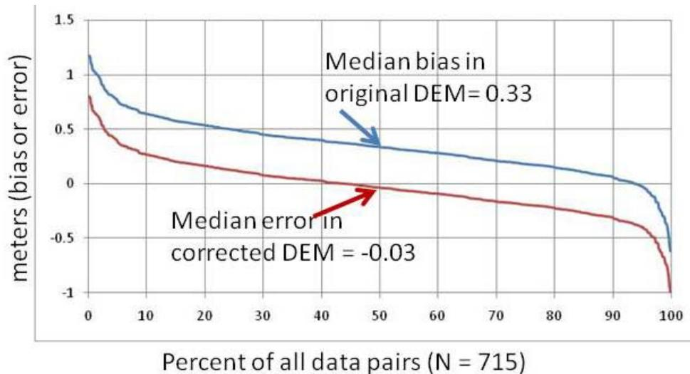
Figure 22. Summary of LiDAR bias and correction error.
