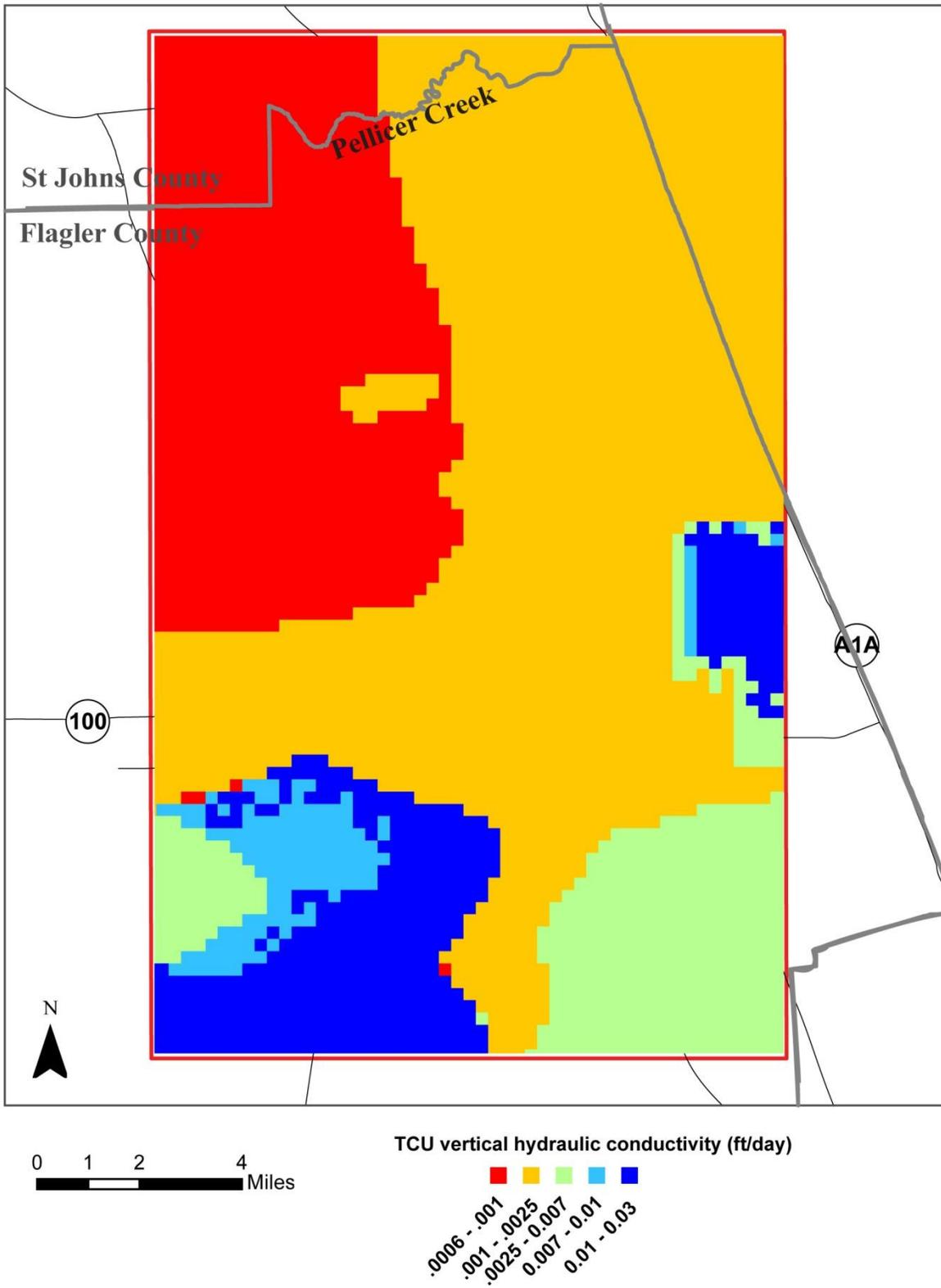
**Figure 72** Model derived vertical hydraulic conductivity of Top Confining Unit
