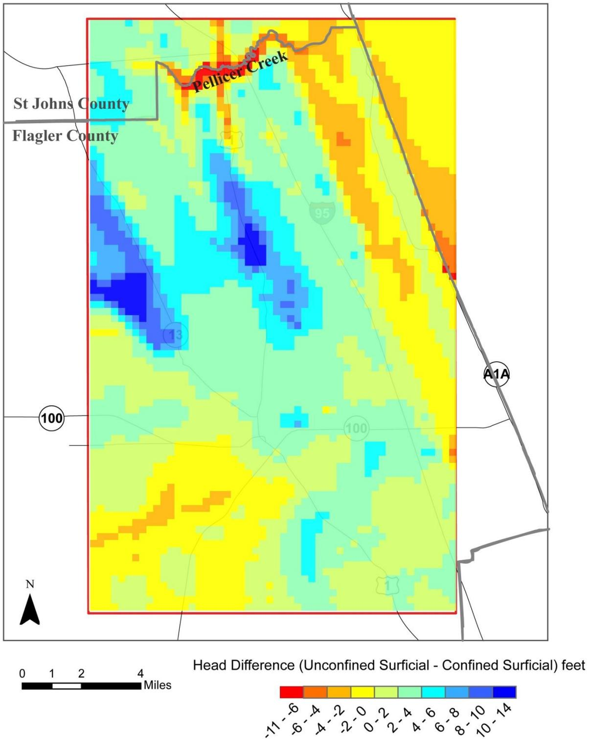
**Figure 55 Simulated average 1995 head difference between Unconfined Surficial and Confined Surficial aquifers**
