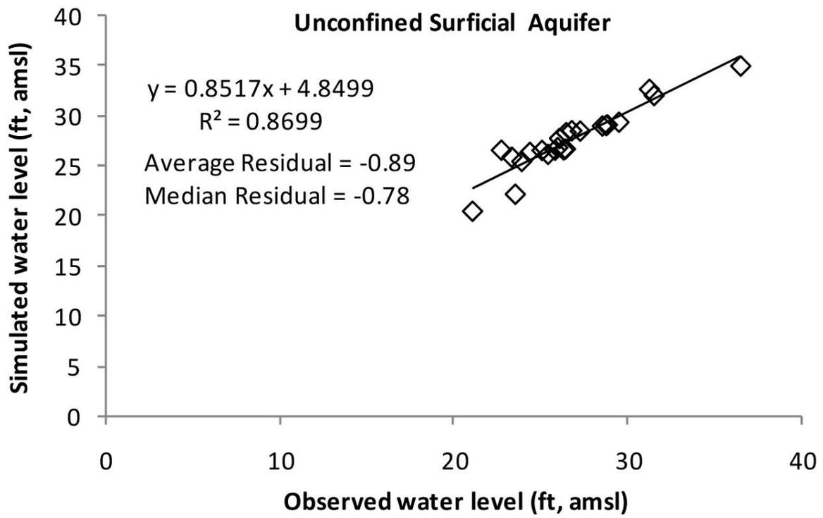
**Figure 52** Observed versus simulated water levels in the Unconfined Surficial aquifer for 1995
