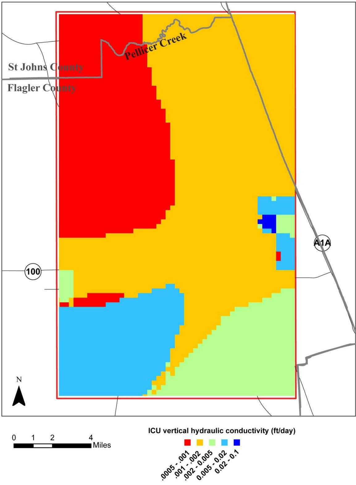
**Figure 73** Model calibrated vertical hydraulic conductivity of Intermediate Confining Unit
