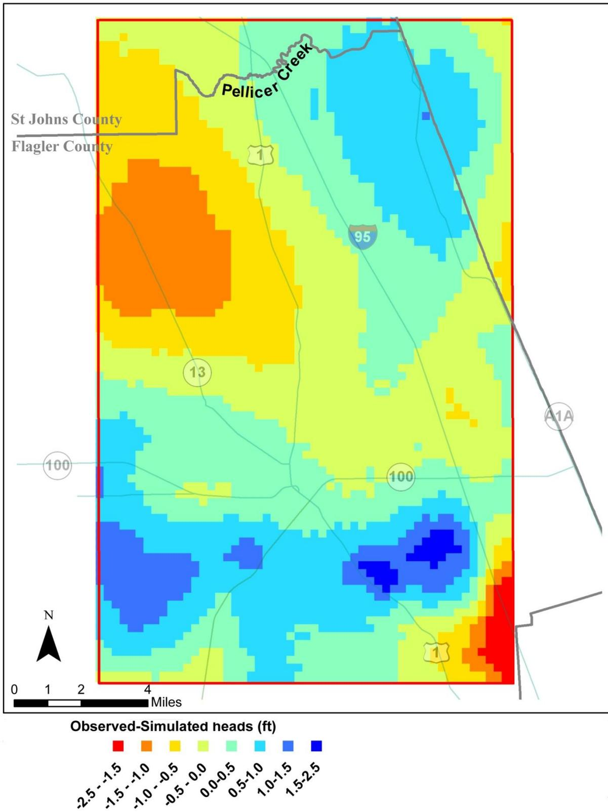
**Figure 61** Difference between simulated and interpreted average 1995 potentiometric surface in Upper Floridan aquifer
