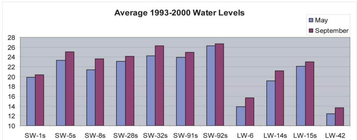
**Figure 40** Water levels in Unconfined Surficial aquifer monitoring wells
