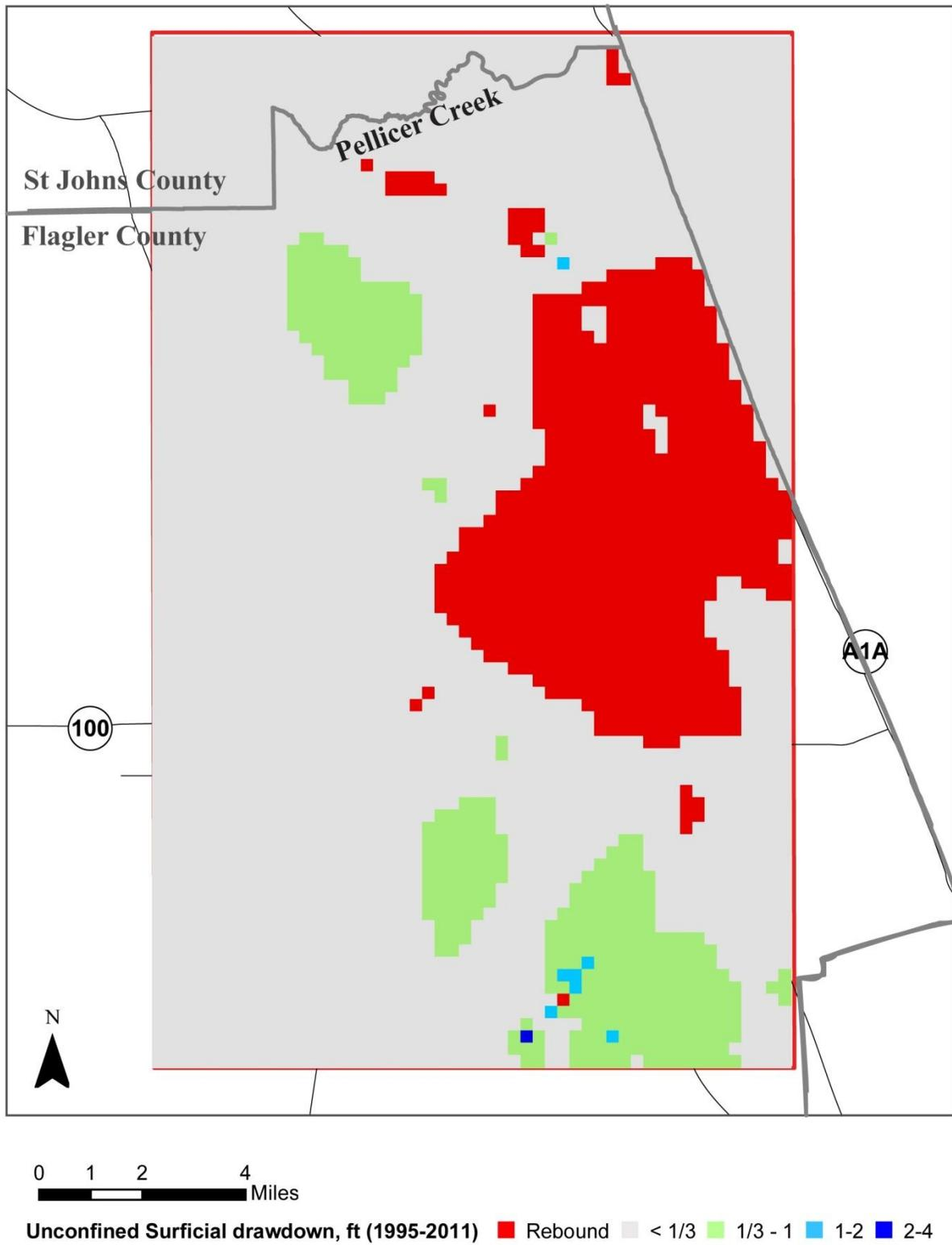
**Figure 86 Simulated drawdowns in Unconfined Surficial aquifer (1995-2011)**
