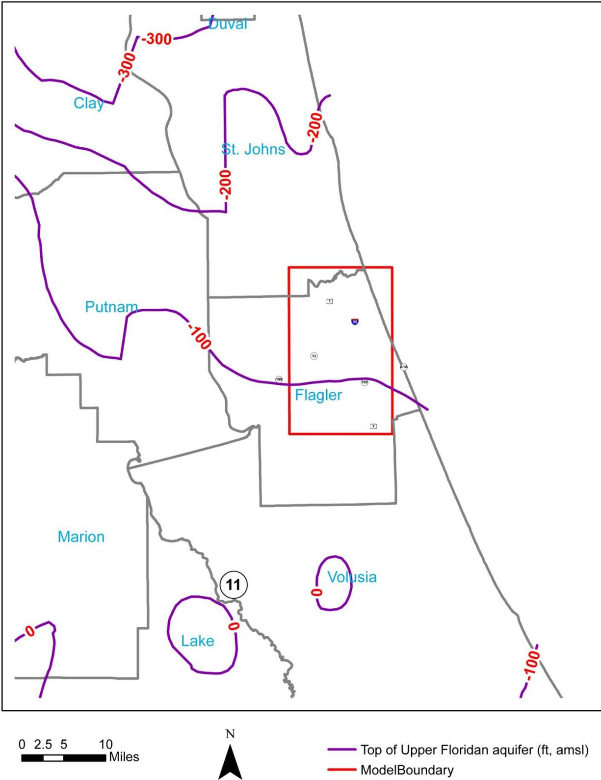
**Figure 19 Elevation to top of Upper Floridan aquifer**
