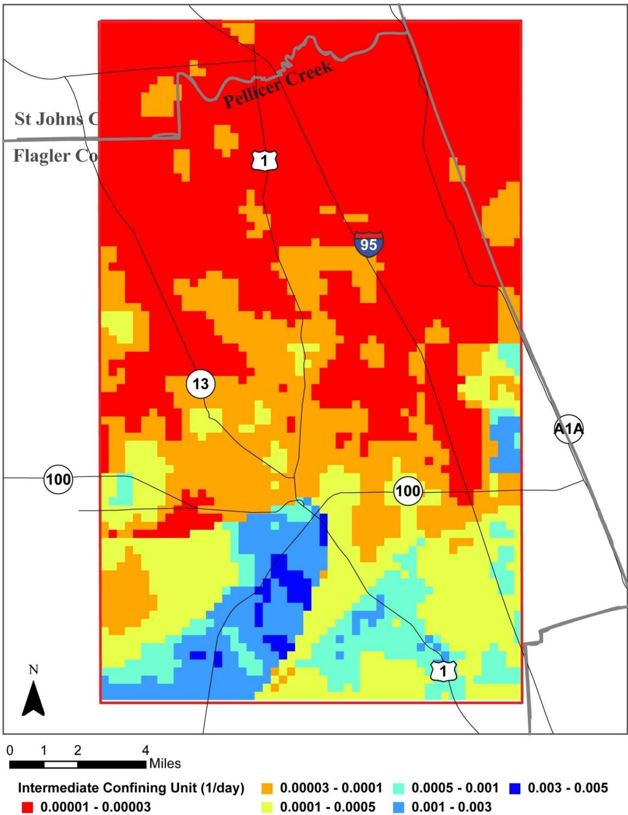
**Figure 75 Model derived leakage of Intermediate Confining Unit**
