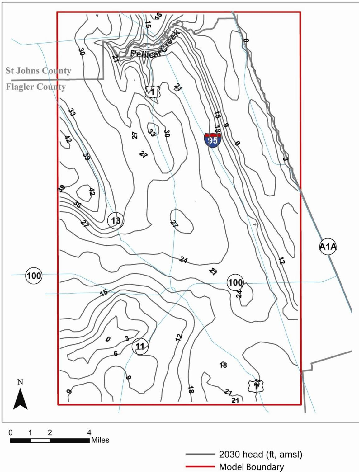
**Figure 96 Simulated average 2030 potentiometric surface in Unconfined Surficial aquifer**
