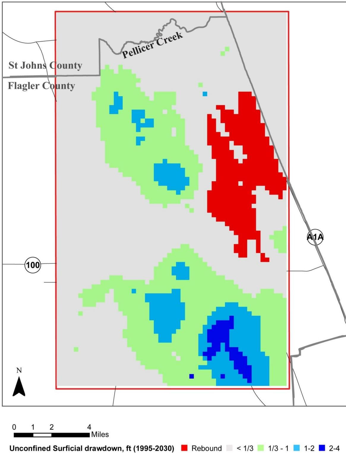
**Figure 101 Simulated drawdowns in Unconfined Surficial aquifer (1995-2030)**
