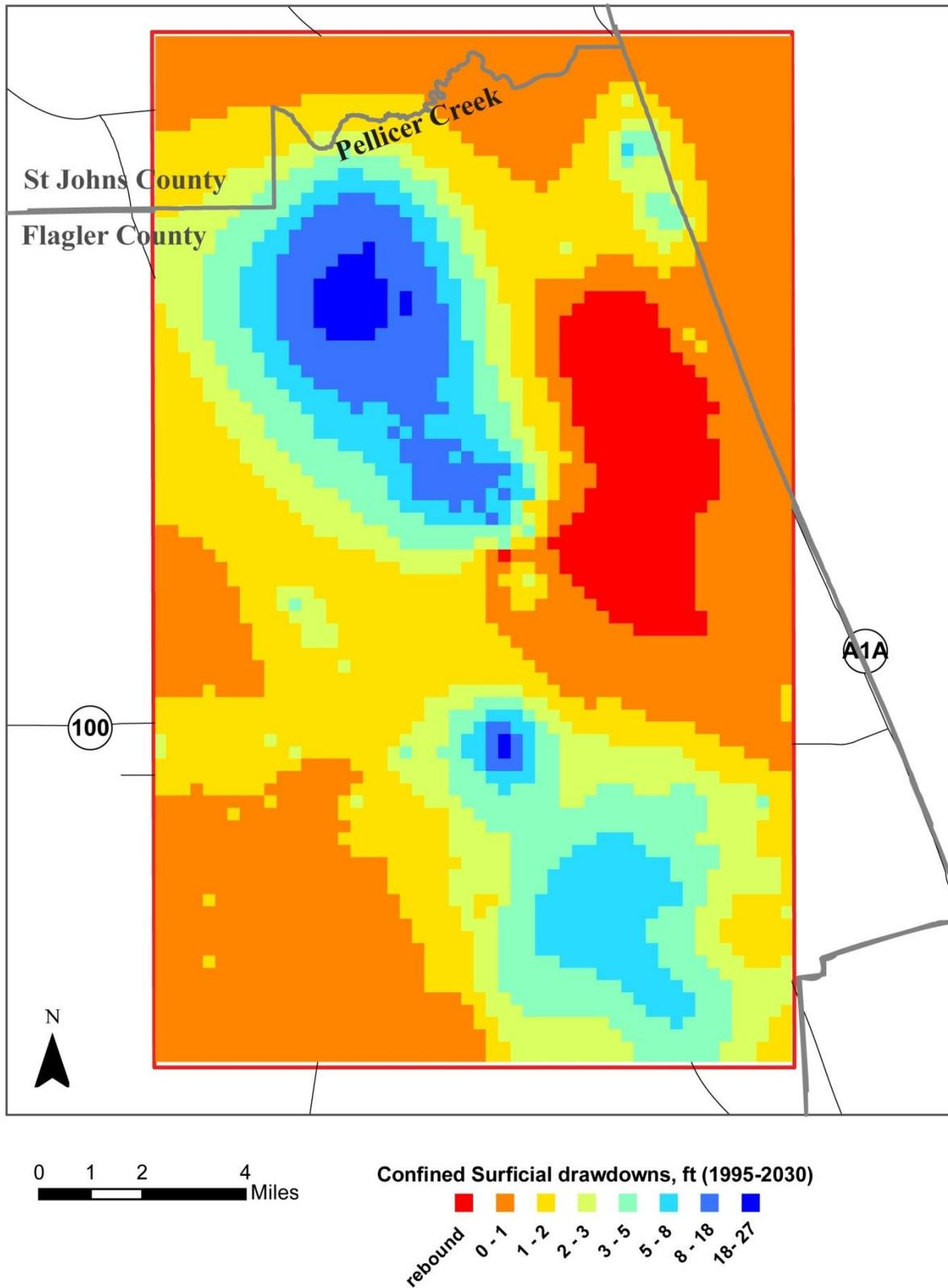
**Figure 100 Simulated drawdowns in Confined Surficial aquifer (1995-2030)**
