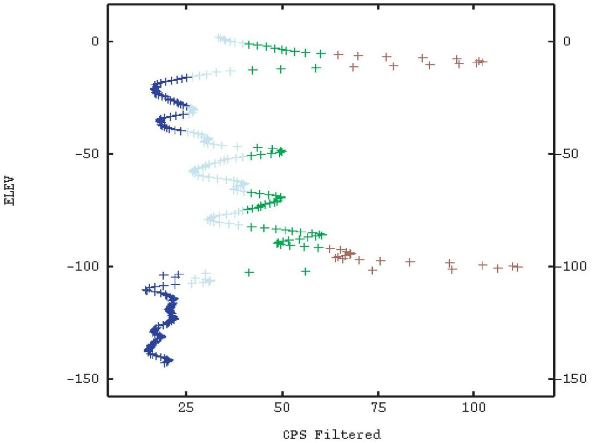
**Figure 21** Facies delineation based on natural gamma log response
