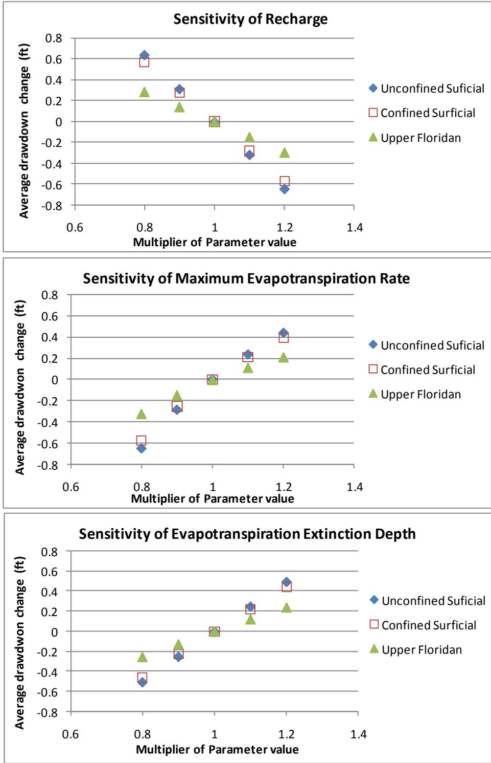
**Figure 94 Recharge and evapotranspiration sensitivity drawdown change simulation results for 2011**
