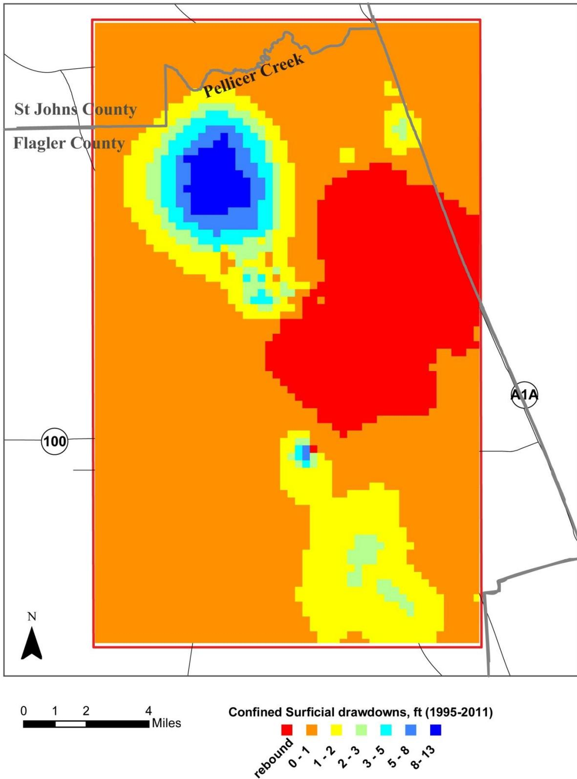
**Figure 85 Simulated drawdowns in Confined Surficial aquifer (1995-2011)**
