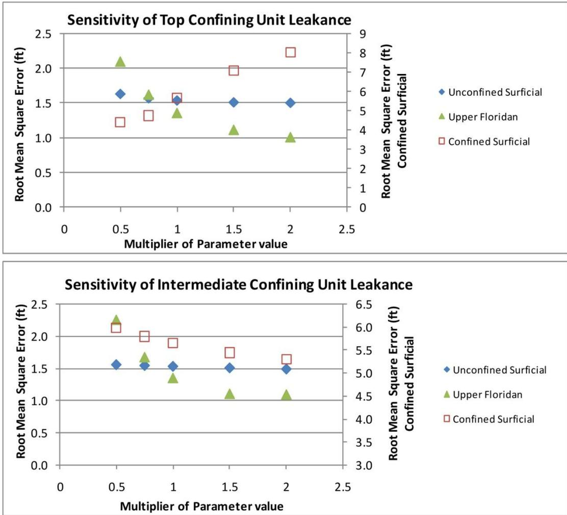
**Figure 89** Confining unit leakance sensitivity mean square error results for 2011
