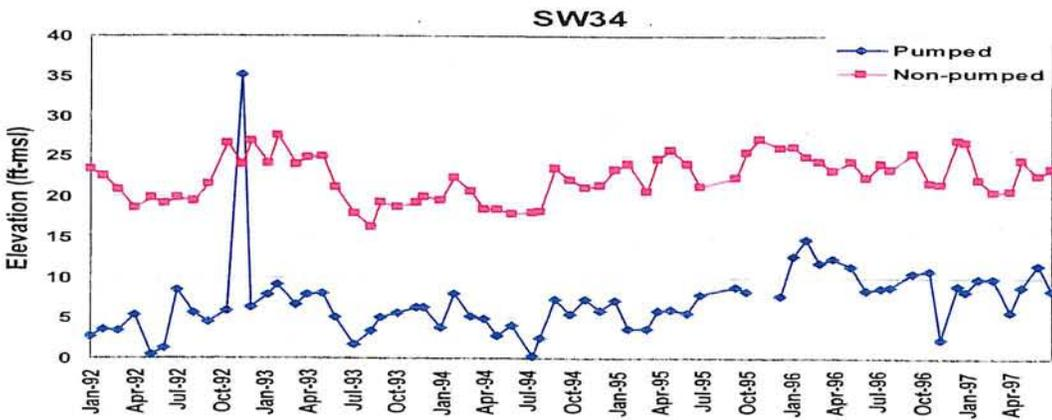
Water level hydrographs in Confined Surficial aquifer at SW-32, SW-33, and SW-34
