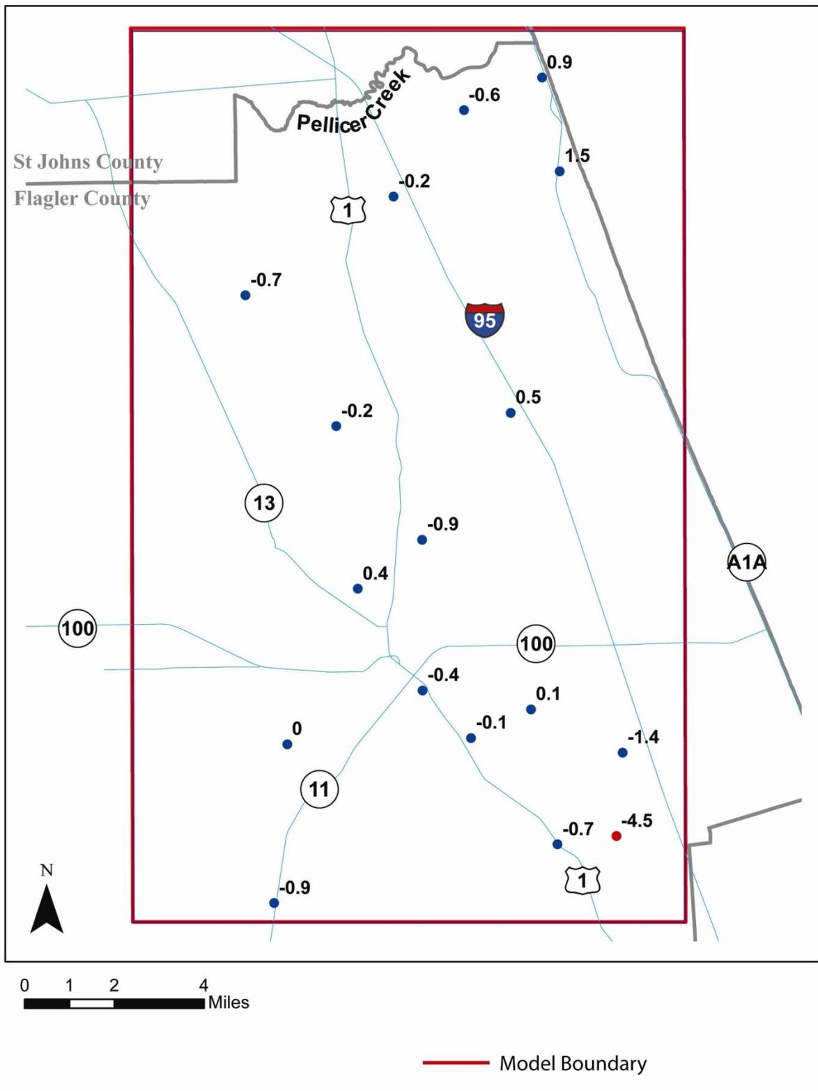
**Figure 59** Average 1995 head residual (observed-simulated) at Upper Floridan aquifer monitoring wells
