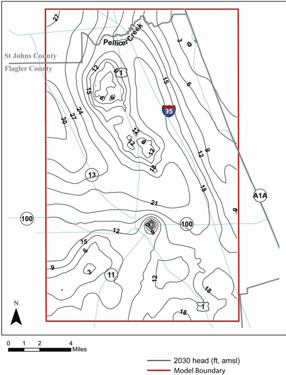
**Figure 97 Simulated average 2030 potentiometric surface in Confined Surficial aquifer**
