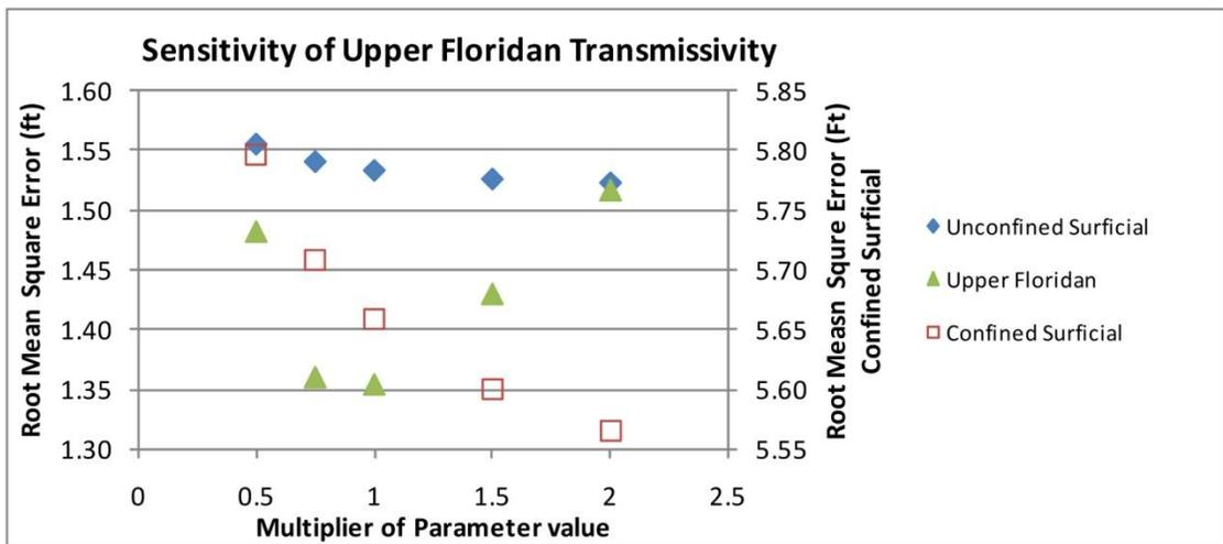
Figure 88 Aquifer transmissivity sensitivity root mean square error results for 2011
