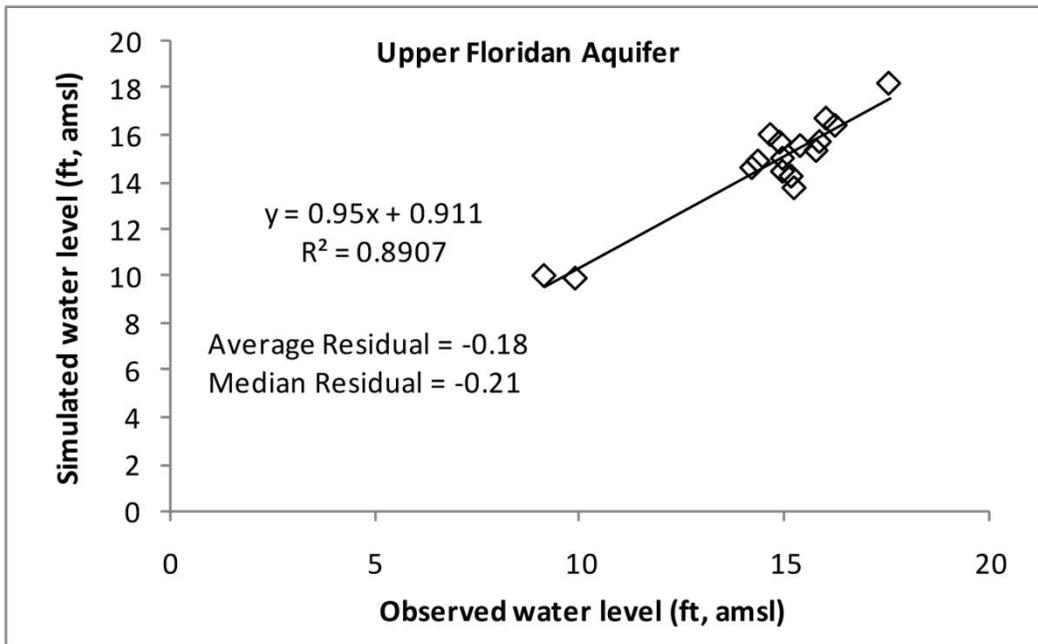
**Figure 60** Observed versus simulated water levels in the Upper Floridan aquifer for 1995
