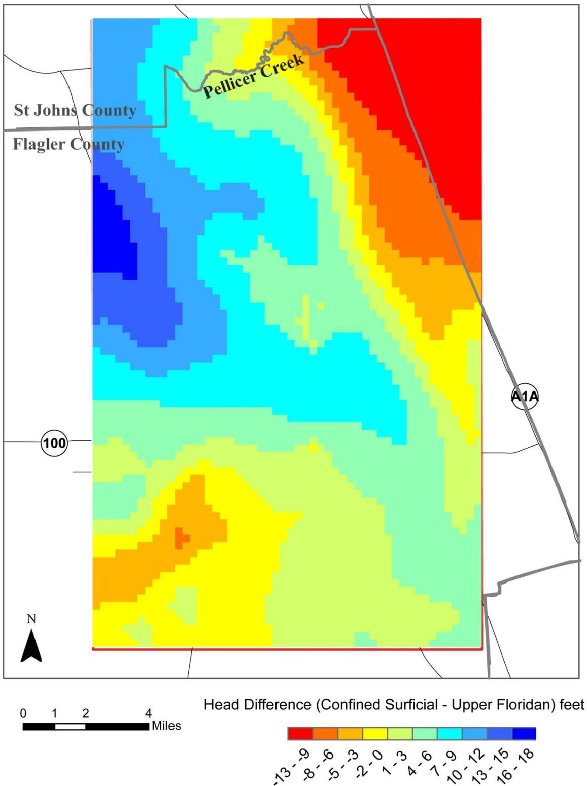
**Figure 62** Simulated average 1995 head difference between Confined Surficial and Upper Floridan aquifers
