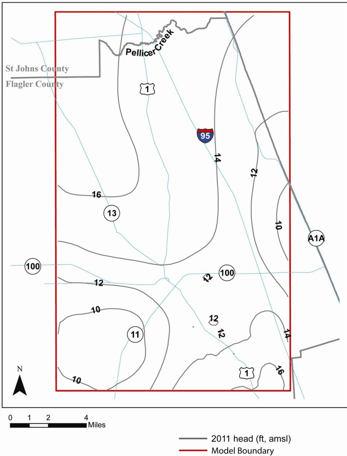
**Figure 83 Simulated 2011 potentiometric surface in Upper Floridan aquifer**
