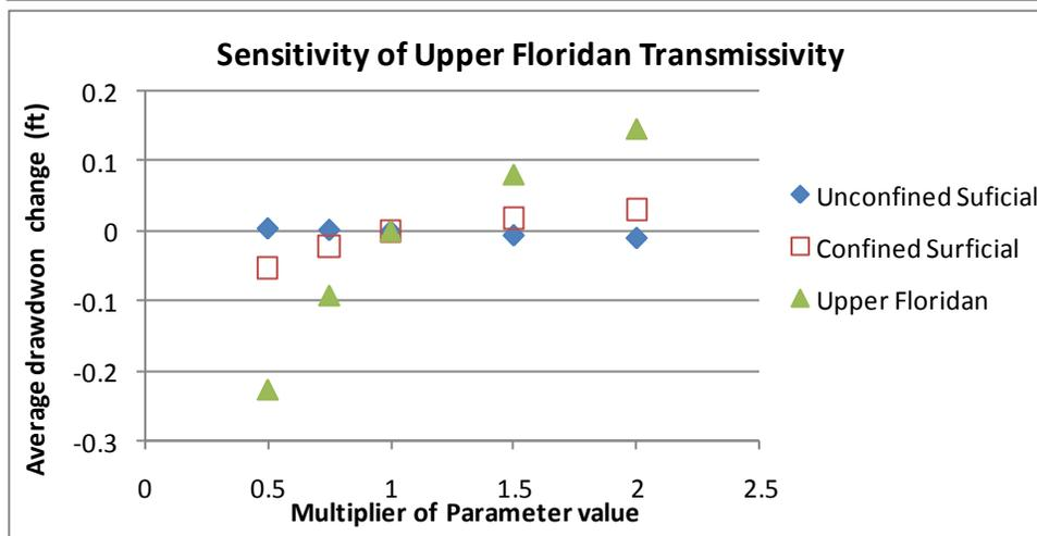
**Figure 92** Aquifer transmissivity sensitivity drawdown change results for 2011
