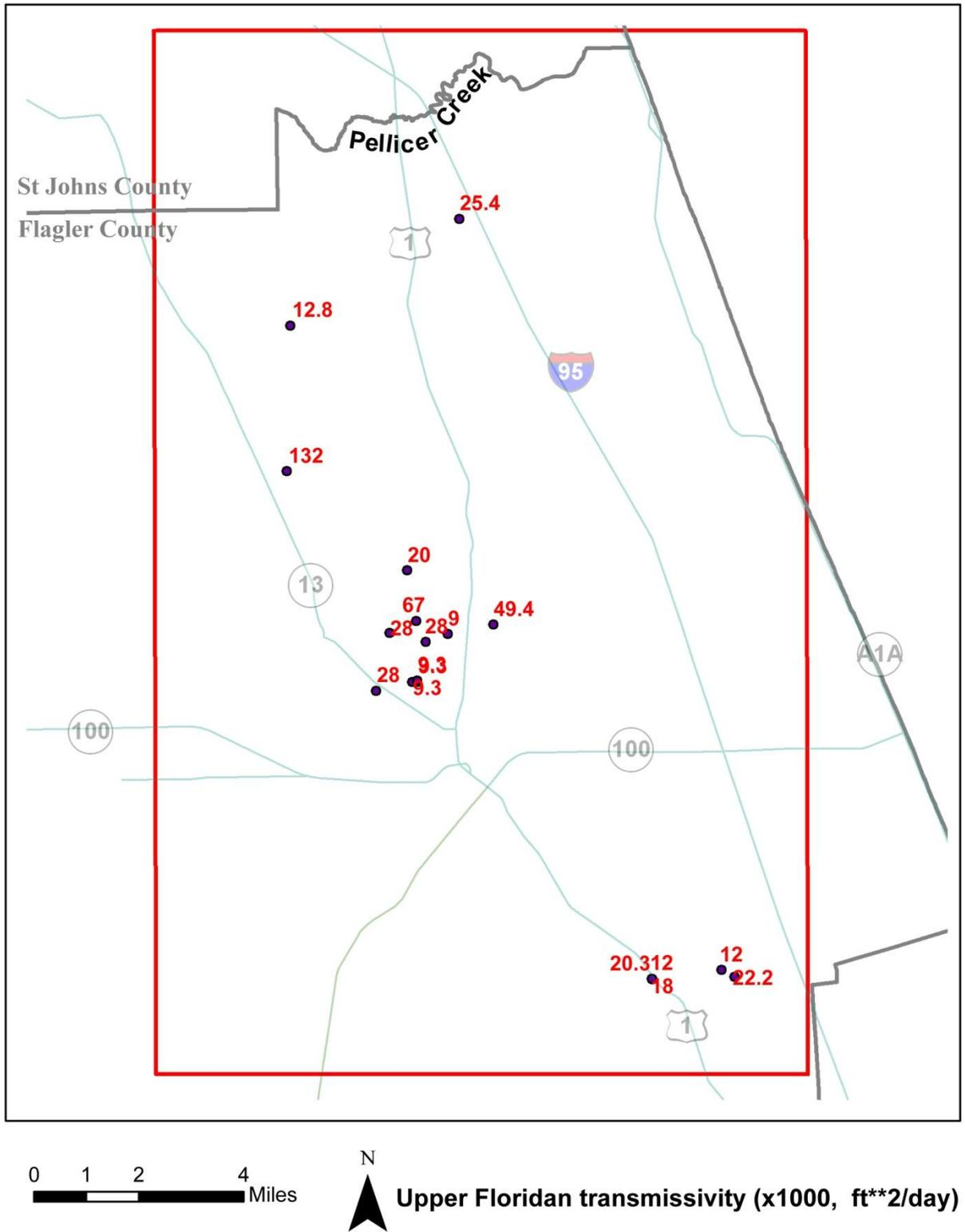
**Figure 32 Pump-test based transmissivity of Upper Floridan aquifer (x1000)**
