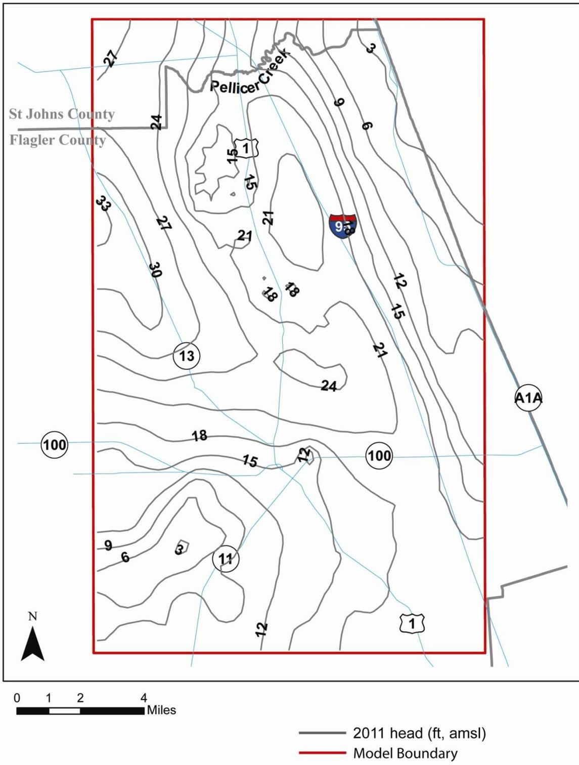
**Figure 82 Simulated 2011 potentiometric surface in Confined Surficial aquifer**
