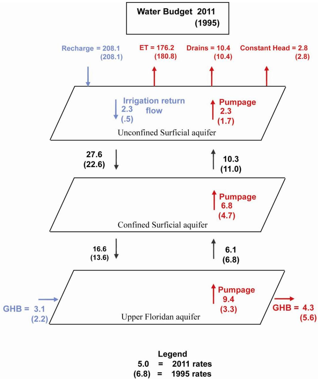
**Figure 87 Model simulated water budget for 2011 (MGD)**
