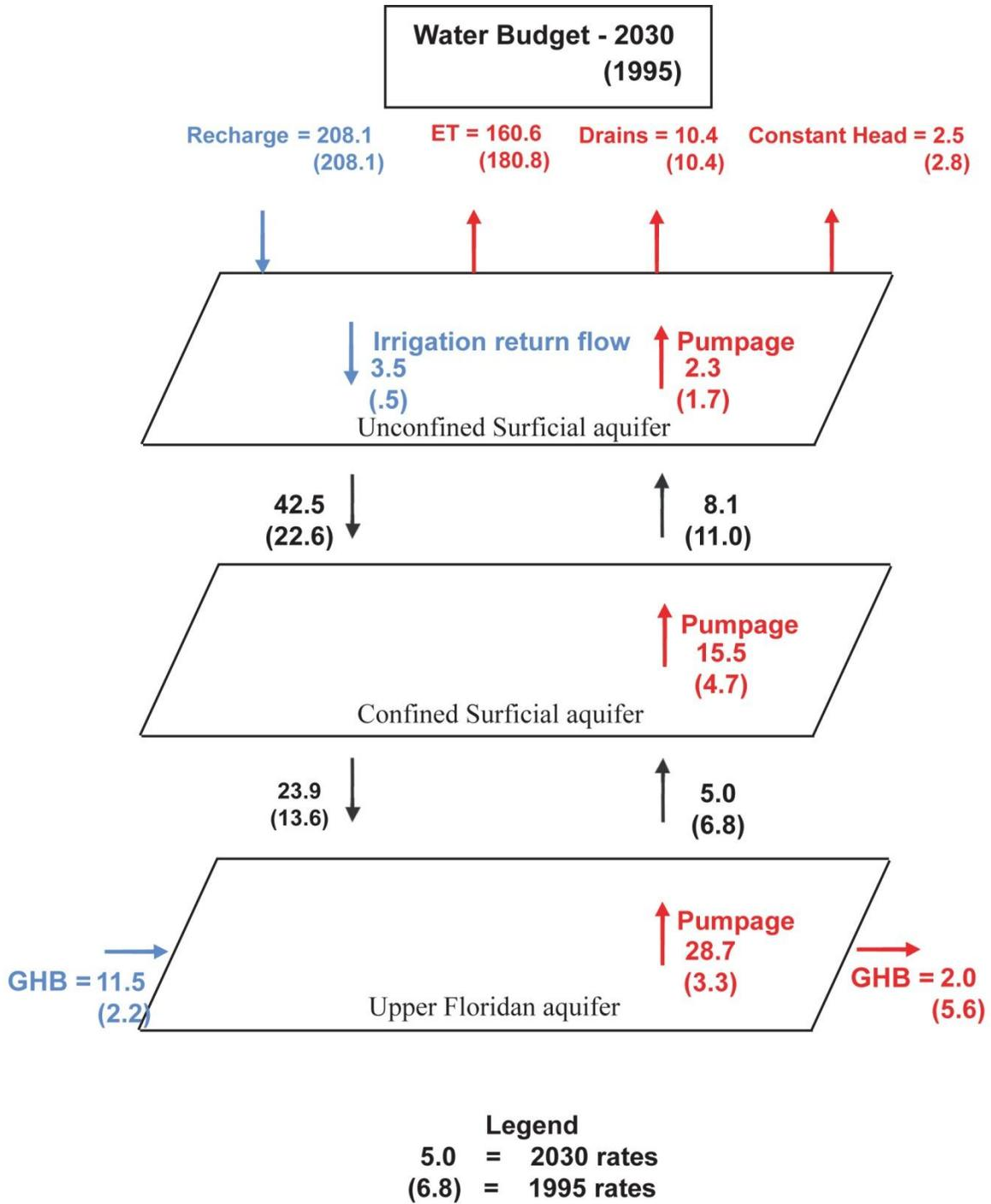
**Figure 102 Model simulated water budget for 2030 (MGD)**
