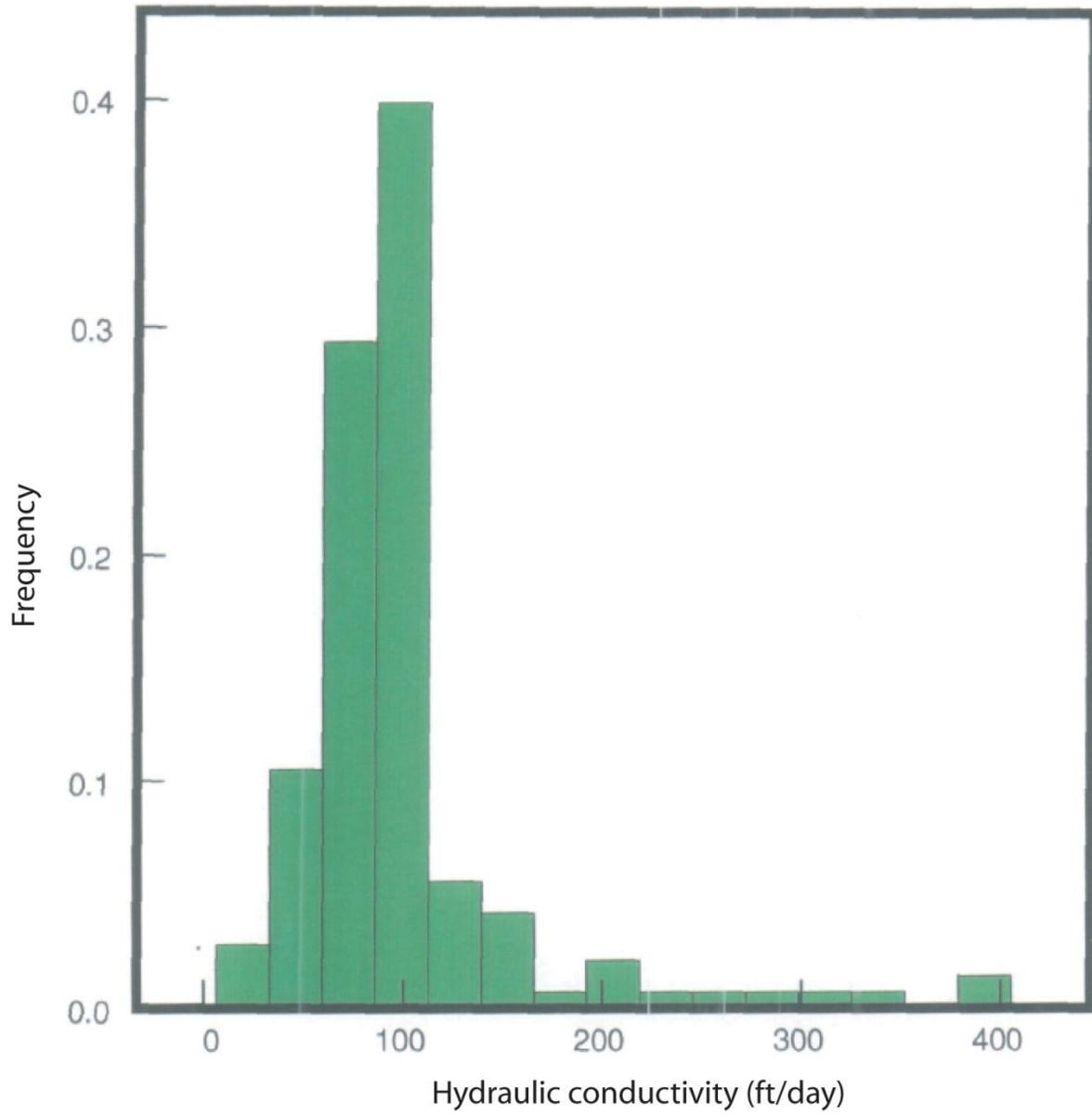
**Figure 29** Histogram of hydraulic conductivity of the Confined Surficial aquifer
