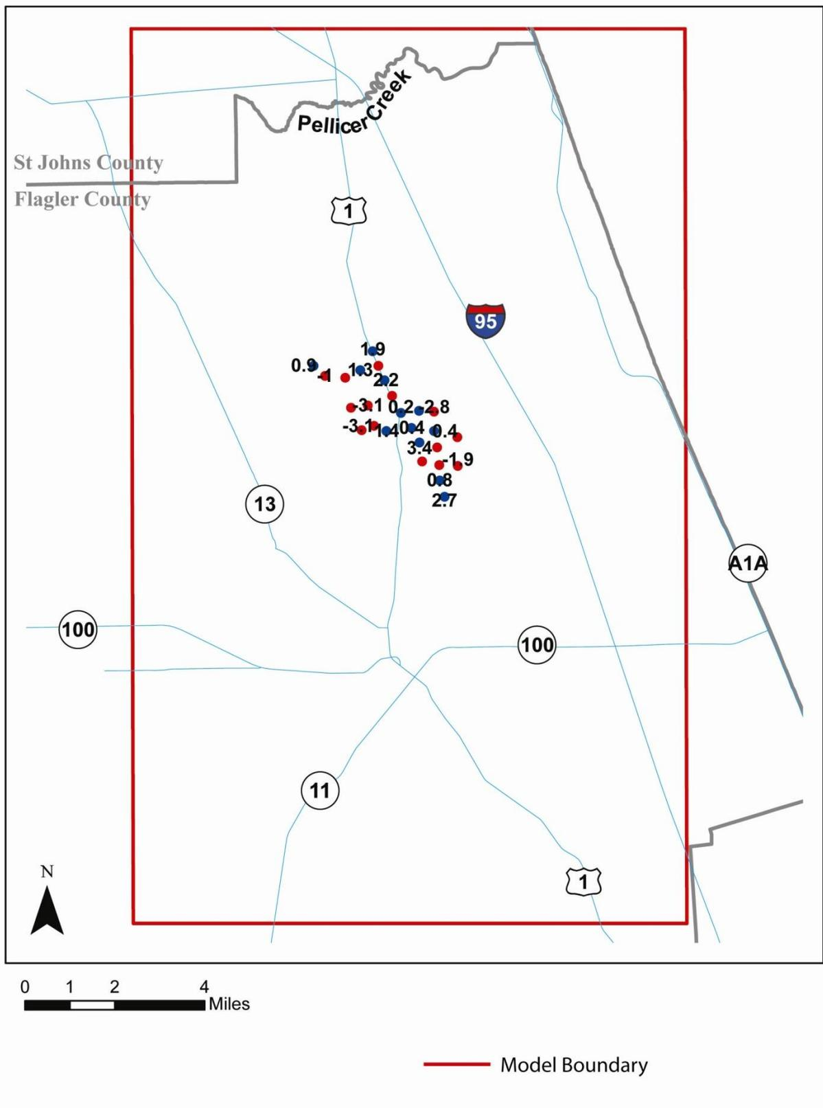
**Figure 56** Average 1995 head residuals (observed - simulated) at Confined Surficial aquifer wells
