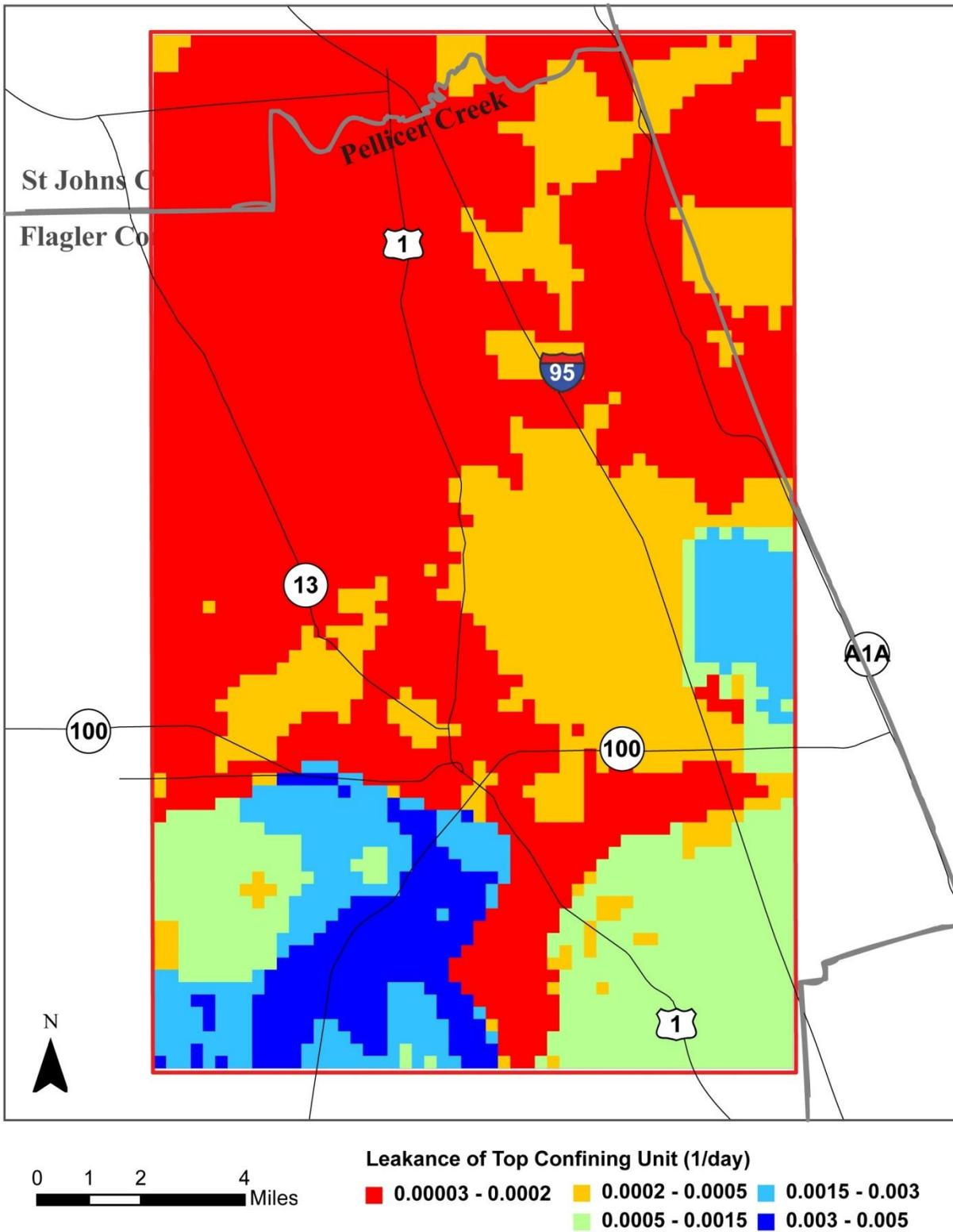
**Figure 74** Model derived leakage of Top Confining Unit
