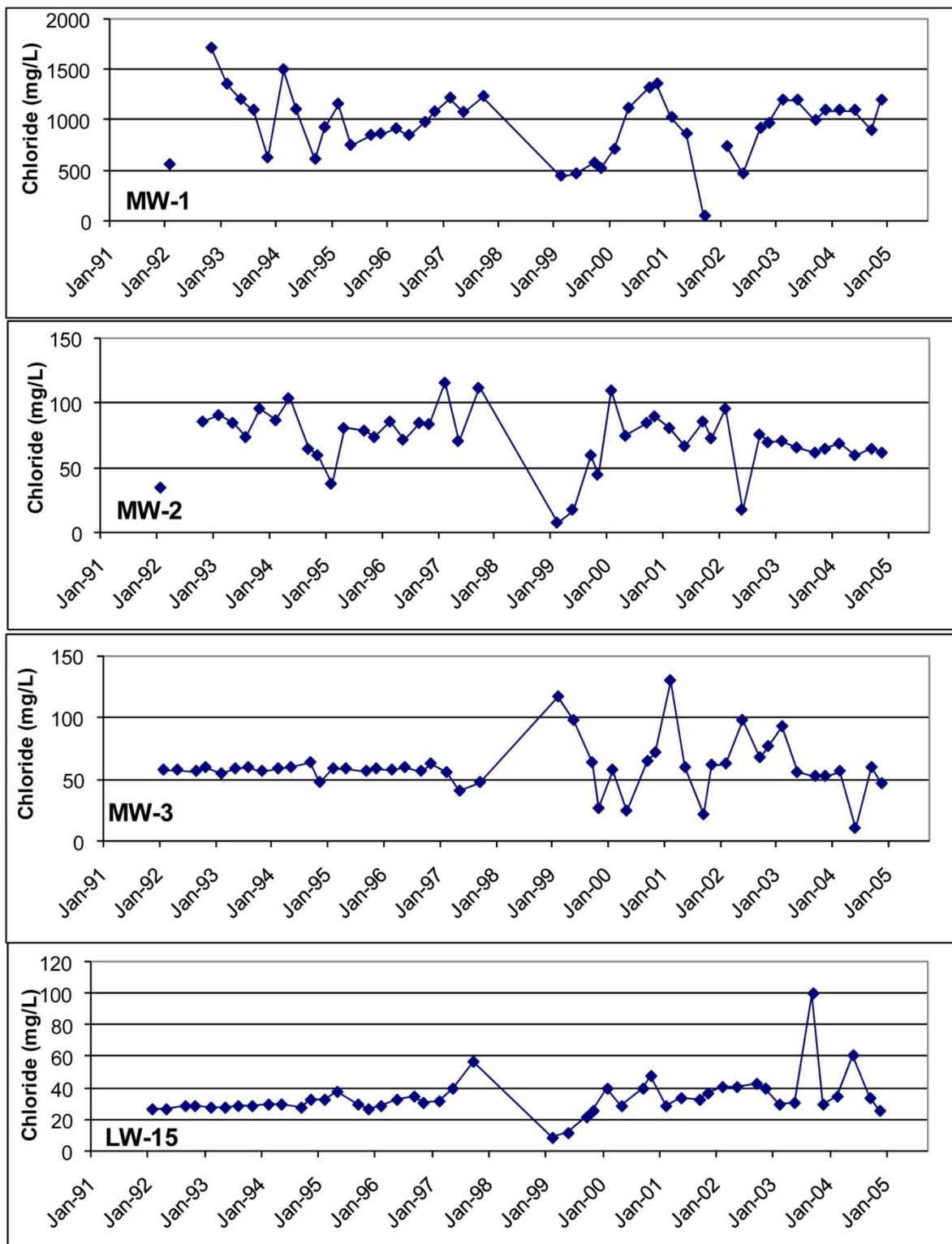
**Figure 36 Chloride concentration at Salt Water Intrusion Monitoring (SWIM) wells MW-1, MW-2, MW-3, LW-15**
