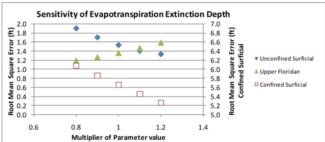
**Figure 90** Recharge and evapotranspiration sensitivity simulation mean square error results for 2011
