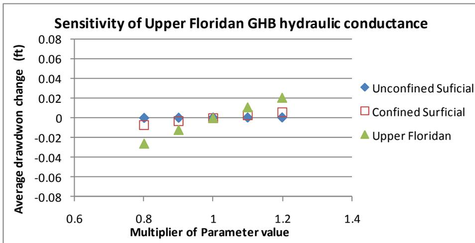
**Figure 95** General-Head Boundary sensitivity simulation drawdown change results for 2011
