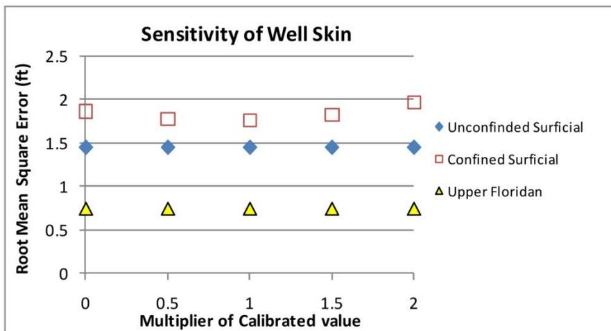
**Figure 79** General-Head Boundary and well skin sensitivity simulation results for 1995 calibration period
