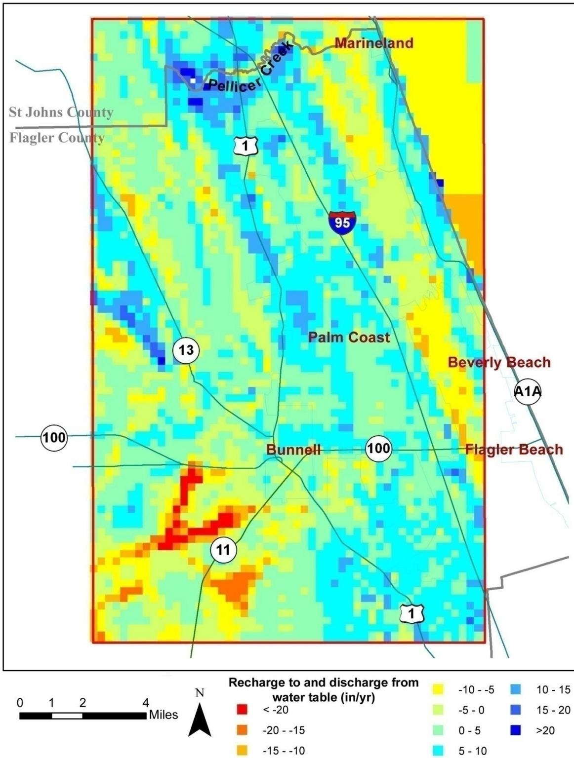
**Figure 66** Average 1995 simulated net recharge to Unconfined Surficial aquifer
