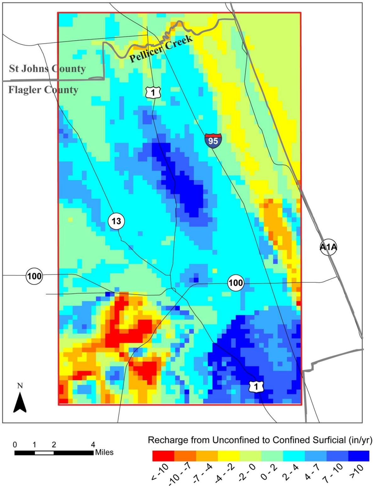
**Figure 67** Average 1995 simulated recharge from Unconfined to Confined Surficial aquifer
