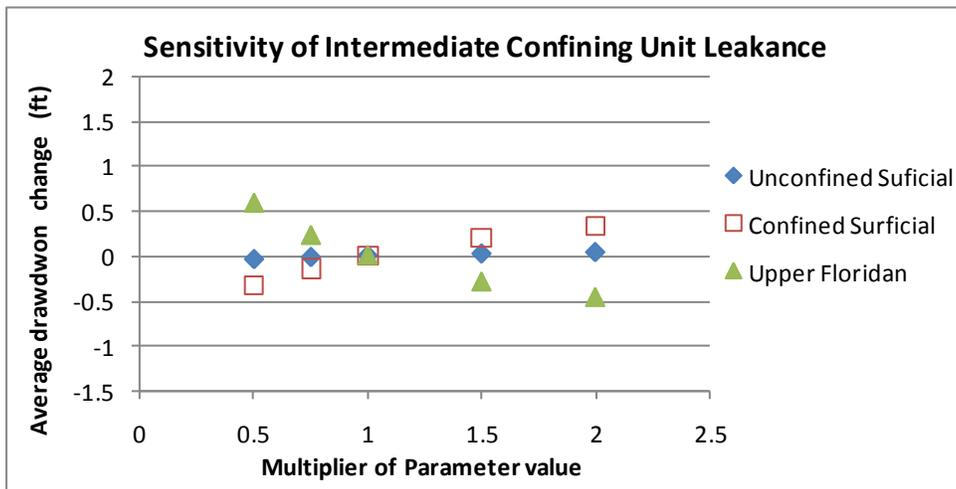
**Figure 93** Confining unit leakance sensitivity drawdown change results for 2011
