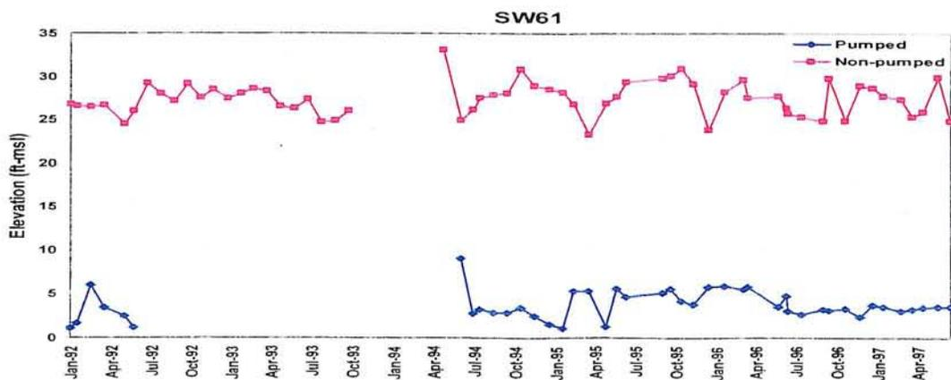
**Water level hydrographs in Confined Surficial aquifer at SW-59, SW-60, and SW-61**
