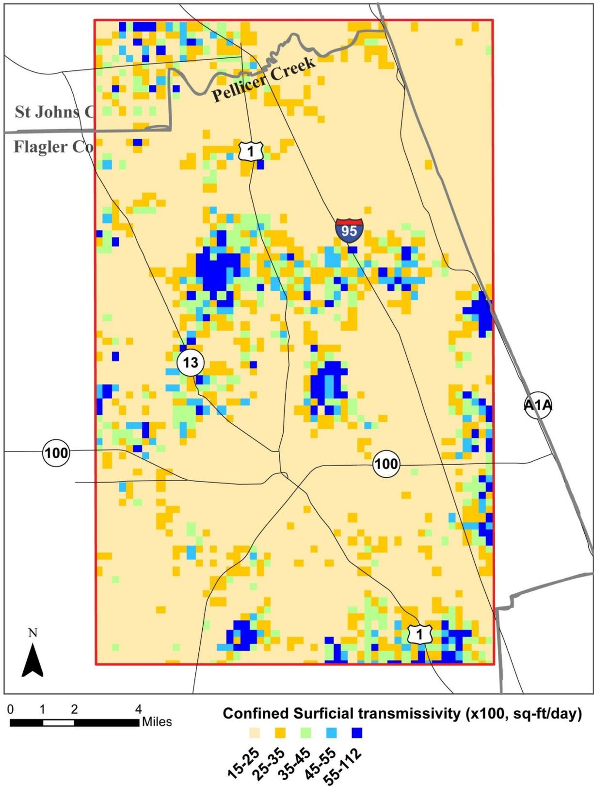
**Figure 70** Model derived Confined Surficial aquifer transmissivity
