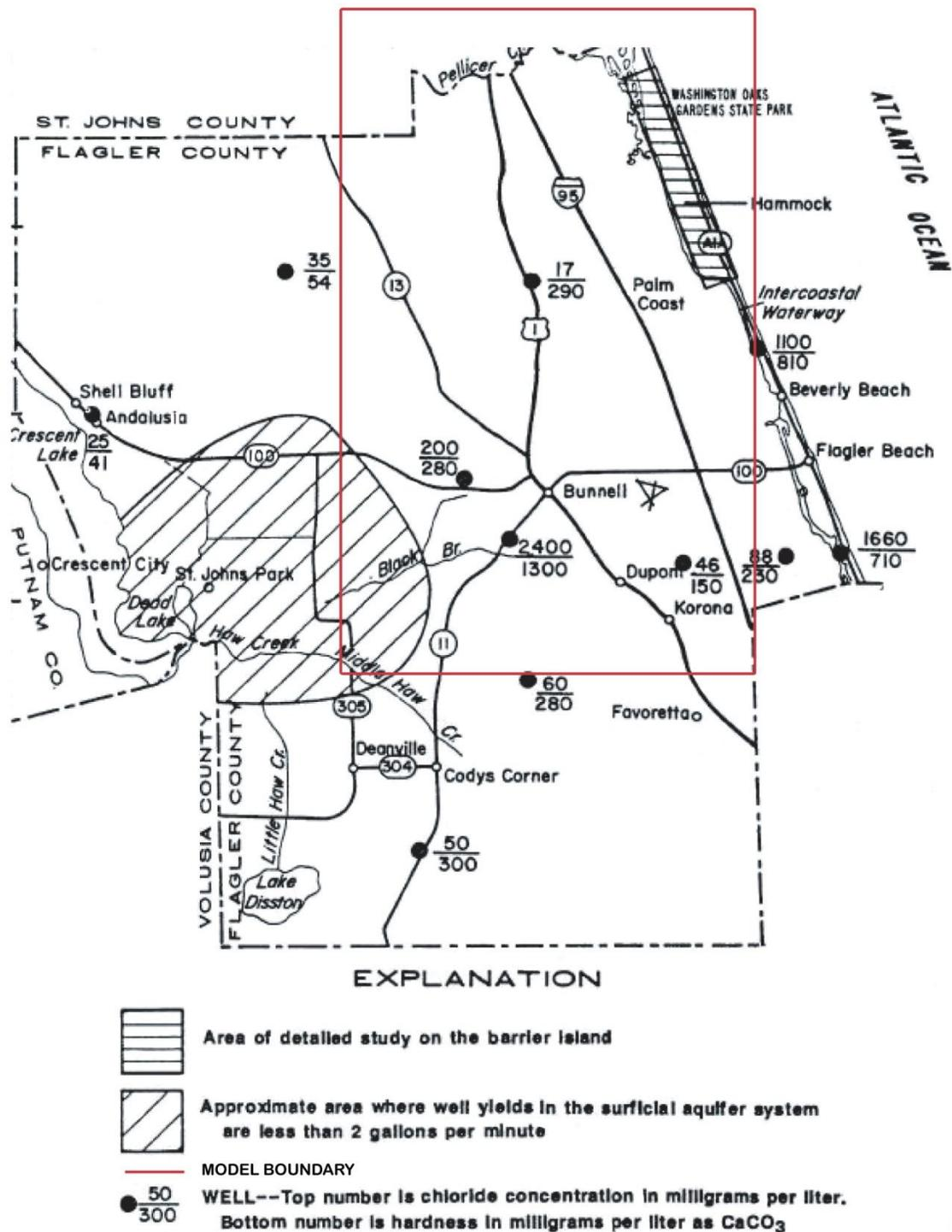
Figure 35 Chloride concentration and hardness in the Unconfined Surficial aquifer
