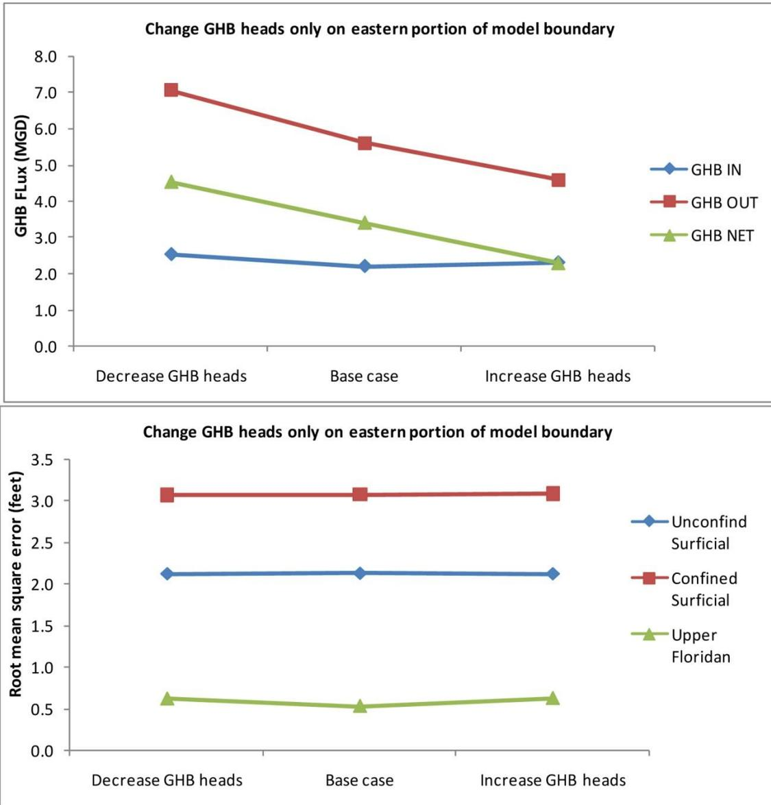
**Figure 80** General-Head Boundary sensitivity simulation results for gradient change for 1995 calibration period
