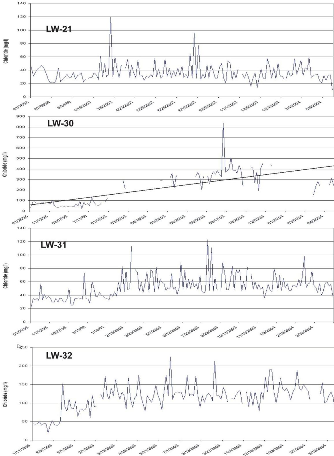
**Figure 38 Chloride concentration in Upper Floridan production wells**
