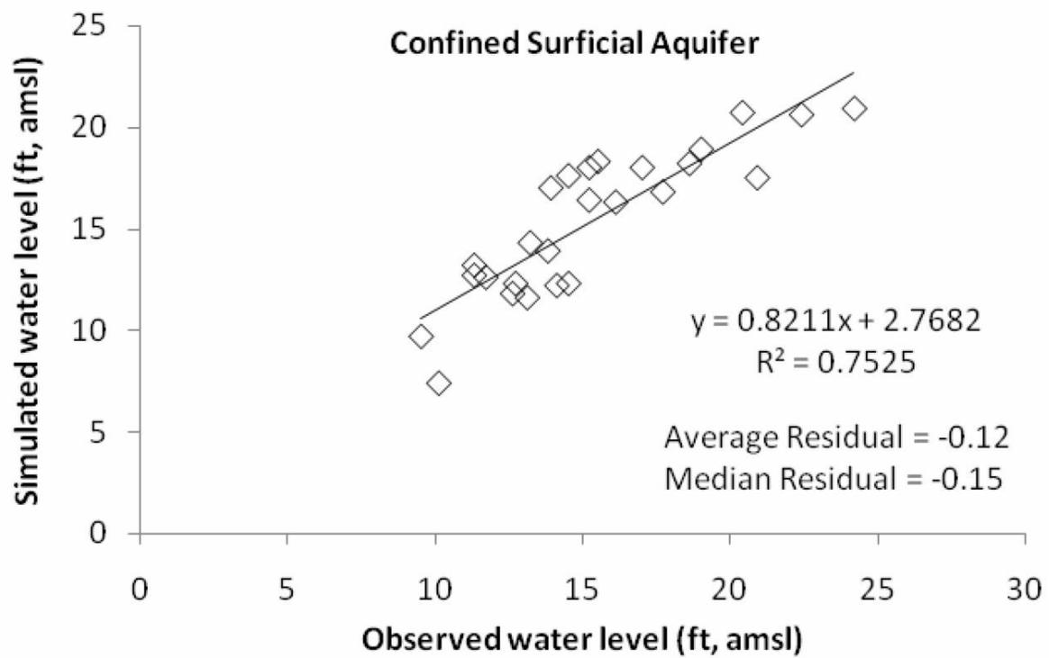
**Figure 57** Observed versus simulated water levels in the Confined Surficial aquifer for 1995
