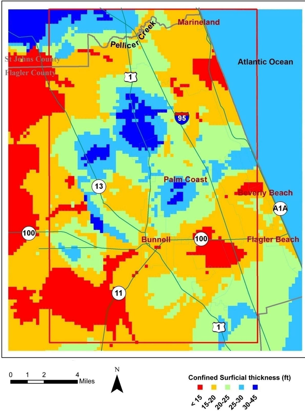
**Figure 17** Thickness of Confined Surficial aquifer
