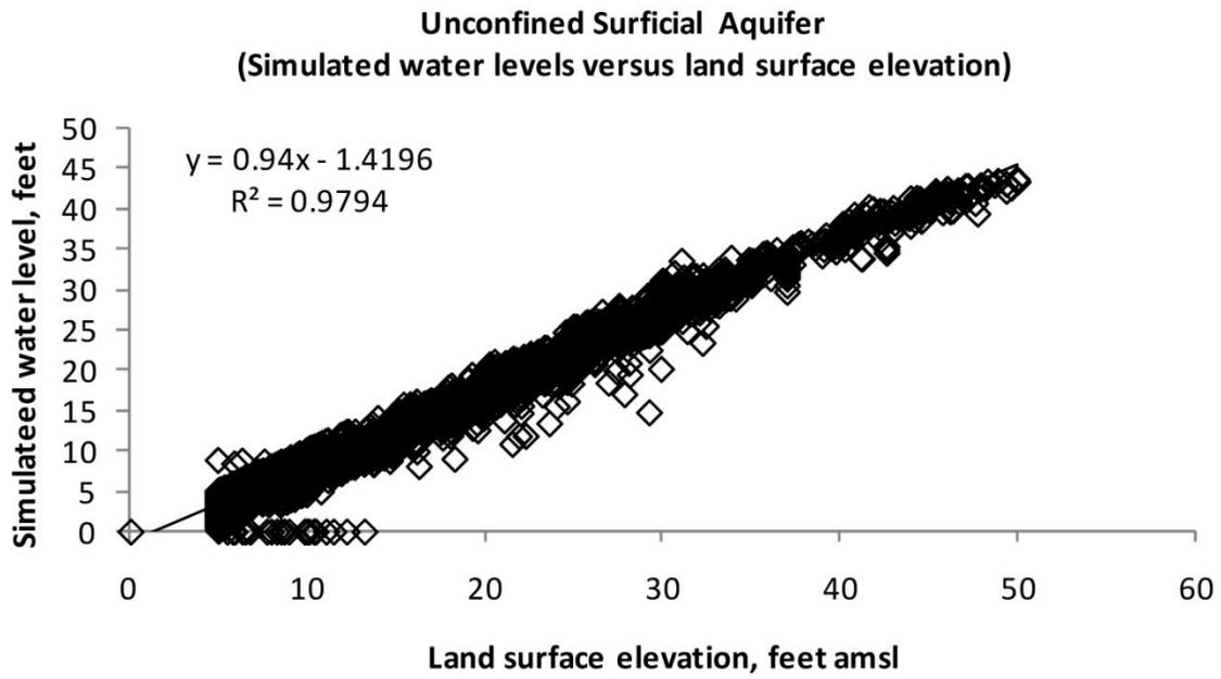
**Figure 53 Simulated 1995 water levels versus land surface elevation in Unconfined Surficial aquifer**
