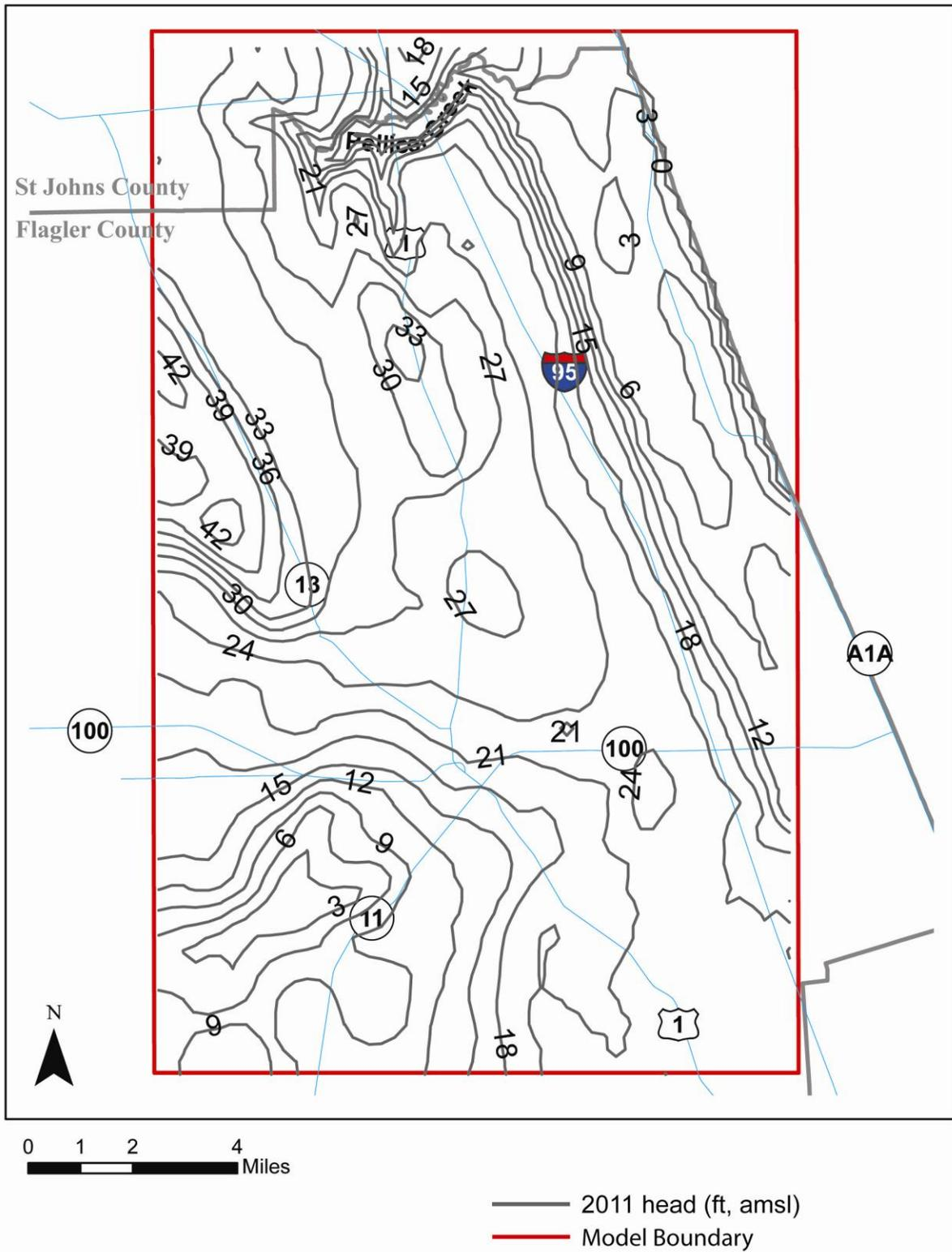
**Figure 81 Model simulated potentiometric surface of Unconfined Surficial aquifer for 2011**
