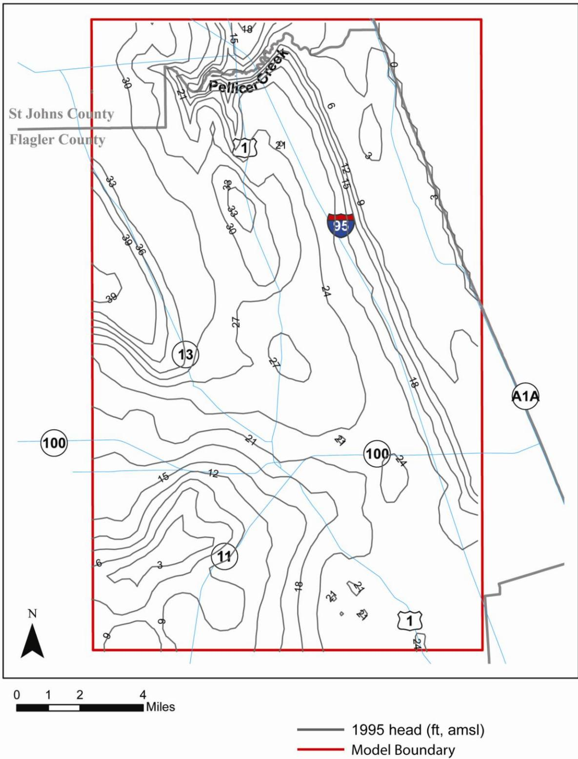
**Figure 50 Simulated average 1995 water table in Unconfined Surficial aquifer**
