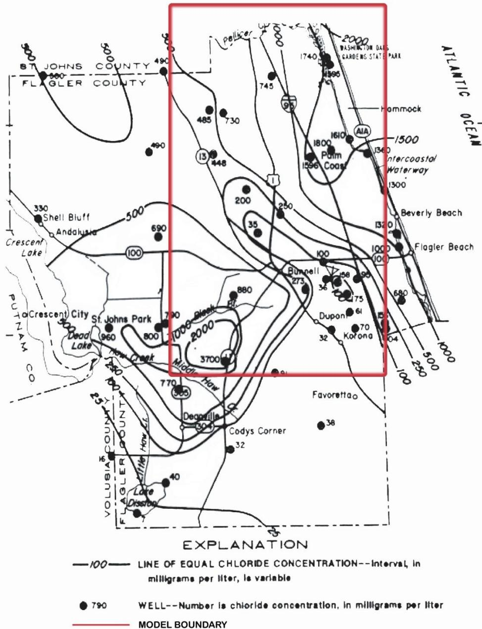
**Figure 33 Chloride concentration in the Upper Floridan aquifer**
