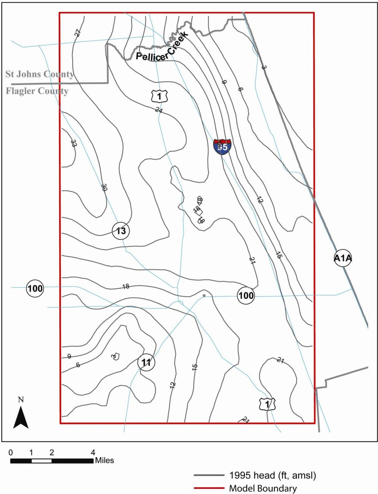
**Figure 54 Simulated average 1995 potentiometric surface in Confined Surficial aquifer**
