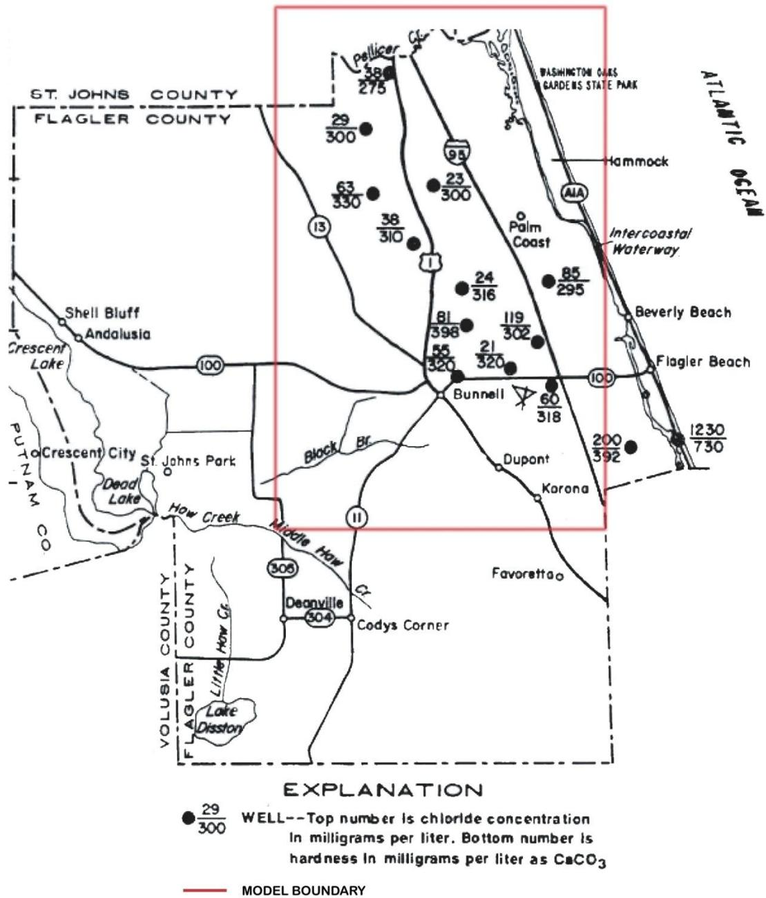
Figure 34 Chloride concentration and hardness in the Confined Surficial aquifer
