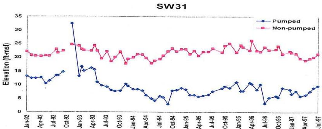
Water level hydrographs in Confined Surficial aquifer at SW-29, SW-30, and SW-31
