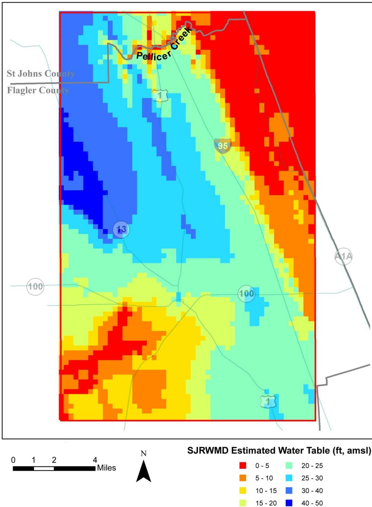
**Figure 42** Estimated water table in Unconfined Surficial aquifer
