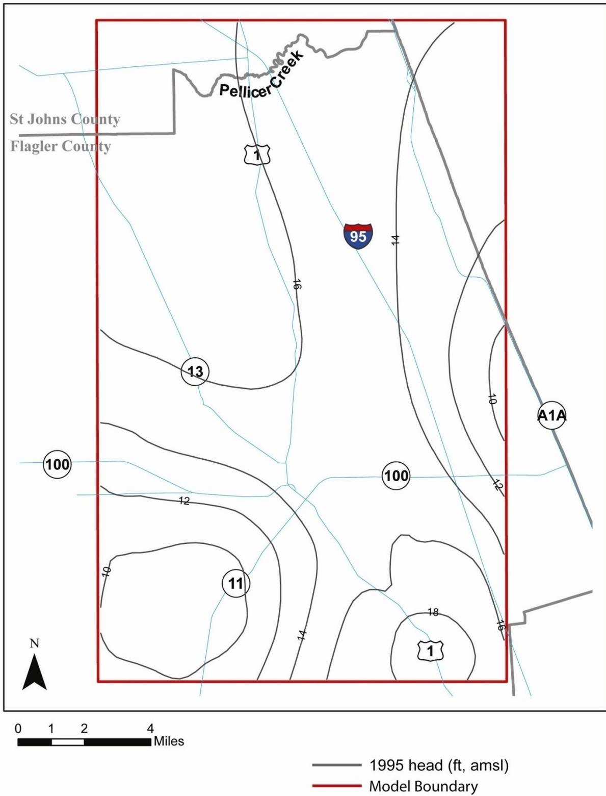
**Figure 58 Simulated average 1995 potentiometric surface in Upper Floridan aquifer**
