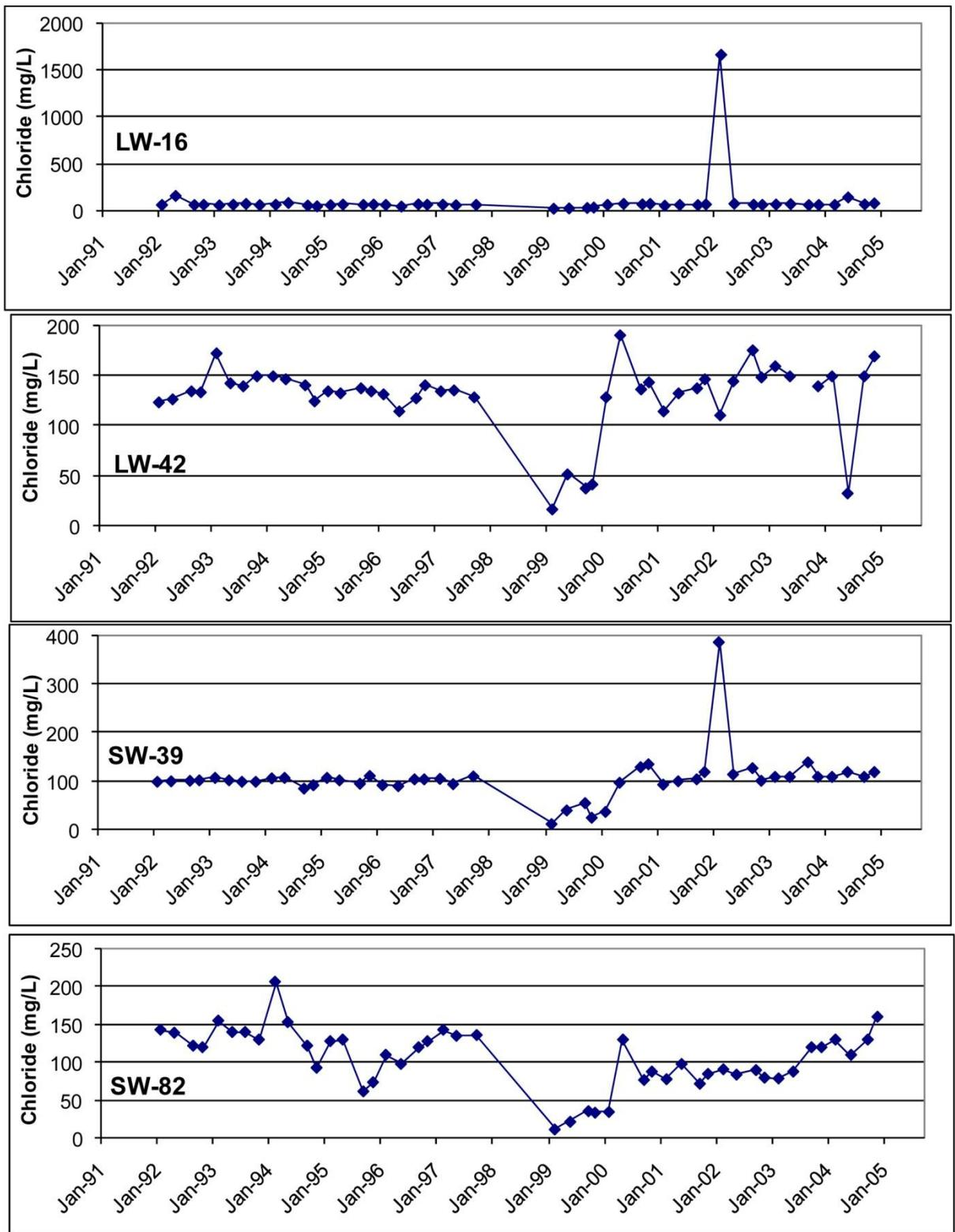
**Figure 37 Chloride concentration at Salt Water Intrusion Monitoring (SWIM) wells LW-16, LW-42, SW-39 and SW-82**
