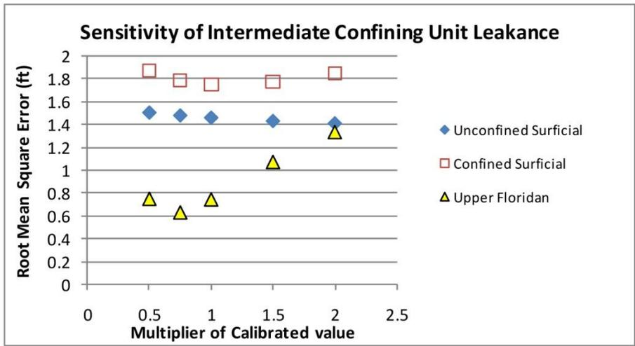
**Figure 77** Confining unit leakance sensitivity results for 1995 calibration period
