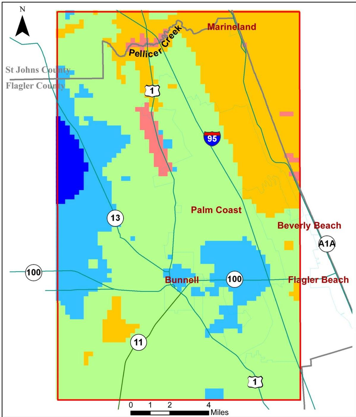
**Figure 69** Model derived Unconfined Surficial aquifer transmissivity
