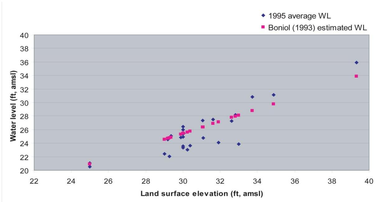
**Figure 41 Relationship between 1995 water levels in Unconfined Surficial aquifer and land surface elevation**
