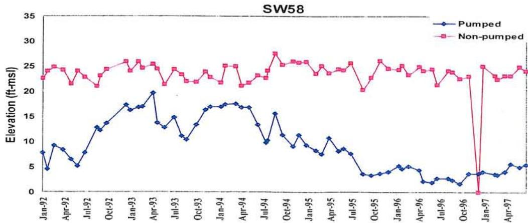
**Water level hydrographs in Confined Surficial aquifer at SW-35, SW-36, and SW-58**
