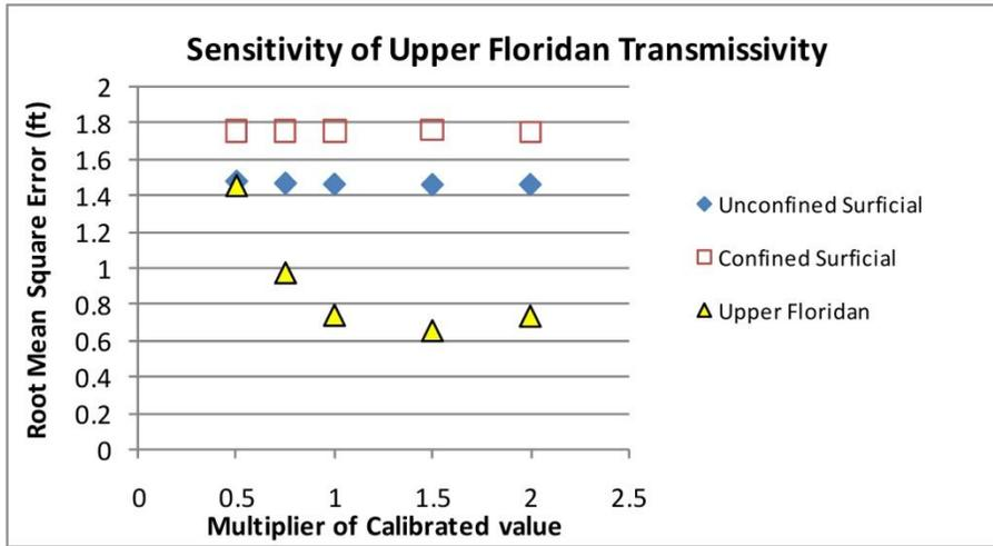
**Figure 76** Aquifer transmissivity sensitivity results for 1995 calibration period
