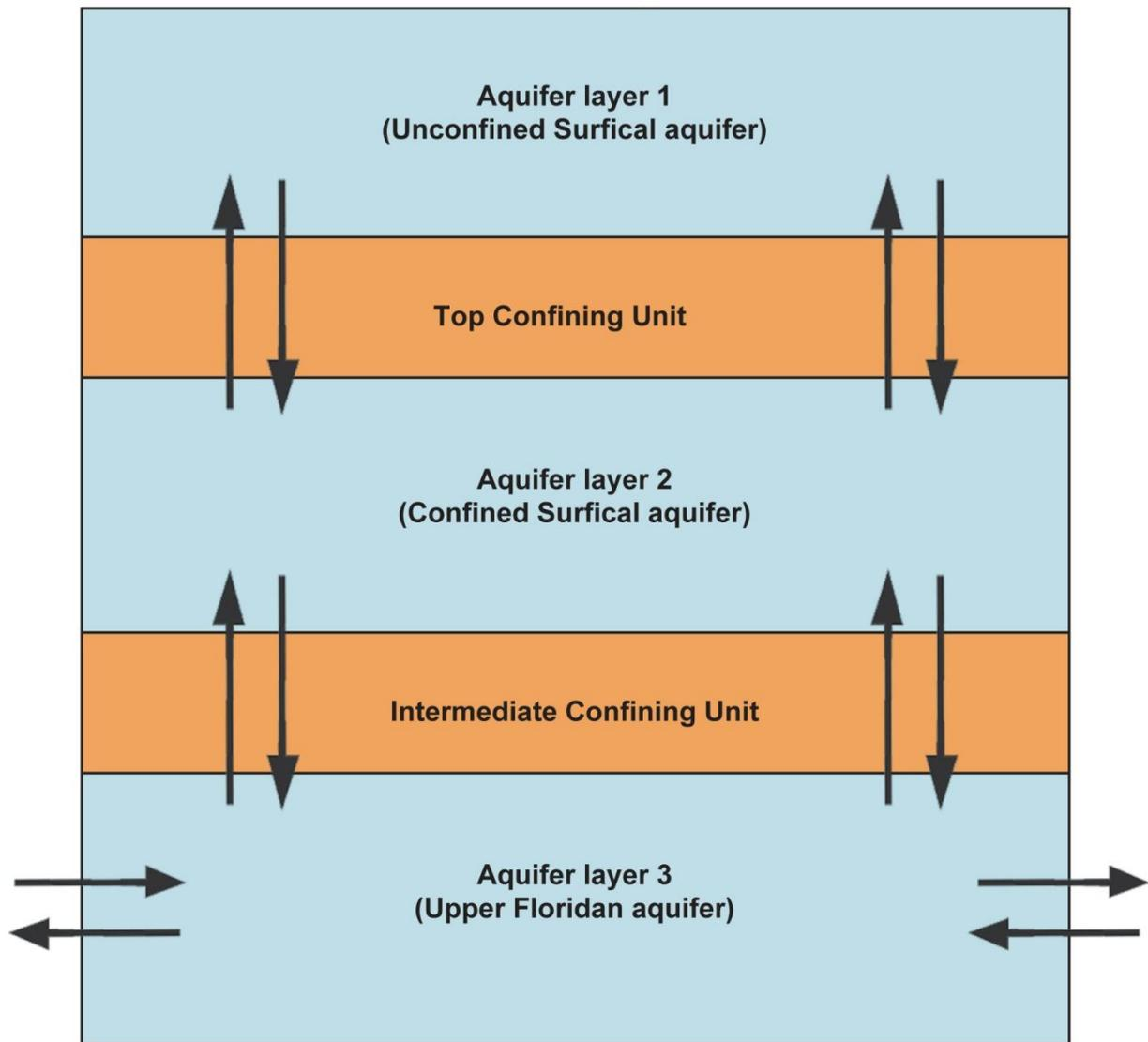
**Figure 49** Conceptualization of groundwater model
