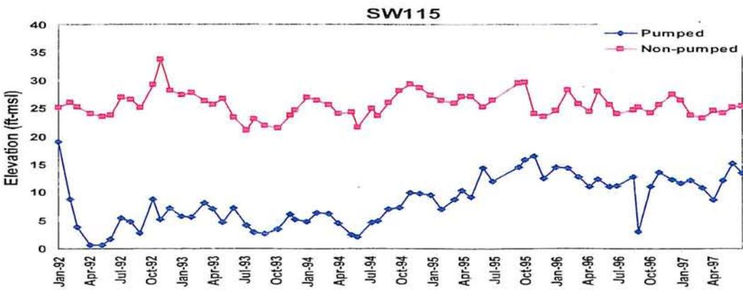
Water level hydrographs in Confined Surficial aquifer at SW-107, SW-114, and SW-115
