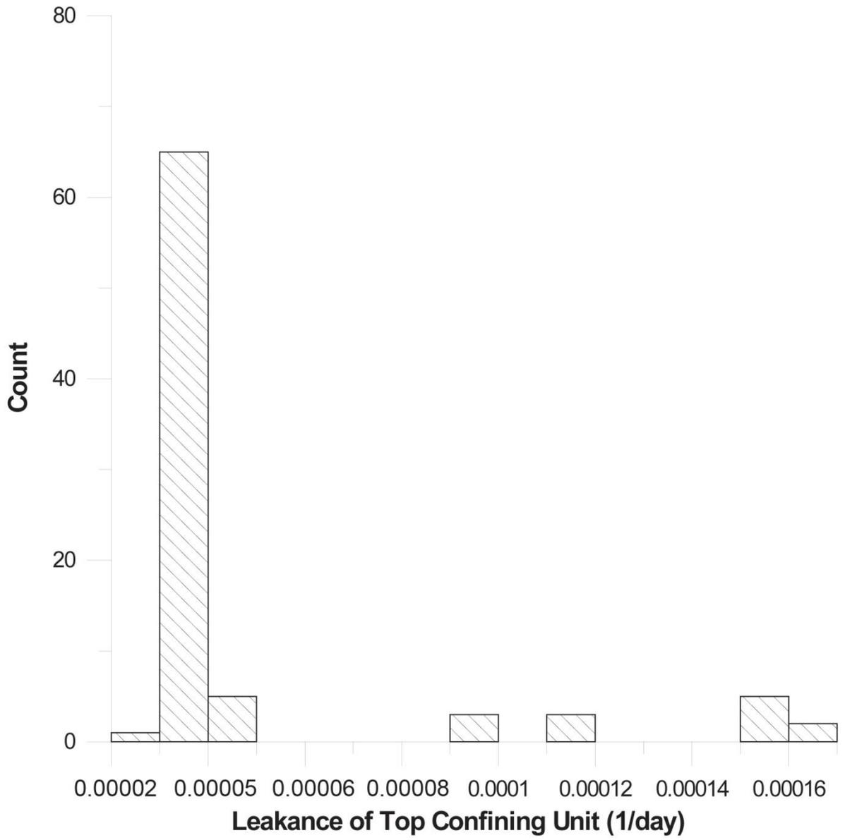
**Figure 25 Histogram of field based leakance of Top Confining Unit**
