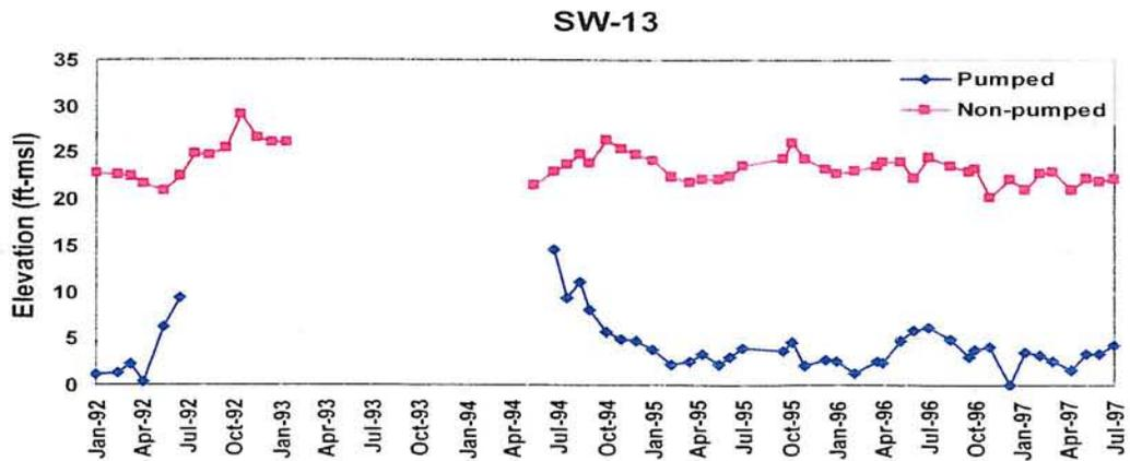
Water level hydrographs in Confined Surficial aquifer at SW-7, SW-8, and SW-13
