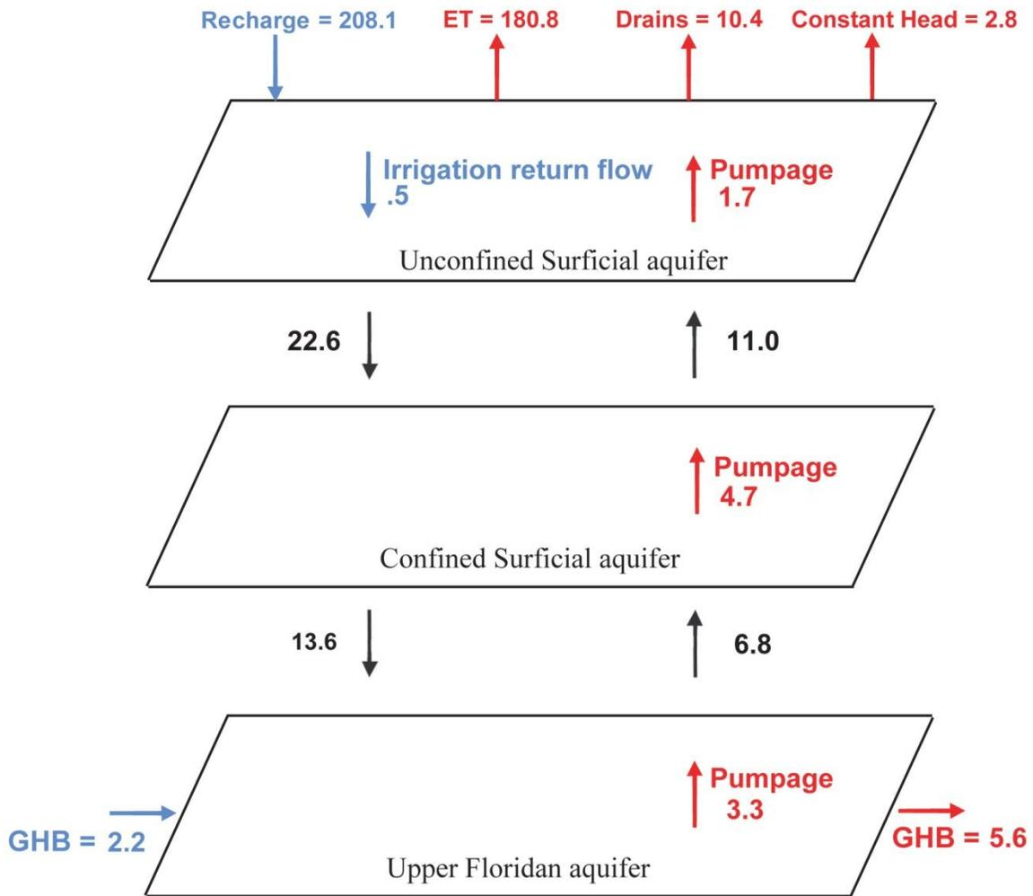
**Figure 63 Model simulated water budget for 1995**
