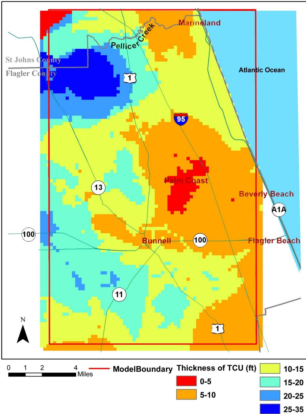
**Figure 18** Total thickness of Top Confining Unit
