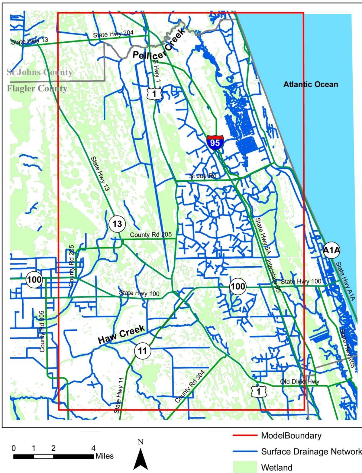
**Figure 4** Drainage network in study area
