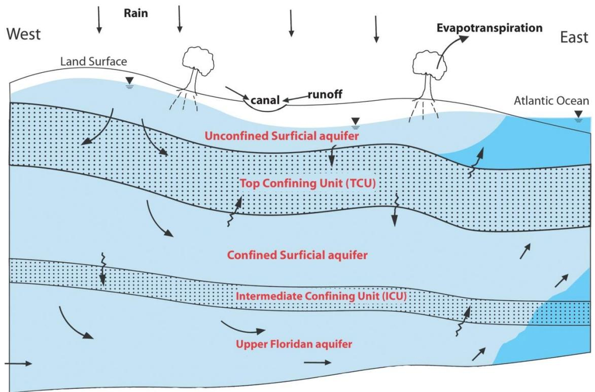
**Figure 48** Conceptual model of groundwater flow
