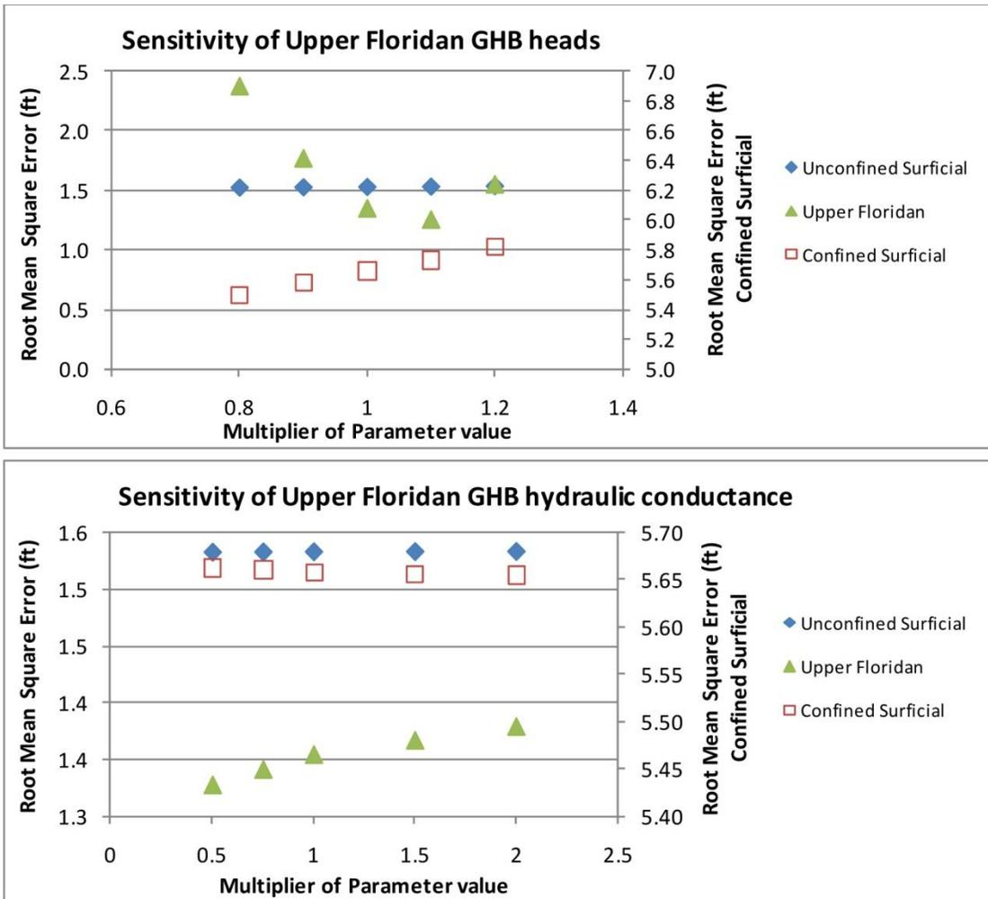
**Figure 91** General-Head Boundary sensitivity simulation mean square error results for 2011
