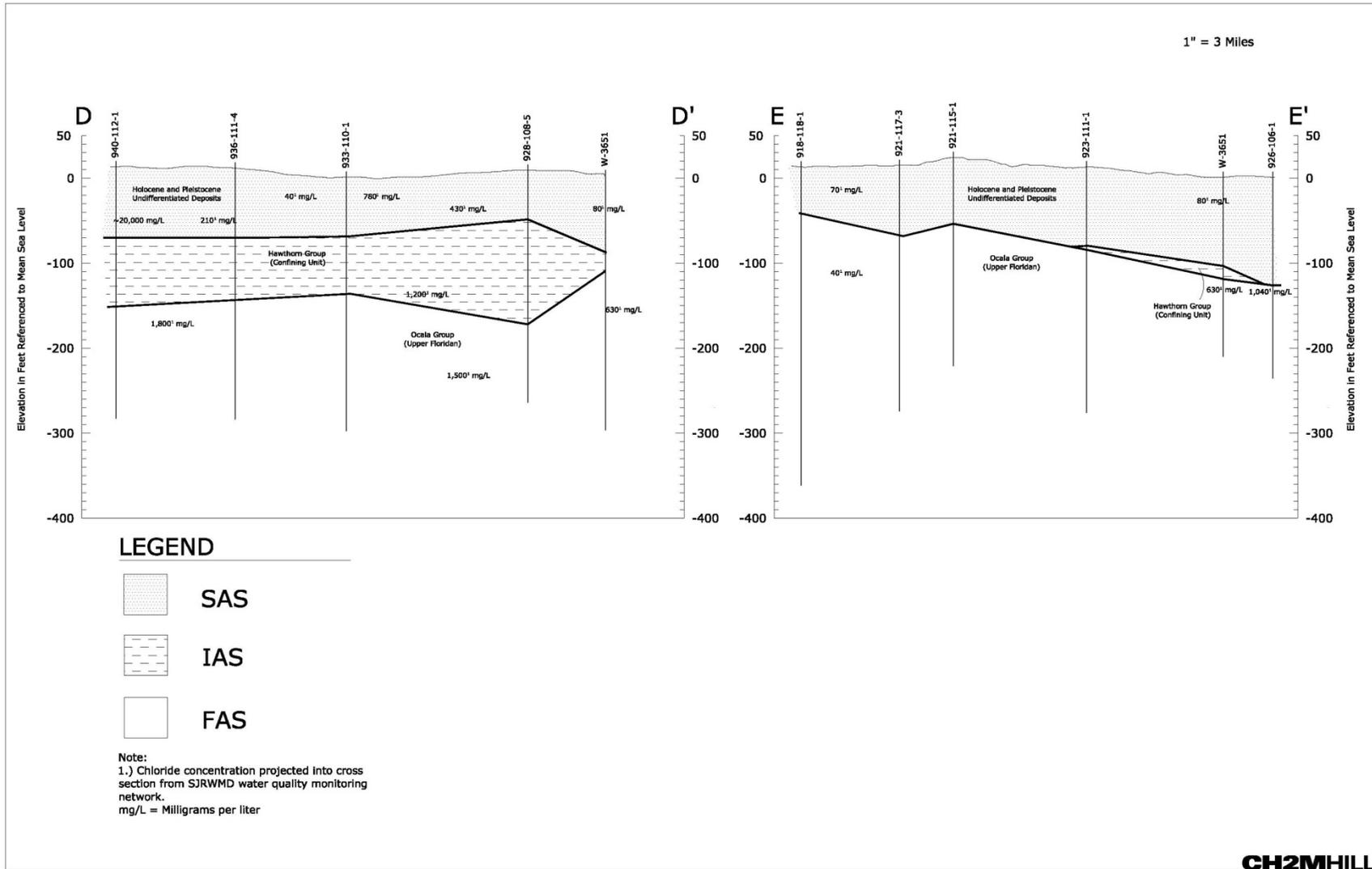
Figure 7. Hydrogeologic cross sections in Flagler County
