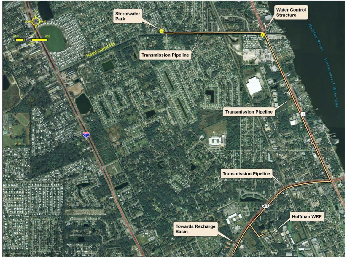
**Figure 5. Conceptual pipeline for diversion of stormwater from Reed Street Canal system**
