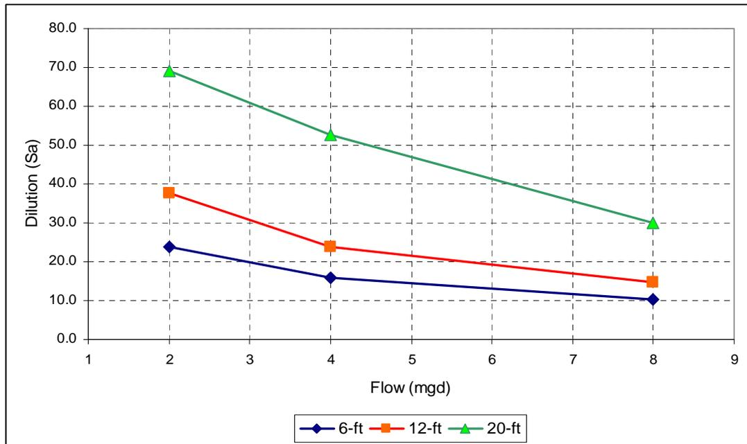
Figure 33. Dilution at the water surface for a median velocity and 95 percentile salinity case at Sanford location (summer conditions)
