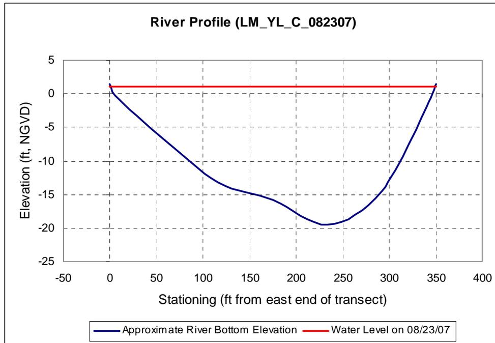
Figure 20. Bottom substrate elevations in relation to water level on August 23, 2007, at transect LM\_YL\_C
