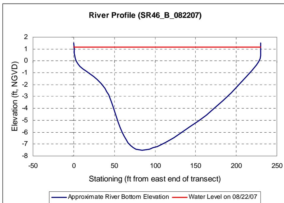
Figure 23. Bottom substrate elevations in relation to water level on August 22, 2007, at transect SR46\_B
