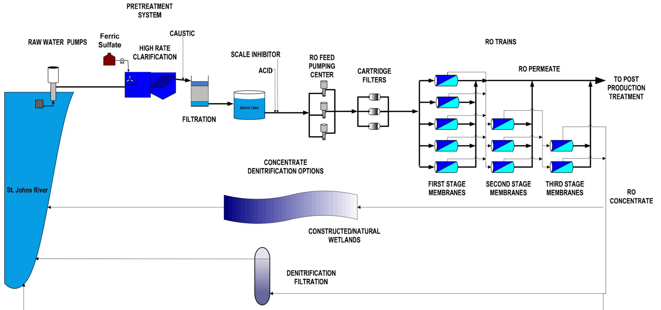
Figure 35. Process schematic for high-rate clarification, reverse osmosis, and optional concentrate treatment processes
