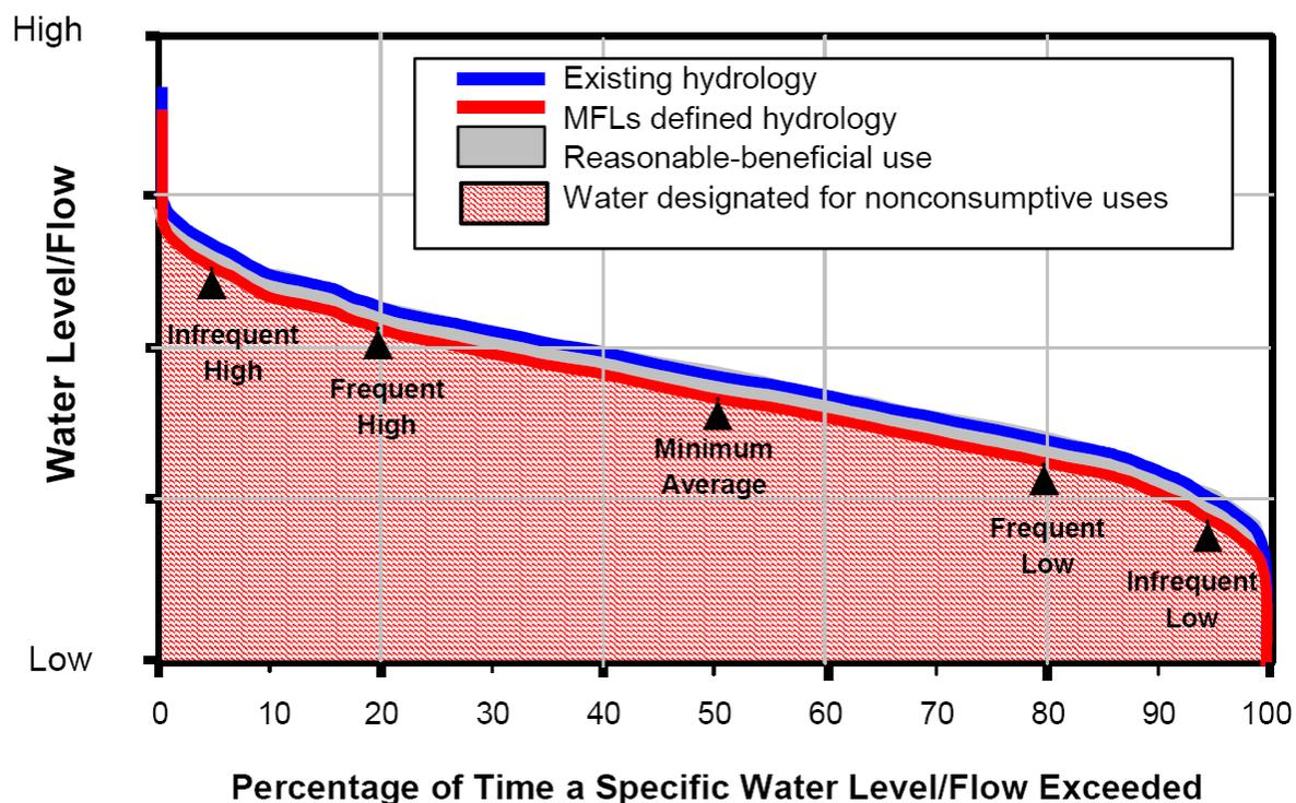
Figure 11. Hypothetical percentage exceedance curves for existing and MFLs-defined hydrologic conditions (Mace 2007a)
