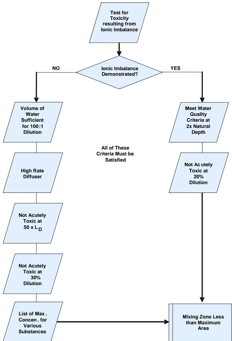
Figure 2. Selected Florida criteria for determining mixing zones when discharge is acutely toxic (Rule 62-4.244, F.A.C.)
