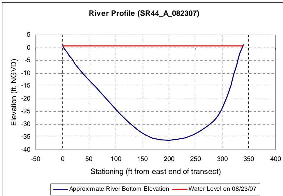
Figure 13. Bottom substrate elevations in relation to water level on August 23, 2007, at transect SR44\_A
