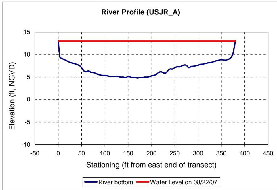
Figure 26. Bottom substrate elevations in relation to water level on August 22, 2007, at transect USJR\_A
