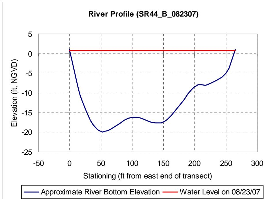
Figure 14. Bottom substrate elevations in relation to water level on August 23, 2007, at transect SR44\_B
