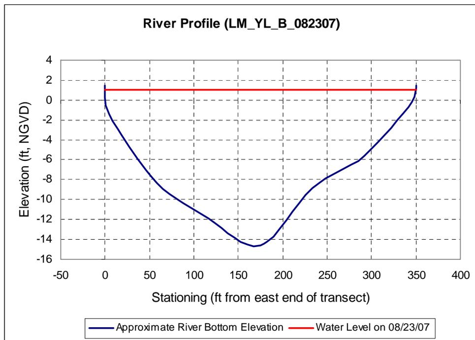
Figure 19. Bottom substrate elevations in relation to water level on August 23, 2007, at transect LM\_YL\_B
