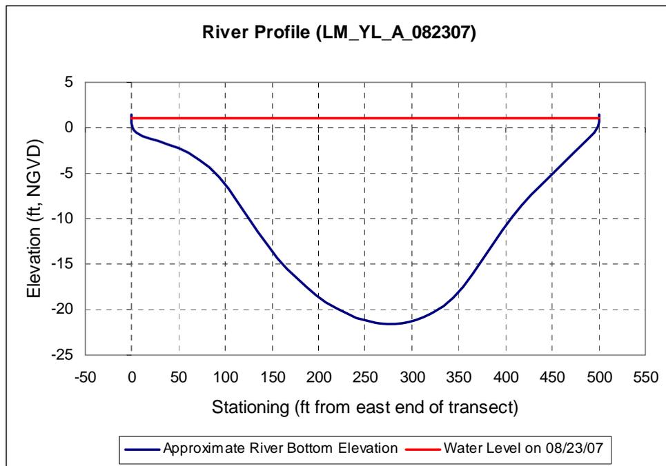
Figure 18. Bottom substrate elevations in relation to water level on August 23, 2007, at transect LM\_YL\_A
