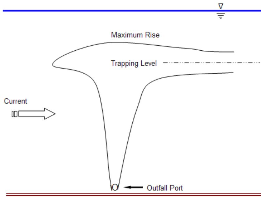
Figure 30. Example of a trapped plume
