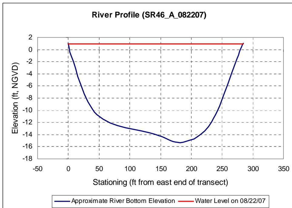
Figure 22. Bottom substrate elevations in relation to water level on August 22, 2007, at transect SR46\_A
