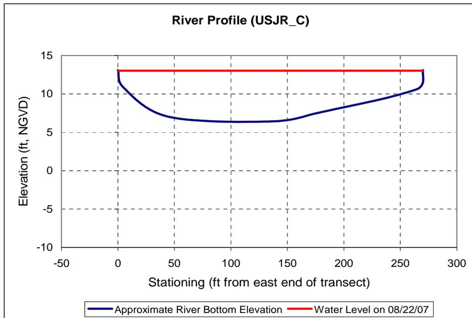
Figure 28. Bottom substrate elevations in relation to water level on August 22, 2007, at transect USJR\_C
