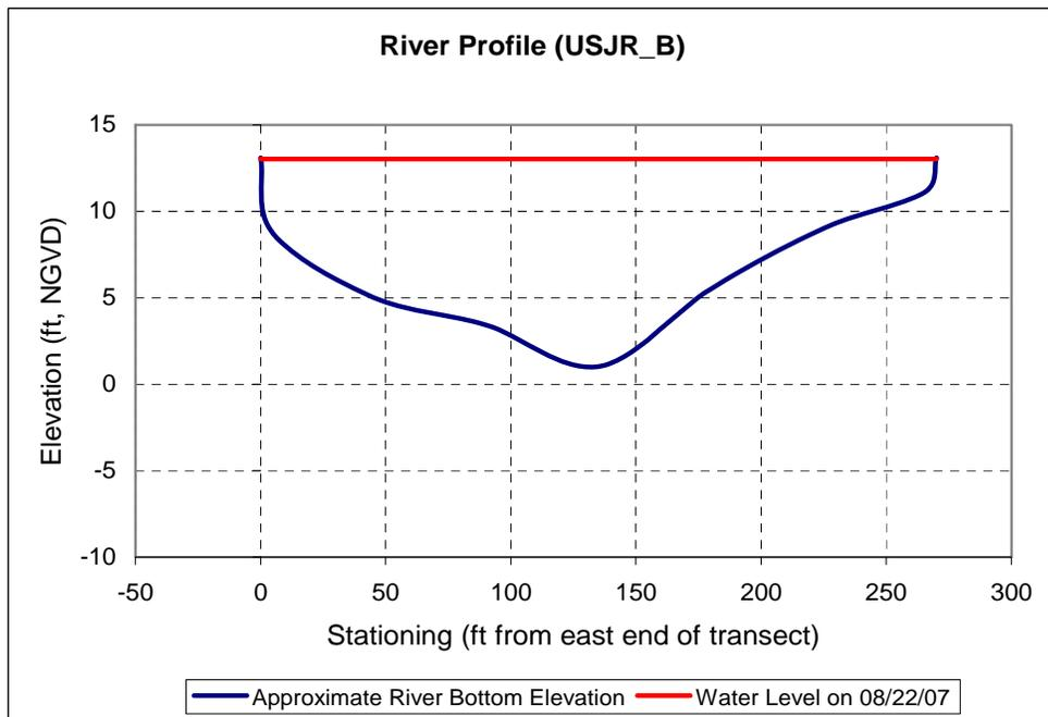
Figure 27. Bottom substrate elevations in relation to water level on August 22, 2007, at transect USJR\_B
