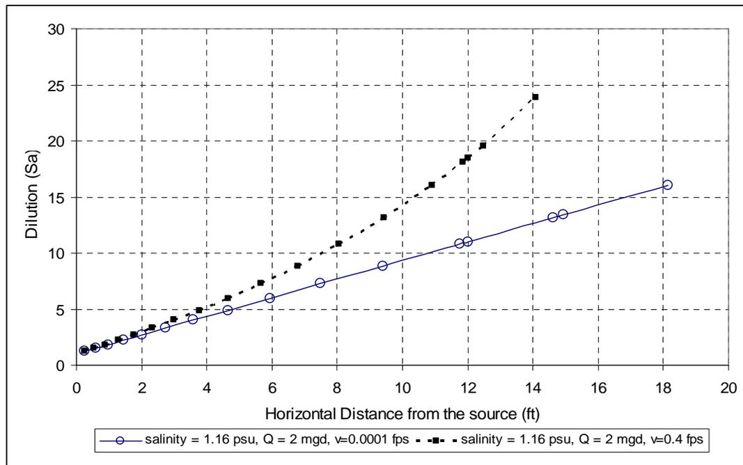
Figure 34. Dilution versus distance for high salinity at Sanford location
