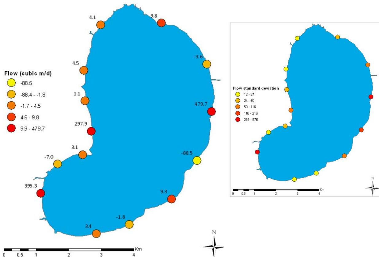
Fig. 57 – Well locations and estimated mean flow rates (to lake = positive, out of lake = negative). Flow estimates are in  $m^3/day$  across a seepage face that extends from each sampling well halfway to the next well in each direction. Inset is flow standard deviation, also in  $m^3/day$ .
