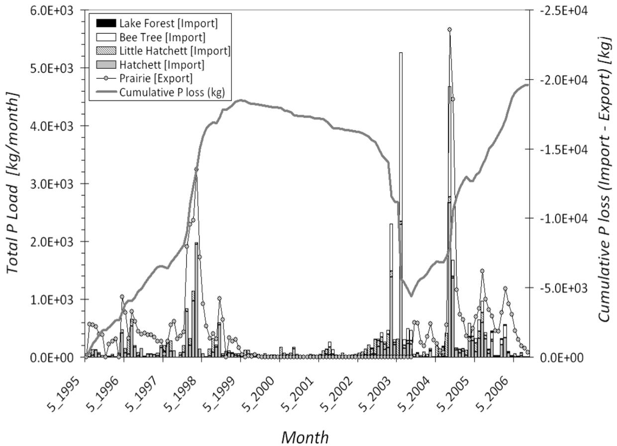
Fig. 75 – Estimated P balance (Imports = bars; Exports = black line with grey circles) between May 1995 and September 2006. The cumulative P deficit (grey line) is just under 20 metric tons.
