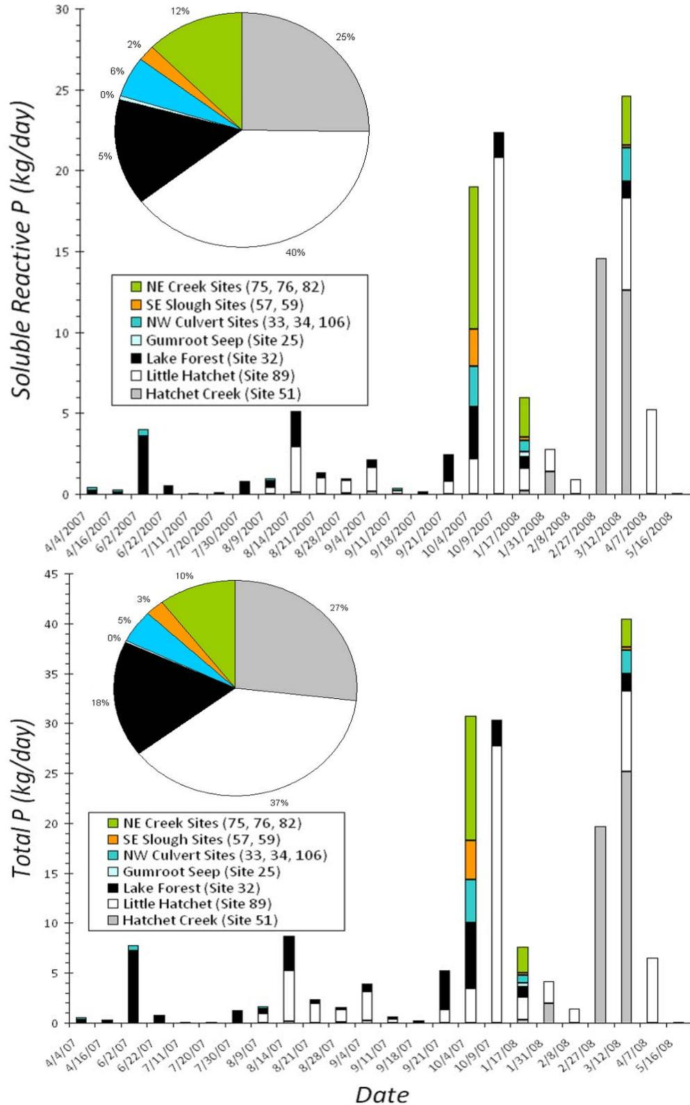
Fig. 77 – Loading of P loads (soluble and total) to Newnans Lake from multiple sources for each sampling instance ( $\pm 2$  days) for which data available. Inset is estimate of total fractional load for the period of record.
