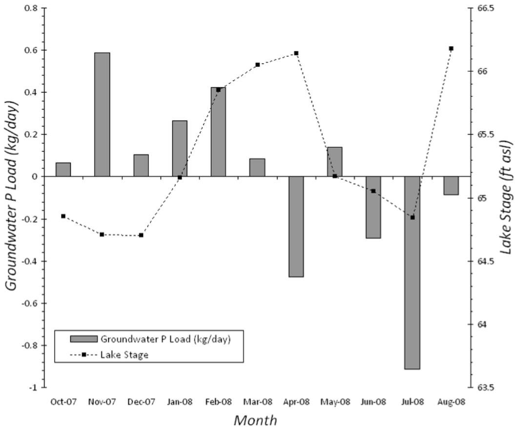
Fig. 63 – Monthly load of P to Newnans Lake from groundwater as inferred from perimeter wells. Note that groundwater is a sink for P (i.e., high TP concentrations leaving the lake) during April and July 2008.
