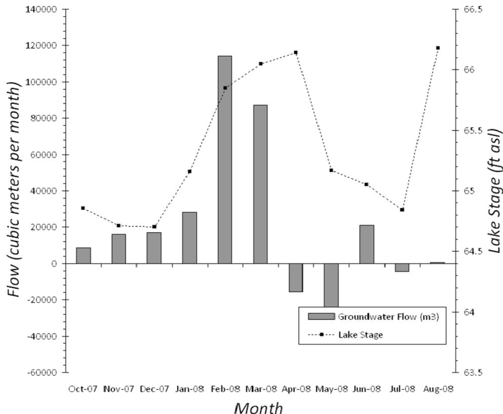
Fig. 59 – Estimated groundwater flow ( $\text{m}^3$  per month) and lake stage over period of observation.
