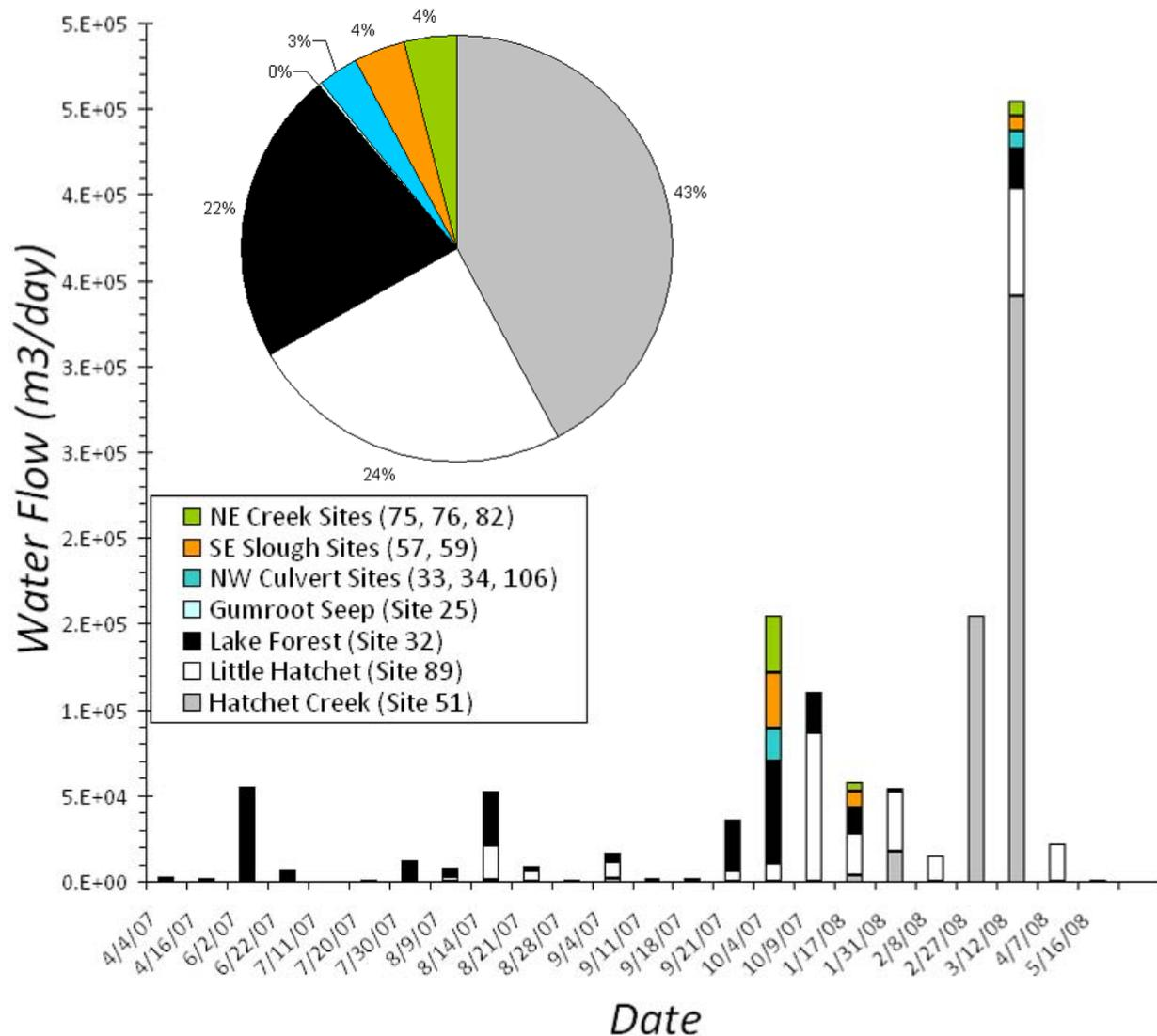
Fig. 76 – Loading of water flows to Newnans Lake from multiple sources for each sampling instance ( $\pm 2$  days) for which data available. Inset is estimate of total fractional load for the period of record.
