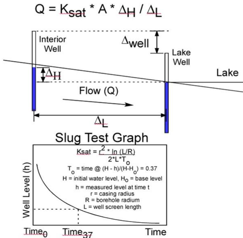
Fig. 11 – Schematic of well elevation measurements for inference of groundwater flow, including (lower panel) estimation of hydraulic conductivity from a slug test.
