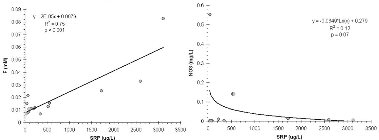
*Fig. 62 – Mean well concentrations of SRP vs. covariates suggestive of source. A) Covariance with F, a tracer of geologic P, and B)  $\text{NO}_x$ , a tracer of fertilizer or wastewater sources. Positive covariance with F suggests that most of the P arriving to the lake from groundwater is of geologic origin (though extreme values of F at one site may be due to F loading from municipal water supply). Correlations with  $\text{NO}_x$  are negative but not statistically significant.*
