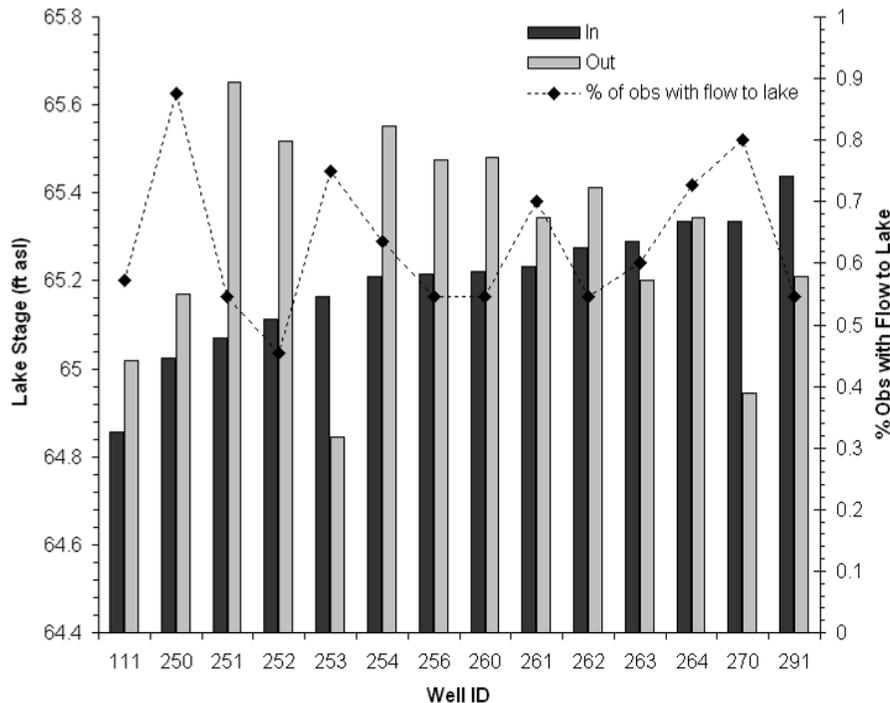
*Fig. 58 – Mean lake stage for flows into and out of the lake from each well. Flows out of the lake occur at higher lake stage for most wells, but flow reversal does not occur at the same lake stage. Note that not all wells were visited all months due to access constraints.*
