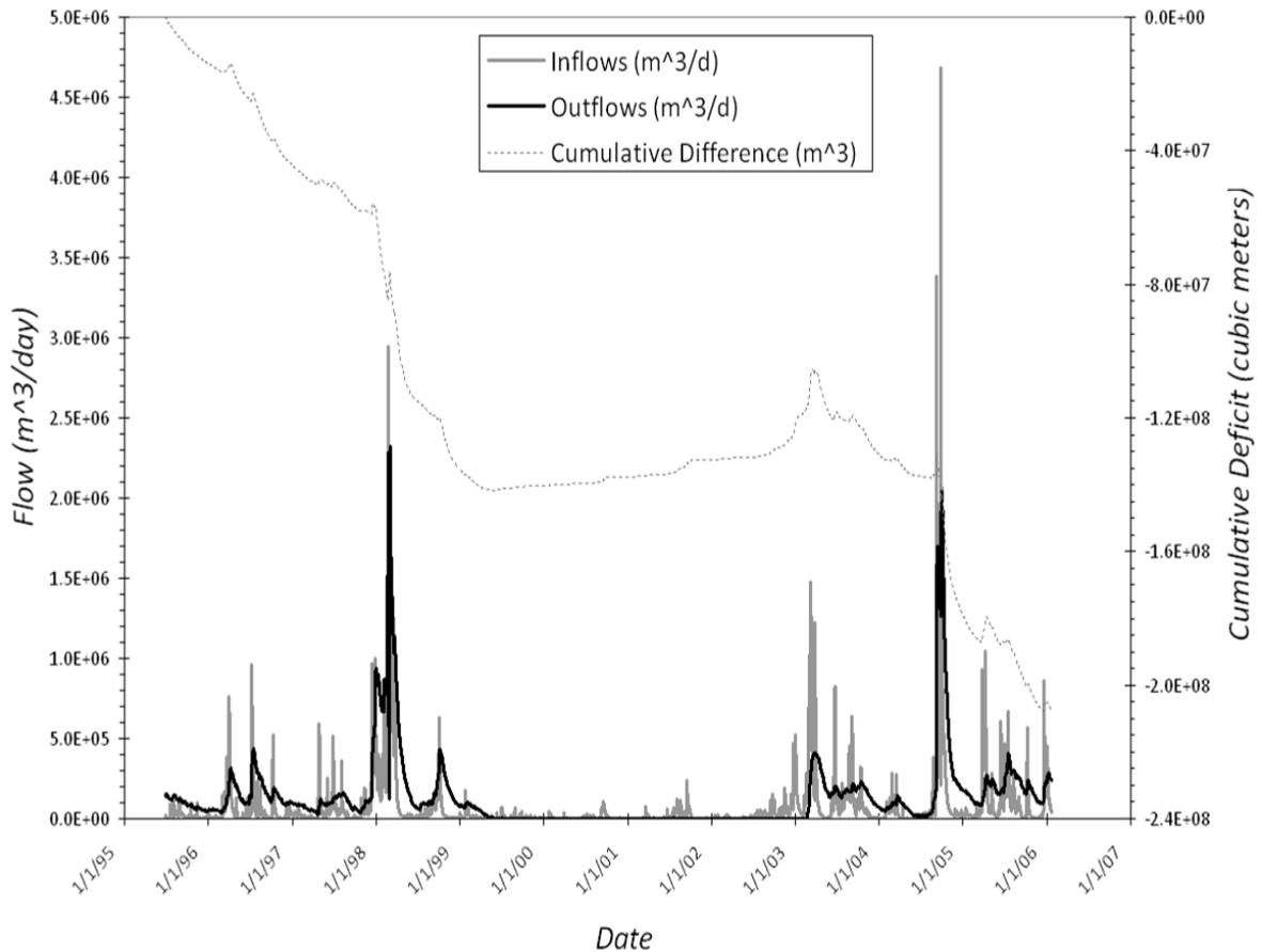
Fig. 69 – Water budget for Newnans Lake for June 1995 though April 2006. Inflows (sum of measured creek flows) minus outflows (Prairie Creek) are summed over the period of record to determine the period deficit. Net rainfall inputs (precipitation – evaporation) average  $5.8E+06 \text{ m}^3$  per year over the lake area ( $6.1E7$ ).
