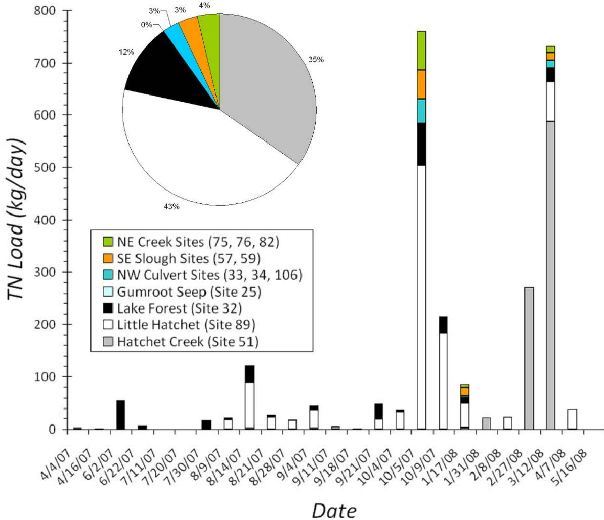
Fig. 79 – Loading of N to Newnans Lake from multiple sources for each sampling instance ( $\pm 2$  days) for which data available. Inset is estimate of total fractional load for the period of record.
