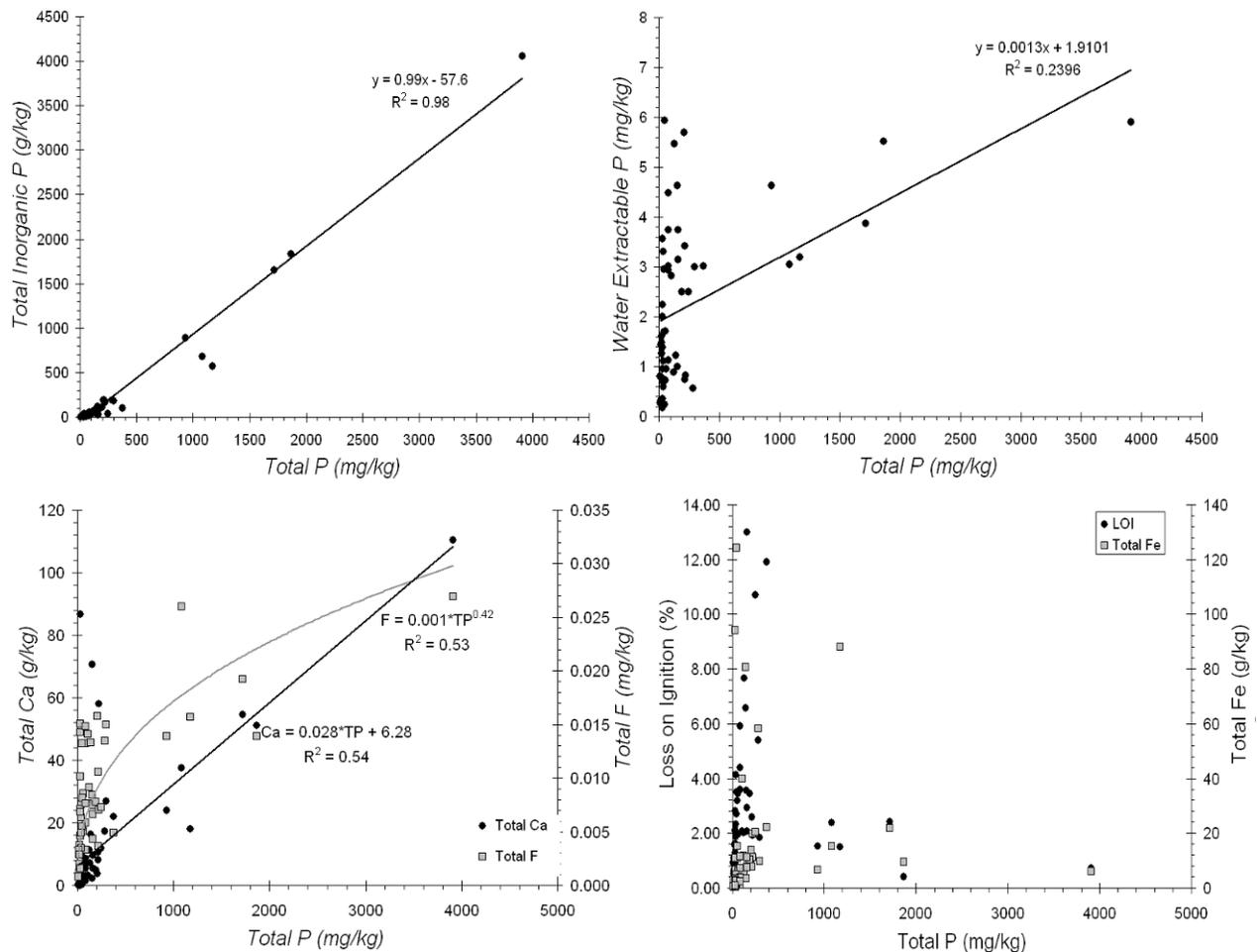
Fig. 65 – Patterns of covariance within creek sediments. A) Between total P and total inorganic P; B) Between total P and water extractable P, C) Between total P and Ca and F, D) between total P and LOI and Fe. Together, these suggest P is principally in mineral form in creek sediments, and remains closely associated with fluoride bearing apatite minerals
