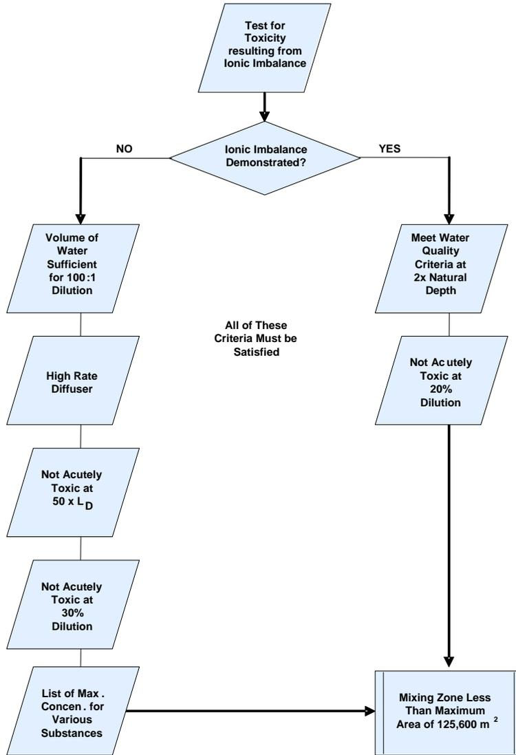
**FIGURE 1.** Selected Florida criteria for determining mixing zones when discharge is acutely toxic (62-4.244, F.A.C.).
