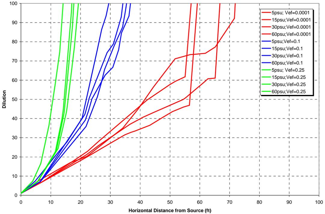
Figure 11. Dilution versus distance for selected cases to illustrate the sensitivity of dilution to ambient current speed
