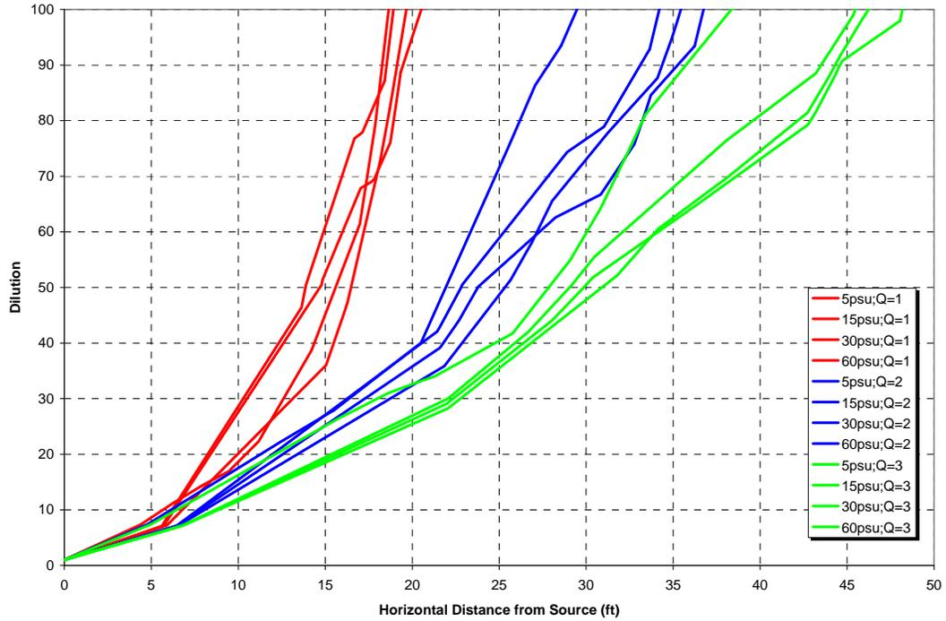
Figure 15. Dilution versus distance for selected cases to illustrate the sensitivity of dilution to port velocity
