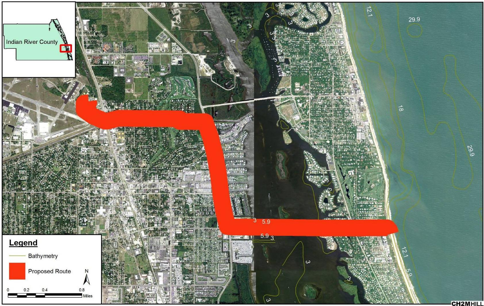
Figure 30. Conceptual route for a regional concentrate conveyance pipeline in Indian River County
