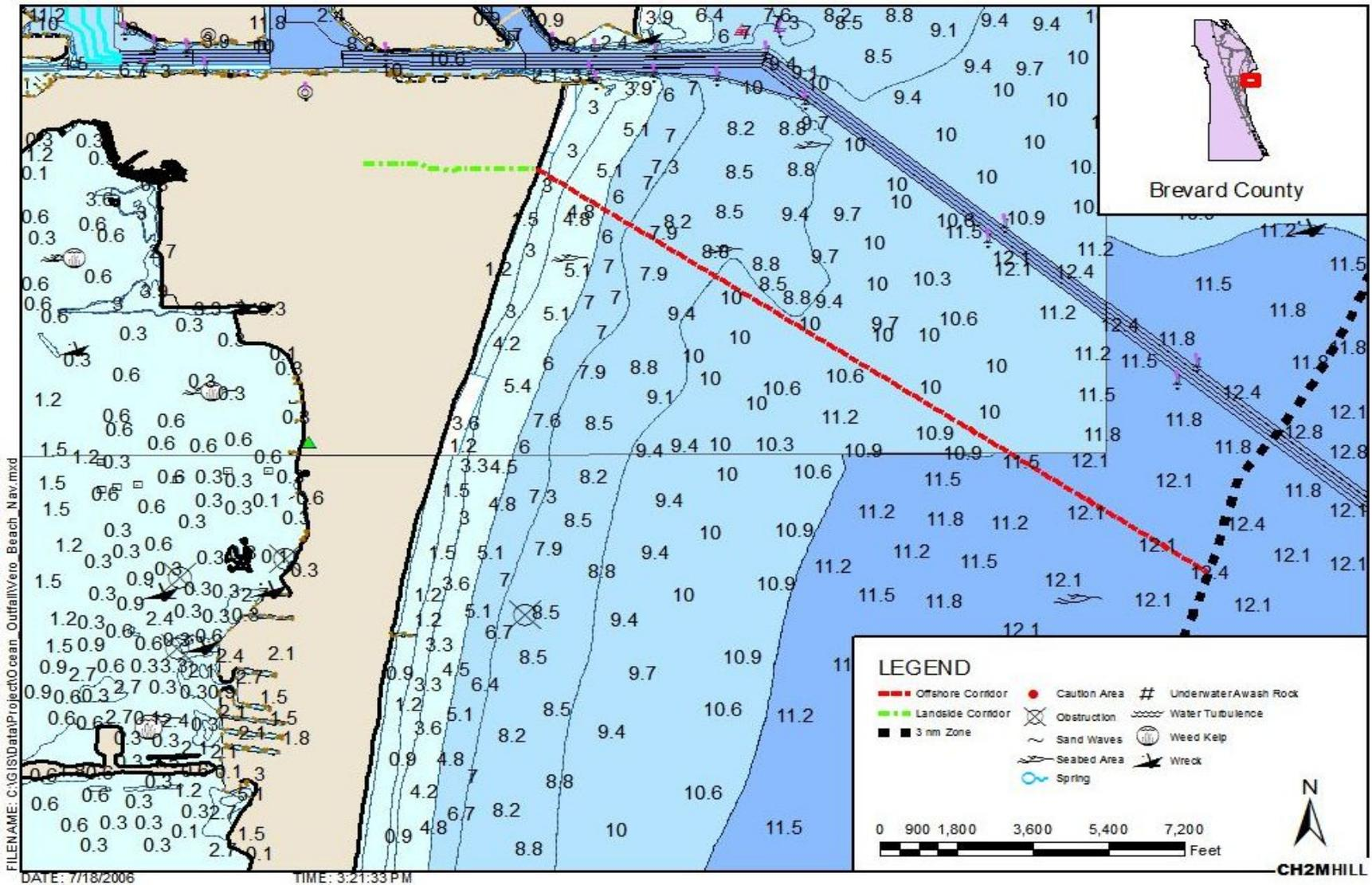
Figure 32. Potential location for an ocean outfall in Port Canaveral area (depths reported in meters)
