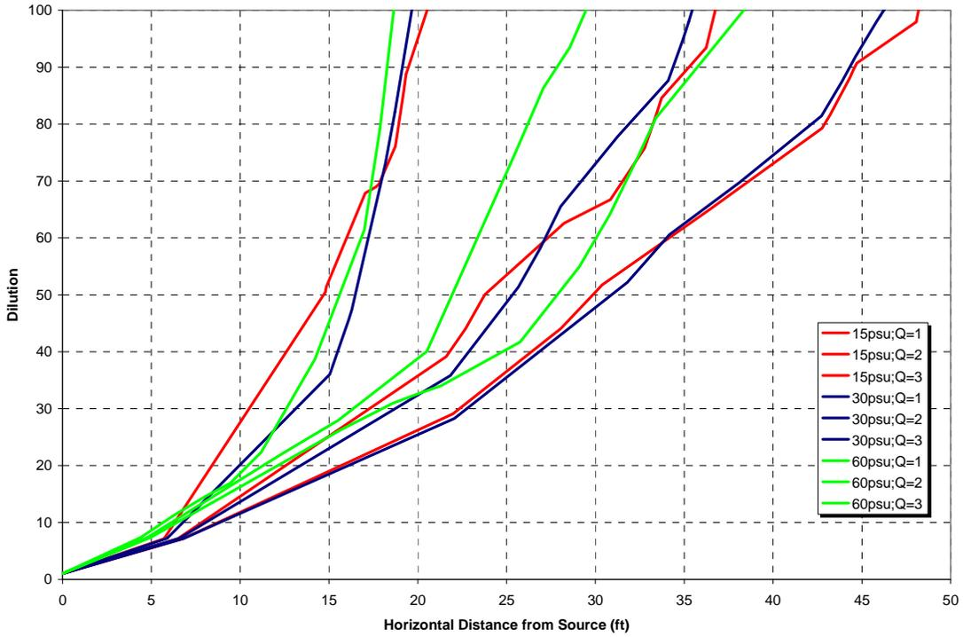
Figure 19. Dilution versus distance for selected cases to illustrate the sensitivity of dilution to discharge salinity
