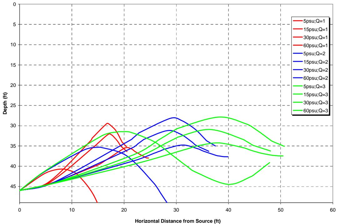
Figure 16. Plume depth versus distance for selected cases to illustrate the sensitivity of dilution to port velocity
