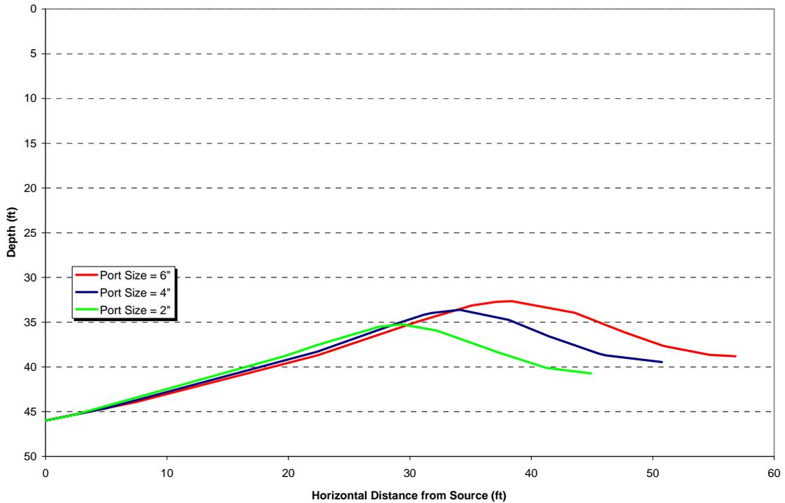
Figure 24. Depth versus distance for 6-in. (red), 4-in. (blue), and 2-in. (green) diameter ports with exit velocities at 15.8 fps
