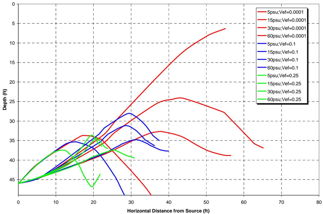
Figure 12. Plume depth versus distance for selected cases to illustrate the sensitivity of dilution to ambient current speed
