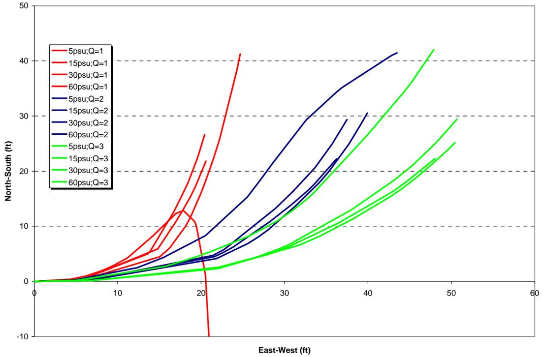
Figure 17. Plan view of plume trajectory for selected cases to illustrate the sensitivity of dilution to port velocity
