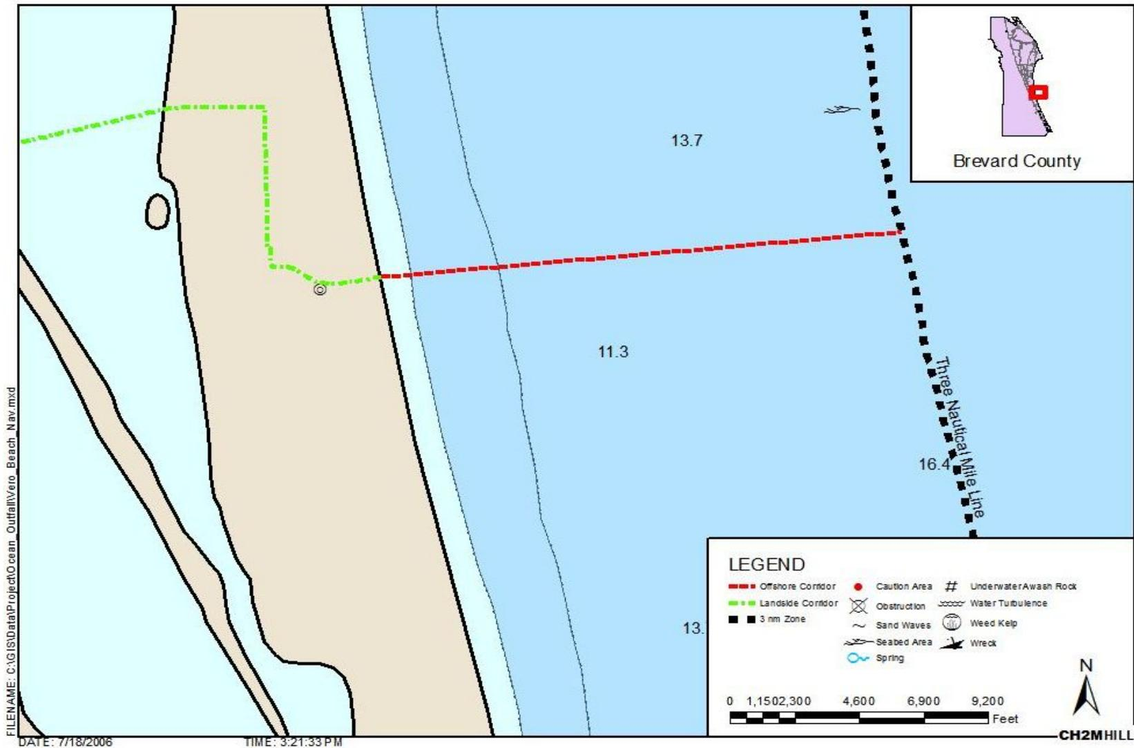
Figure 33. Potential location for an ocean outfall in the Satellite Beach area (depths reported in meters)
