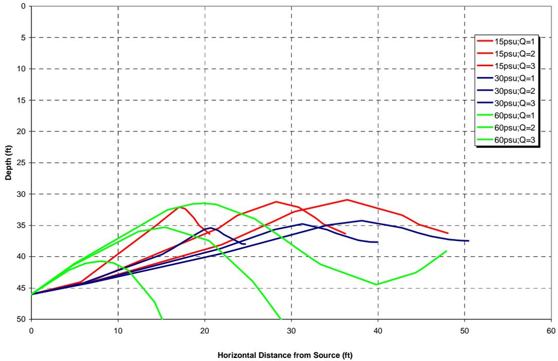
Figure 20. Plume depth versus distance for selected cases to illustrate the sensitivity of dilution to discharge salinity
