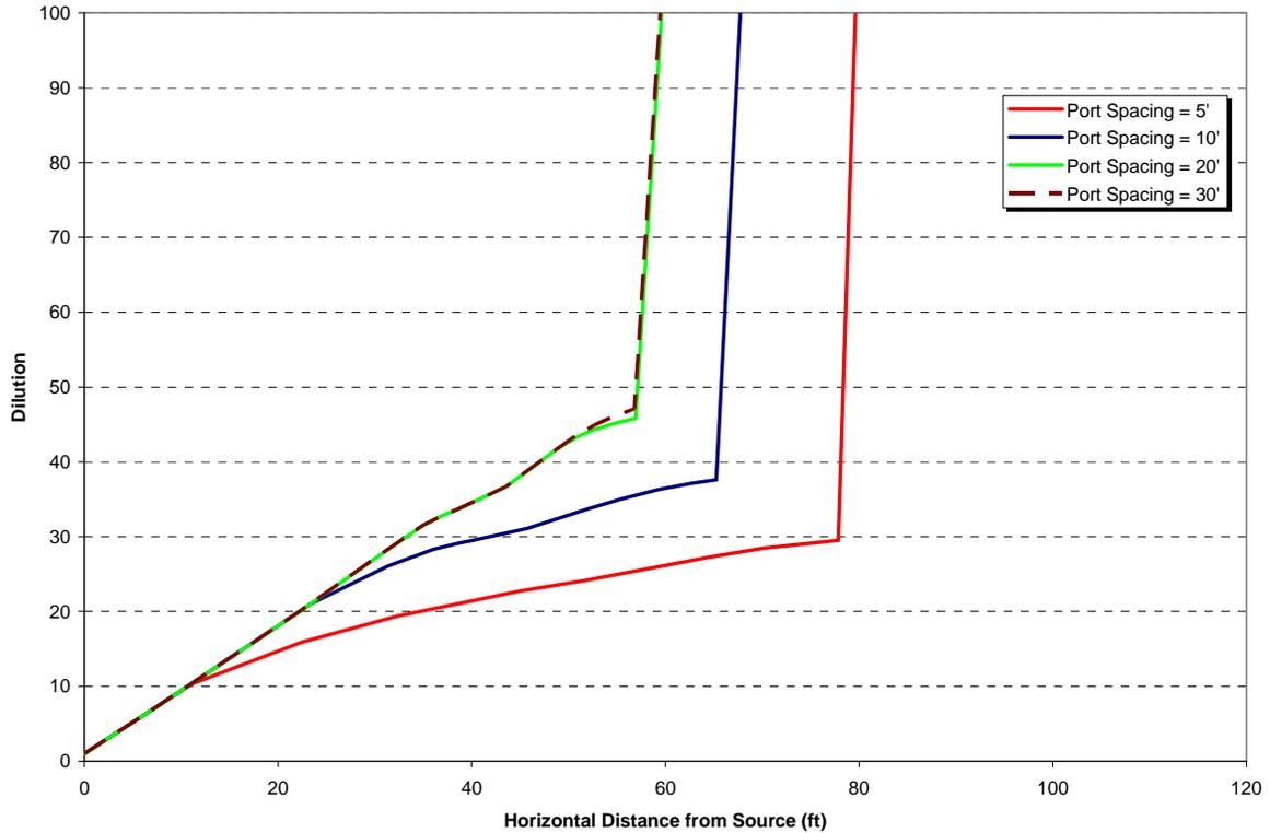
Figure 25. Dilution versus distance for port spacing of 5 (red solid), 10 (blue), 20 (green), and 30 ft (brown dashed)
