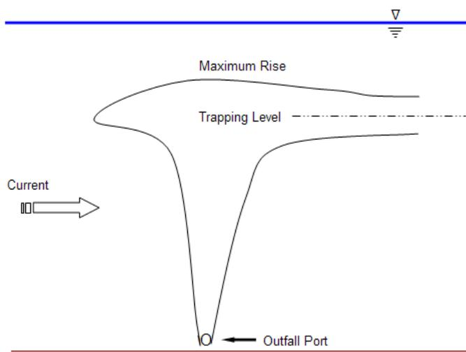
Figure 6. Example of a trapped plume
