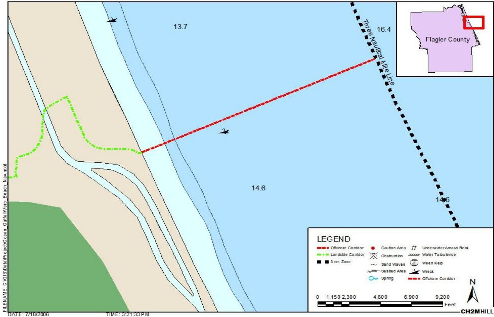
Figure 31. Potential location for an ocean outfall in the Flagler County area (depths reported in meters)
