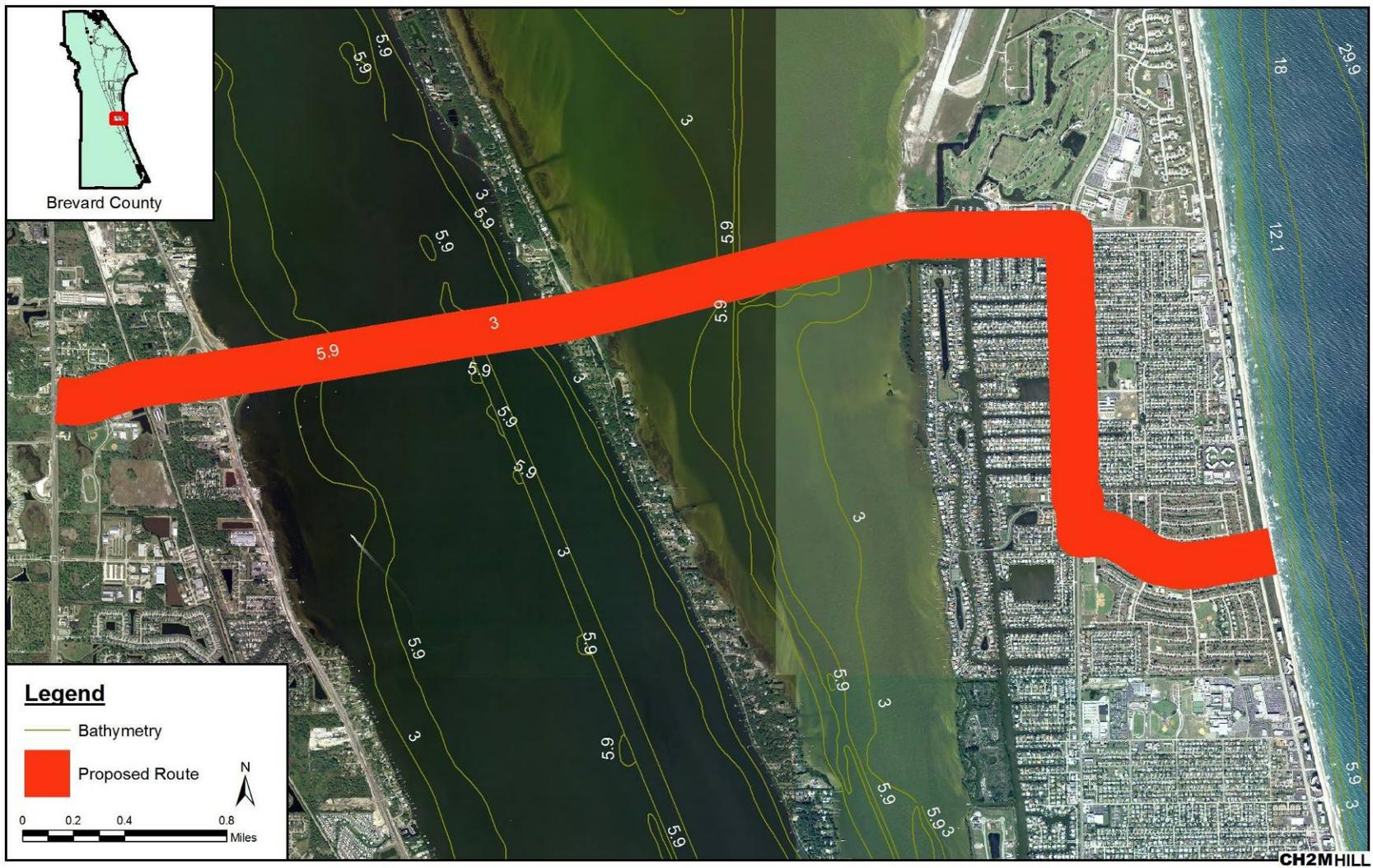
Figure 29. Conceptual route for a regional concentrate conveyance pipeline in Brevard County
