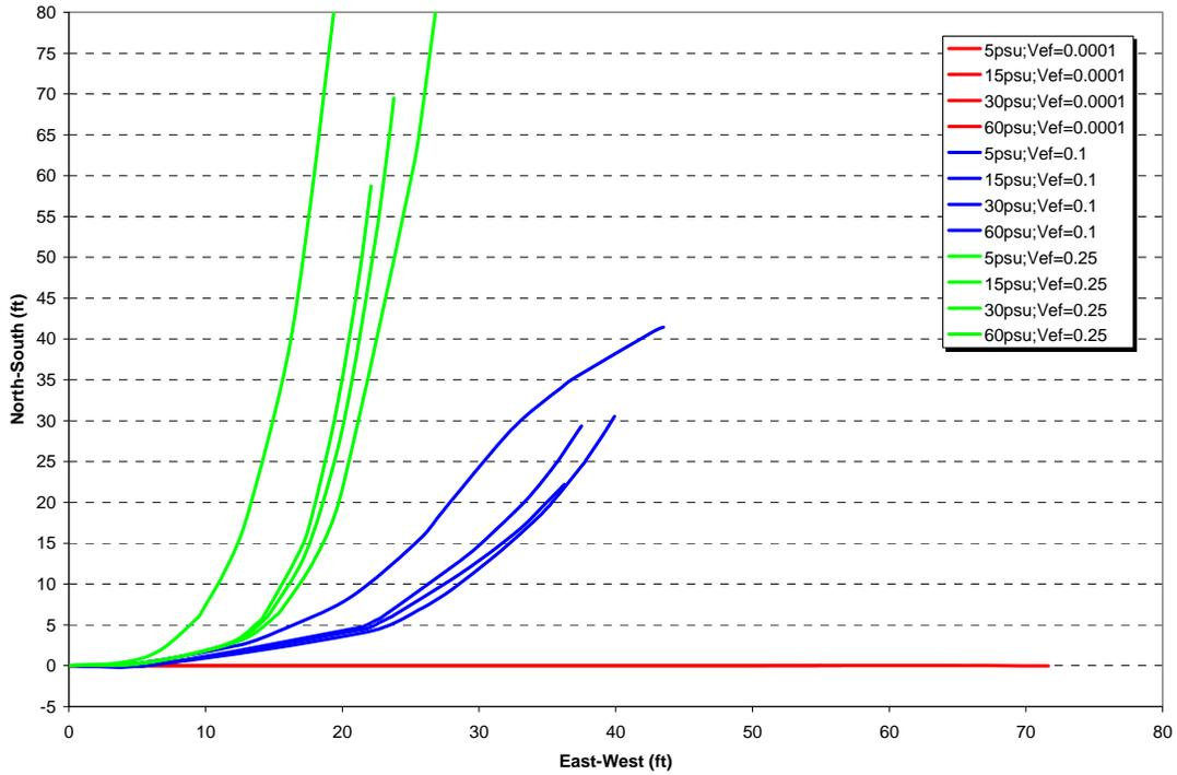
Figure 13. Plan view of plume trajectory for selected cases to illustrate the sensitivity of dilution to ambient current speed
