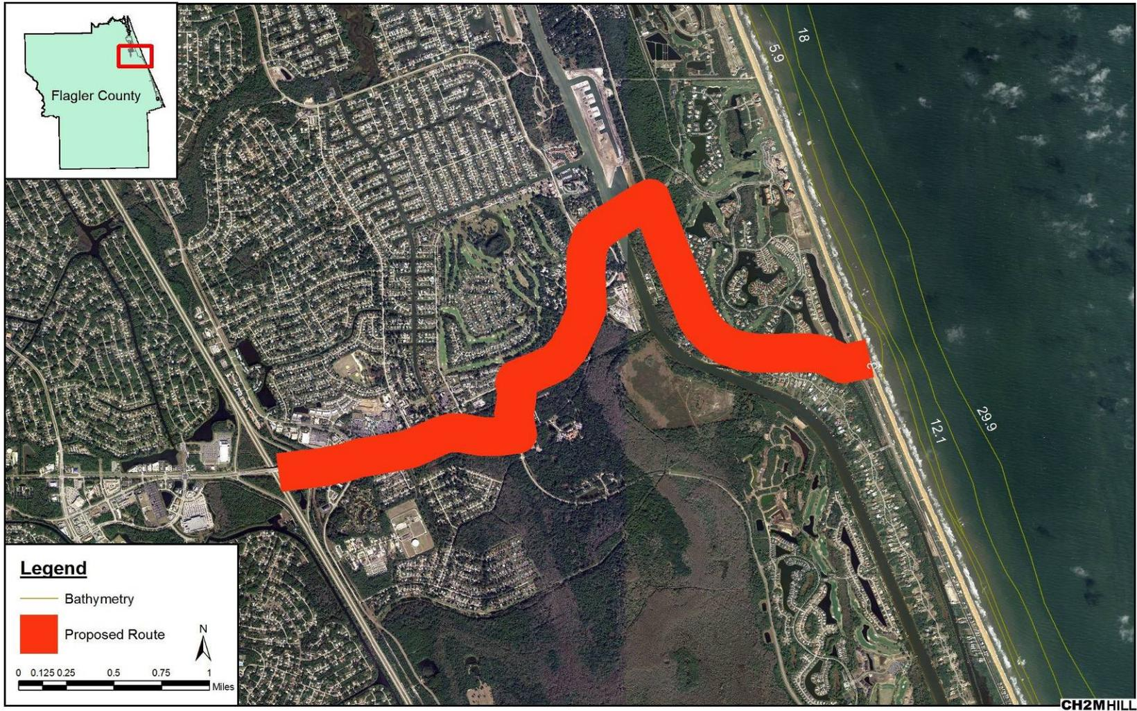
Figure 27. Conceptual route for a regional concentrate conveyance pipeline in Flagler County
