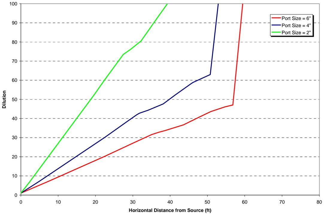
Figure 23. Dilution versus distance for 6-in. (red), 4-in. (blue), and 2-in. (green) diameter ports with exit velocities at 15.8 fps
