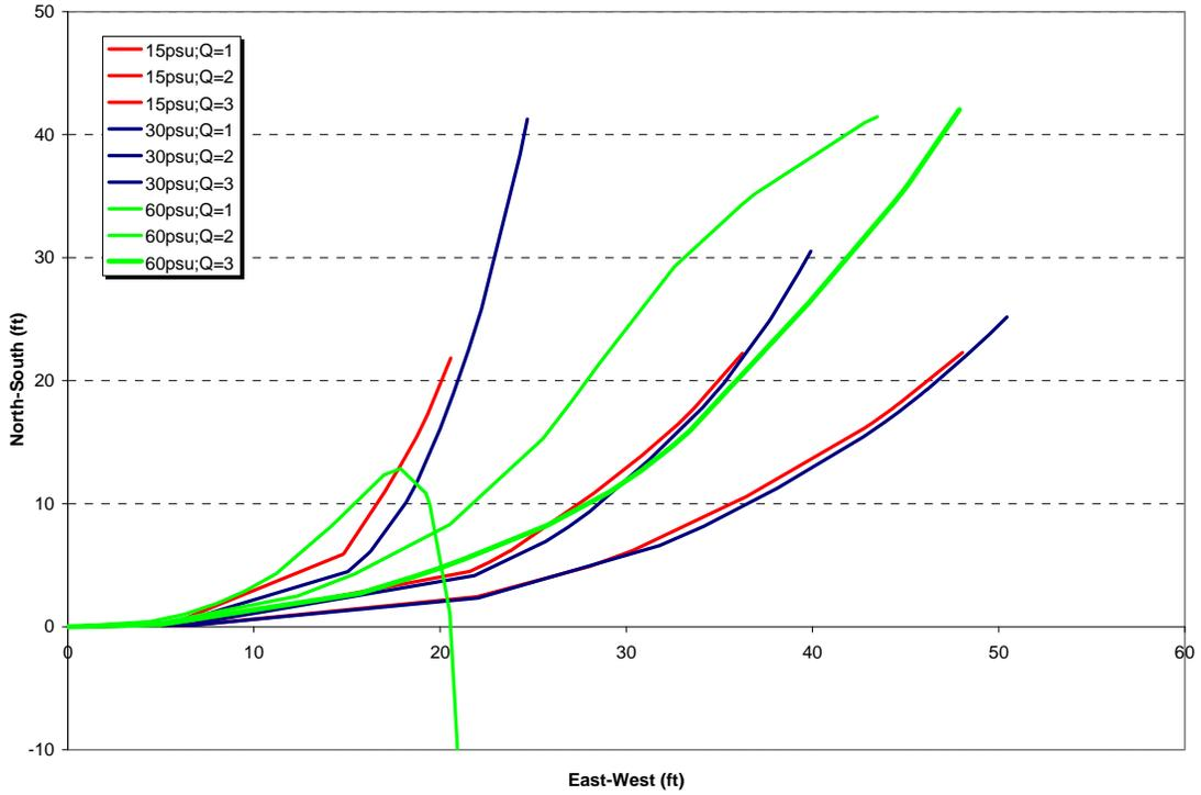
Figure 21. Plan view of plume trajectory for selected cases to illustrate the sensitivity of dilution to discharge salinity
