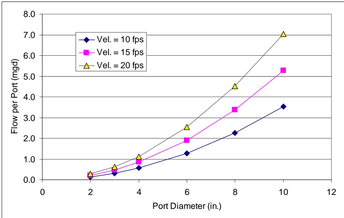
Figure 10. Flow through a port of given diameter with three velocities (10, 15, and 20 fps)
