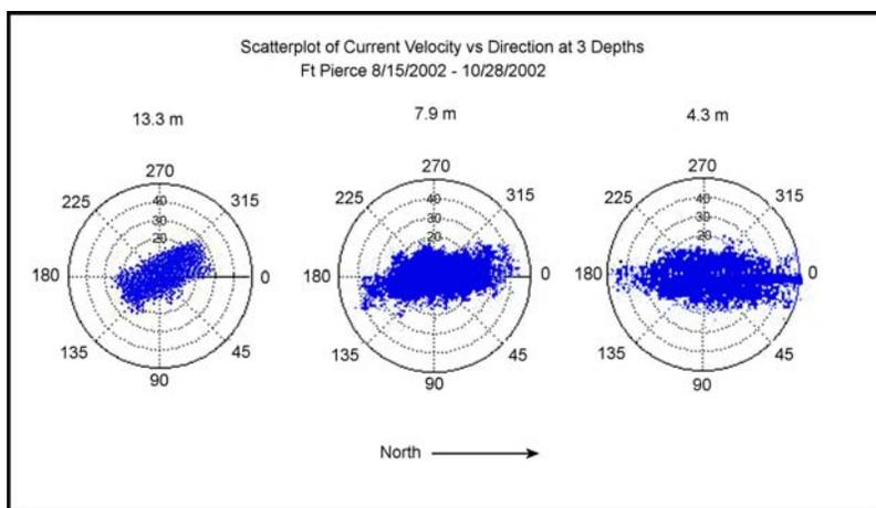
Figure 4. Current velocity and direction data at three depths for a site offshore of Ft. Pierce Inlet, August to October 2002 (Data Source: AOML, in CH2M HILL 2005) (Note: Current velocity scale ranges from 0 to 50 mm/sec.)
