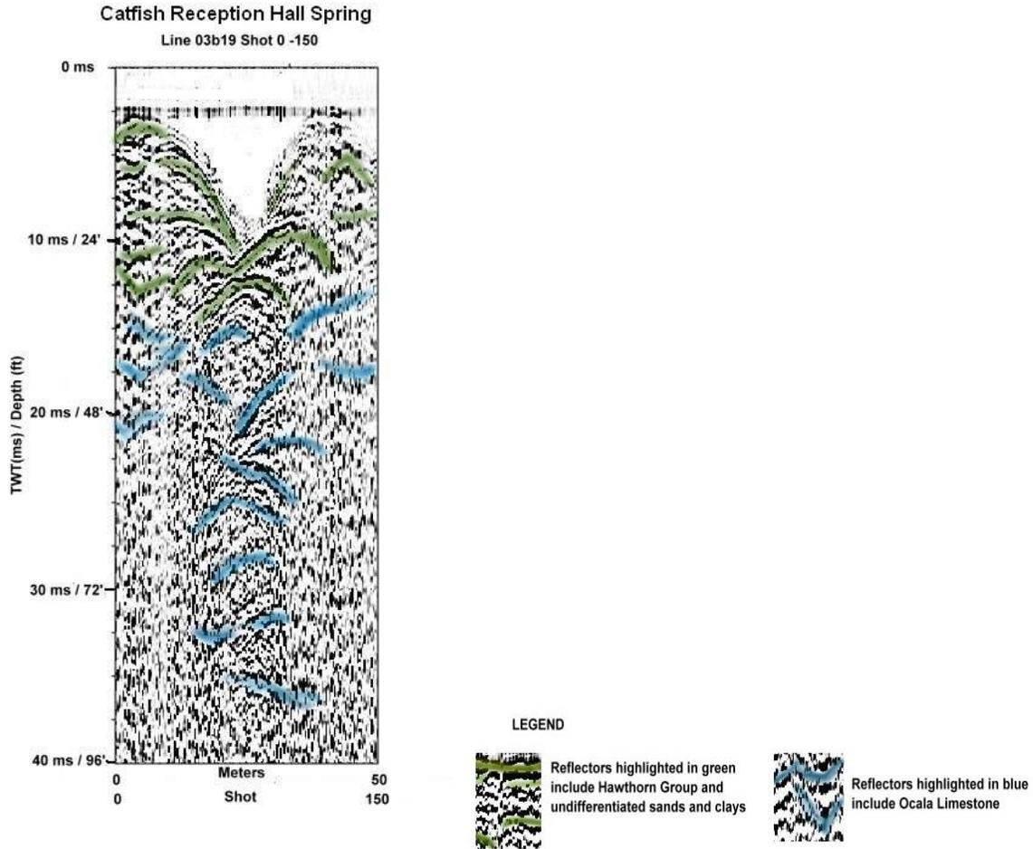
**Figure 5-20** Seismic profile Line 03b19 shot 0 to shot 150 within section B-B' by Catfish Reception Hall Spring. Location of profile is shown in Figure 5-19. Highlighted reflectors indicate the subsurface orientation of individual beds. The central region is highly deformed, suggesting collapse into a void.
