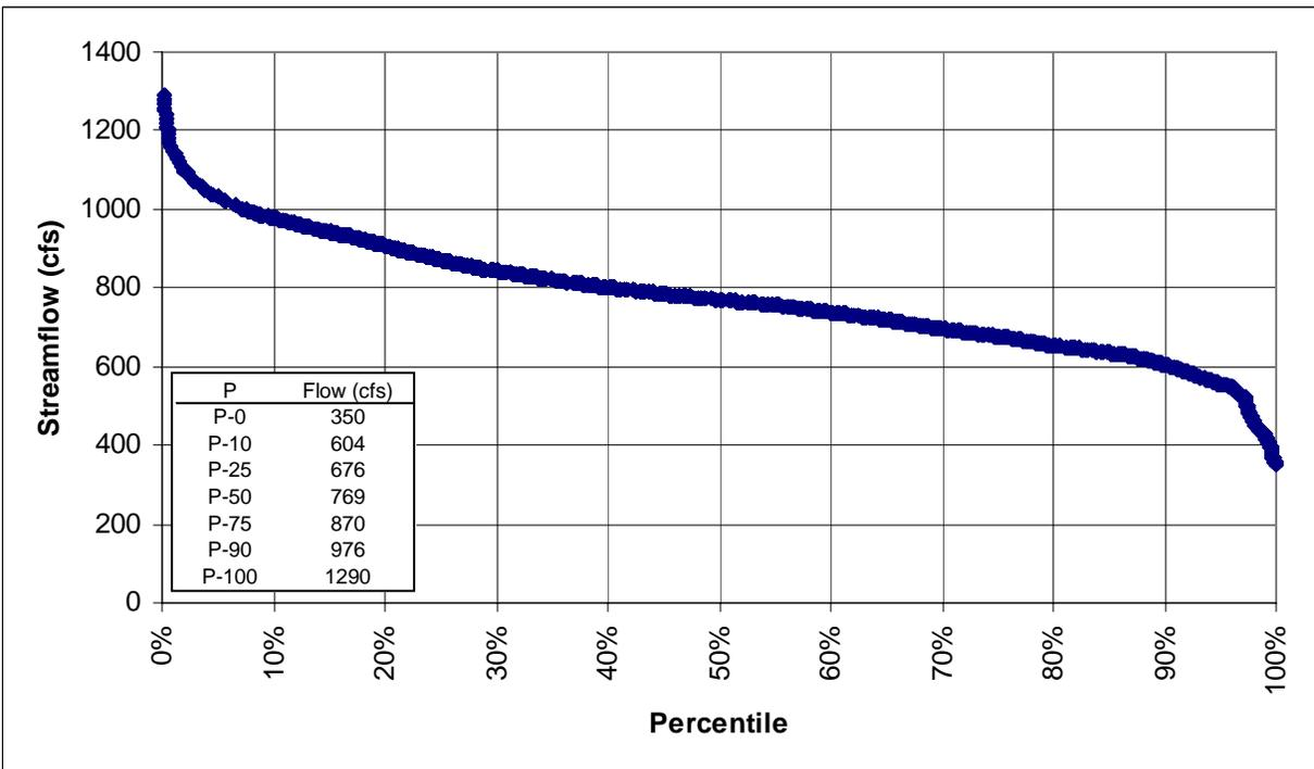
Figure 3-4 Silver Springs USGS 02239500 streamflow (1932 – 2005) (Note: 10/03 – 2/05 preliminary data)
