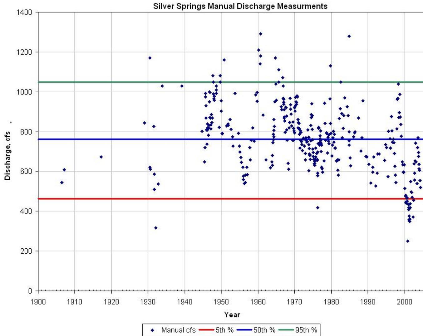
Figure 2-22 Silver Springs Manual Discharge Measurements (from USGS data)
