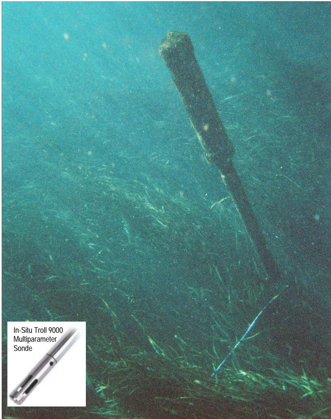
**Figure 4-14** WSI's In-Situ Troll 9000 recording datasonde installation at the 1,200-m station in Silver Springs.
