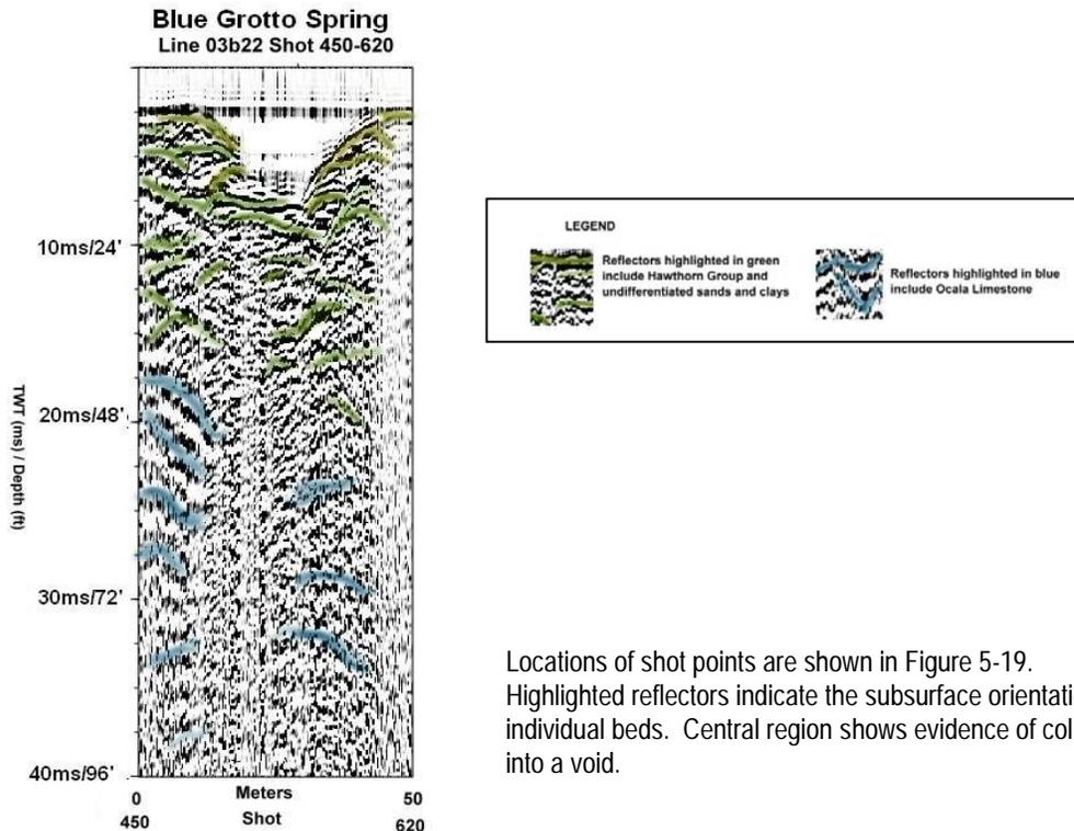
**Figure 5-22** Seismic profile Line 03b22 shot 450 to shot 620 within section B-B' showing the profile of Blue Grotto Spring.
