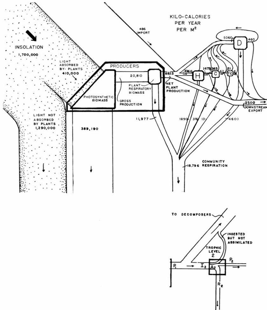
Figure 2-27 Energy flow diagram with estimates of energy flows in kilo-calories per square meter per year in the Silver Springs community (Odum 1957)
