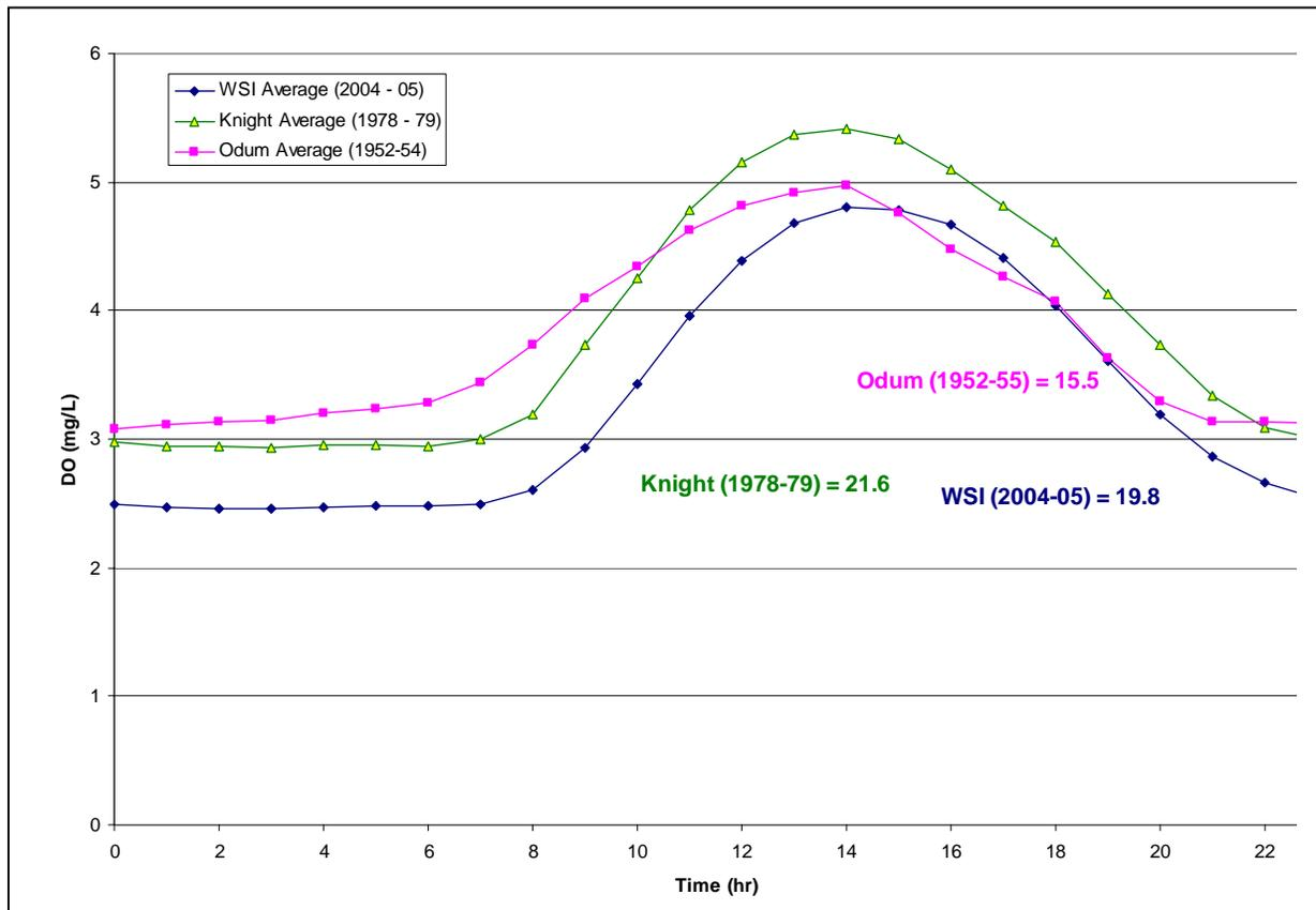
**Figure ES-5** Comparison of Silver Springs average diurnal oxygen curves at the 1,200-m station; estimated gross primary productivity in units of ppm-hrs. Higher total GPP estimates for [Knight \(1978-79\)](#) and [WSI \(2004-05\)](#) are a result of increased submerged area in Silver Springs Run above the 1,200-m station due to the addition of the Back Channel Extension in the late 1970s.
