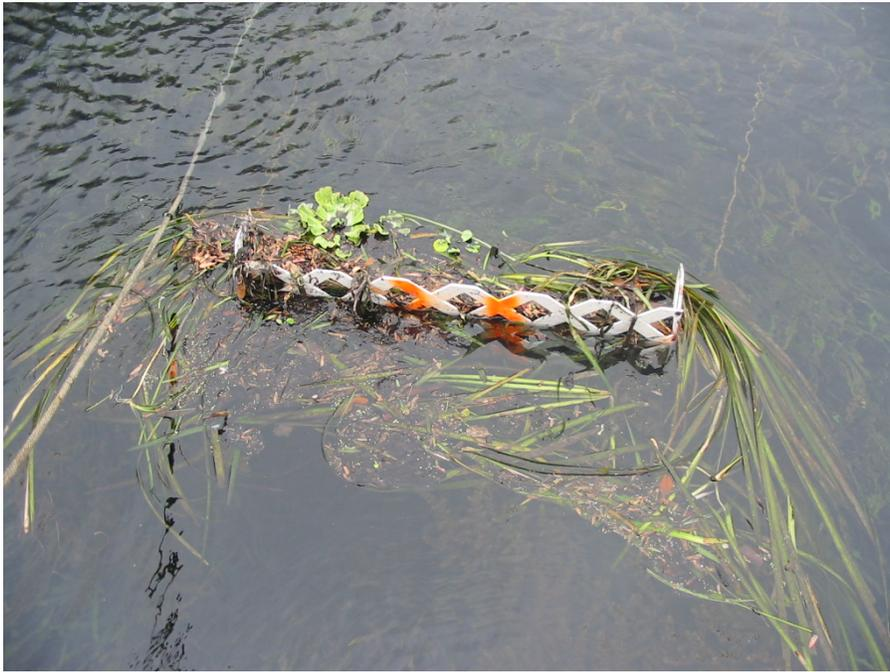
**Figure 4-16** Typical plant export trap deployed in the Silver River.
