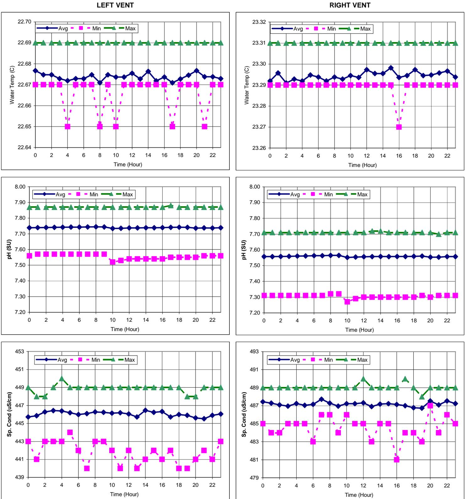
Figure 3-2 Diurnal summary of field parameters measured hourly for twenty-one days at two discrete vents in Silver Springs Main Spring Boil during May 1997
