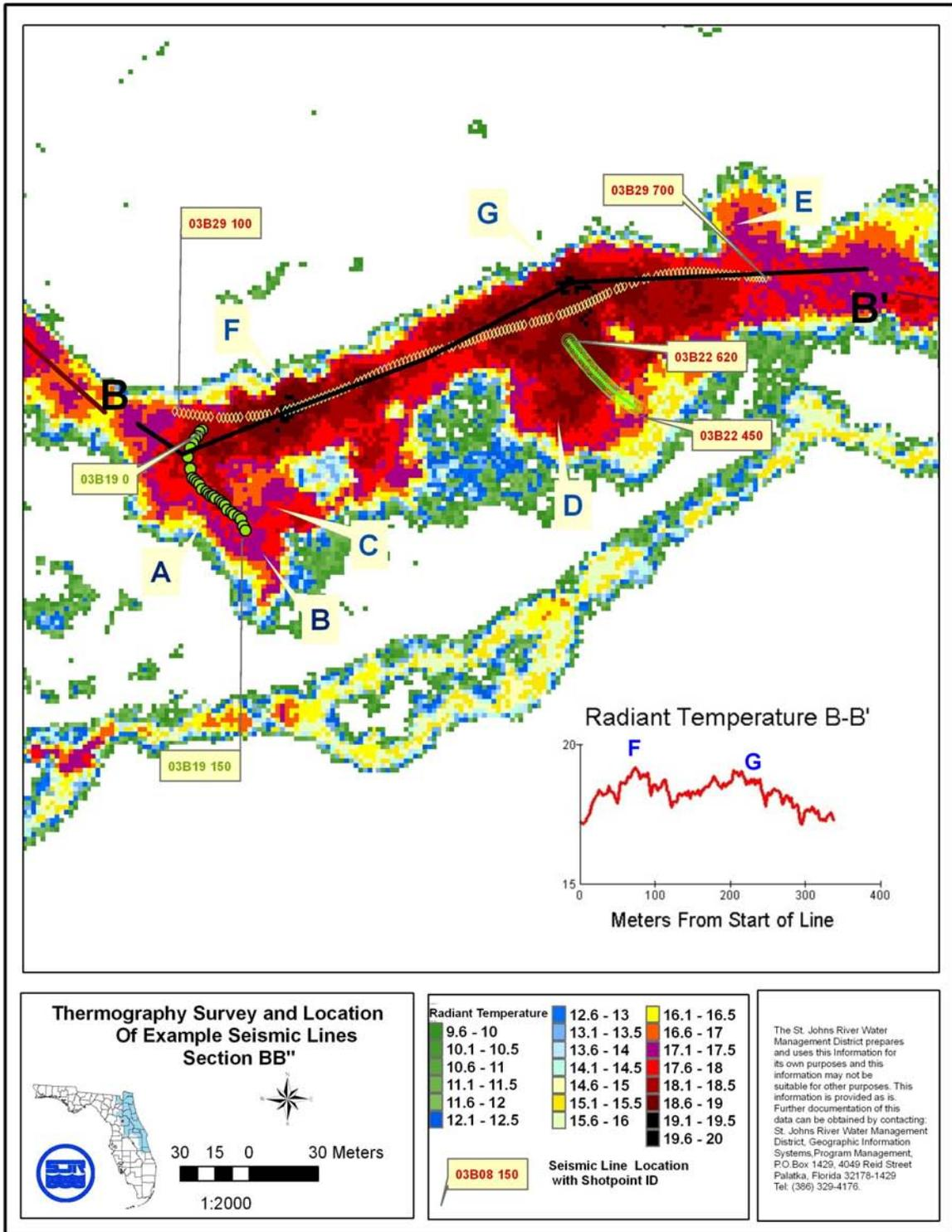
Figure 5-19 Thermography survey and location of example seismic lines, section B-B'
