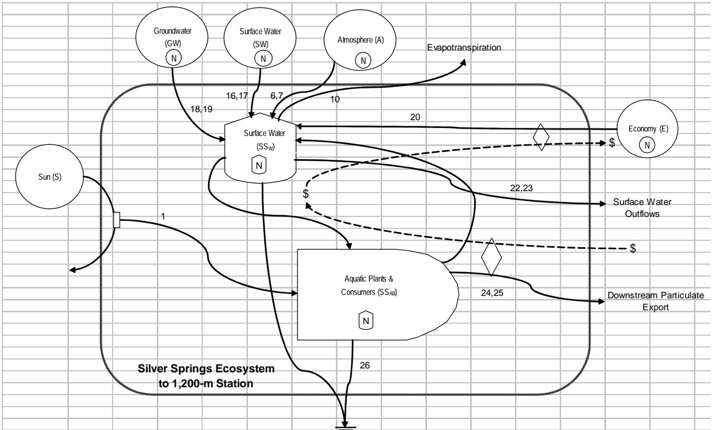
Figure 4-11 Silver Springs ecosystem model (Main Spring Boil to 1,200-m Station)
