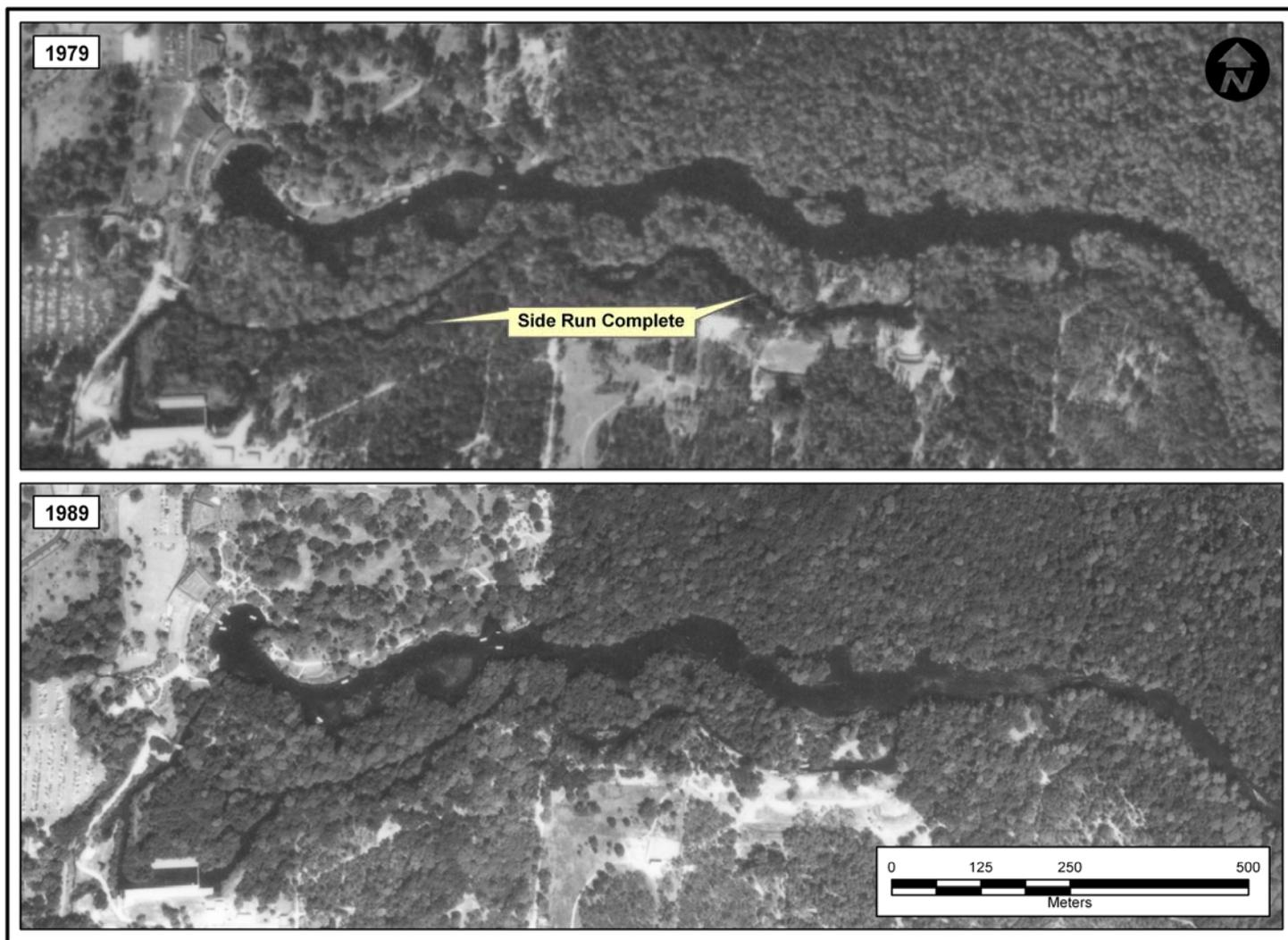
**Figure 2-20** Spring Run Area Changes 1979 – 1989 – Side Run (Back Channel) Completed Between 1972 and 1979
