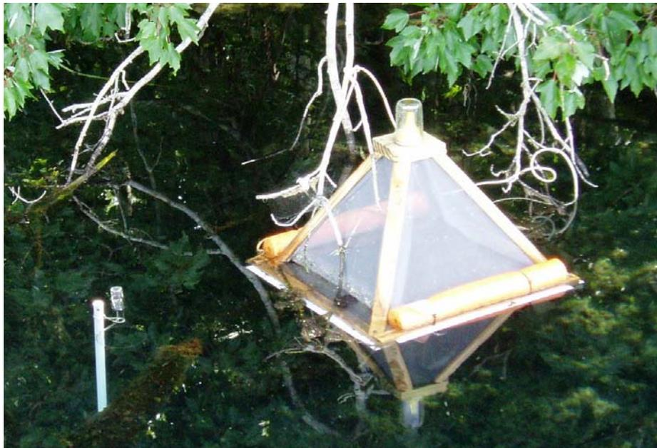
**Figure 4-17** Typical pyramidal insect emergence trap and inverted glass funnel deployed at Silver Springs
