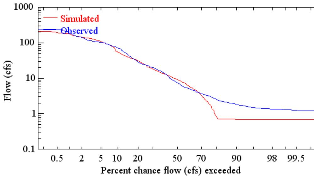
Figure B.18. Observed and simulated daily flow frequency curves for Howell Creek near Slavia (10/1997 – 09/1999).
