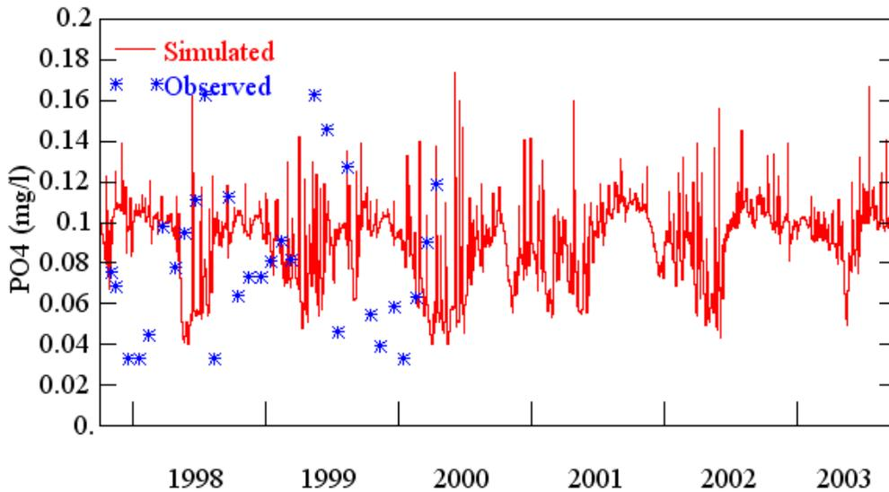
Figure C.6. Observed and simulated PO<sub>4</sub> concentrations for Howell Creek near Oviedo (10/1997 – 09/2003).
