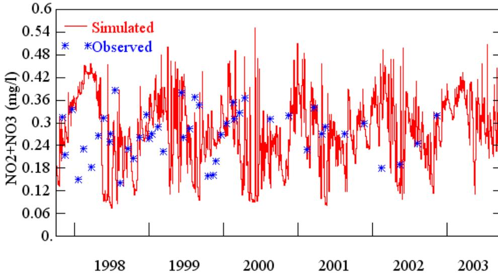
Figure C.5. Observed and simulated NO<sub>2</sub>+NO<sub>3</sub> concentrations for Howell Creek near Oviedo (10/1997 – 09/2003).
