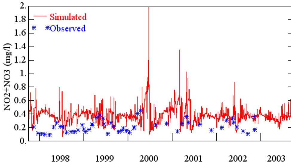
Figure C.19. Observed and simulated NO<sub>2</sub>+NO<sub>3</sub> concentrations for Soldier Creek near Longwood (10/1997 – 09/2003).
