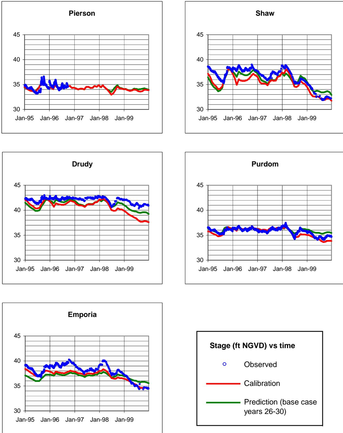
**Figure 62. Comparison of Calibration Results to Predictive Results, Lake Stage**
