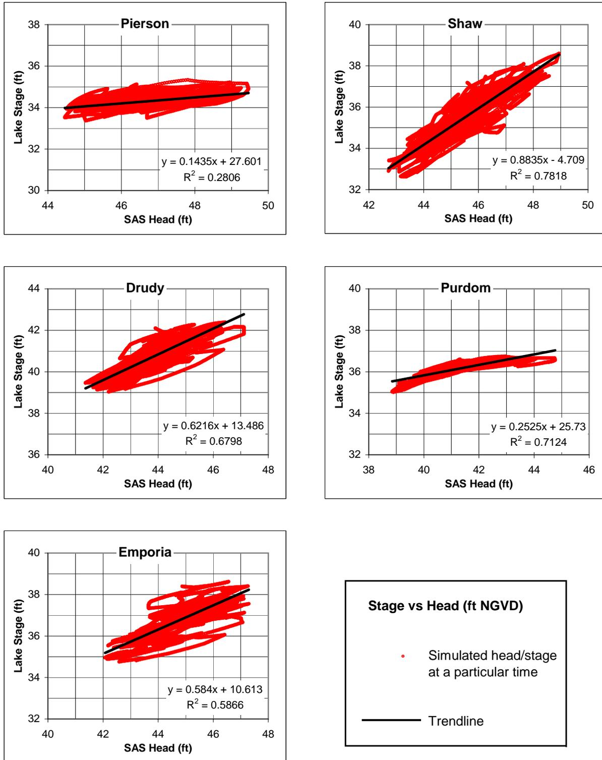
Figure 65. Correlation between Simulated Lake Stage and Simulated SAS Head
