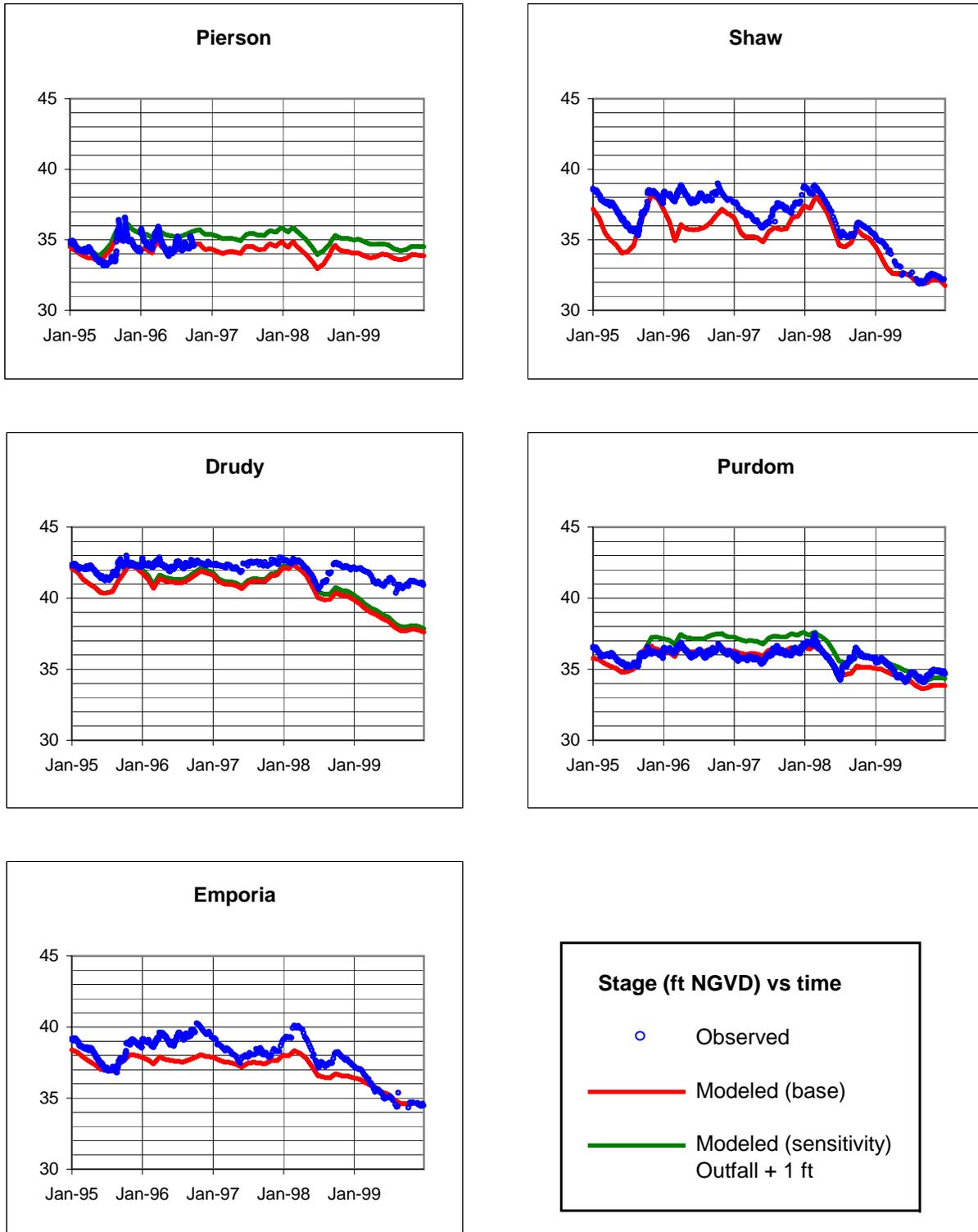
Figure 51. Sensitivity of Lake Levels to Increased Outfall Elevations
