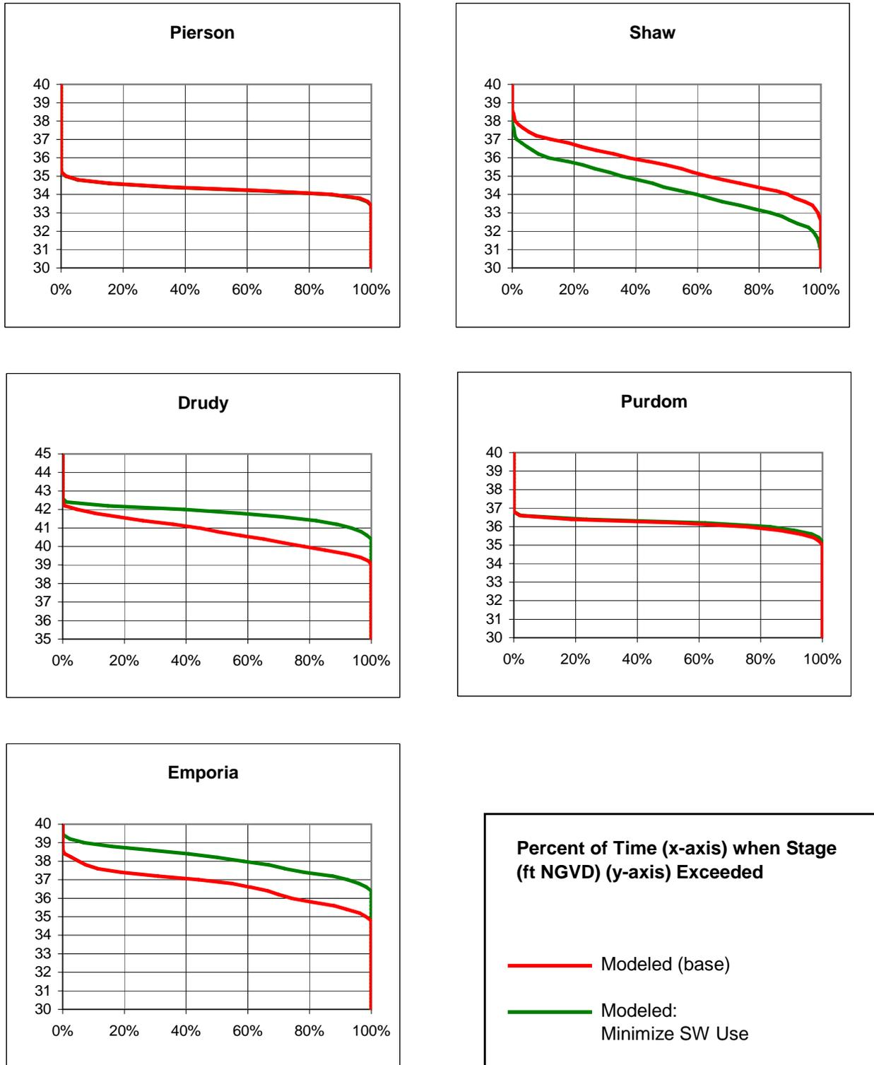
Figure 71. Simulated Stage-Duration Curves for the Minimized Surface-Water Use Scenario
