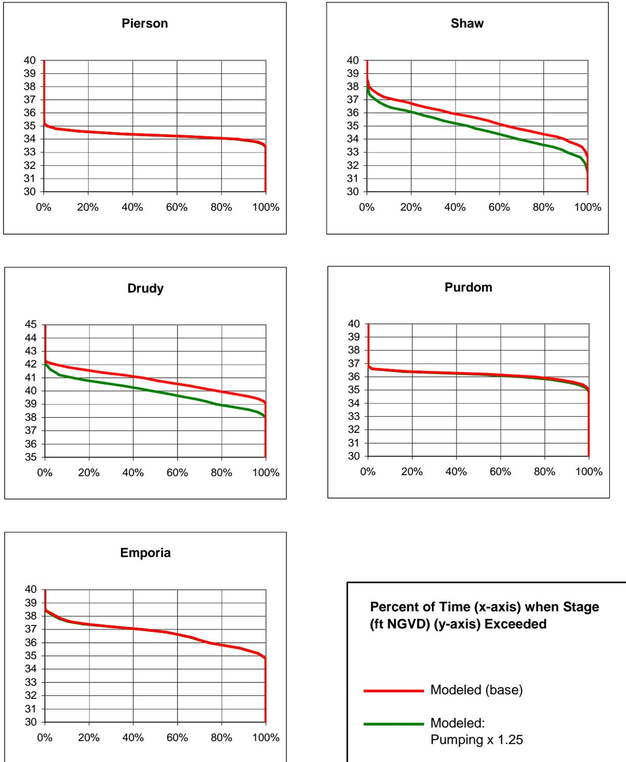
Figure 66. Simulated Stage-Duration Curves for the Increased Pumping Scenario
