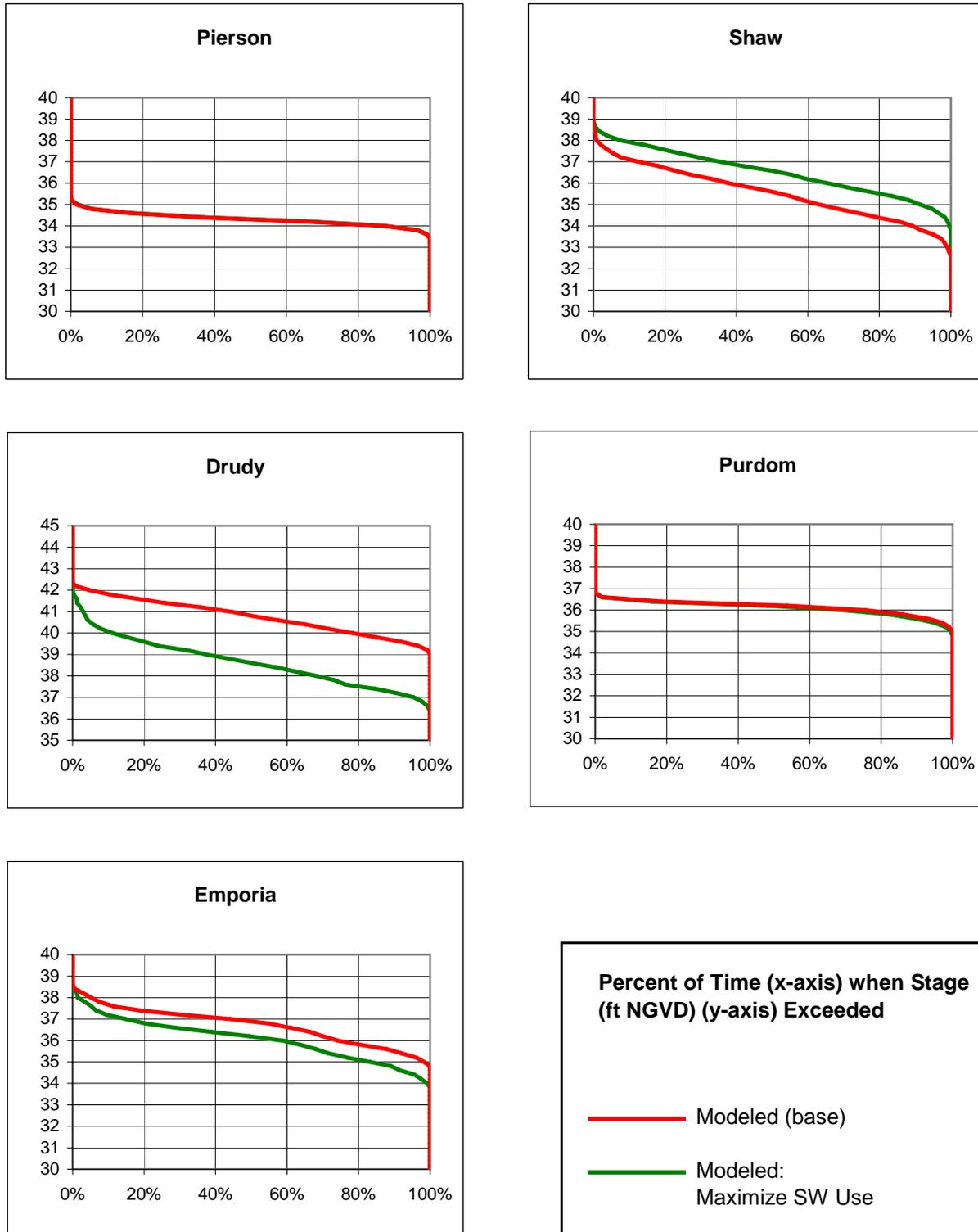
Figure 70. Simulated Stage-Duration Curves for the Maximized Surface-Water Use Scenario
