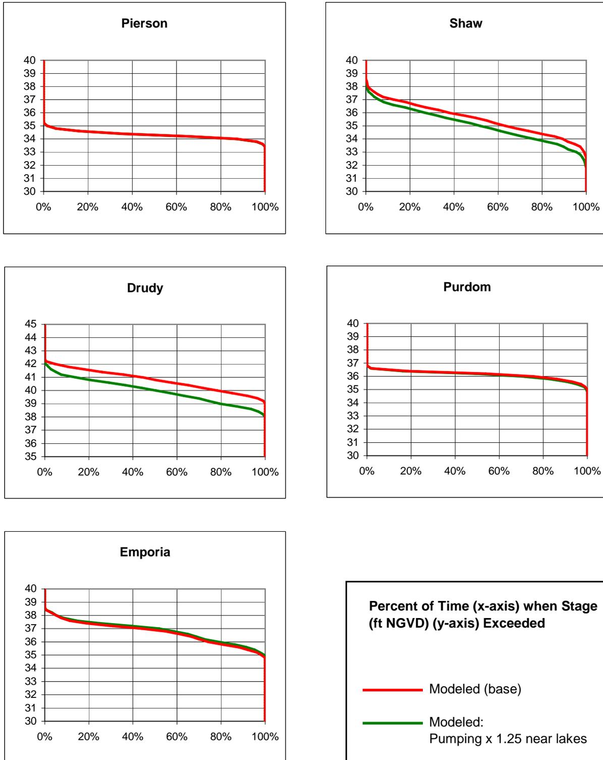
**Figure 68. Simulated Stage-Duration Curves for the Increased Pumping (near Lakes Only) Scenario**
