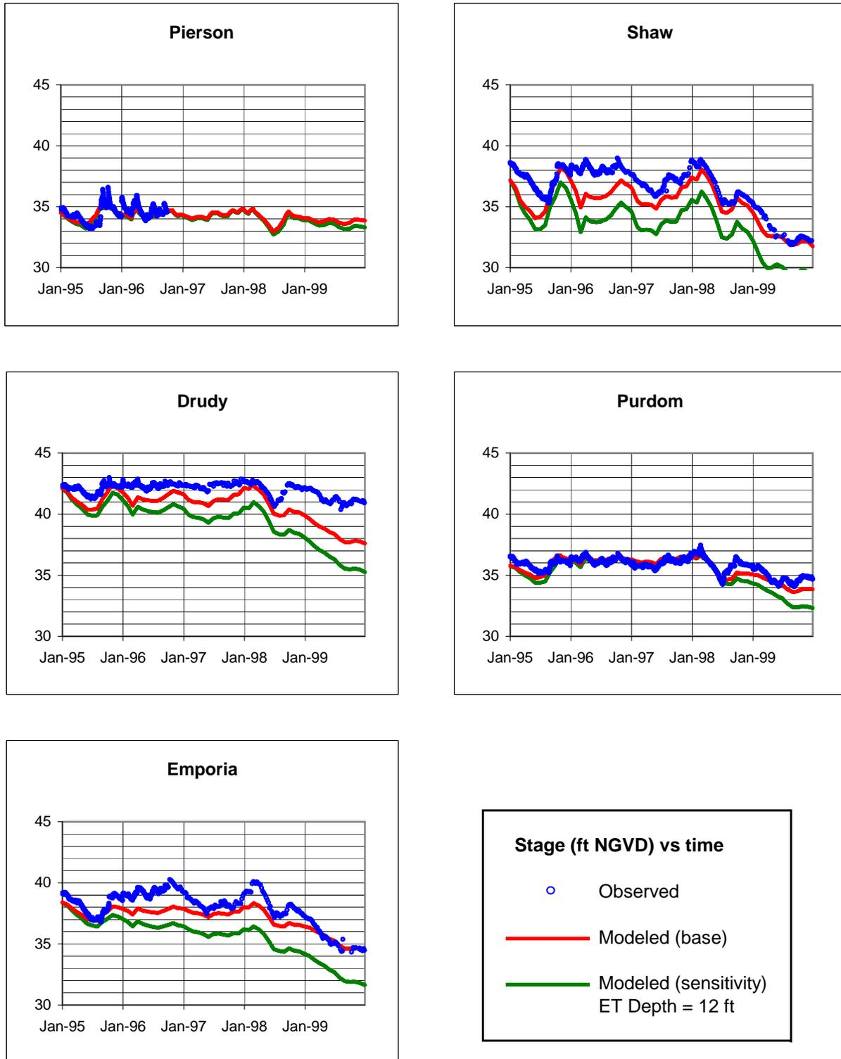
Figure 46. Sensitivity of Lake Levels to Increased ET Extinction Depth
