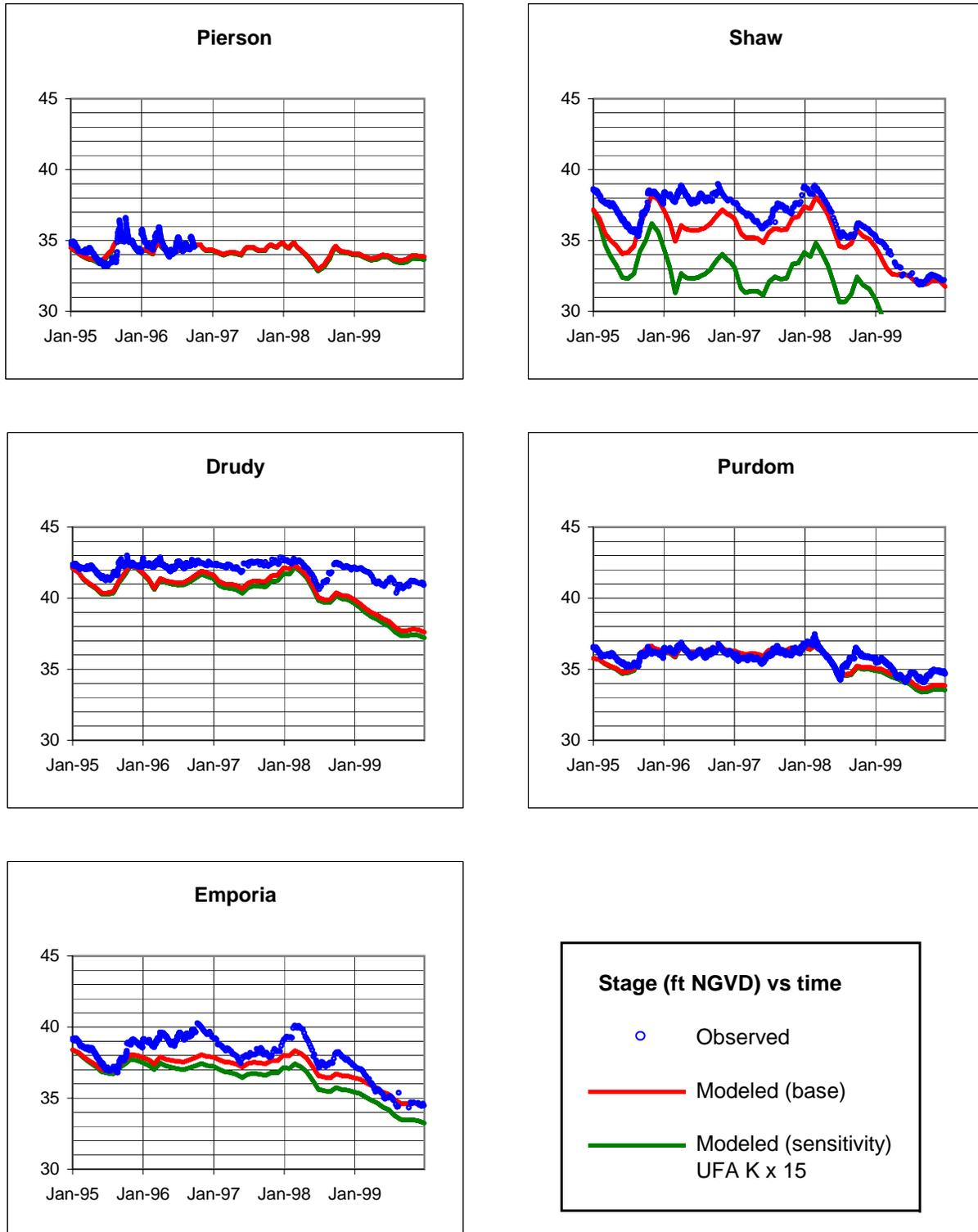
Figure 43. Sensitivity of Lake Levels to Increased UFA Hydraulic Conductivity
