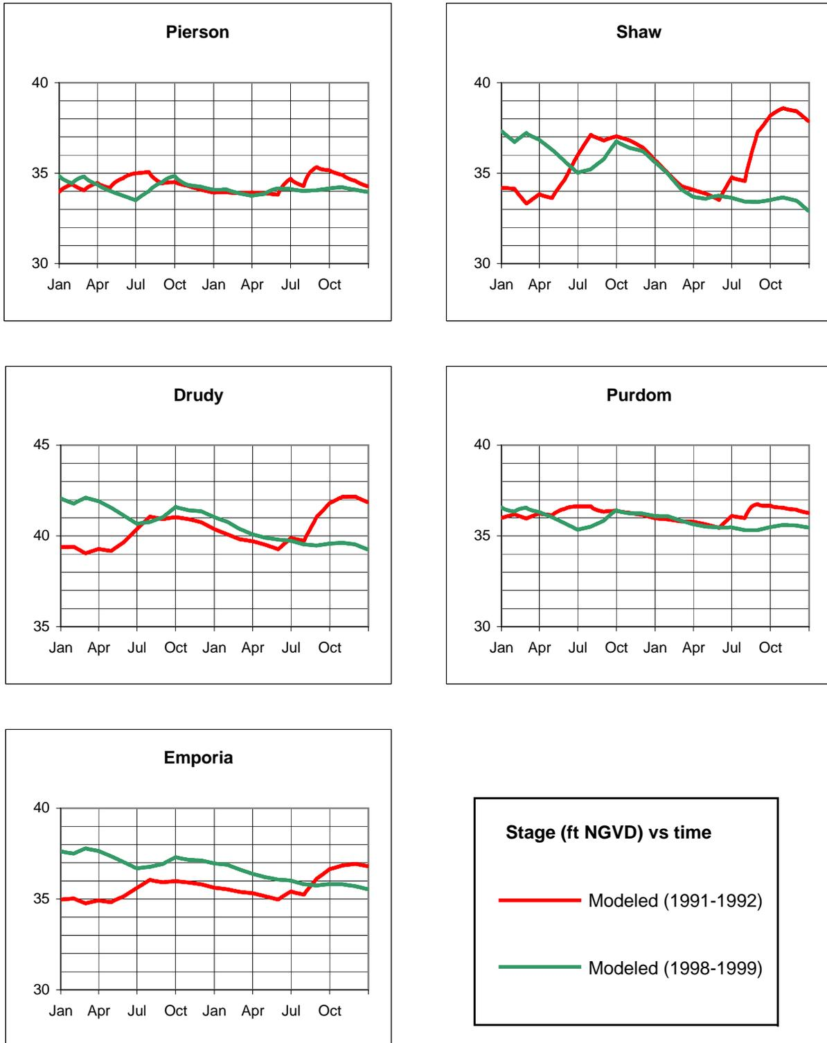
Figure 64. Simulated Lake Levels during Periods of Extreme Wet and Dry Conditions
