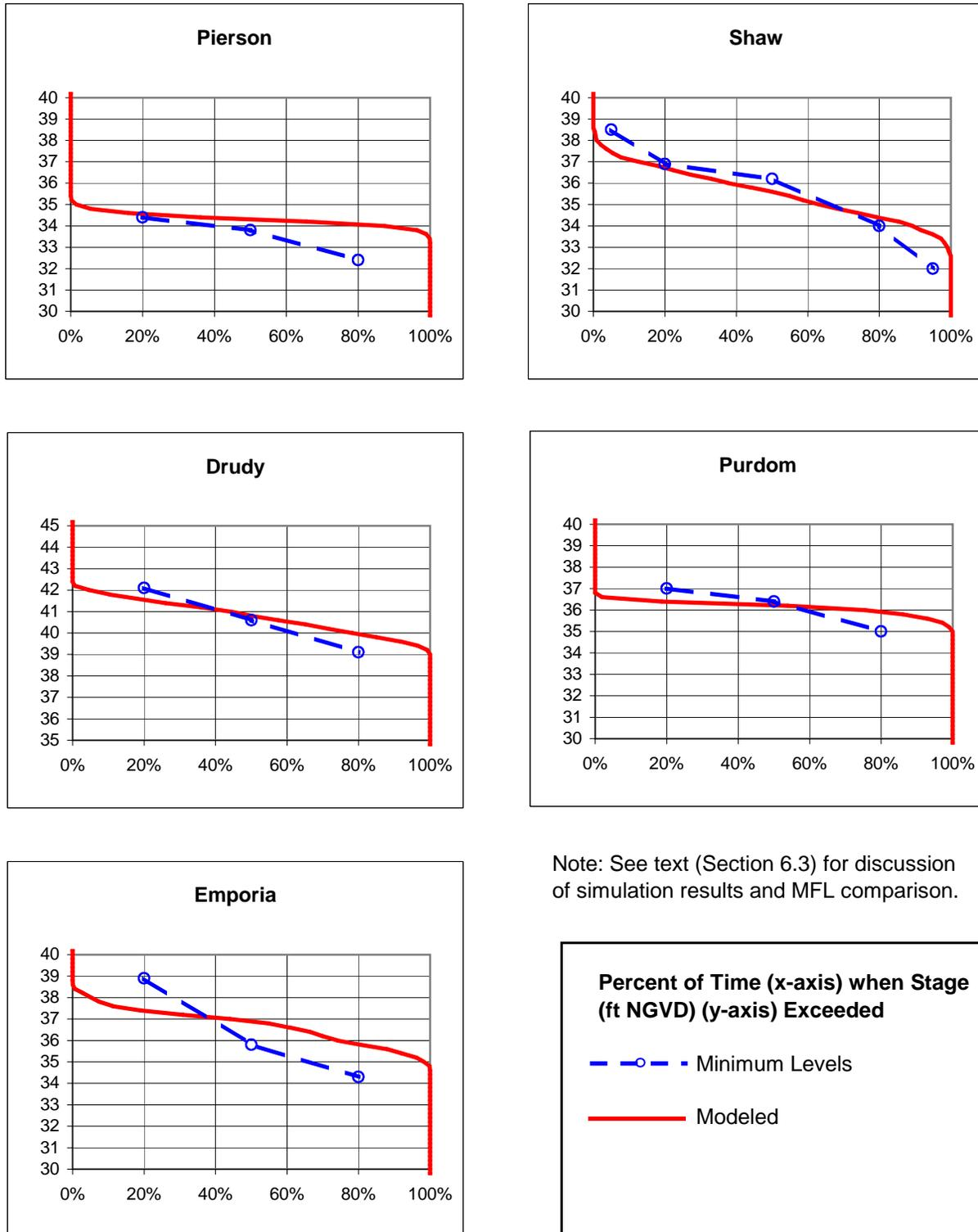
Figure 63. Simulated Stage-Duration Curves for the Base Case Scenario
