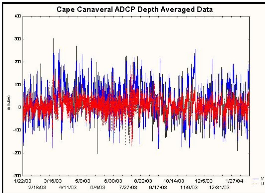
The time series data depicted in Figure 5 can be used to depict the velocity-frequency relationships needed to support ocean outfall mixing zone modeling. Histograms of the North-South (V) and East-West (U) current components are presented in Figures 6 and 7, respectively. The mean for the V and U components are approximately 3 cm/sec and 0.8 cm/sec, respectively.
