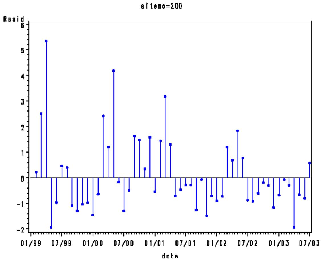
Figure 30 Plot of the residuals for site 200 over the reduced period for which site-specific rainfall is available. The trend in residuals does not seem to be very different after adjusting for rainfall effects. The reduction in extreme irrigation pumpage over time could be due to a number of factors. Physical factors, such as a change from furrow to micro-jet irrigation methodologies or simply changes in management philosophy could explain this pattern.
