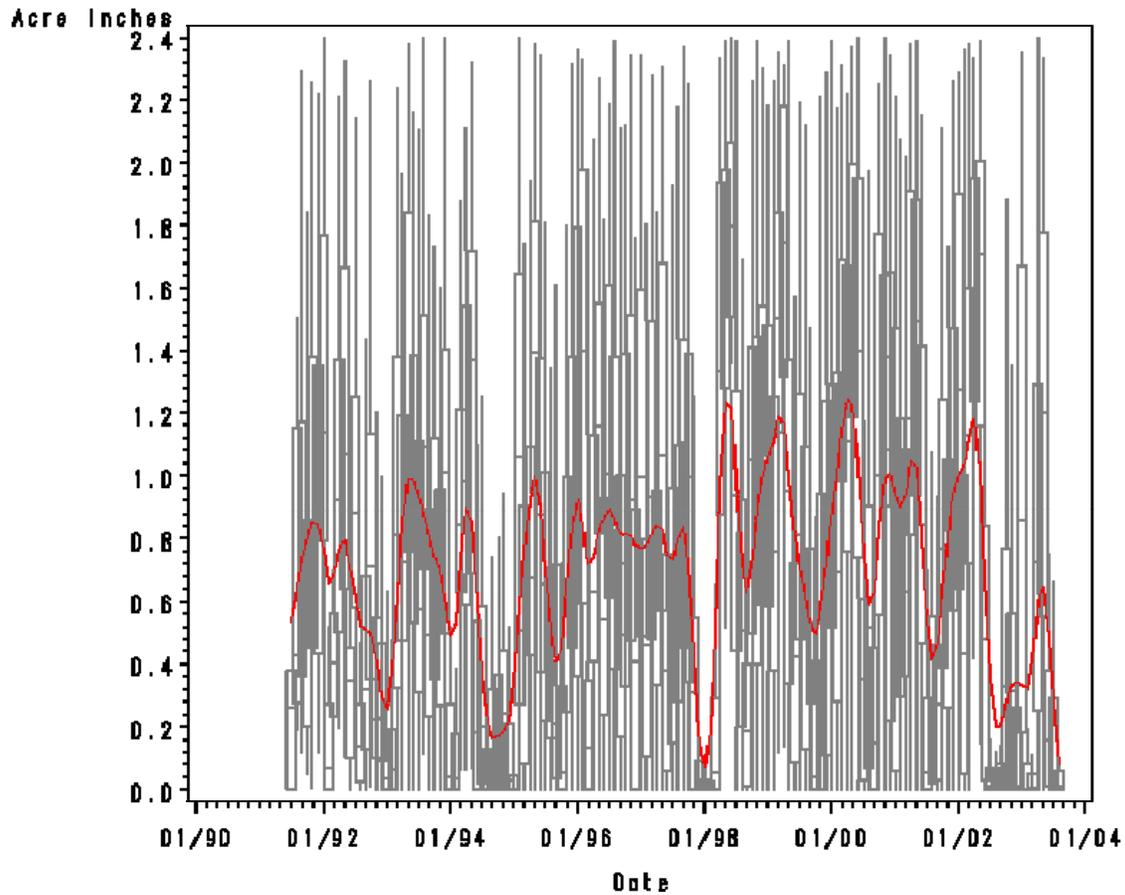
**Figure 13 Monthly acre-inches distributions for ridge citrus for the entire monitoring period with the average monthly mean estimates connected by a smoothed curve. Monthly patterns are very evident with year differences more difficult to see. The objective of the analysis is to decompose the variability seen here into site, year, month and residual effects. The scale of the vertical axis is in acre-inches.**
