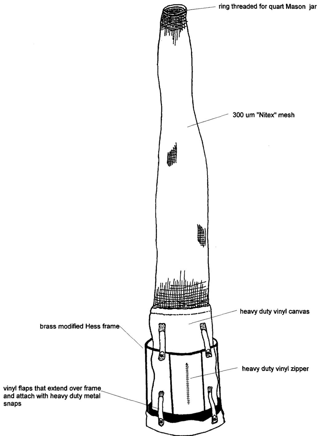
FIGURE 2. Depiction of modified Hess stream sampler used for sampling invertebrate communities associated with Nuphar luteum in Blue Cypress Lake. Sampler frame diameter = 34 cm; frame height = 36 cm; total height = 185 cm; mesh size = 300 microns.
