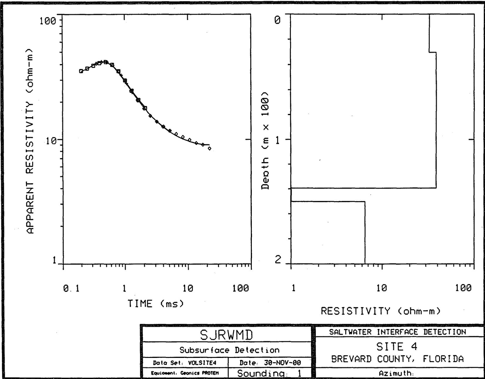
Figure 5.5-1 Measured TDEM Apparent Resistivity and 1-D Inversion - Site 4
