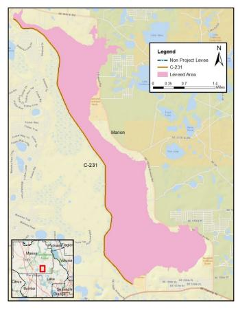
to overtop the levee in a storm that has a 1 in 500 chance of occurring in any given year. If the levee breaches or overtops, the range of flooding in portions of the leveed area could be up to 13 feet deep.
