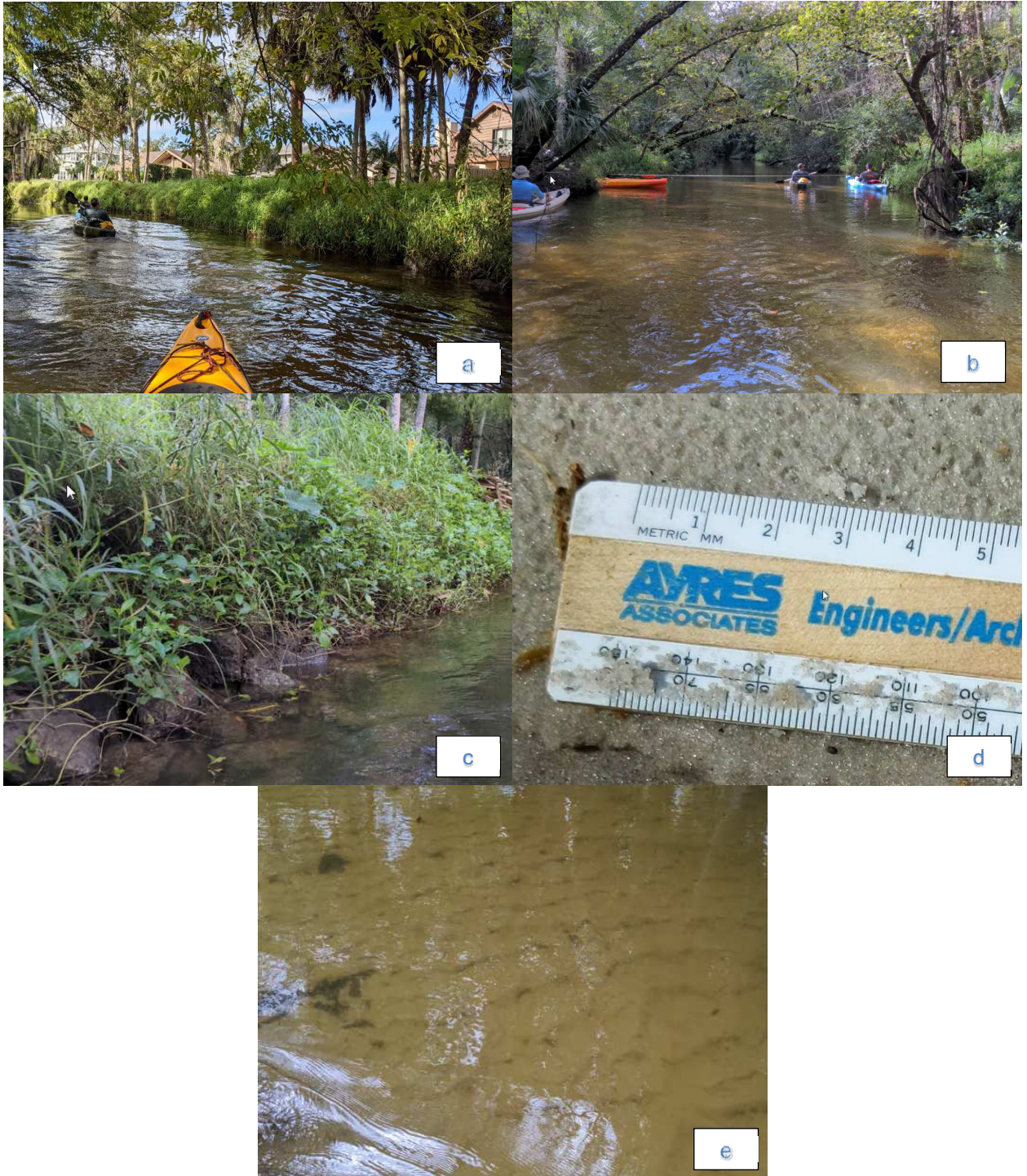
Figure 4: (a) Tall and steep bank slopes; (b) Sign of lateral instability shown by leaning trees into channel; (c) Riprap placed along banks of channel; (d) Representative sediment size shown; (e) Ripple bedforms shown.
