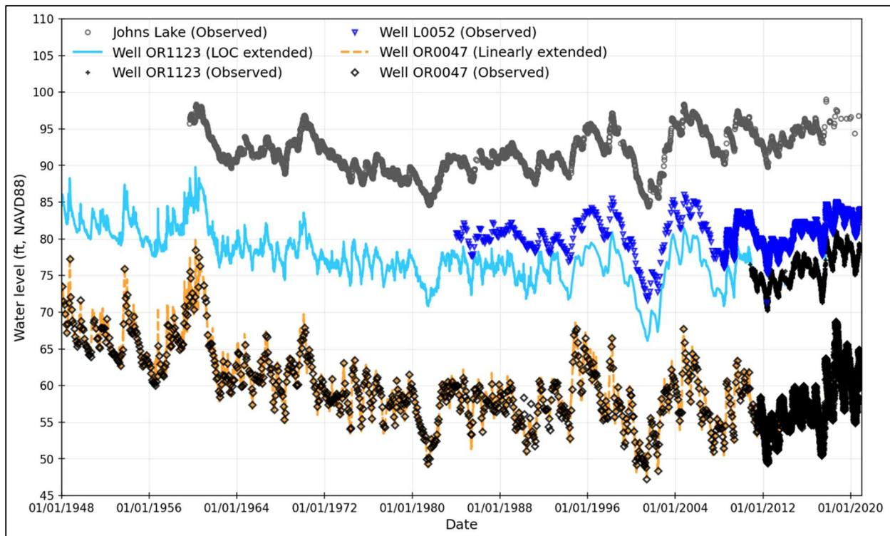
Figure B-6: Observed and extended groundwater levels along with observed water levels of Johns Lake (LOC = Line of Organic Correlation).
