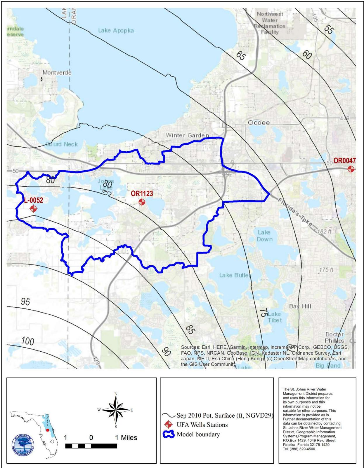
Figure B-5: Groundwater monitoring stations along with the representative September 2010 potentiometric surface contours.
