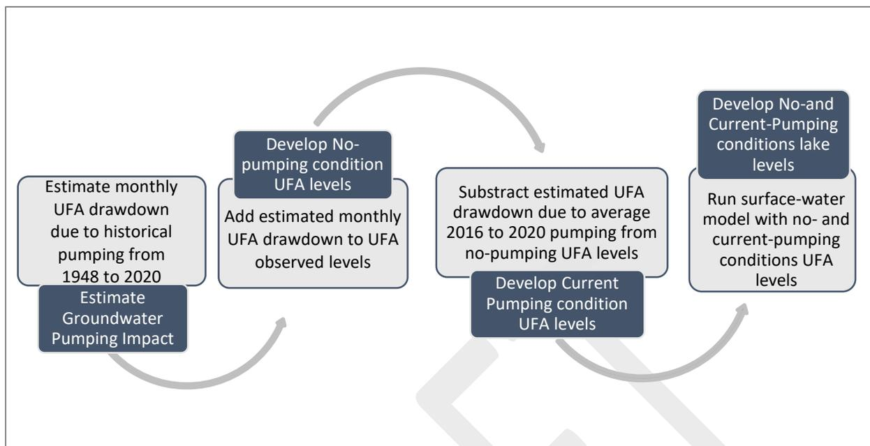
Figure B-9: Steps for developing no-pumping and current-pumping condition lake levels
