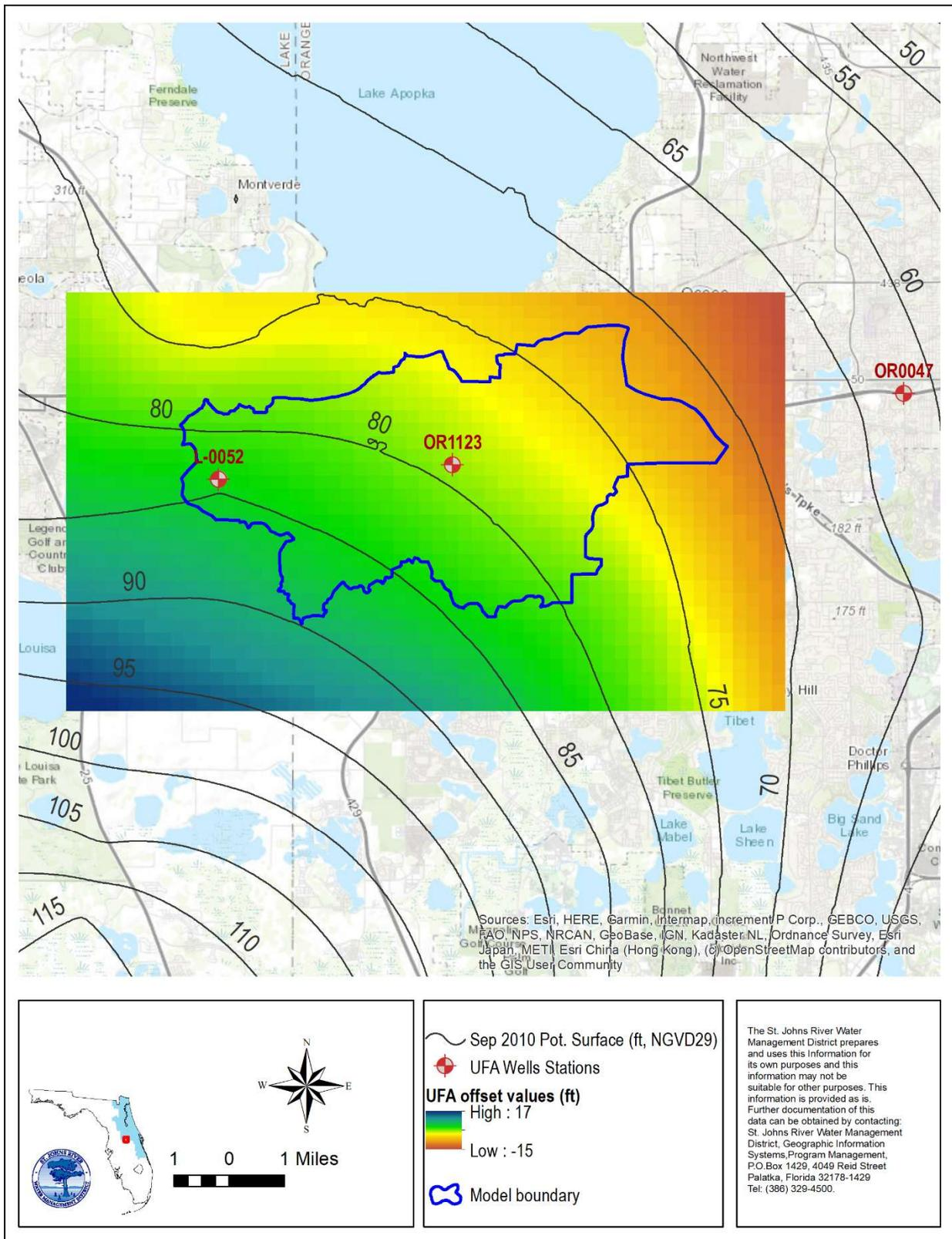
Figure B-7: Annual average offset values with respect to OR1123 as derived from May and September potentiometric levels from 1978 to 2017.
