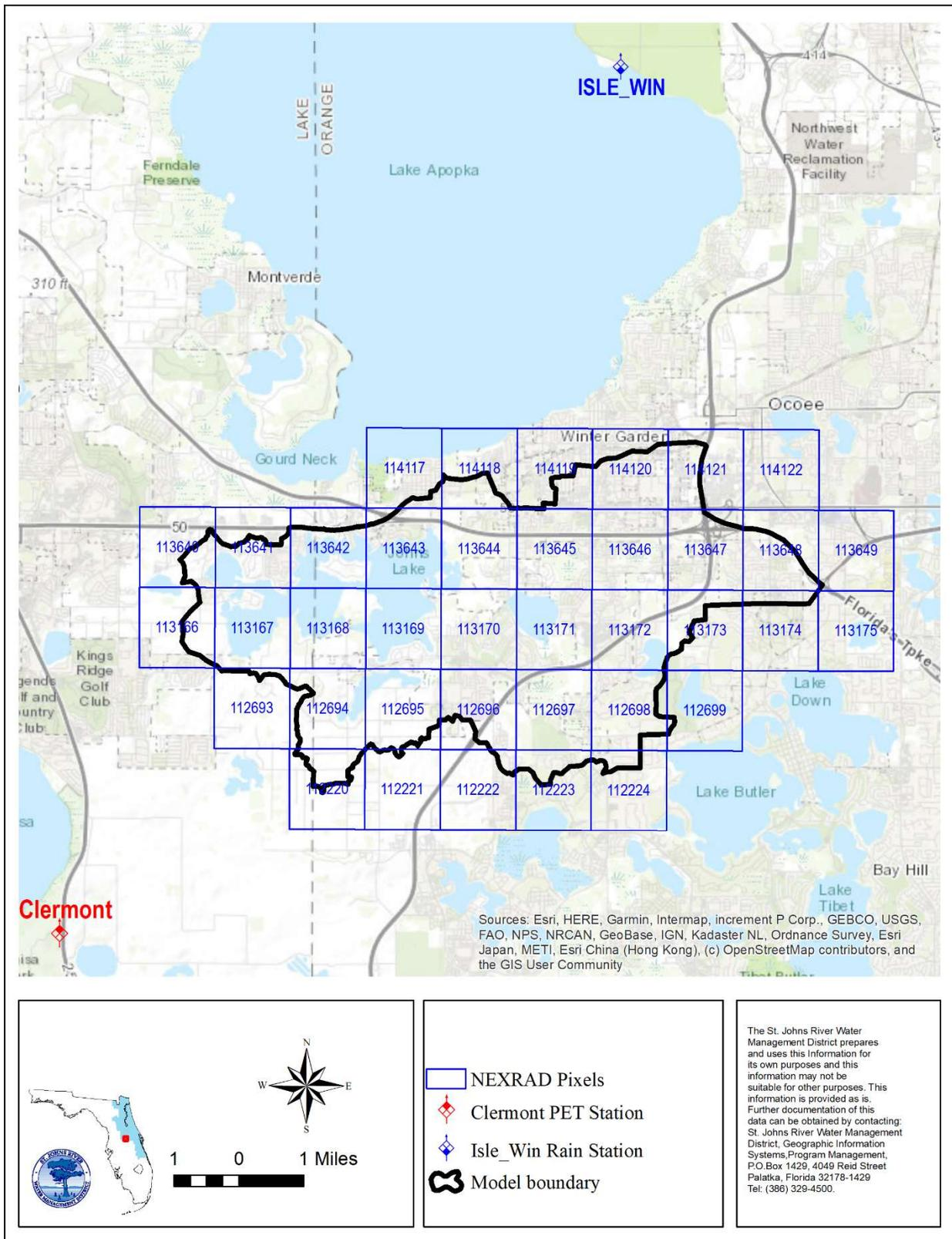
Figure B-3: NEXRAD pixel identifications and hydro-meteorological stations of Johns Lake.
