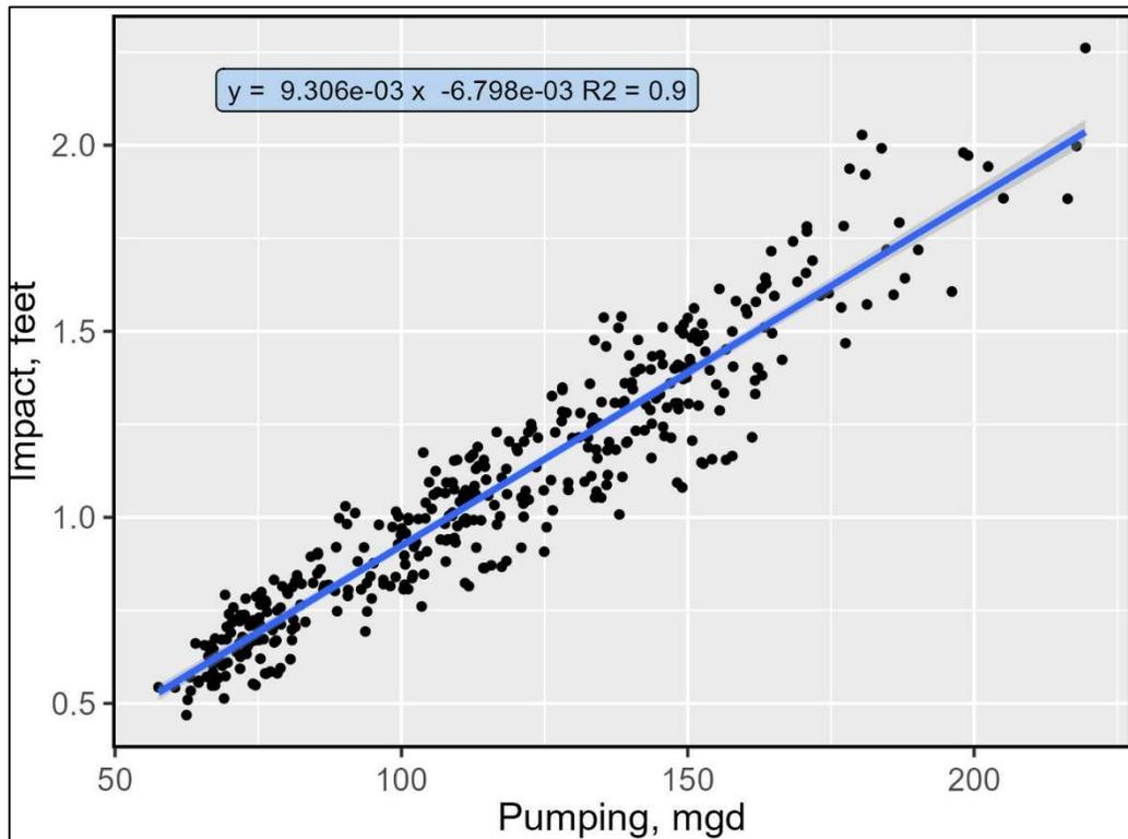
Figure B-11: Linear regression between UFA drawdown near Johns Lake and groundwater pumping within 15-mile buffer area. “mgd” represents a million gallons per day.
