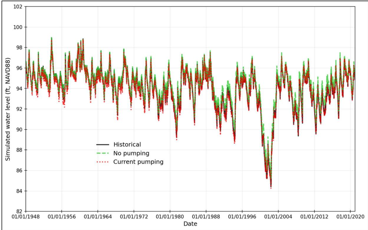
Figure B-15: The simulated historical, no-pumping, and current-pumping condition levels for Johns Lake.
