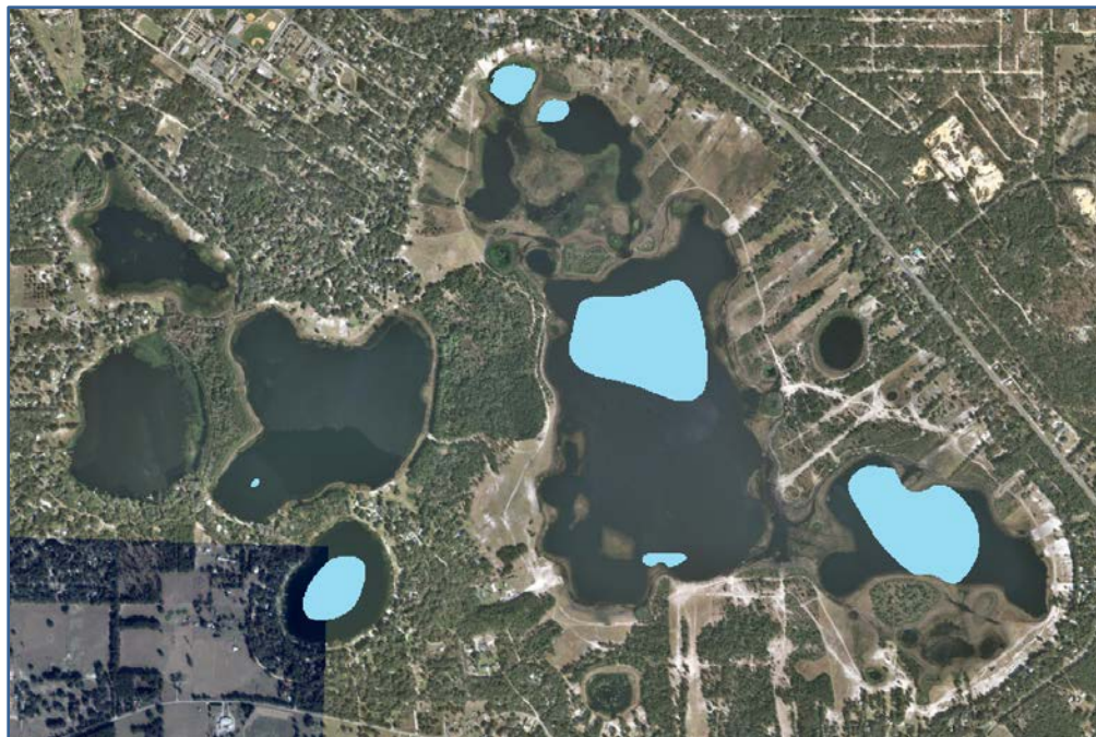
Figure 17. Aerial photo of Lake Geneva with hydroperiod tool output data showing minimum water level based on minimum ski corridor elevation (81.0 ft NAVD88).
