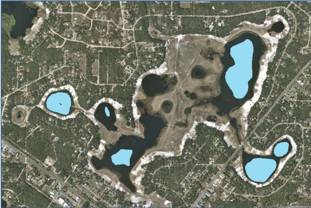
Figure 16. Aerial photo of Lake Brooklyn with hydroperiod tool output data showing water level based on minimum ski corridor elevation (86.5 ft NAVD88).
