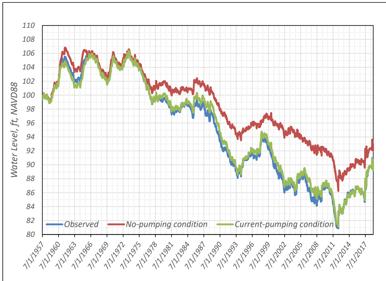
Figure B-25. The estimated no-pumping and current-pumping condition levels for Lake Geneva
