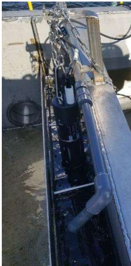
EXO2 water quality sonde in the influent port chamber
