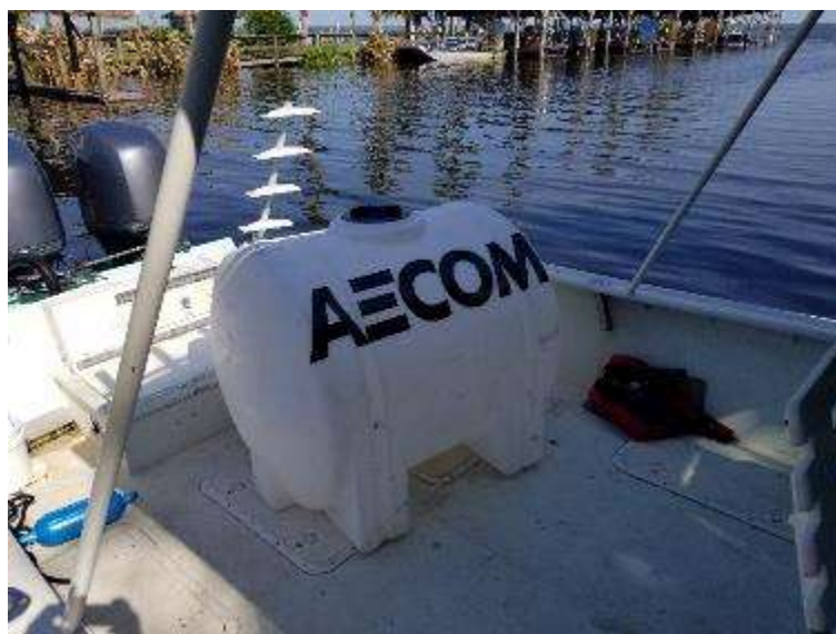
Poly-tank on work boat to transfer slurry from the barge to the shoreside storage tank.
