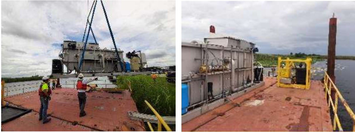
Loading of the algae harvester onto the barge (left) and moving the barge to Barge Station 1 using a push boat partially visible behind the yellow frame of the spud winch (right).
