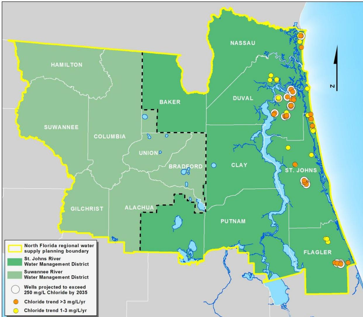
Figure 17: Wells with Increasing Trends in Chloride Concentration
