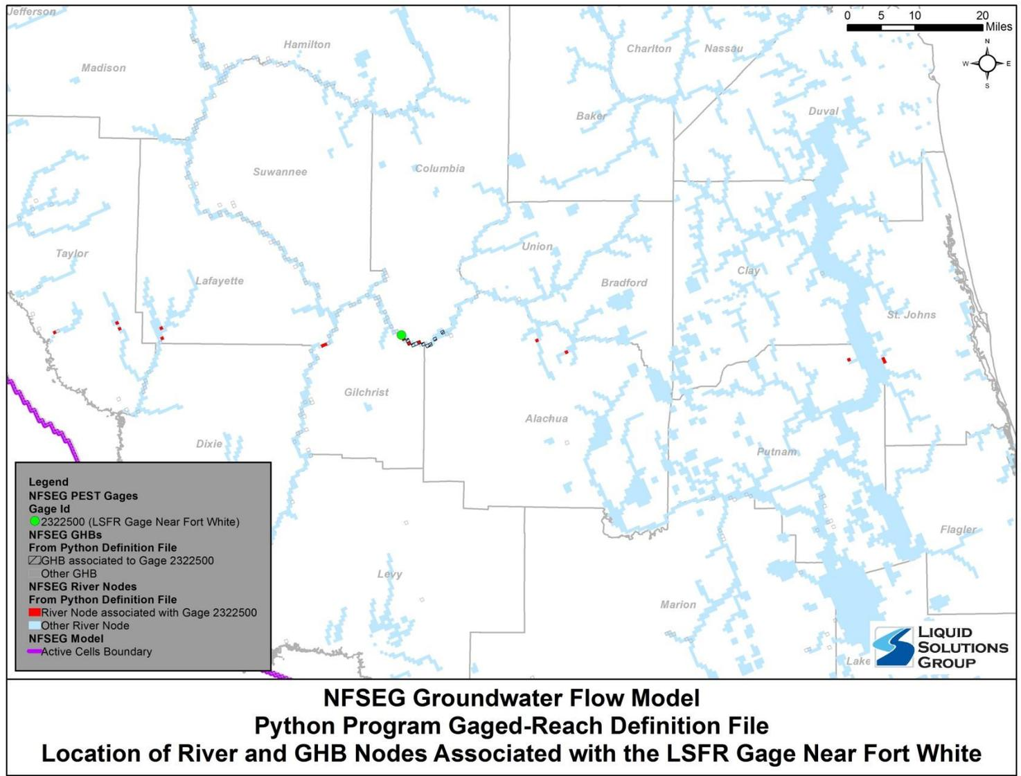
**Figure 15 – Hydrologic Boundary Conditions set for the Lower Santa Fe River**
