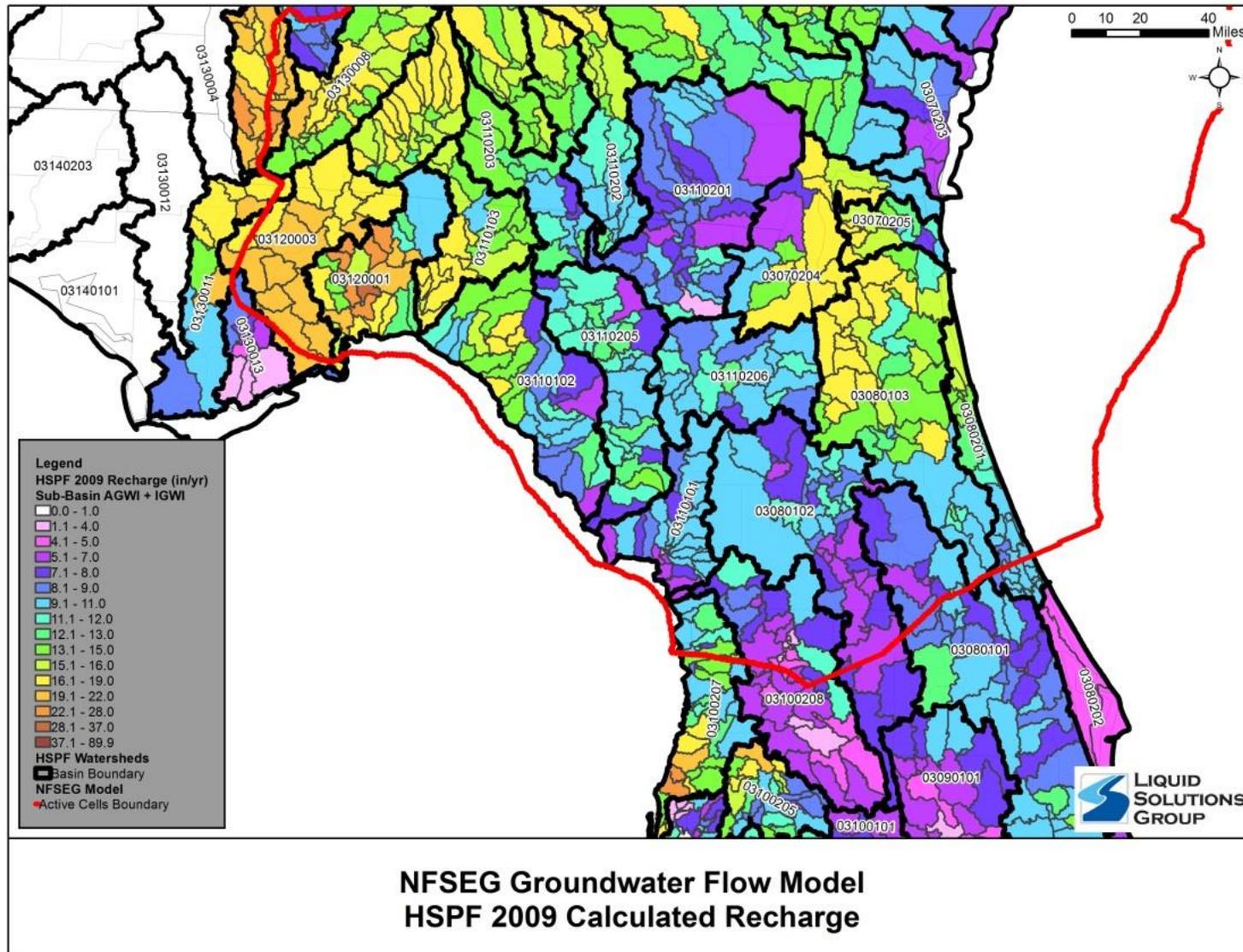
Figure 6 – 2009 MODFLOW Net Recharge
