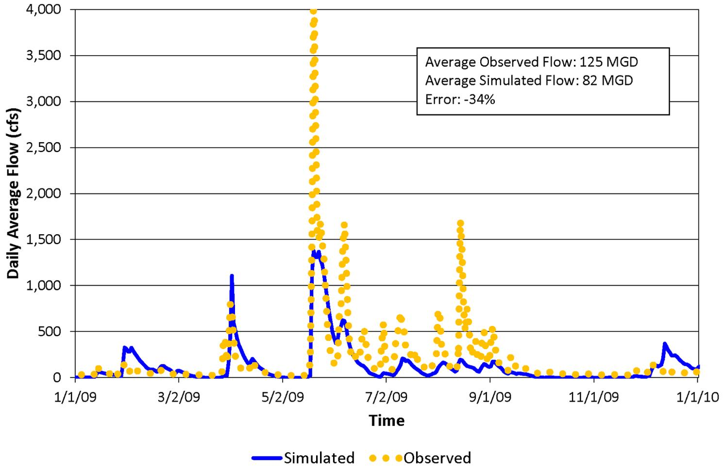
Figure A7 – 2009 MODFLOW Calibration Results
