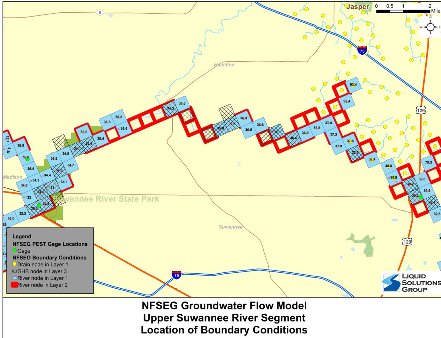
Figure 17 – Hydrologic Boundary Conditions set for the Suwannee River 2
