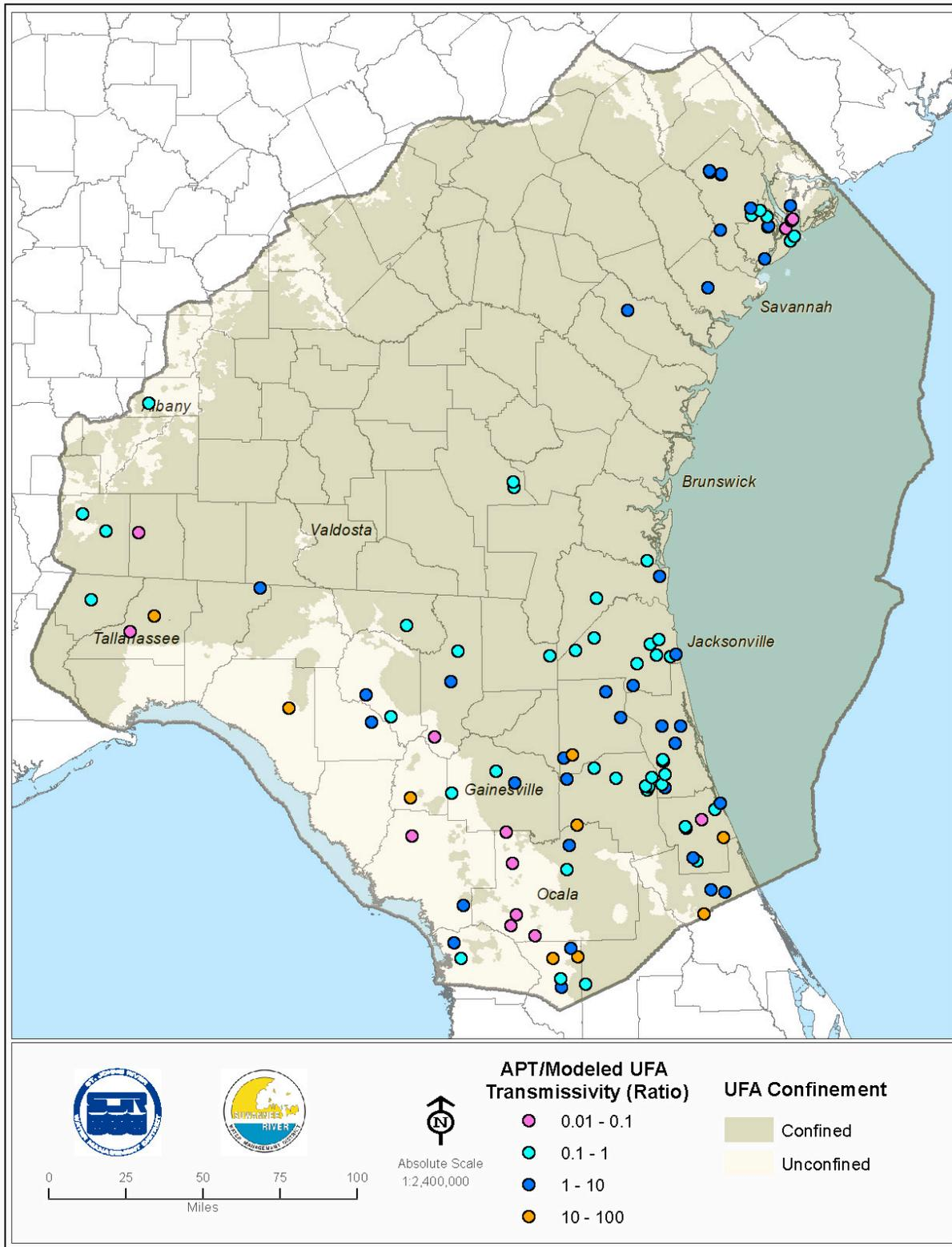
Figure 7. APT/Modeled UFA Transmissivity Ratio
