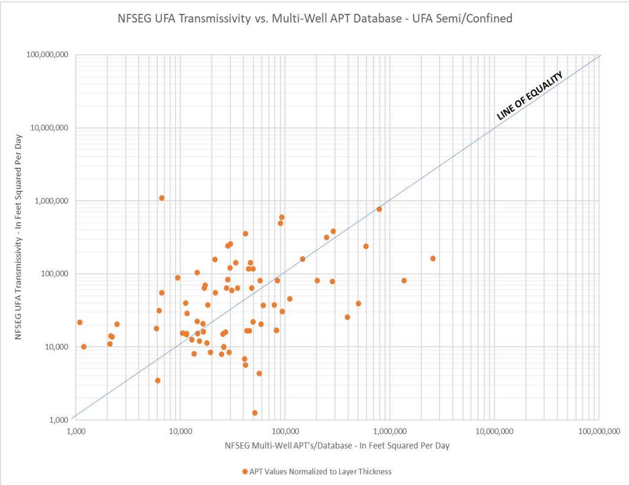
Figure 5. NFSEG UFA Transmissivity vs. NFSEG APT Database – Confined Region
