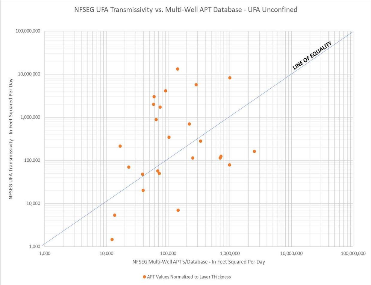
Figure 6. NFSEG UFA Transmissivity vs. NFSEG APT Database - Unconfined Region
