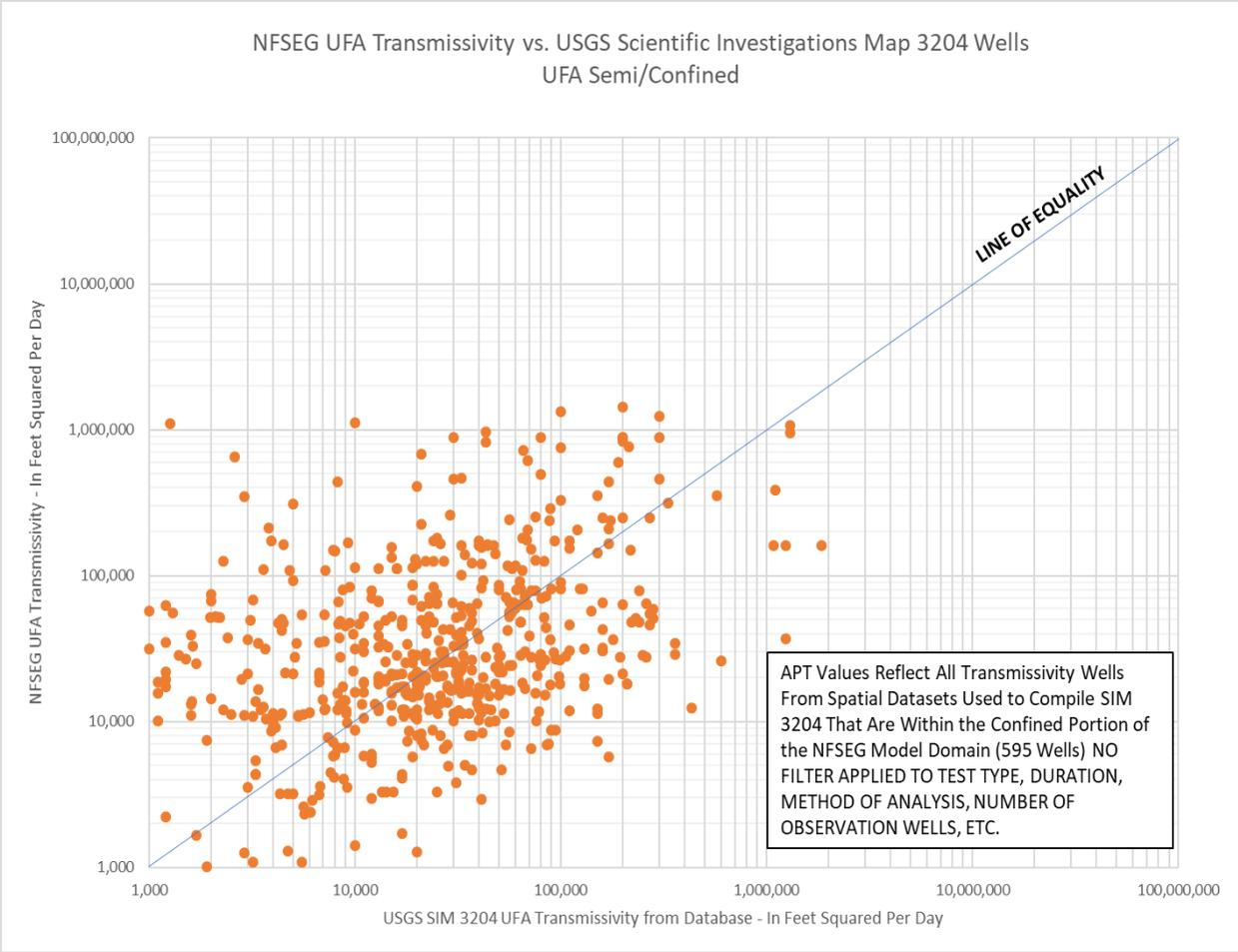
Figure 2. NFSEG UFA Transmissivity vs. USGS Sim 3204 APT Wells – Confined Region
