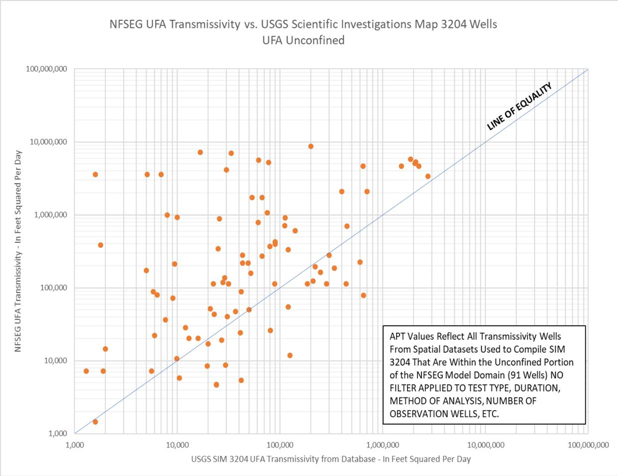
Figure 3. NFSEG UFA Transmissivity vs. USGS SIM 3204 APT Wells - Unconfined Region
