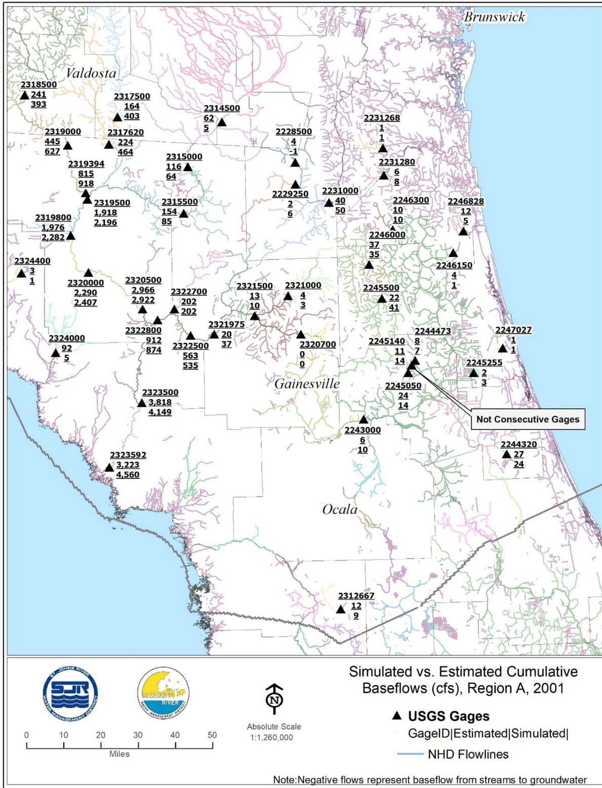
Figure 8. Simulated vs. Estimated Cumulative Baseflows, Region A, 2001
