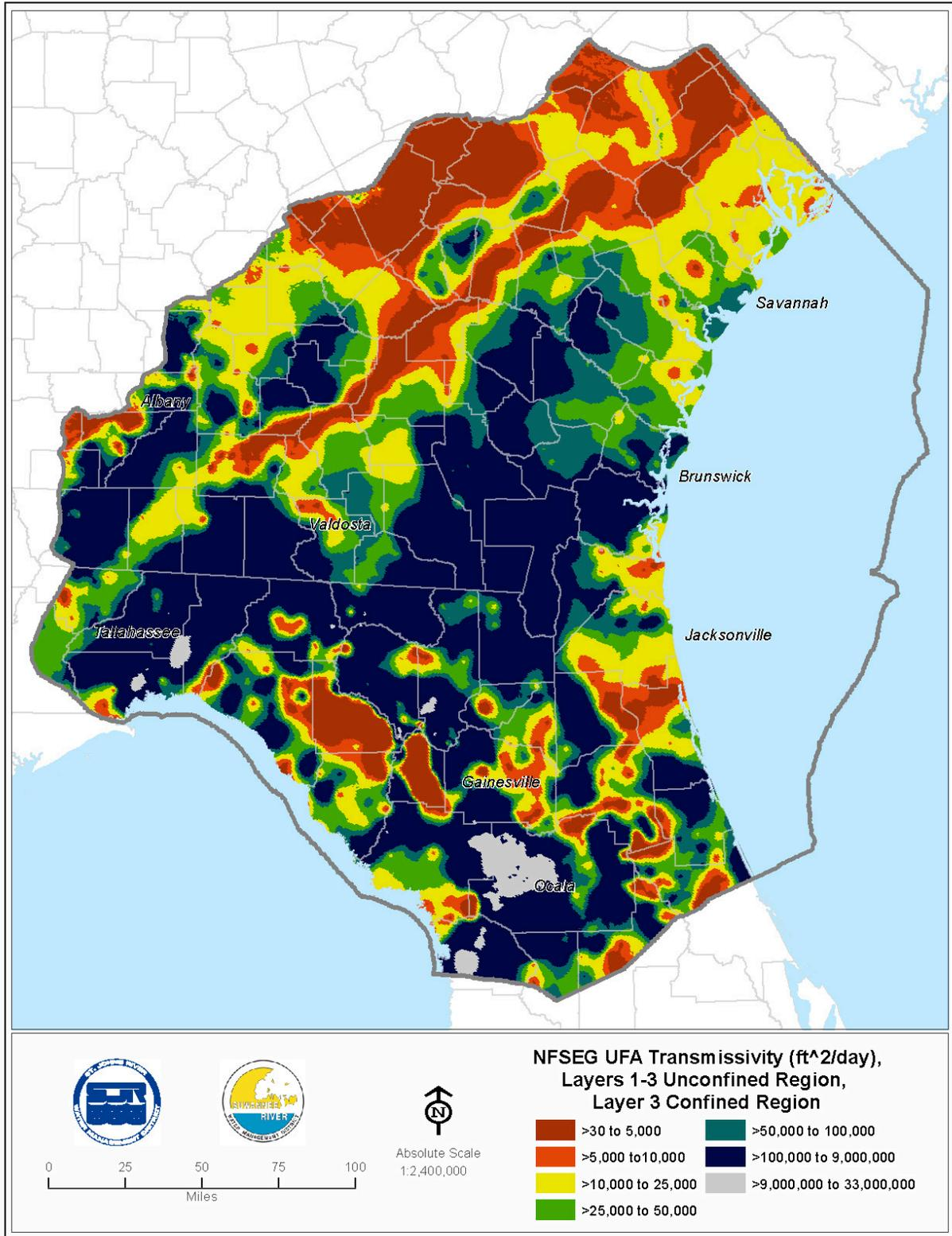
Figure 4. NFSEG V1.1 Modeled UFA Transmissivity.
